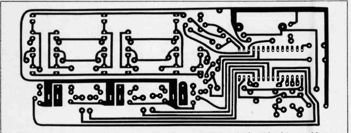
By using this full-sized printed circuit board template you can make your own BCD clock printed circuit board. Any one of the popular photo-etching techniques should work well for this board. Be careful to check the finished board for accuracy and solder bridges.
