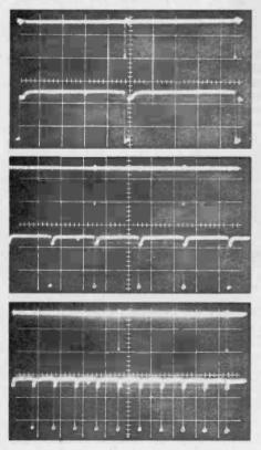
These three oscilliscope photos show the clock signal (top trace) and the resulting marker signal (bottom trace) for 100 kHz, 50 kHz and 20 kHz outputs respectively. brated marker generator. HertzMarker will sound off with a sharp tone each time you tune through a preset band spread on your tuning dial. If you set HertzMarker up for a 100-kHz marker you will, for example, hear a tone five times if you tune from 2000 to 2500 kHz.
