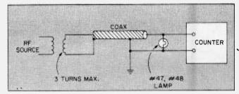
Three turns of number 18 gauge wire is fed by a suitable length of coaxial cable that is terminated in a number 47 lamp. This lamp will act as a 50 ohm termination for the coax. Such a scheme will work at the counter's one megohm or 50 ohm input impedance sources.
