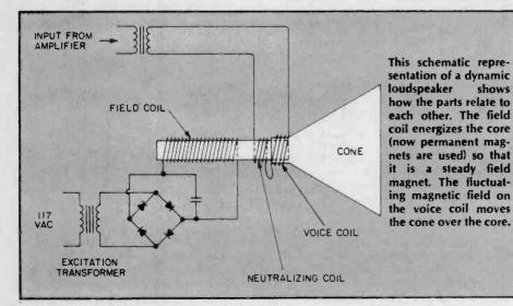
removing the speaker field winding. If you are replacing the speaker in a console radio, you may have room to leave the field coil connected and place the coil in an out of the way spot. Mount the new speaker in the proper place and use the old output transformer with the new speaker. If there isn't room, as in a table model radio, then you can use a small inductor and resistor to get the correct impedance.
