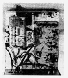
The T-82's tuning capacitor is at top left, and the receiver's PC board at lower right.
