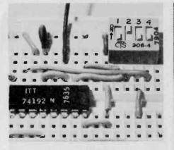
The heart of the circuit is the 74192 IC chip and the DIP switch that controls it.
