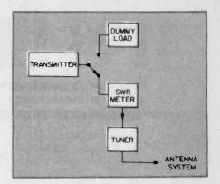
Fig. 6. This shows the basic configuration of the antenna line circuit with antenna tuner and SWR bridge in position on one side, and the dummy load (for tune-up purposes) on the other side of the coaxial antenna switch. See the text for all details.
