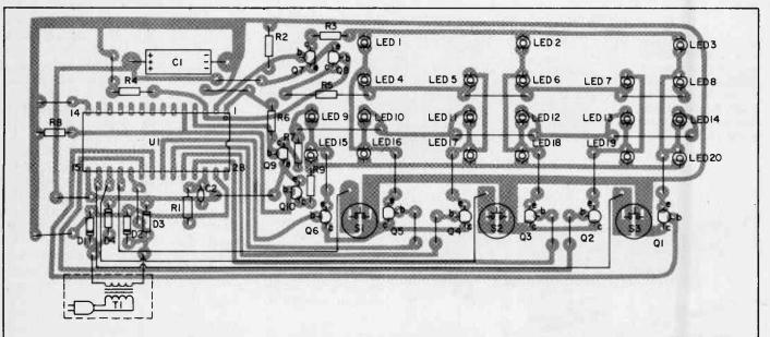
This component location diagram shows where all the parts are located on the printed circuit board. The foil side is down in this view so don't worry about jumpers shorting. Although most LEDs are oriented as shown here, be sure to check the polarity.
