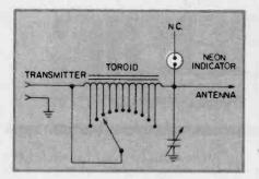
Fig. 3. SST's T1 antenna tuner uses an L network, as seen in example A of Figure 1. The neon bulb shows relative RF transmitter power being fed to the antenna.
