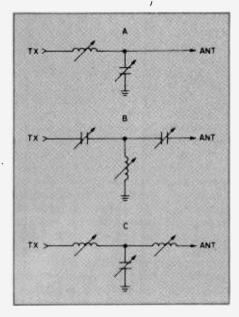
Fig. 1. These are the three basic circuit configuations for antenna tuners. Type A is an L network, B and C are T networks.
