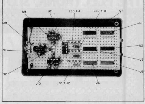
We cut some surplus DIP sockets in half to hold the rows of LEDs. If you don't care to ruin your sockets, wire the LEDs directly to the perfboard, using tie points to raise the LEDs up off the surface of the hoard so that they can protrude through the faceplate.
