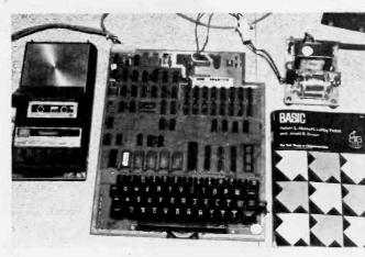
row. You can set the line length anywhere from 16 to 64 characters in length. This is a great feature when using a TV set since you can eliminate the common problem of characters being lost off the righthand side of the picture. The characters are easy to read but, the ROM programmers could have put a bit more vertical spacing between the lines.
