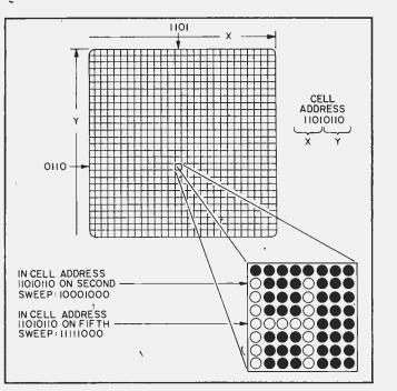
A video terminal screen is divided into thousands of cells which are in turn divided into dots. A cell is called a character matrix. The one illustrated here is an '8-by-8' matrix. The matrix, which is identified by an address, is scanned eight times, once for each row of dots.
