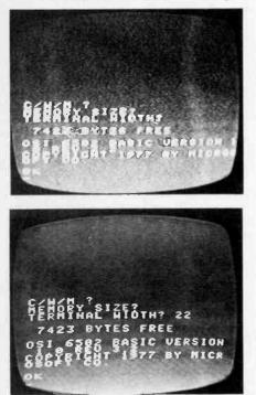
Overscanning, shown in the top photo, is easily cured by setting a shorter terminal width that will fit on the screen being used.
