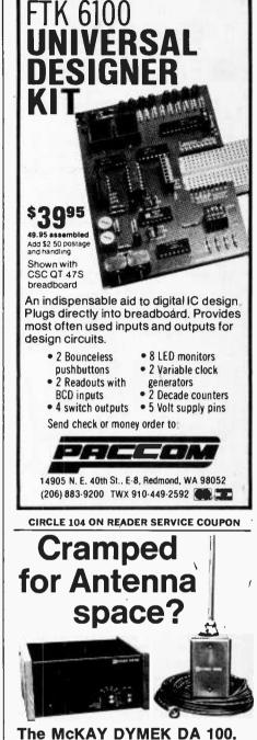
The DA 100 is a compact, wide dynamic range, broadband, untuned, omni-directional receiving antenna covering the frequency range of 50 kHz to 30 MHz. The exterior module, a small weather-proof box with a 56 inch (142 cm) whip delivers the signal to the power supply unit through a supplied 50' coaxial cable.
