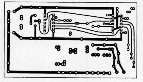
This is the etching guide for the PC board, shown in exact scale. If a project of this magnitude is beyond your abilities, you can obtain a ready-made circuit board from LEC-TROGRAPHIX. Their address and ordering information is shown beneath the parts list.
