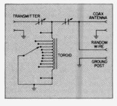
Fig. 2. This is a simple schematic for an antenna tuner showing the tapped inductor, and outputs for longwire and coax-fed antennas. You can see that this is based on example B in Figure 1. This is probably the most popular design for the smaller types of commercial antenna tuners sold.
