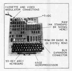
Everything is on one board with room to grow. You might want to build a small case to protect the Superboard II from damage.
