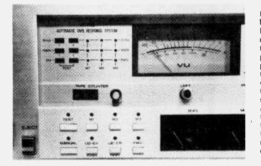
Each tape type can be manually selected, or the parameters for each tape type can be computer-optimized by pressing the Test button. The set of indicators directly aboue the Test and memory selectors (M1, M2, M3) indicate which tests are being run by the computer, also the tape type adjustments are stored in each of the memories cells in a compartment on the rear of the deck. The memory is reprogrammed whenever a *Test* is run.
