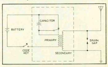
Fig. 2. Marconi's first transmitter, although remarkably similar to Hertz's, had the addition of a grounded spark gap and high antenna.
