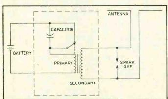
Fig. 1. This is the schematic of Hertz's original spark gap transmitter. There was no key, as it was set to oscillate continuously.
