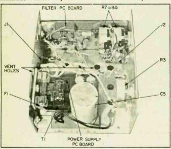
The photo at left illustrates the physical layout of the filter's chassis. It is important that you be sure to drill ventilation holes where indicated, in order to avoid excess heat accumulation by the semiconductors.
