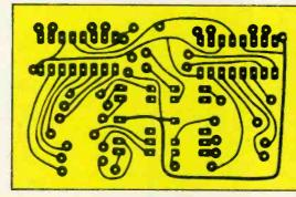
This is the full-scale template for etching the printed circuit used on the display board. Cut the board itself to allow a ½-inch margin around the edges. This is done in order to accommodate different chassis mounting schemes, something which you can decide yourself in later phases of construction.
