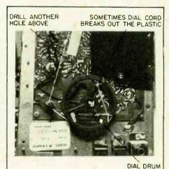
Fig. 9. If the original hole in the drum is broken, simply drill annother hole as close as possible to the location of the original.
