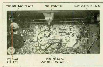
Fig. 3. No matter where the dial cord happens to part, don't waste time trying to tie a knot in the cord. Replace cord entirely with a new one.
