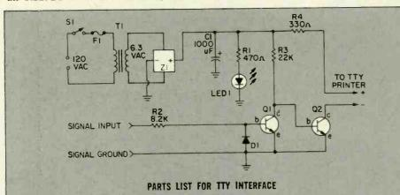
C1-1,000-uF electrolytic capacitor, 25-VDC
