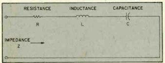
plus reactive components of the circuit. Coils and capacitors determine the magnitude of the reactance of a given circuit. It is beyond the scope of this article to deal in depth with the problem of complex impedance, but some knowledge is necessary for an understanding of voltage measurements.
