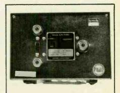
The rear panel switch allows selection of a dummy load for tuneup purposes.
