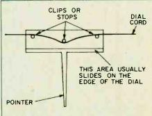
Fig. 6. A drop of plastic cement placed on the stops of the dial pointer will usually prevent the pointer from slipping around.
