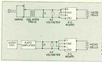
There hare two acceptable methods for calibrating the meter. The top diagram shows house current as a source, with an AC voltmeter in parallel with our meter for reference. At bottom, an AF generator is used as the AC current source.
