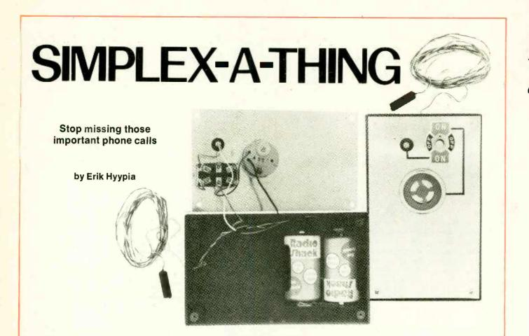
YOU WON'T MISS any more phone calls when out of hearing range of your telephone, if you add this simple remote signalling unit which alerts you to incoming calls by means of either a buzzer or blinker light. The unit is self powered for easy placement in any room in your home, or even outdoors where there are no AC outlets.
