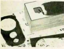
Paint the front panel, grill frame and back panel with the black latex paint—two coats.
