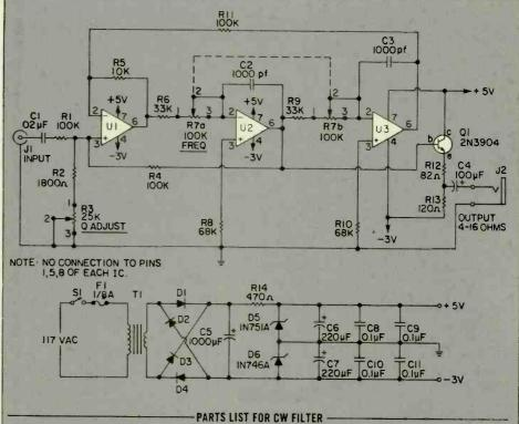
C1-0.02 uF ceramic capacitor, 15 VDC
