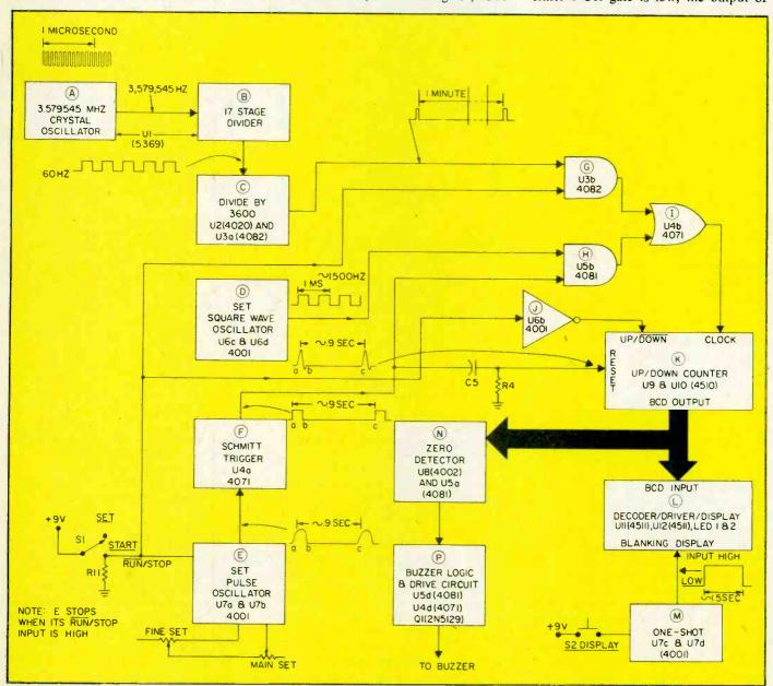
This block diagram depicts the flow of signals within CRYDIT. We have included the waveforms and time bases as well here to help relate the functions to the technical explanation which you will find in the text. This diagram can also serve as a troubleshooting guide (if you have an oscilloscope), allowing you to intercept the signals at various points and to compare with the specs.
