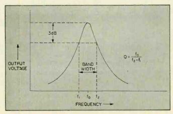
Fig. 1. Above is a sample graph depicting the bandpass curve for a theoretical filter derived from the formula at the left of the graph. This formula demonstrates the manner in which "Q" derives.
