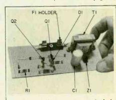
Breadboard offers the easiest method of construction for the TTY Interface.
