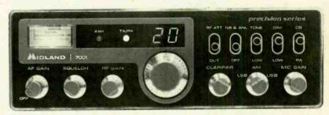
The 1980s will be the era of high technology in CB as well as other forms of radio communication. The Midland 7001 has an advanced SWR indicator, bright green fluorescent LED readout, and combines AM and SSB operation in the same space as an old 23-channel AM rig.
