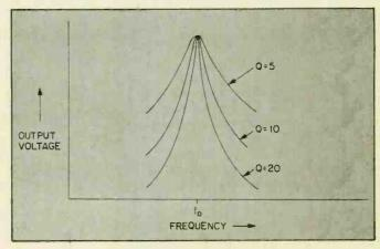
Fig. 2. The higher the "Q" value of the filter, the narrower the bandpass frequency width will be. Obviously, a filter with a "Q" value of 20 will exhibit a narrower width than one with a "Q" of 5.
