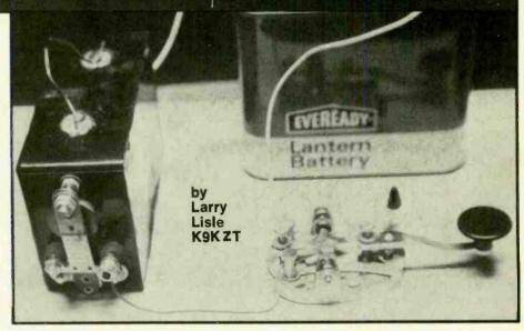
The contacts of the interrupter would then close as the magnetism of the core subsided and the cycle would repeat, usually 10 to 50 times per second.
