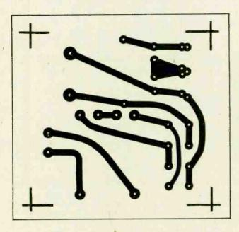
The etching diagram for the power supply PC board is shown at left. As with the filter board, allow room along the edges for drilling holes for the chassis mounting screws. There should be room for drilling holes (if needed) to secure the power transformer to the board.
