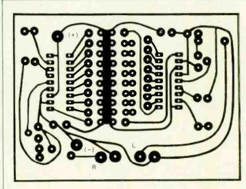
This is the full scale etching guide for the printed circuit board, seen foil side up. Check your finished board carefully for foil bridges and other errors.
