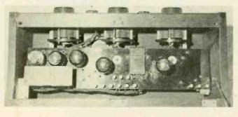
This interior view of the Federal shows the clean, rugged construction. The 3 small terminals at the lower right of the chassis are antenna and ground connection points.
