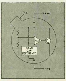
Here is an internal schematic of the band gap zener diode, which serves as the heart of the calibrator. Use the tab on the case as the reference point for making circuit connections. No heatsink is required here. Where:
