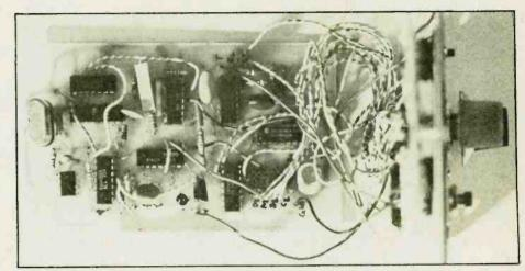
The photo above shows the assembled main board swung away from the chassis. Almost all of the wiring used to interconnect the two boards leaves from the right hand side, which allows plenty of flexibility and accessibility in assembly and checkout, if needed.
