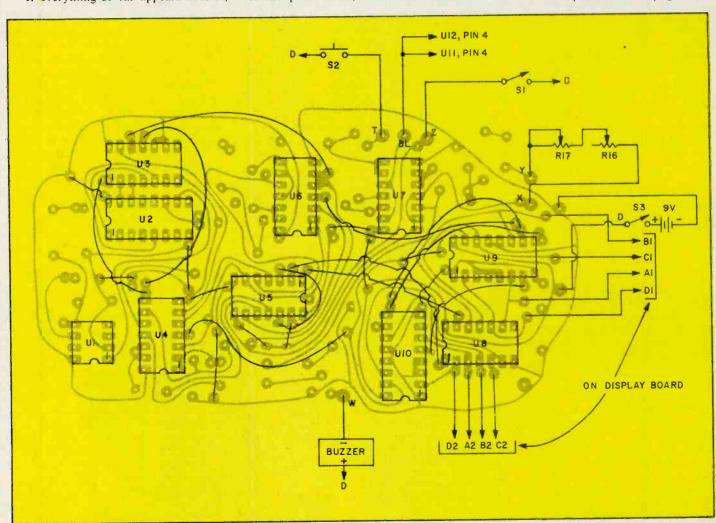
The jumper location diagram above also includes the wiring connections for the remainder of the off-board components, as well as the interconnections between it and the display circuit board. Point D at S3 is a junction for several connections (hot side of buzzer, hot side of S1 and S2). Simply attach all incoming leads to the terminal on the switch back (switch S3) after mounting.
