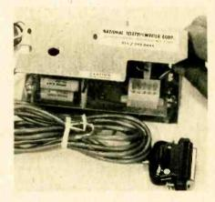
Fig. 1. The complete conversion kit, including both wiring harnesses and connectors.
