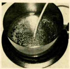
Allow 5 minutes in bolling water to compensate for thermal inertia in the diode.
