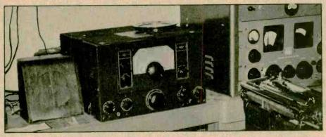
This National Radio Corporation long wave receiver dates from the 1930s. Sets like this one were used aboard ships and at coast stations to monitor distress calls and ship-to-ship traffic on the low-frequency bands below 500 Kilohertz reserved for these purposes.
