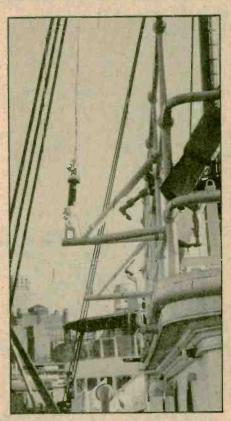
The 40 meter antenna line feeds from the transmitter, through the port bulkhead via an insulated fitting, and up the after mast. The Brooklyn skyline is in the distance.
