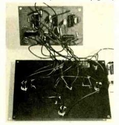
Board to panel connections and wiring of FasTouch. There's a lot of wiring, so be sure that you keep track of it all, and are careful.
