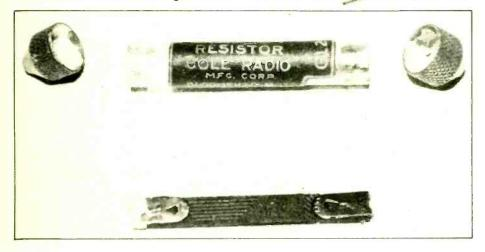
These parts make up one type of old grid leak. The grid leaks in use during the early days of radio tended to vary from 100,000 ohms to 10 megohms. While purists will insist on accurate restorations or replicas, a 500,000 ohm, 1/2-watt resistor is as good.
