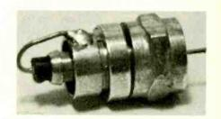
If you get "ghosts" from unused splitter outputs, make up terminations from F-type connectors and 1/2-watt carbon resistors.
