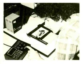
Here the PT-1500 is being programmed to time an enlarger exposure. There is an AC outlet on the back for switching the enlarger on and off.
