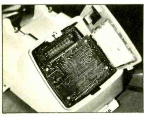
Intelli-Phone with its front dial plate off. You're looking at the nine-digit fluorescent display, and the foil side of the PC board. Circle R. S. number 80.
