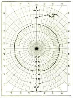
Fig. 5A. In practice, the ellipsoid of Fig. 5 becomes an irregular circle (omnidirectional), but the emitted radiation pattern is still a useable one.
