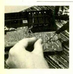
Cracked PC Board. You may find a cracked PC board after careless handling or after an accident. When the calculator is accidently dropped or knocked around, check for broken wiring connections or a cracked PC board. In one particular instance, a pocket calculator was accidently dropped upon the cement floor of a garage and the cover accidently run over by a car. The only damage incurred was a broken corner of the cal-
