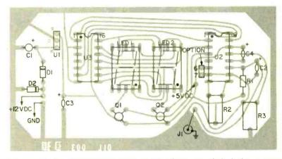
Parts layout for the Digital Oil Pressure gauge. There are relatively few components to worry about, those that there are, are relatively well-spaced. VCR's on other side.
