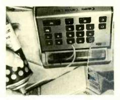
come tax, adding today's enormous sance when trying to figure your ina soft cloth. Sticky buttons are a nui-Wipe off all excess oil or cleaner with up all the buttons while you're at it. until it is free. You might as well clean well. Work the button up and down A drop or two of light oil will work as cleaner down around the buton area.
