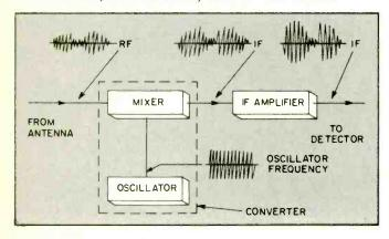
The IF Amplifier—The abbreviation for intermediate frequency is IF. In most home receivers the IF is 455 kHz. Amplifying a single frequency in the IF circuit is much easier and causes less distortion than if it were necessary to tune this amplifier to each of the many station frequencies. The only purpose of this stage is to amplify the IF (which still retains the original audio frequency) and pass it on to the detector.
