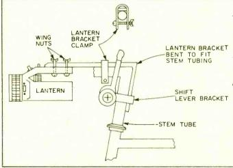
The entire Bike Light assembly bolts onto a bracket and is easily removable by loosening two wing nuts. The bracket is held against the bicycle's stem tubing with a Uclamp. DO NOT DRILL through the frame, since this may seriously weaken it, possibly causing injury to the rider and machine.
