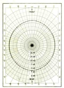
Fig. 5. The ideal radiation pattern for 1/8-wavelength spacing of elements results in a fat ellipsoid. It's strongest front to back.
