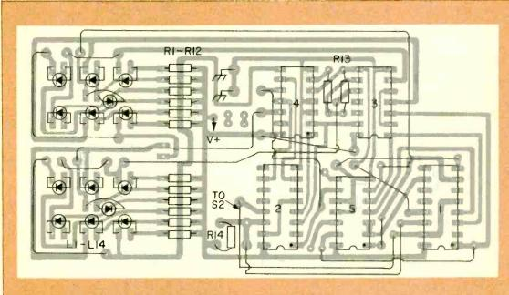
The parts overlay diagram shows the placement of components on the PC board. As in all projects using a number of delicate ICs care must be taken with the pins and with the use of soldering irons too near to the chips. Digi Dice is a project to gladden a gambler.
