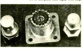
The most commonly used coaxial connectors are, from left to right, the BNC, SO-239 and F-type. These cover nearly every coax use.
