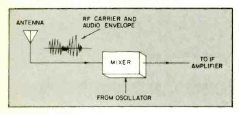
In CB sets the frequency to which the oscillator is tuned is often two to 11 MHz above (or below) the incoming RF carrier frequency, instead of 455 kHz.
