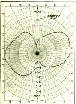
Fig. 3. A co-phased array utilizing 1/2-wave radiators spaced 1/8-wavelength apart will give a radiation pattern similar to this. This is not a particularly effective pattern for mobile use, as the maximum amount of energy is radiated off the sides of the array instead of front and back as is needed for road usage.
