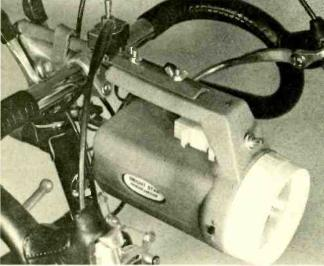
When the Electronic Bike Light is mounted between the handlebars, all controls are in easy reach. Whether in the rest position or "down on the grips," the rider has access to everything. This allows instant response in all bicycling situations.
