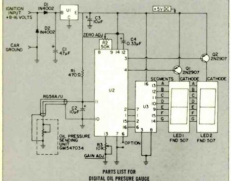
C1—47-uf, 25-VDC electrolytic capacitor C2, C3—10-uf, 16-VDC tantalum capacitor
