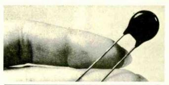
Metal oxide varistors are installed across AC power lines, protecting against line transient surges caused by lightning hitting a nearby power line.
