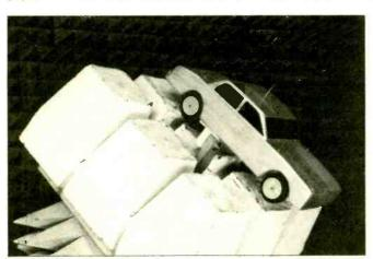
Fig. 1. In a special, non-reflective RF testing chamber, NASA technicians are able to measure the effects of antenna placement on a vehicle using a reduced scale model and appropriate harmonics.
