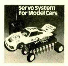
A complete receiver and servo controller on one chip, EXAR's XR-2266 can receive and act on all commands necessary to control every function of this radio-operated model car, even to turning on the directional signals and back up lights. It may be the heart of next year's Christmas best setlers.
