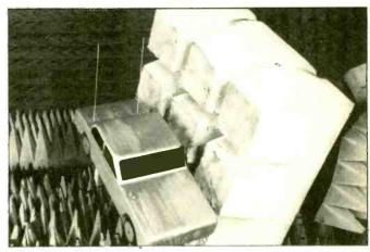
Fig. 1A. In this test, co-phased trunk-mounted monopoles are used to simulate 30 MHz (roughly the CB band) signal patterns. Due to the 1/10 scale, a frequency of 300 MHz is fed to the antennas.
