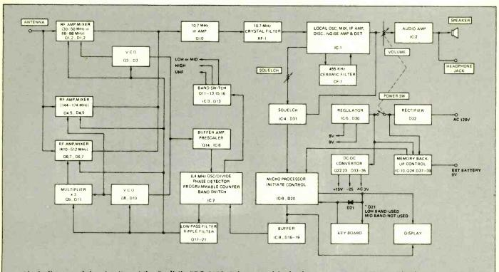
Block diagram of the circuitry of the Realistic PRO-2008. Take a good look—there are separate RF Amplifier/Mixer circuits for each band, and two VCOs (Voltage Controlled Oscillators). There is a crystal filter in the first 1F, and a cermic filter in the second 1F. A lot of careful planning has gone into the design and production of this scanner—and this block diagram reflects it.
