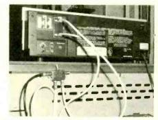
The DPDT switched splitter is attached to the main TV set. Note the wiring layout.
