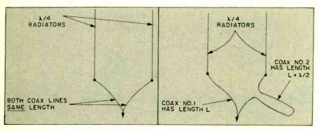
Fig. 2. Configuration depicts a co-phased array using equal length feed lines to obtain a 0-degree phase relationship.
