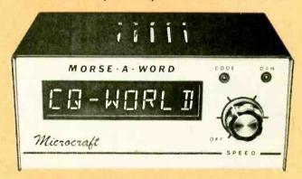
The "Morse-A-Word" by Microcraft is a CW only reader with eight digit LED display. Like all CW readers, it works best with a good fist on the other end. Circle no. 71 on the R.S. Coupon.
