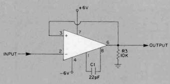
Fig. 2B is the amplifier circuit design most commonly used with the RCA BiMos. It saves space, is more flexible in organization.
