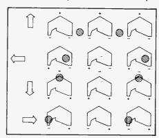
Fig. 3. By applying a rotating magnetic field, bubbles can be made to move. To be useful bubbles must be totally manipulated.
