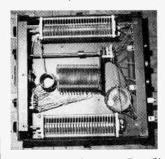
This inside view of the Versa Tuner IV shows rugged coils that let unit take 2KW.
