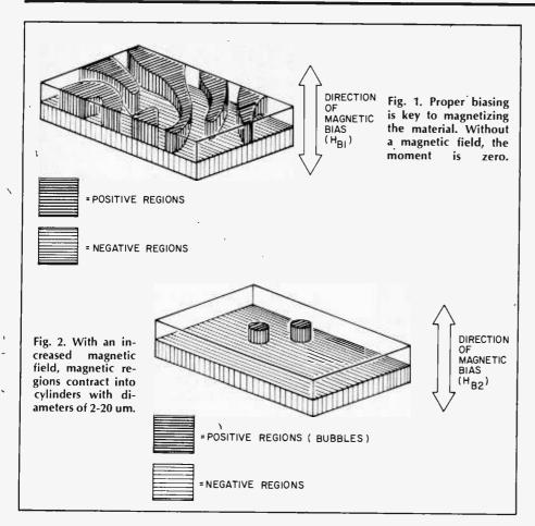
field coils is energized, the bubbles move simultaneously, in order, through predetermined paths in the crystal structure.
