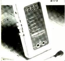
B&K-PRECISION's new 2845 is a major advance in digital multimeter technology. At a price comparable to ordinary manually operated units the 2845 brings microcomputer intelligence to a handheld portable DMM. When applied to a circuit, its computer selects the range providing maximum resolution without the slow "hunting" action characteristic of many bench-type autoranging DMMs.
