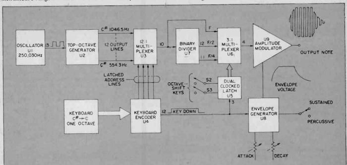
Fig. 1. Starting with a 250,030 Hz oscillator, 12 notes are generated. By using a binary divider and a 3:1 multiplexer, 36 possible frequencies can be retrieved from the Digital Clarinet. Attack, decay, sustained and percussive commands are channeled through the envelope generator to the amplitude modulator. A keyboard encoder sorts out the notes that will be played.
