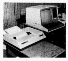
The H-14 can be connected to the H-89, H-8, H-17 or H-19 computer systems. The H-17 operates at Baud rates of 110 to 4800.
