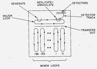
Fig. 5. This is a block diagram of the major/minor loop organization of Texas Instruments' TIB0203 92 kbit bubble memory. For reading, data is transferred from the minor to the major loops.
