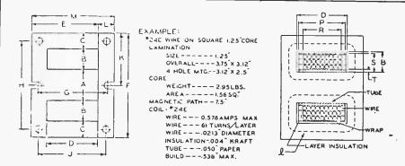
As noted in the text, many transformers have an E shaped and an I shaped piece of steel that forms the transformer body. Insulated copper wire surrounds the center post.
