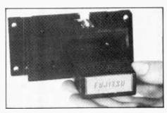
Bubble memory storage is compact and easy to handle. Many units, such as this Fujitsu are just plugged into various hardware.
