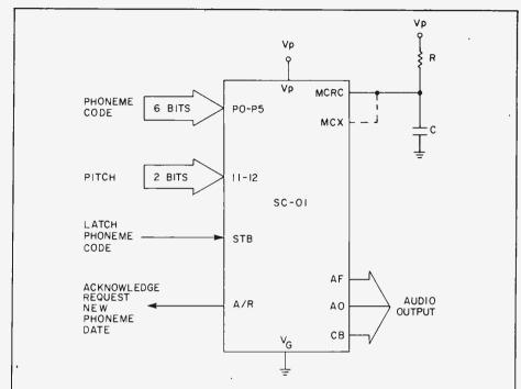
Fig. 1. This flow diagram of the Vortrax SC-01 chip illustrates the complexity of this talking IC. Phoneme, pitch, latch and other codes are used to get a good audio output.
