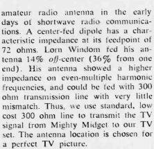
Our Mighty Midget has one advantage over Windom's design: Because of the high frequencies involved, our antenna has very thick elements compared with their lengths. This results in wideband performance.
