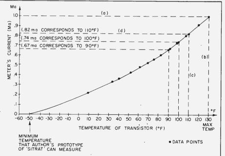
This is the graph that you will need to calibrate the temperature reading meter scale. Make a couple of trial runs on graph paper until you get the knack of drawing smoothly.
