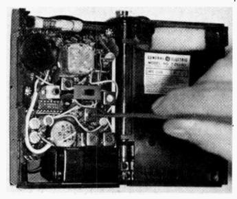
bands on either side of the carrier frequency, as far away as 75 KHz. Such a wide bandwidth in the IF stages of an FM receiver cannot be attained by tuning each stage to the same frequency. What is done is to stagger tune each stage, so that the resultant overall response has the required bandwidth. Note that each IF transformer
