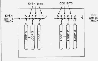
Fig. 6. The data storage area is divided into odd and even storage banks.
