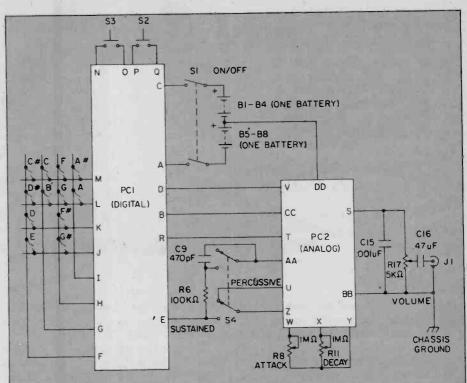
Fig. 2. The various notes that are generated by the Digital Clarinet are created by PC 1. The other controls work out of the analog printed circuit board, PC 2.
