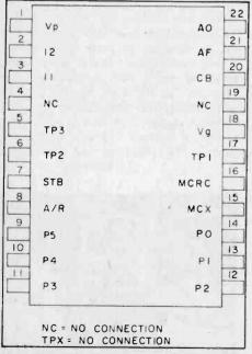
Fig. 2. This shows the placement of each pin in the Vortrax SC-01. P0-P5 are the phoneme command points. 11-12 give the electronic word tones or inflections. Input STB controls latching. AF, AO and CB are audio outputs. MCX and MCRC are timing controls. A/R acknowledges receipt of phoneme data.
