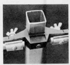
Sturdy wing nuts are utilized to hold and allow for easy removal of the TV wire.
