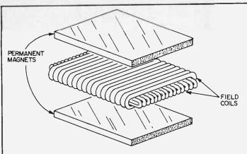
Fig. 4. Field coils and permanent determine the direction of the bubbles as they move. Thus, a serial shift register is created.
