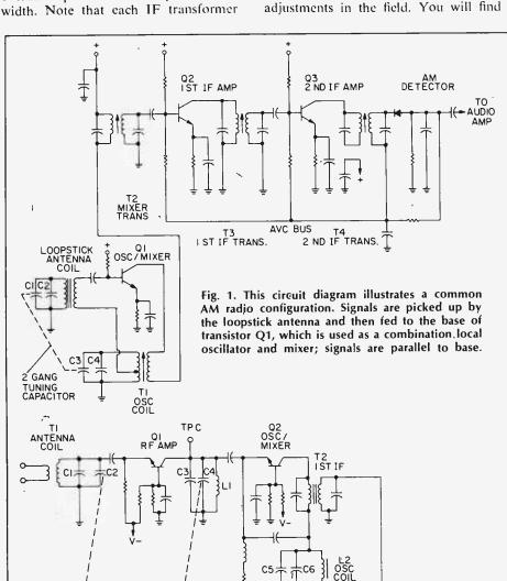
Fig. 2. While there are similarities between FM and AM circuitry, the most obvious difference shown in this FM circuit schematic is an RF amplifier stage to boost signals.
