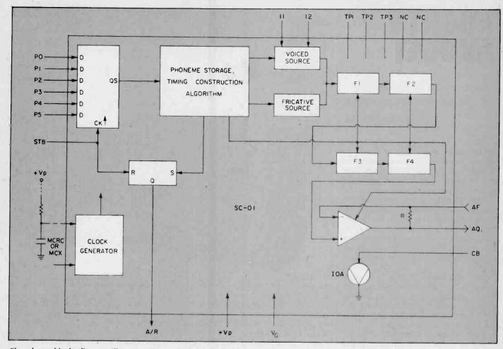
The above block diagram illustrates the various interconnections in the Vortrax SC-01 speech synthesizer chip. Through a very complicated process, electronic commands are sorted, amplified and given tonal characteristics. The chip emits a versatile voice,
