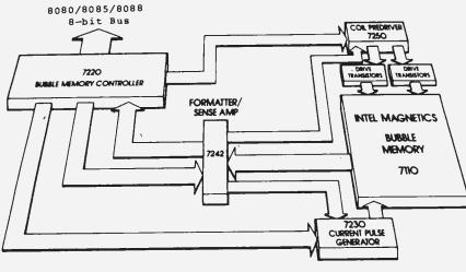
Fig. 7. Support large scale integration (LSI) circuits available with the Intel 7110 megabit bubble memory chip turn the memory module into a complete storage system.
