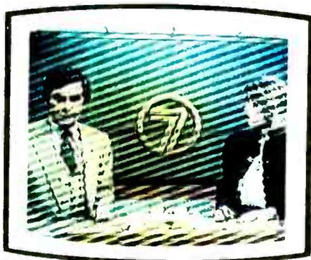
This pattern may appear on your television screen when your set is receiving signals from a CB, amateur, police, or other two-way radio transmitter. The pattern will only appear when the operator transmits. It may vary according to the type of signal being received. You may also hear the operator's voice.
