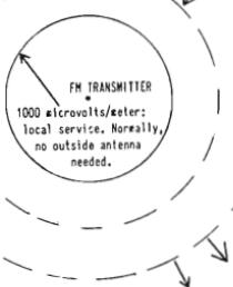
accompanying diagram shows the relationships among the different coverage contours and the general quality of receiving system needed to obtain good reception in each zone. To calculate coverages for a given station, use the FCC FM coverage chart in the Appendix, making reference to the power and height data given in the first part of the Station Directory.
