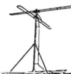
Undoubtedly, the best FM antenna installations consist of some variation of the yagi, which is a high-gain, directional antenna that must be precisely pointed at the desired station in order to get optimum reception.
