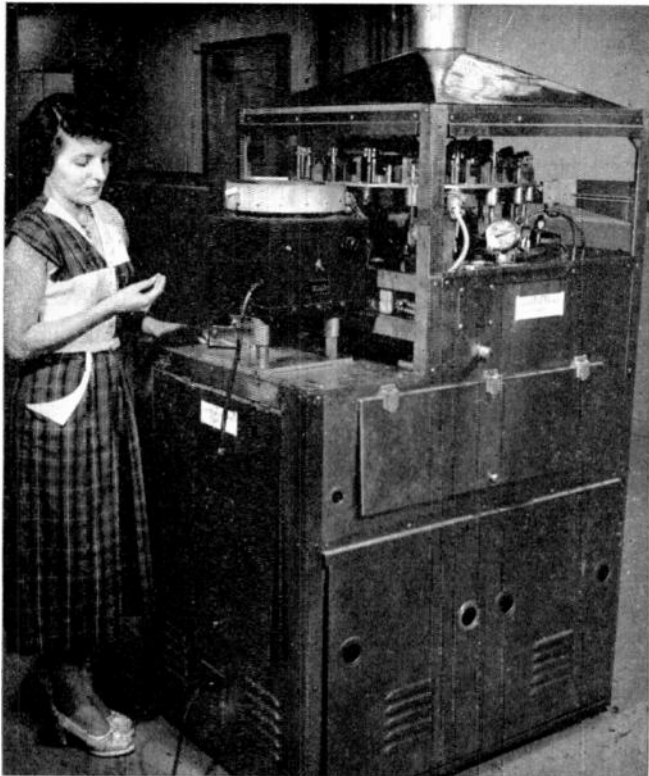
FIG. 10. ONE OF THE AUTOMATIC FACTORY'S SURFACE TINNING MACHINES
