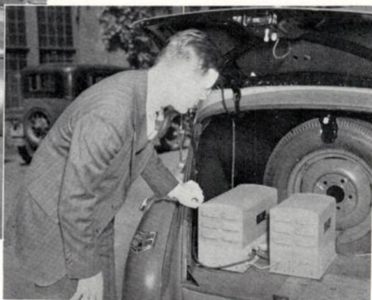
G.E. TRANSMITTER UNIT 4GFA1, LEFT, AND RECEIVER 4SFJA1, COMPLETELY INSTALLED IN CAR, AND READY TO OPERATE
