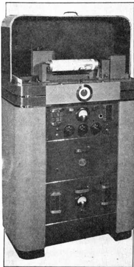
FIG. 2. TRANSMITTING SCANNER AND AMPLIFIER FOR STUDIO OPERATION
