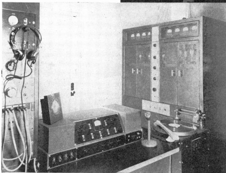
VIEWS OF FINCH SOUND-FACSIMILE BROADCASTING STATION. ABOVE, 1-KW. FM TRANSMITTER AND SCANNER
