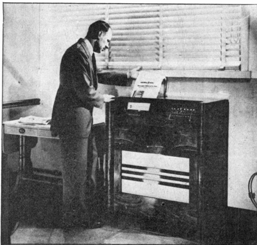
FIG. 3. A SPECIAL RCA MODEL HOME RADIO RECEIVER AND FACSIMILE RECORDER
