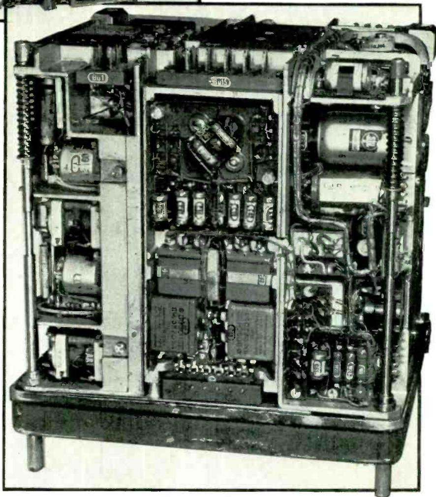
parts in this equipment were made in that way except for the front of the set, which seems to be an aluminum stamping. The use of die-castings is another feature around which the assembly was designed. The castings are amazingly complicated, and some require draws in four directions. Just how intricate they are can be seen from the illustrations.
