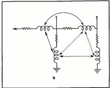
FIG. 3. ILLUSTRATING MUTUAL INDUCTANCE BETWEEN ELEMENTS OF ATTENUATOR
