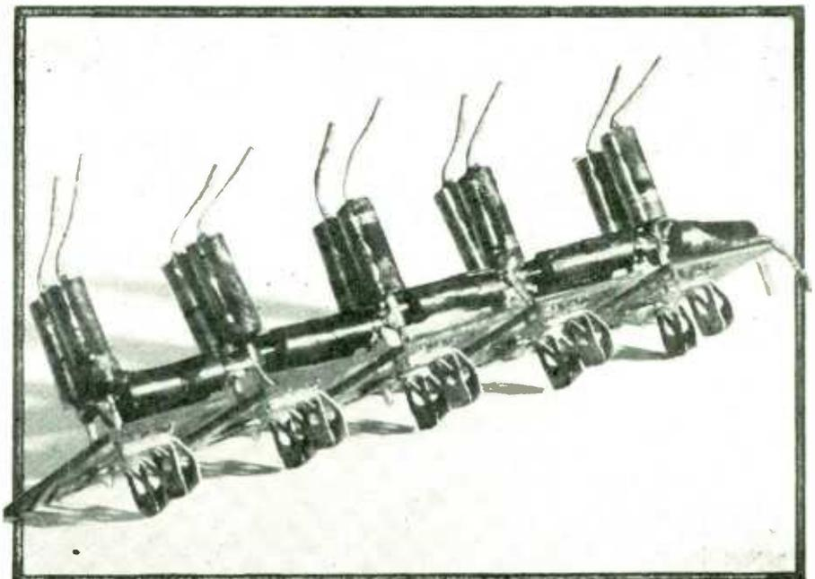
FIG. 11. COMPLETE SET OF SERIES AND SHUNT RESISTORS MOUNTED WITH THEIR SILVER LEAF SPRINGS FOR GROUNDING THE SWITCH DRUM ILLUSTRATED IN FIG. 12
