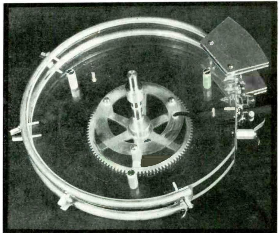
FIG. 5. RESONANT CIRCUIT COMPRISING PARALLEL RODS, CONDENSER PLATES, AND OSCILLATOR TUBE, AT RIGHT, DESIGNED AS A ROTATABLE MECHANICAL ASSEMBLY
