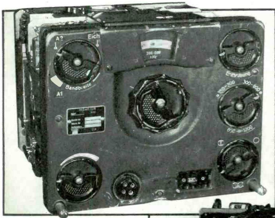
FIG. 1. CAPTURED GERMAN AIRCRAFT RECEIVER, WITH COVER REMOVED
