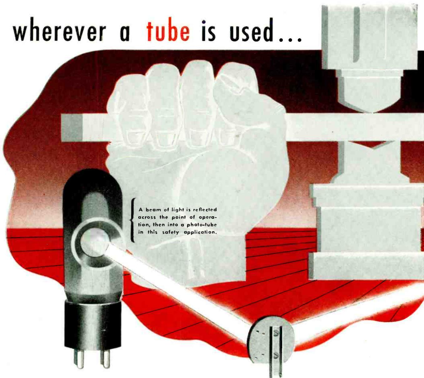
A beam of light is reflected across the point of operation, then into a photo-tube in this safety application.
