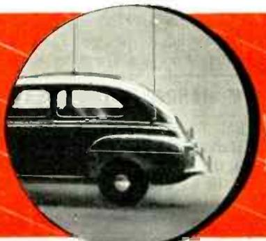
6. Mobile Antenna: Furnished with FM mobile transmitters shown above. Two models, one for roof-top, the other for fender mounting. Simple one-hole mounting. Supplied complete with connecting coaxial line.
