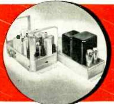
4. 60-Watt FM Station Transmitter: Uses same chassis as #5, but is furnished with chassis brackets for rack-mounting. A.C. power supply is a separate chassis unit. Not furnished for shelf-mounting.
