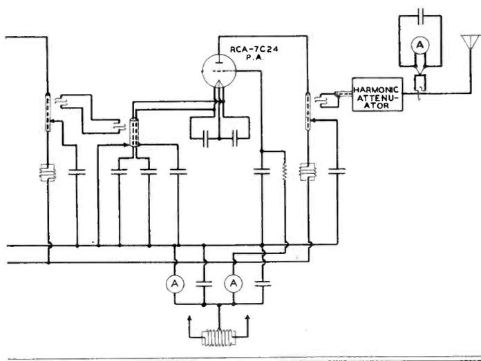
FIG. 14. COMPLETE CIRCUIT OF THE 3-KW. RCA FM BROADCAST TRANSMITTER. THE LOWER DIAGRAM IS A CONTINUATION OF THE OUTPUT OF EXCITER, WHICH TERMINATES IN A COAXIAL LEAD AT THE RIGHT, ABOVE. CIRCUIT OF THE SPARE EXCITER IS A DUPLICATE OF THAT SHOWN HERE, AS INDICATED IN FIG. 7, LEFT
