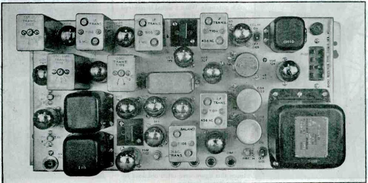
FIG. 7. TOP VIEW OF THE RECEIVER CHASSIS, USED WITH THE 50-WATT AND 250-WATT TRANSMITTERS
