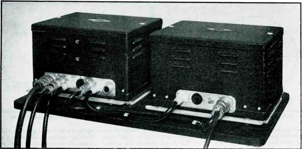
FIG. 11. COMPLETE MOBILE TRANSMITTER AND RECEIVER FOR EMERGENCY SERVICE ON THE 72- TO 76-MC. BAND
