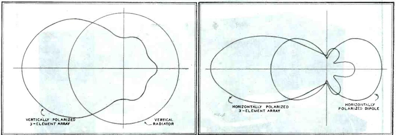
FIGS. 8 AND 9. COMPARISONS OF RADIATION PATTERNS OF VERTICALLY AND HORIZONTALLY POLARIZED ANTENNAS
