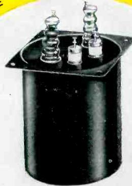
Typical of the special units produced by UTC is this high gain, 100 cycle, matching transformer. Primary impedance 500 ohms, secondary impedance 37,500,000 ohms, shielding suitable for -160 DB signal level.
