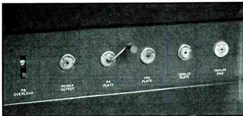
FIG. 13. REMOVABLE CRANK IS USED TO ADJUST THE CIRCUITS
