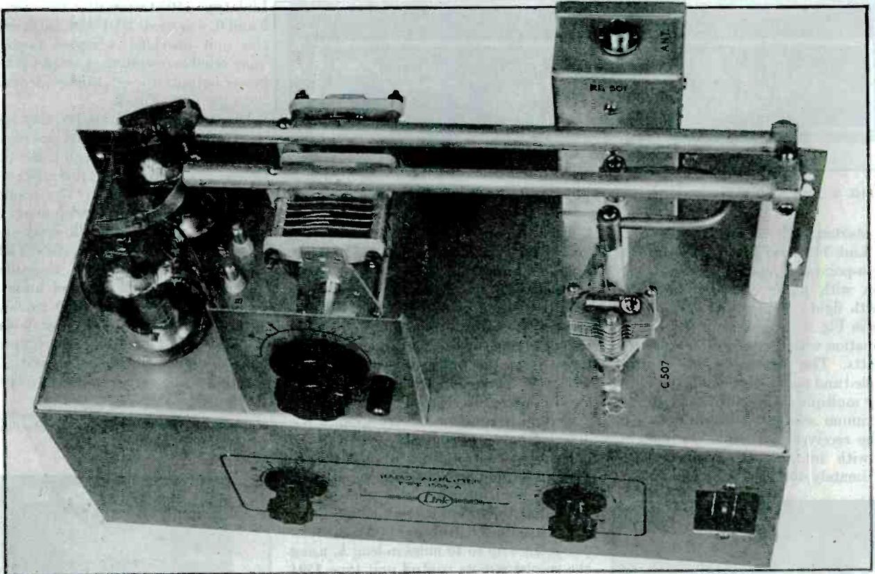
FIG. 6. OUTPUT STAGE OF THE 250-WATT TRANSMITTER, SHOWING THE ARRANGEMENT OF THE 251B (4E27) TUBES
