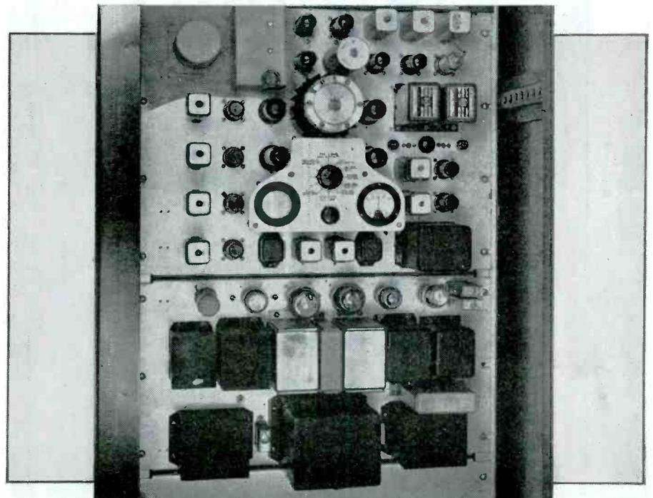
FIG. 6. EXCITER ASSEMBLY, RF AND MODULATOR CIRCUITS ABOVE, POWER SUPPLY BELOW
