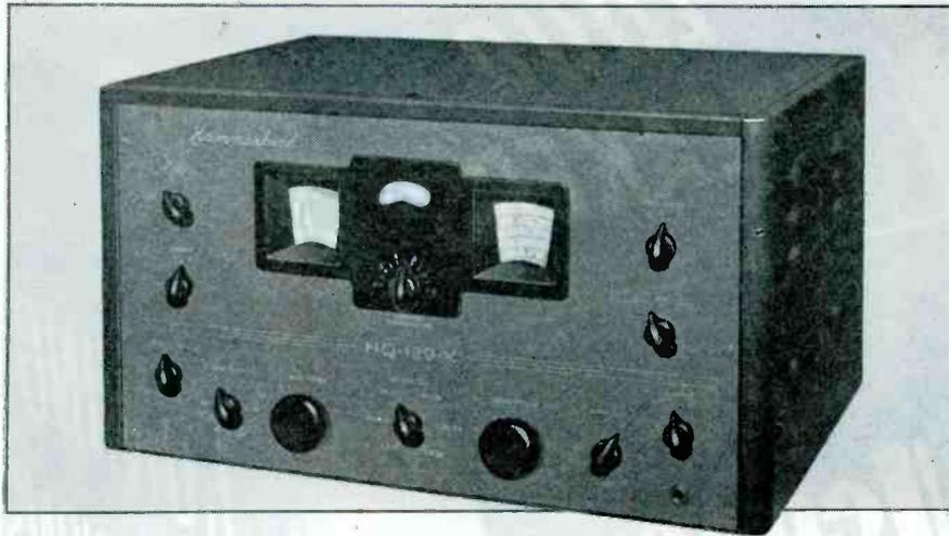
FIG. 1. HAMMARLUND COMMUNICATIONS RECEIVER FOR .54 TO 31 MC.
