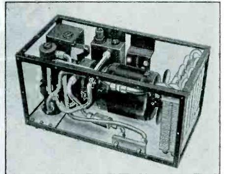
FIG. 4. HEAT DISSIPATING UNIT FOR COOLING POWER TUBE EQUIPMENT
