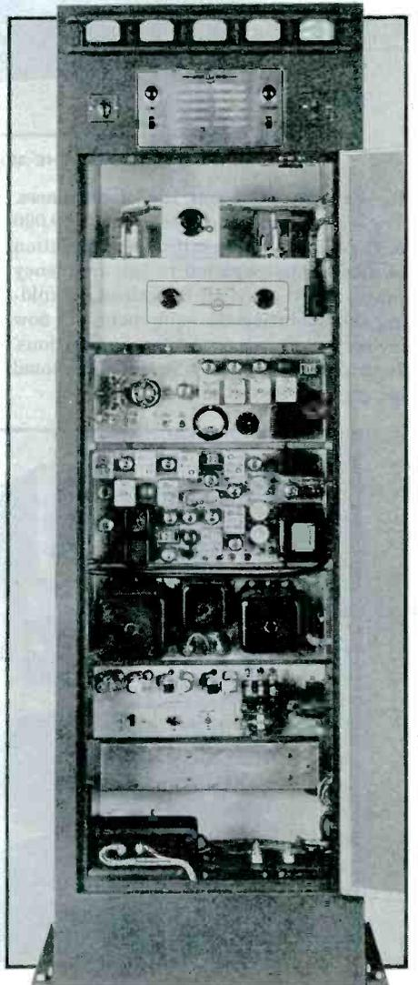
FIG. 5. THE 250-WATT TRANSMITTER AND RECEIVER UNIT FOR 72 TO 76 MC.
