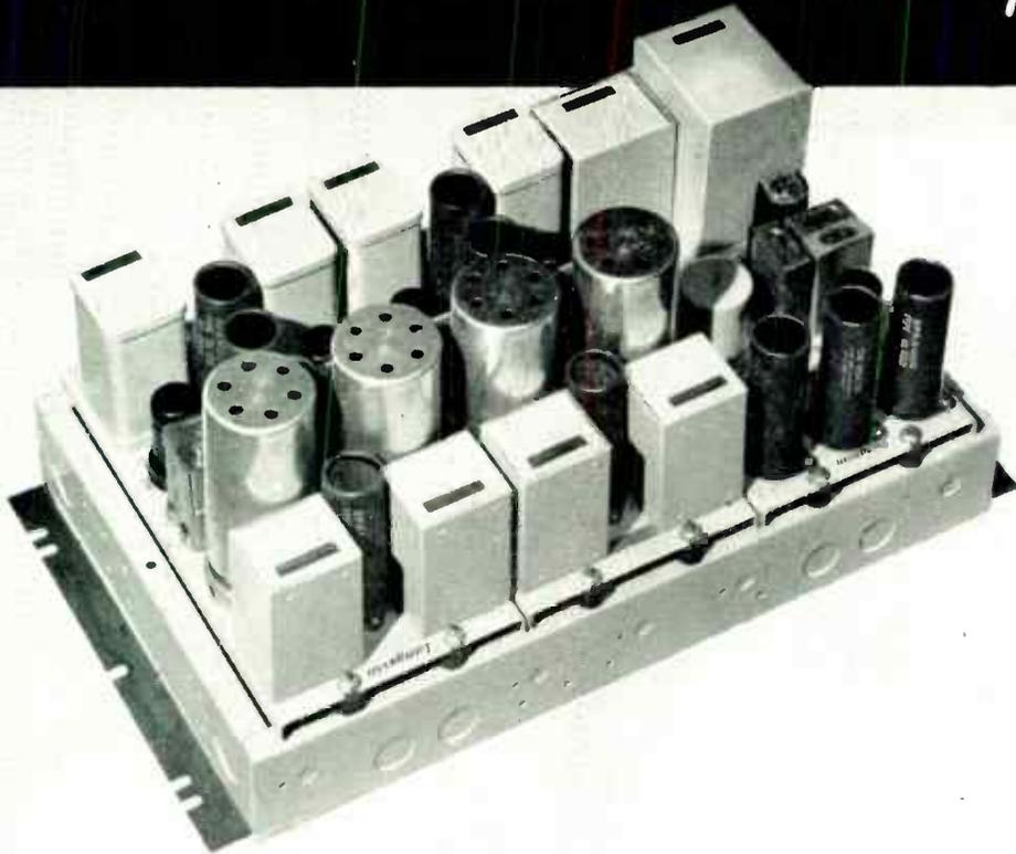
AT LEFT: Two Langevin Type 111-A Dual Pre-Amplifiers and one Langevin Type 102-A Amplifier on a Type 3-A Mounting Frame. This unit provides four pre-amplifiers and one line amplifier, or three pre-amplifiers, one booster amplifier and one line amplifier, all occupying 10½ in. of rack mounting space. An external power supply, the Langevin 201-B Rectifier, as shown below, is required. The Type 3-A Mounting Frame can be housed in a Type 201-A Cabinet, for wall mounting, if desired.
