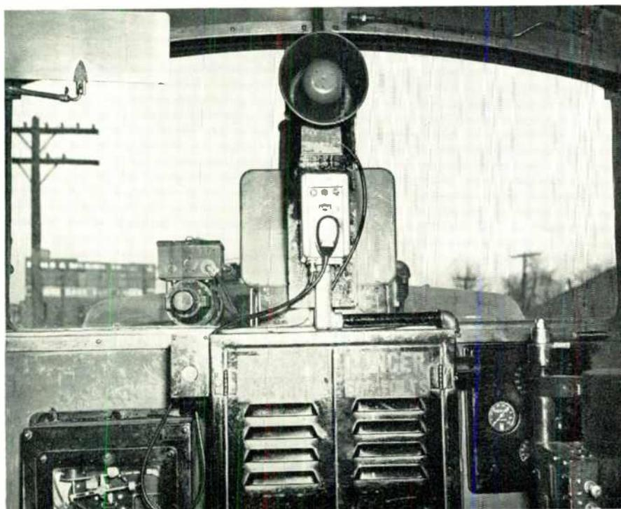
FIG. 13. LOOKING OUT OF THE DIESEL LOCOMOTIVE CAB. SPEAKER AND MICROPHONE MOUNTING CAN BE SEEN, AS WELL AS THE RADIO EQUIPMENT MOUNTED OUTSIDE
