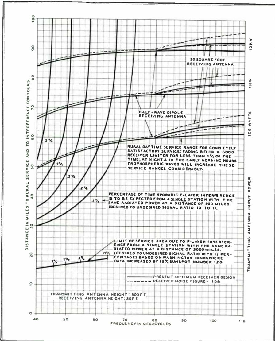
FIG. 4. EXPECTED RURAL SERVICE AND INTERFERENCE RANGES FOR FM BROADCAST STATIONS IN ABSENCE OF THUNDERSTORMS OR MAN-MADE NOISE. TRANSMITTING ANTENNA HEIGHT, 500 FT.; RECEIVING ANTENNA HEIGHT, 30 FT.
