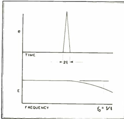
FIG. 1. CURVES SHOWING THE RELATION BETWEEN THE DURATION OF A PULSE,  $2T$ , AND ITS FREQUENCY SPECTRUM
