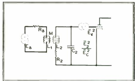
FIG. 11. CIRCUIT SHOWING EQUIVALENT TUBE NOISE GENERATOR,  $E_t$
