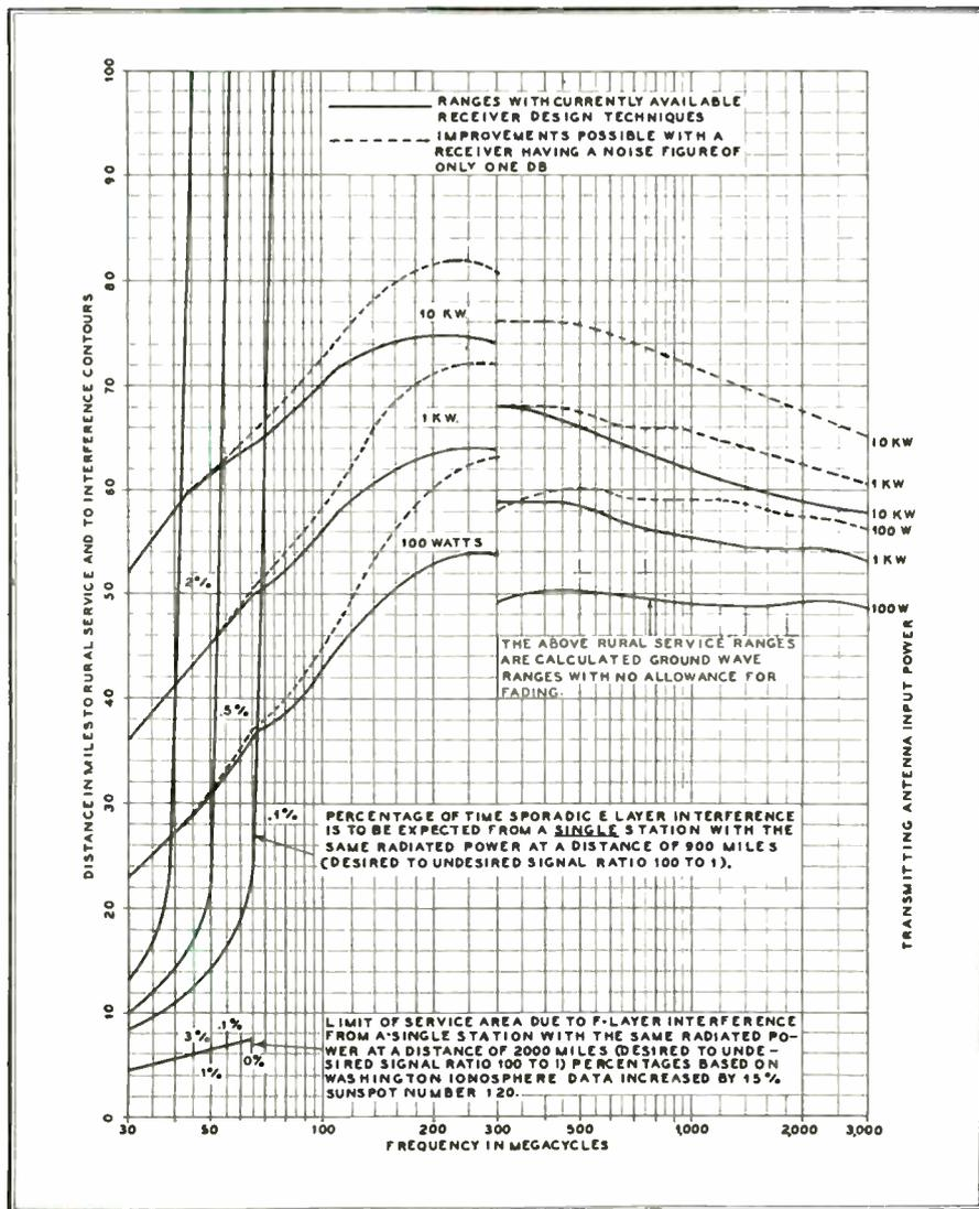
FIG. 5. EXPECTED RURAL SERVICE AND INTERFERENCE RANGES FOR TELEVISION BROADCAST STATIONS IN THE ABSENCE OF THUNDERSTORMS OR MAN-MADE NOISE. TRANSMITTING ANTENNA HEIGHT, 500 FT.; RECEIVING ANTENNA HEIGHT, 30 FT.
