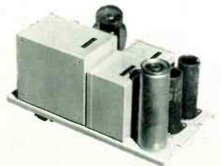
The Type 201-B Rectifier supplies plate and filament power for the Langevin Types 102, 106, 111 and similar amplifiers from a 105-125 volt, 50-60 cycle AC source. The ripple voltage of the 201-B Rectifier is 0.04% at full power output 75MA and 0.02% at a drain of 30 milliamperes.
