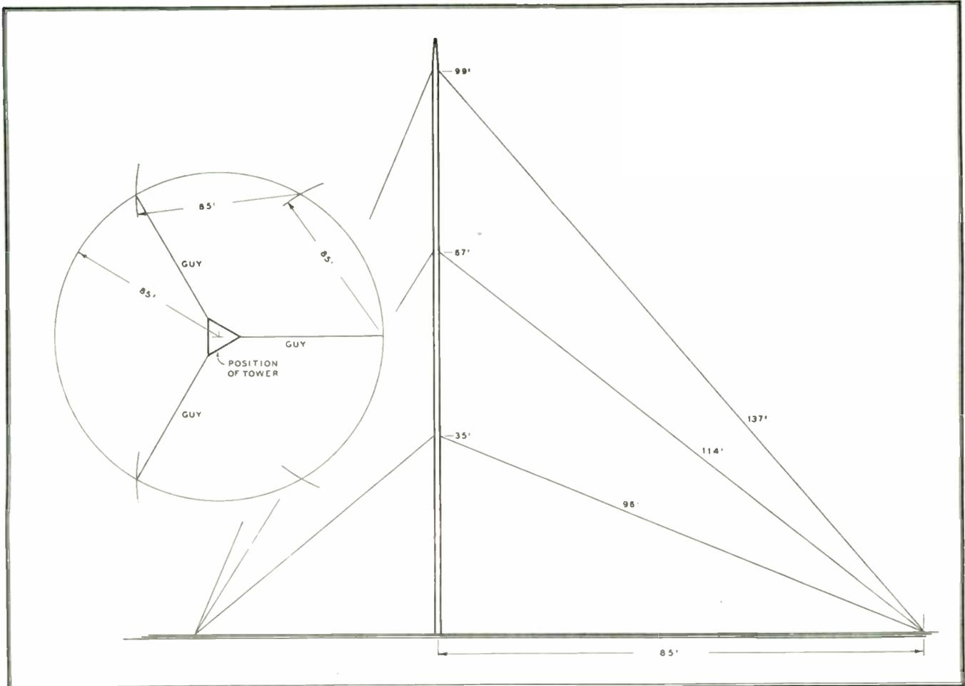
FIG. 2, ABOVE. THREE SETS OF GUY WIRES ARE REQUIRED, SPACED 120° APART ON A RADIUS OF 85 FT., AS THIS SKETCH SHOWS
