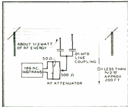
FIG. 7. INDUCTION RADIO CONNECTIONS
