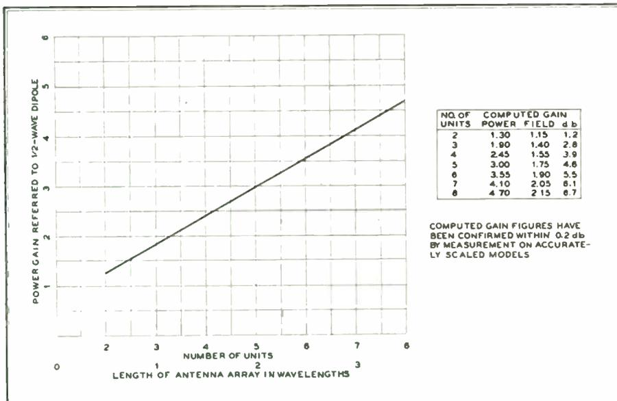
FIG. 3. POWER GAIN VS. NUMBER OF ANTENNA UNITS AND LENGTH OF ARRAY
