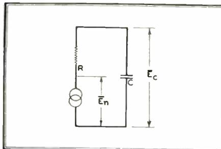
FIG. 2. CIRCUIT USED TO DETERMINE VOLTAGES OF THE EQUIVALENT FLUCTUATION VOLTAGE GENERATOR,  $E_n$
