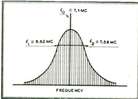
FIG. 6. FREQUENCY SPECTRUM OF THE FLUCTUATION VOLTAGES ACROSS THE CONDENSER IN THE ILLUSTRATIVE PROBLEM. THE BANDWIDTH OF THIS CIRCUIT IS 480 KC. ON EITHER SIDE OF RESONANCE
