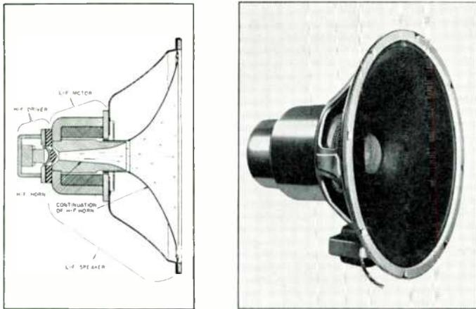
FIG. 1. CROSS-SECTION AND ASSEMBLED VIEW OF JENSEN SPEAKER
