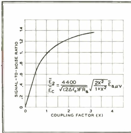
FIG. 10. CURVE OF SIGNAL-TO-NOISE RATIO FOR THE INPUT CIRCUIT OF A RECEIVER PLOTTED VERSUS COUPLING FACTOR,  $x$  ( $x = \omega M / \sqrt{R_a R_2}$ )
