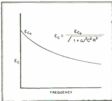
FIG. 3. FREQUENCY SPECTRUM OF THE FLUCTUATION VOLTAGES ACROSS THE CONDENSER OF THE CIRCUIT SHOWN IN FIGURE 2
