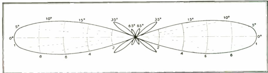
FIG. 2. COMPUTED RADIATION PATTERN FOR A 5-UNIT CLOVERLEAF ARRAY
