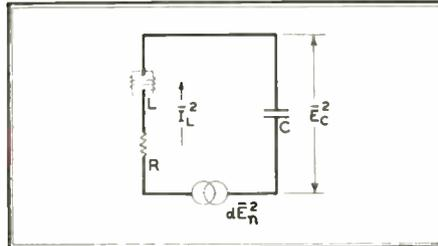
FIG. 4. TUNED CIRCUIT FOR WHICH THE FLUCTUATION VOLTAGES ACROSS THE CONDENSER ARE DETERMINED
