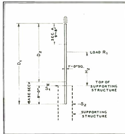
FIG. 5. DIMENSIONS OF THE ANTENNA GIVEN IN ACCOMPANYING TABLE 2
