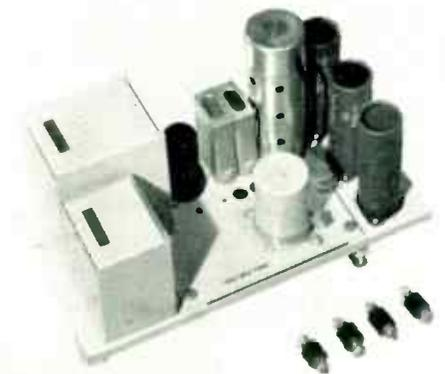
The Type 106-A Amplifier is a two-stage, fixed medium gain, low noise pre-amplifier, or booster amplifier, for use in high-quality speech input systems. The Type 106-A can be mounted on one-third of the space available on a Type 3-A Mounting Frame in combination with two Type 111-A Pre-Amplifiers, or in any similar combination.
