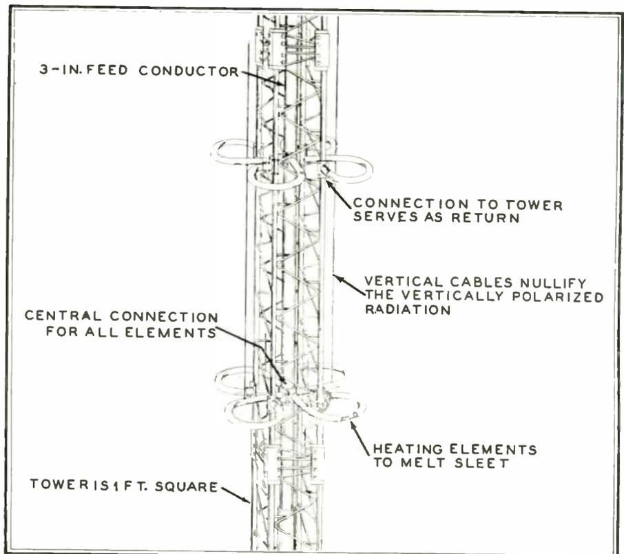
FIG. 1. DETAILS OF THE ANTENNA, SHOWING HOW RADIATORS ARE CONNECTED BETWEEN THE CENTRAL CONDUCTOR AND THE LEGS OF THE SUPPORTING TOWER
