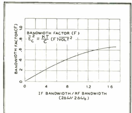
FIG. 8. PLOT OF BANDWIDTH FACTOR, F, VERSUS BANDWIDTH RATIO
