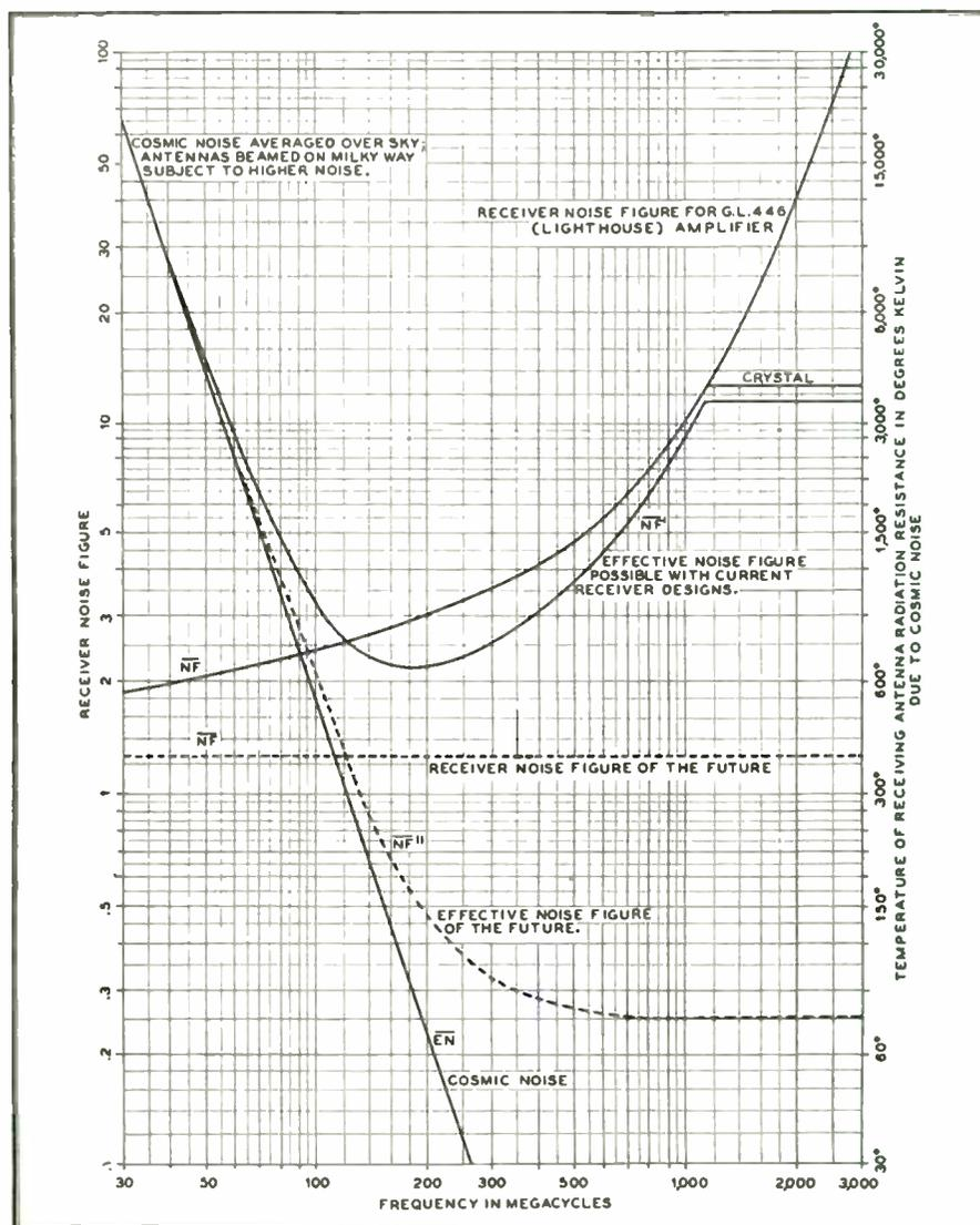
FIG. 1. EFFECTIVE NOISE FIGURES FOR VHF AND UHF RECEIVERS. THIS DATA INCLUDES EFFECTS OF COSMIC NOISE. CURVES ARE FOR PRESENT AND POSSIBLE FUTURE SETS
