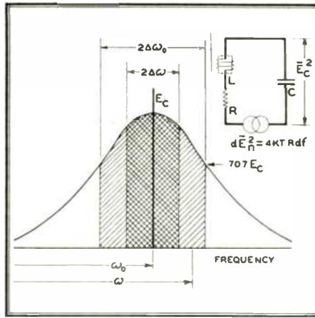
FIG. 7. FREQUENCY SPECTRUM OF FLUCTUATION VOLTAGES SHOWING THE RELATION OF THE R.F. BANDWIDTH ( $2\Delta\omega_0$ ) AND THE BANDWIDTH ( $2\Delta\omega$ ) OF THE INTERMEDIATE FREQUENCY AMPLIFIER FOLLOWING THE RF STAGE
