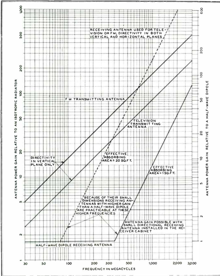
FIG. 2. TRANSMITTING AND RECEIVING ANTENNA GAINS USED IN ESTIMATING EXPECTED SIGNAL RANGE OF FM AND TELEVISION BROADCASTING STATIONS
