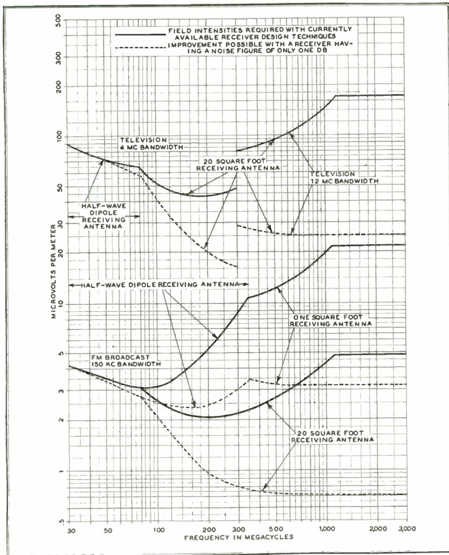
FIG. 3. FIELD INTENSITIES REQUIRED FOR SATISFACTORY TELEVISION OR FM RECEPTION IN THE ABSENCE OF THUNDERSTORMS OR MAN-MADE NOISE
