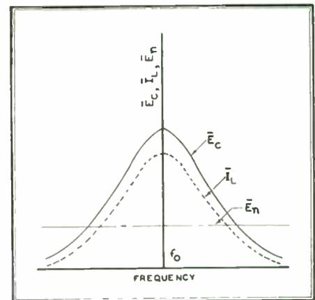
FIG. 5. SPECTRUM OF THE FLUCTUATION VOLTAGES ACROSS THE CONDENSER AND EQUIVALENT GENERATOR AND FLUCTUATION CURRENTS IN THE INDUCTANCE
