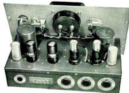
Entire chassis of both amplifiers and power supply instantly slides out of cabinets by merely turning four air lock screws on front panels. Provides complete accessibility to all components and wiring for emergency servicing. Supplied with either Cannon or Hubbell plugs.
