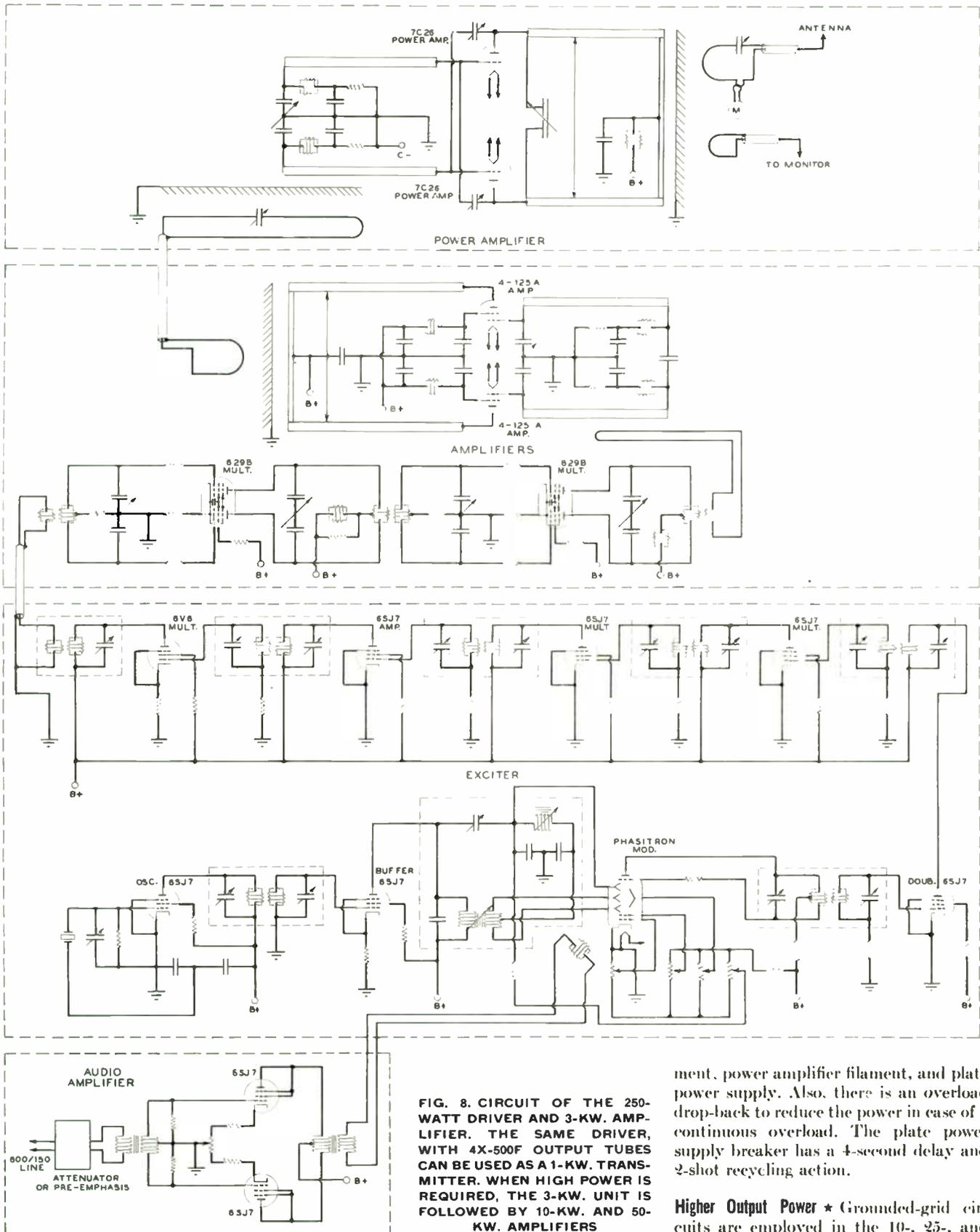
FIG. 8. CIRCUIT OF THE 250-WATT DRIVER AND 3-KW. AMPLIFIER. THE SAME DRIVER, WITH 4X-500F OUTPUT TUBES CAN BE USED AS A 1-KW. TRANSMITTER. WHEN HIGH POWER IS REQUIRED, THE 3-KW. UNIT IS FOLLOWED BY 10-KW. AND 50-KW. AMPLIFIERS
