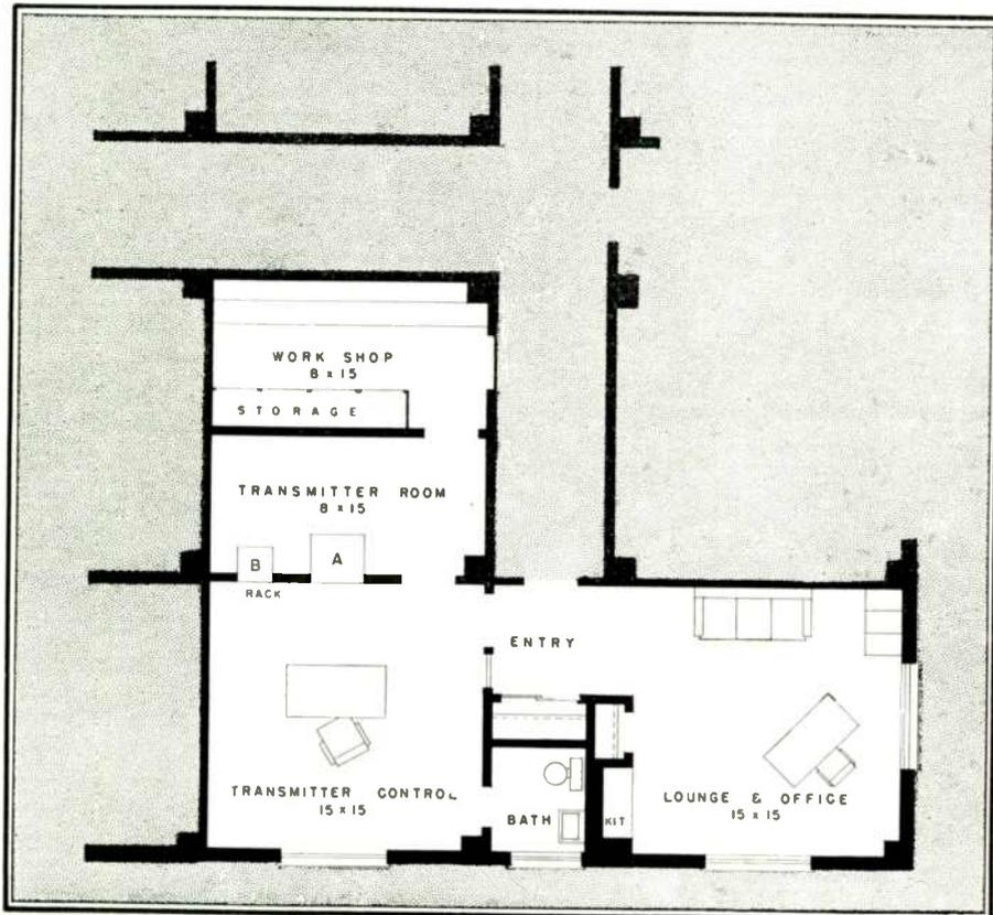
FIG. 3. AN ALTERNATE PLAN, ALSO ADAPTABLE TO A SEPARATE TRANSMITTER BUILDING
