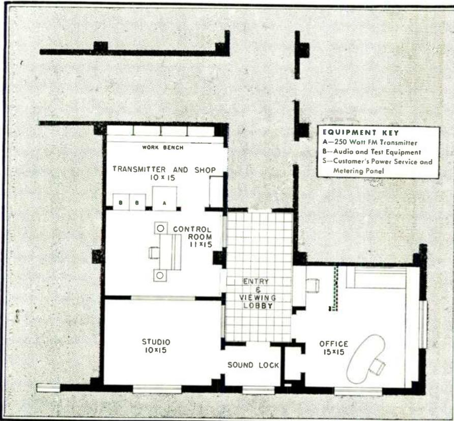
FIG. 2. PLAN FOR THE ARRANGEMENT IN FIG. 1, FOR OFFICE BUILDING LOCATION
