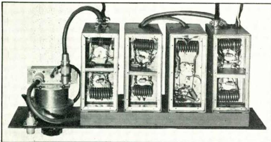
FIG. 6. ONE OF THESE SEPARATE RF ASSEMBLIES IS USED FOR EACH CHANNEL
