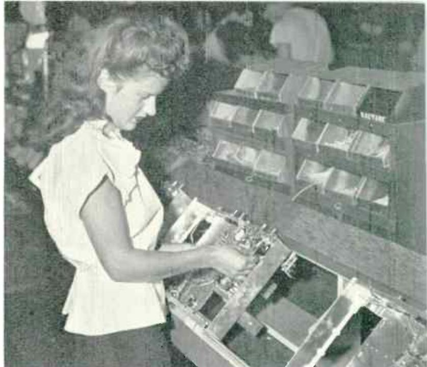
5. SWITCH SECTION SUB-ASSEMBLY IS WIRED BEFORE IT IS MOUNTED ON CHASSIS. 6. CHASSIS STARTS ON MAIN ASSEMBLY LINE
