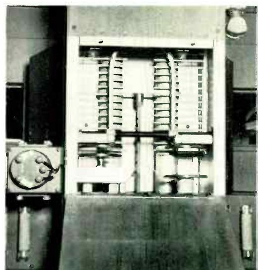
FIG. 4. SHIELD BETWEEN FINAL TANK AND COUPLING
