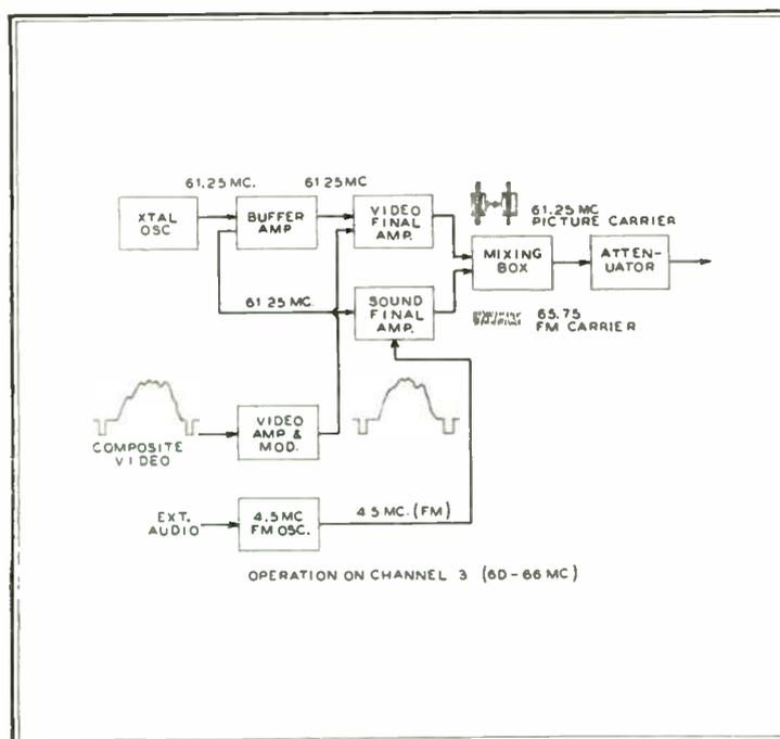
FIG. 2. BLOCK DIAGRAM OF THE VIDEO-AUDIO SIGNAL GENERATOR.
