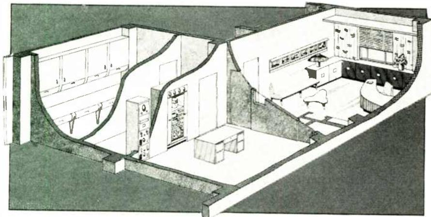
FIG. 1. TRANSMISSION FACILITIES PLANNED FOR A 250-WATT FM STATION
