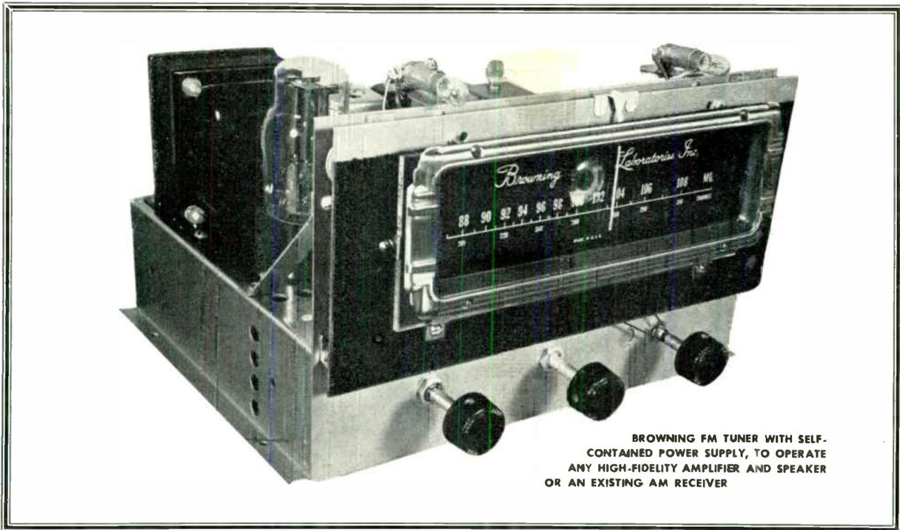
BROWNING FM TUNER WITH SELF-CONTAINED POWER SUPPLY, TO OPERATE ANY HIGH-FIDELITY AMPLIFIER AND SPEAKER OR AN EXISTING AM RECEIVER
