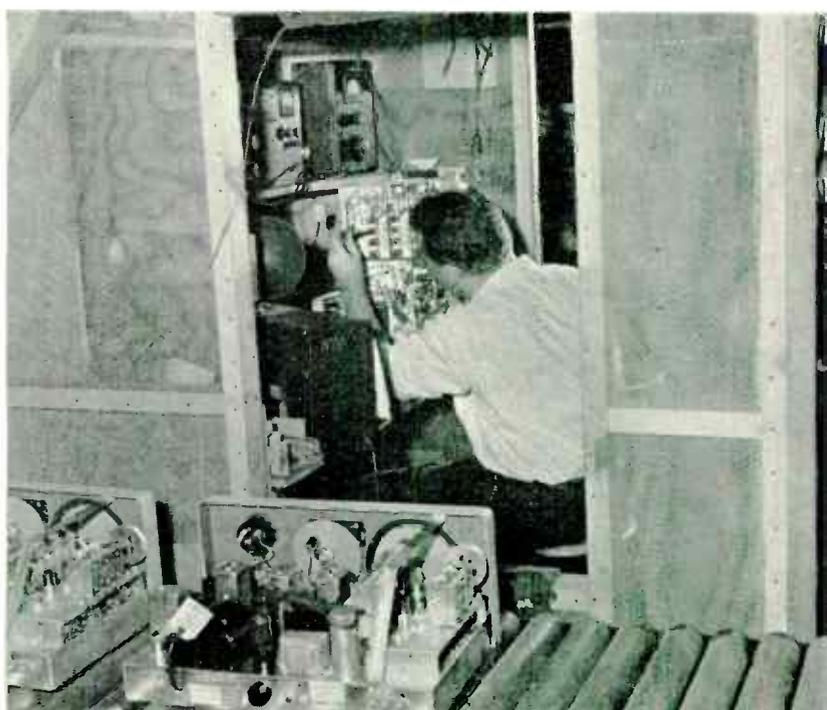
13: FINISHED CHASSIS ROLL TO THE TEST CAGES. 14: LONG PRACTICE AND GOOD INSTRUMENT SPEED FIVE-BAND ALIGNMENT
