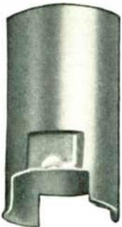
● The XOS tube shield is a two-piece shield for Miniature Button 7-pin base tubes. It mounts with the XOA or XOR socket and is available in three sizes, XOS-1 (1-3/16" high), XOS-2 (1 1/2" high), and XOS-3 (2" high).
