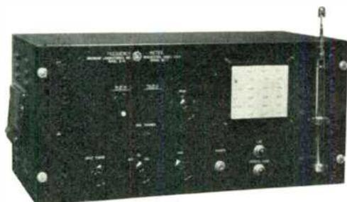
The BROWNING S-5 meter, accurate to  $\pm .0025\%$ , is suitable for all standard and special services on 30 to 500 mc. The crystal, contained in a temperature-controlled oven, is accurate to  $\pm .001\%$ . The electron-coupled oscillator is temperature compensated, and a line-voltage regulator is built into the meter.
