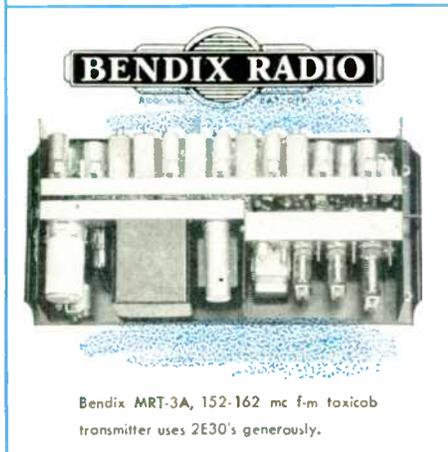
Bendix MRT-3A, 152-162 mc f-m toxicab transmitter uses 2E30's generously.
