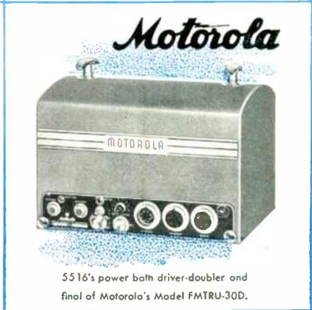
5516's power both driver-doubler and final of Motorola's Model FMTR-30D.
