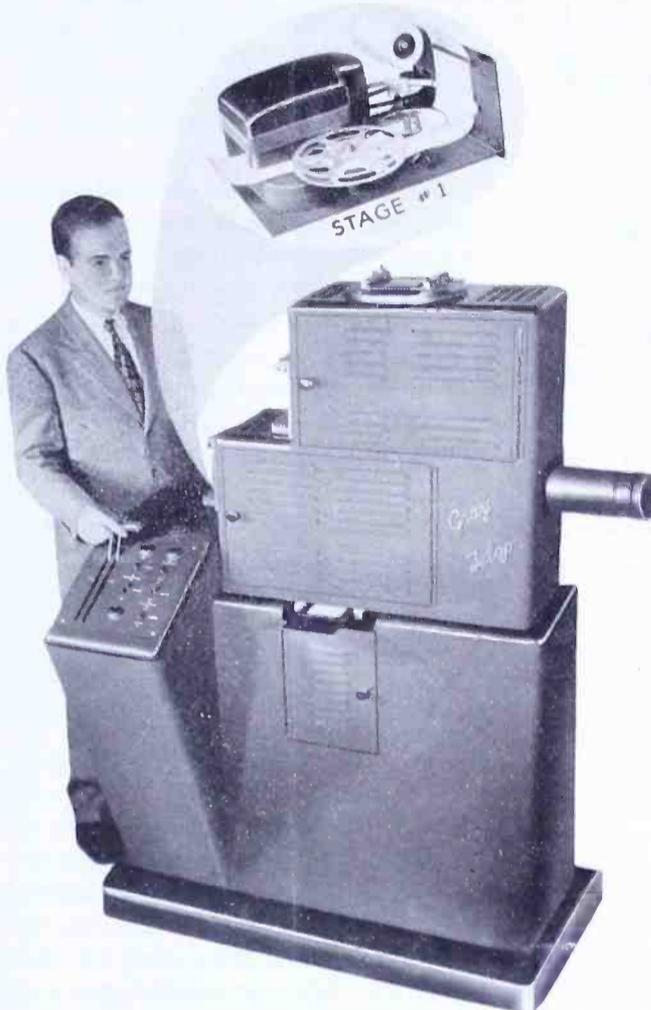
*This most versatile telecasting optical projector enables dual projection with any desired optical dissolve under exact control.*
