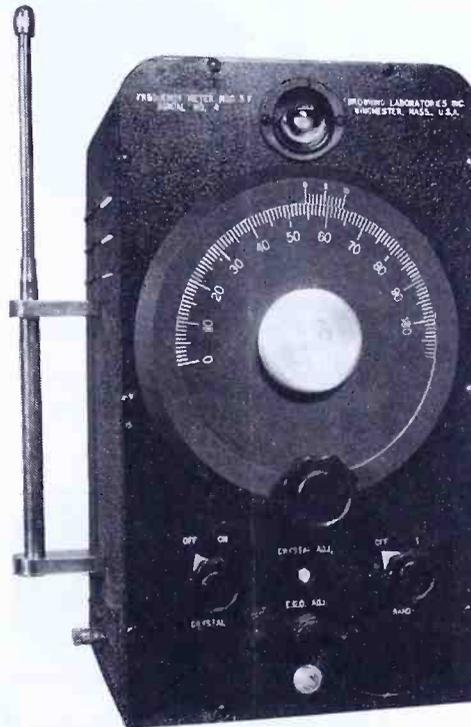
Model S-4 and S-7 Frequency Meters Can't that be done with any make of meter? No, indeed. To check a meter directly against WWV, the crystal must be a submultiple of a WWV frequency. That the secret. That's the reason why every BROWNING meter, regardless of the calibration points, uses a 100-kc. crystal.
