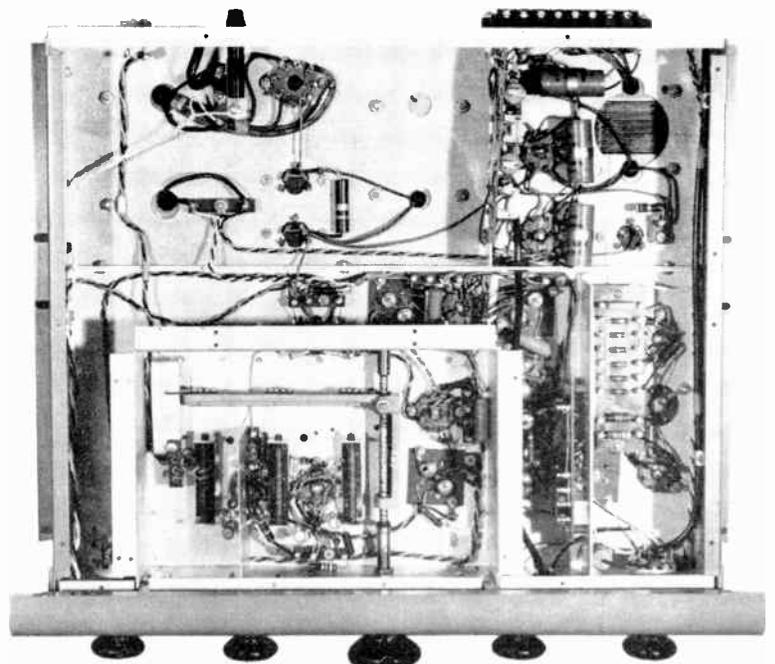
Fig. 2. Permeability tuning is controlled through a worm drive from the tuning knob
