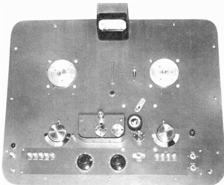
Fig. 2. Layout of the tape transport system and operating controls on the top plate
