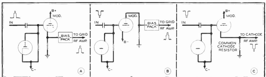
Fig. 7. Three methods of DC modulation which are used for television transmitters
