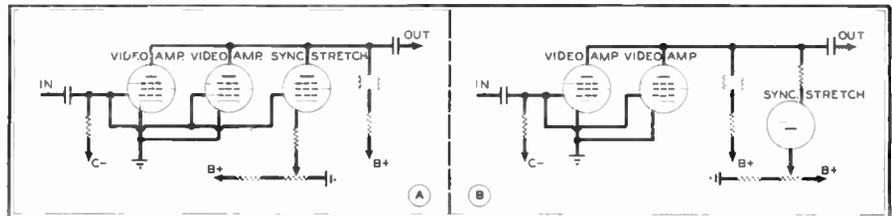
Fig. 6. Two basic types of control circuits which are used for sync expansion
