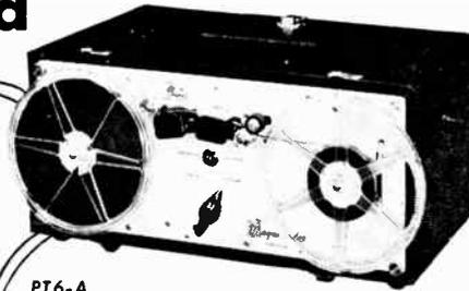
**PT6-A Recorder Mechanism** is the heart of Magnecord combinations for studio and remote recording. Weighs 26 lbs. in carrying case, easily removable for rack mount. Quick-change capstans for recording at 7½ or 15 inches sec. High speed rewind. Frequency response 40 to 15,000 cps ± 2 db. **\$278**
