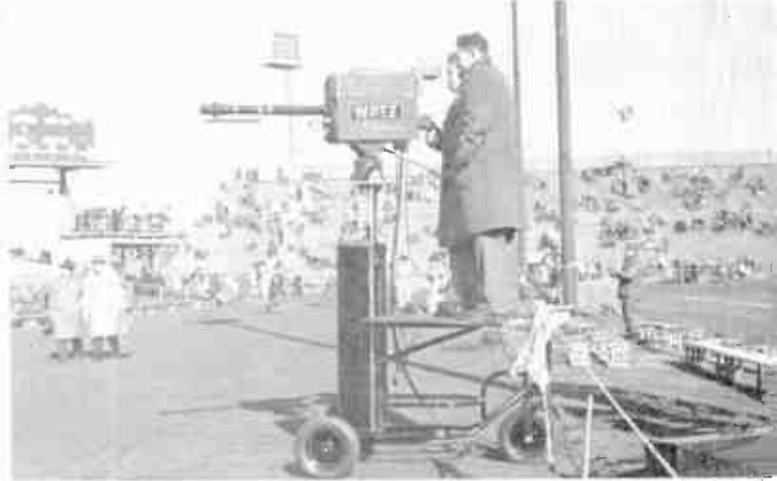
mount a TV camera for picking up sports events. To the ease of moving the camera, this rig adds the advantage of raising both camera and operator above the heads of spectators.
