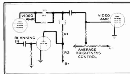
Fig. 5. A second blanking insert system
