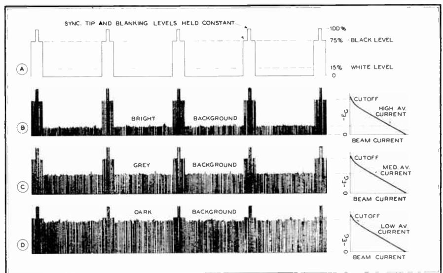
Fig. 1. Average signal amplitude must be changed as the average brightness changes
