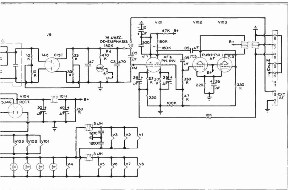
except for a 6-volt supply. Note connections for meters and external audio source
