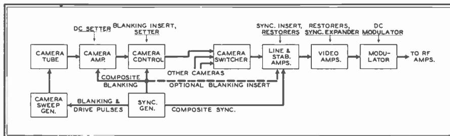
Fig. 2. Major units of a transmitter, showing the locations of the special controls
