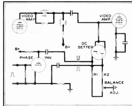
Fig. 4. Arrangement of the DC setter
