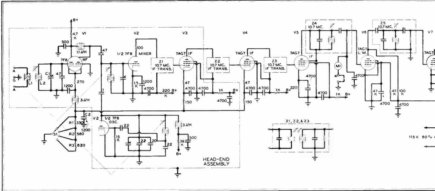
Fig. 1. Schematic of the REL model 616B receiver for the broadcast band, operating on 115 volts, 60 cycles. Model 618B is similar
