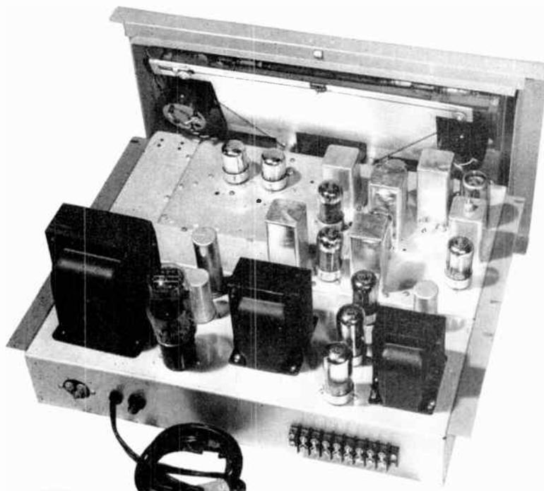
Fig. 3. Heavy steel construction and side fastening on chassis make a rugged assembly
