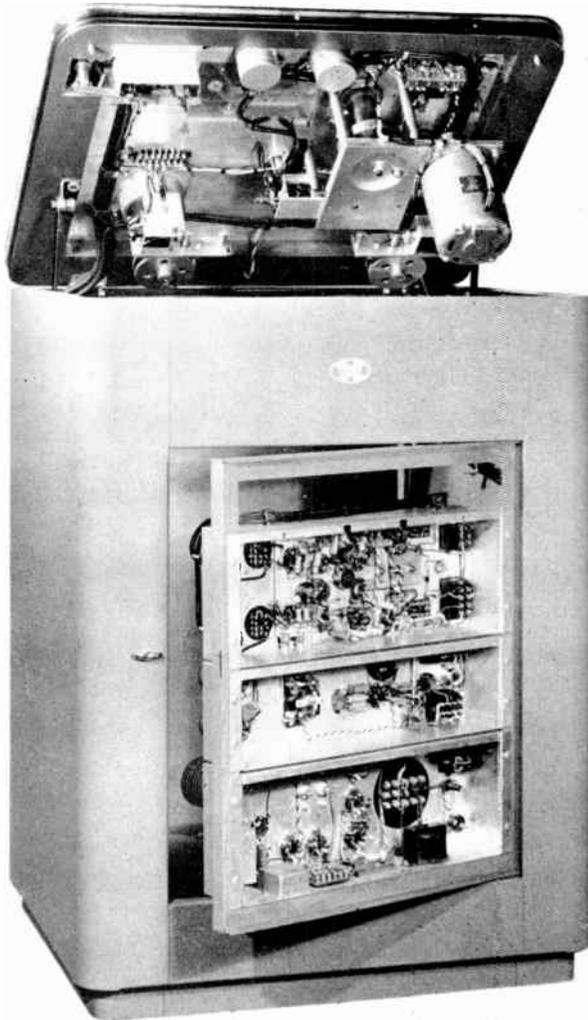
*Fig. 3, left: The complete mechanism is carried on the hinged top plate. Front and rear of the chassis are accessible when the cabinet door is removed. Fig. 4, right: Rear view of the studio recorder, showing the chassis connections*
