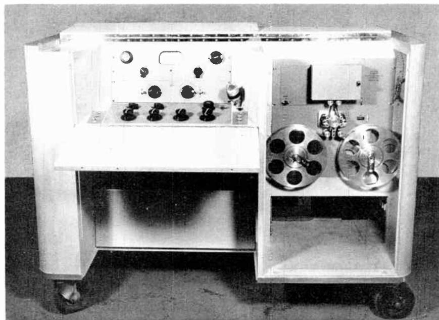
Fig. 3. Complete 35-mm. magnetic film recorder and console built into a mobile unit
