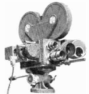
The Maurer 16 mm., designed specifically for professional use, is equipped with precision high-power focusing and the finest view-finder made. Standard equipment includes: 235° dissolving shutter, automatic fade control, view-finder, sunshade and filter holder, one 400 foot gear-driven film magazine, a 60-cycle 115-volt synchronous motor, one 8-frame handcrank, power cable and a lightweight carrying case.
