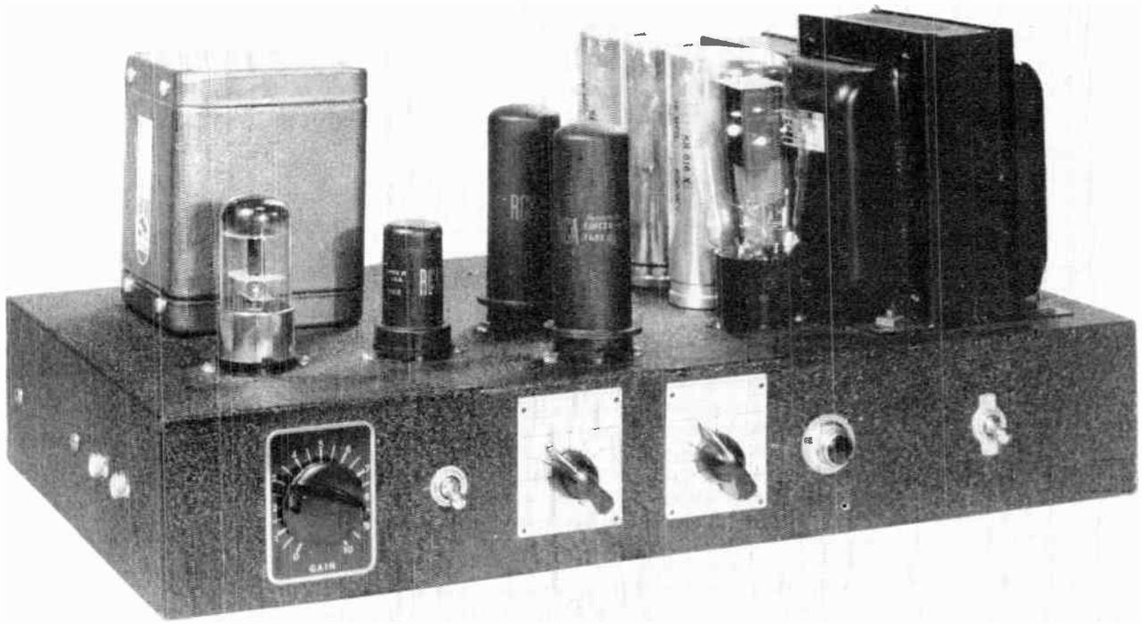
Fig. 4. Correct parts layout helps to reduce hum level. If large chassis cannot be used, power supply should be separate
