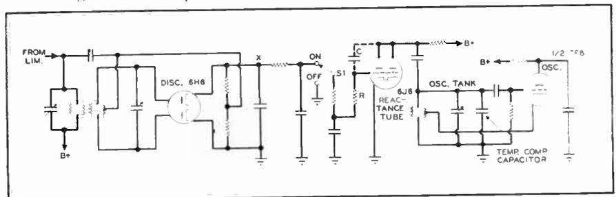
Fig. 4. Simplified diagram of AFC circuit, which employs only one additional tube
