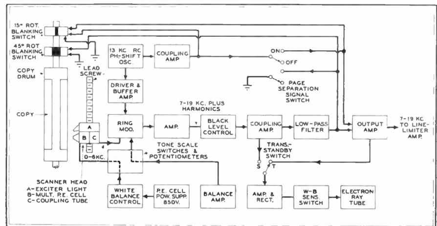
Fig. 4. The scanner and scanner amplifier units, shown at the bottom of Fig. 2
