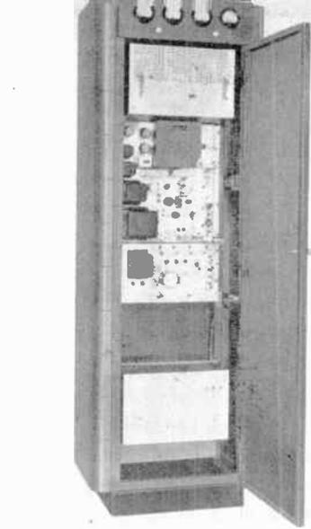
veloped this self-contained Intermodulation Meter, model 31, which can be mounted on a 19-in. rack panel. Output is two sinusoidal waveforms, one high and one low frequency, mixed at a 4-to-1 voltage ratio. These are applied to the instrument under test, the output of which is fed back to the meter. IM is read directly in distortion percentage.
