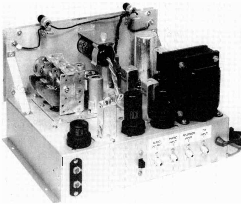
Fig. 2. Rear of model RV-10A. Note subchassis assemblies bolted to main chassis
