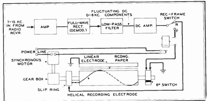
Fig. 6. The line-limiter amplifier unit, shown at top in Fig. 2. Fig. 7. Recorder amplifier and recorder, shown in Fig. 3
