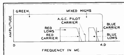
Fig. 9. Adder output frequency spectrum
