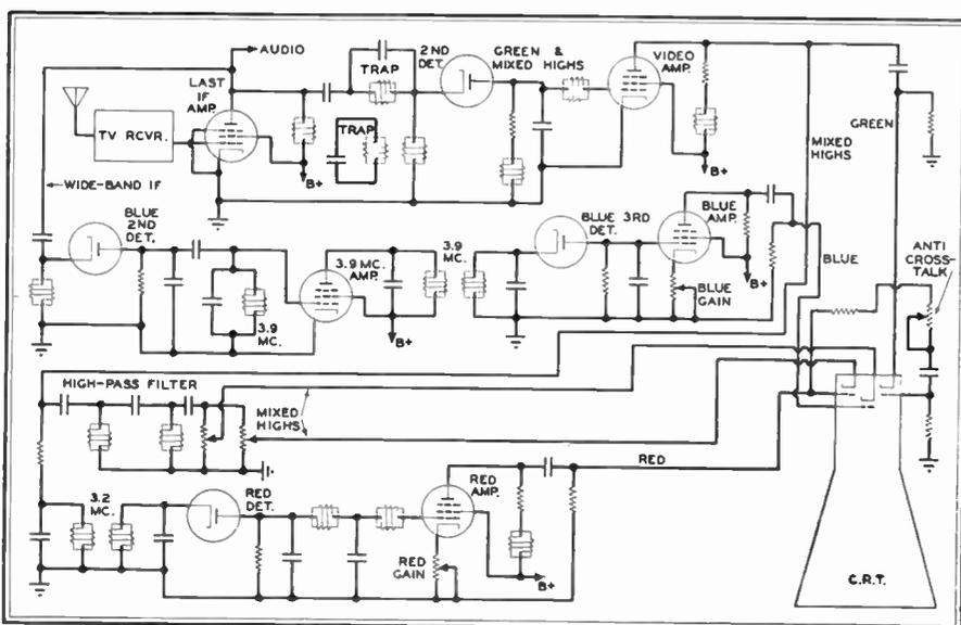
Fig. 6. Color section of simple receiver for use with frequency-interlace system
