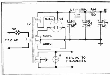
Fig. 3 Power supply has double- $\pi$  filter
