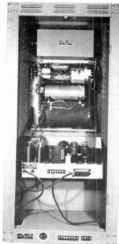
Fig. 3. This rack contains all facsimile receiving terminal equipment components
