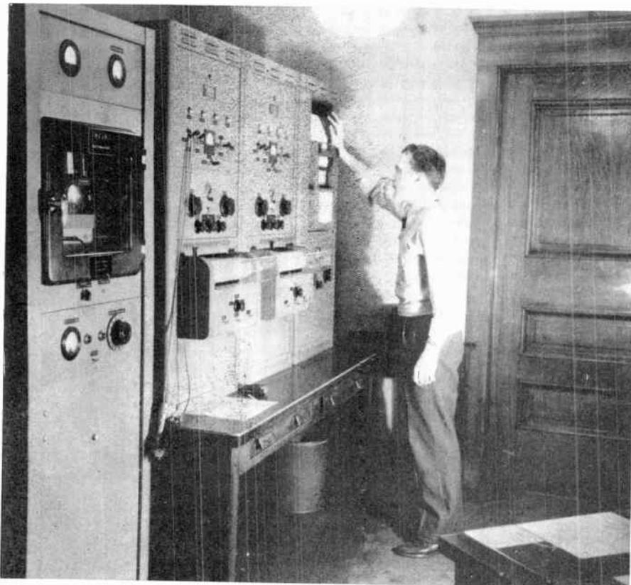
Fig. 1. Facsimile transmitting equipment at weather forecasting center in Chicago October 1950—formerly FM, and FM RADIO-ELECTRONICS
