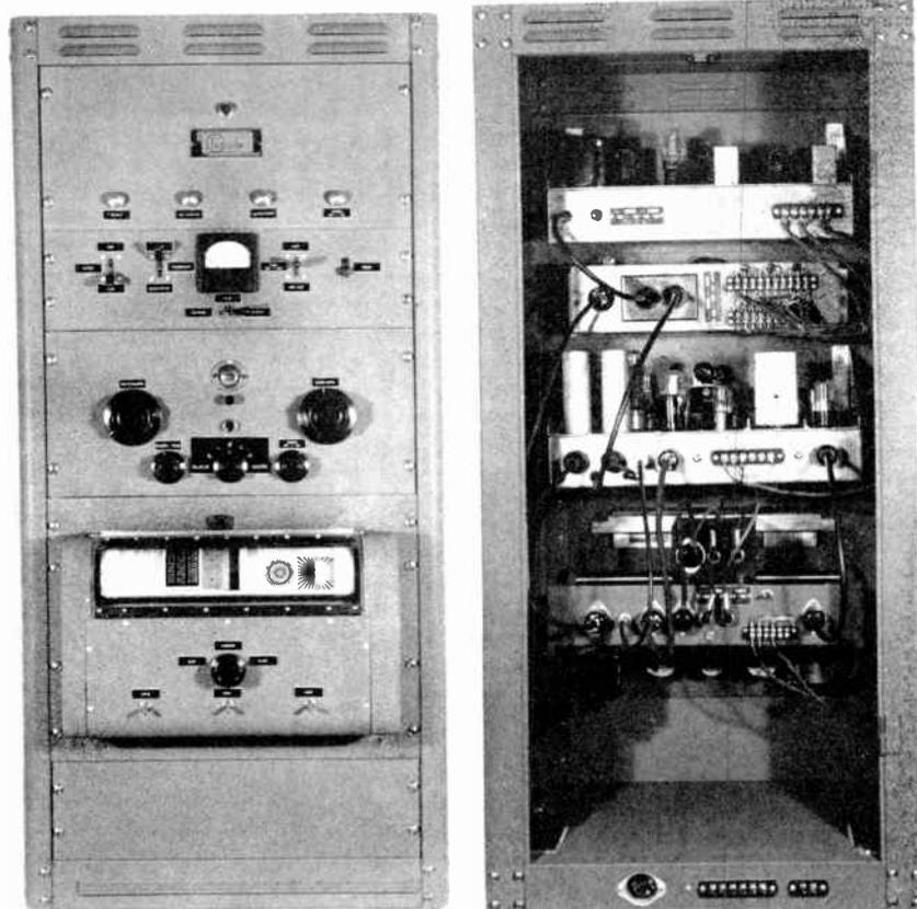
Fig. 2. Front and rear views of facsimile transmitting terminal equipment rack
