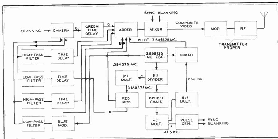
Fig. 8. Critical circuits and expensive components are located at FI transmitter
