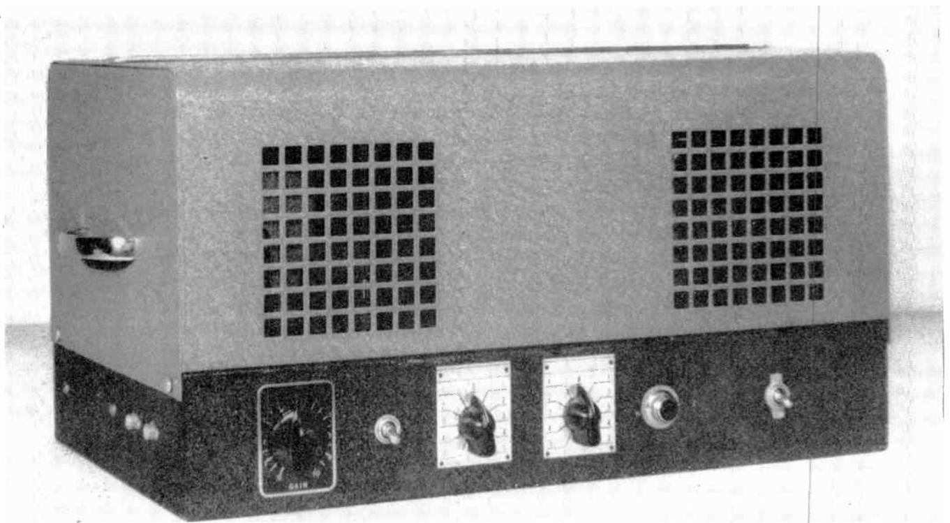
Fig. 1. The FAS amplifier, set up for demonstration purposes. Chassis-cover aids in carrying amplifier as well as shielding
