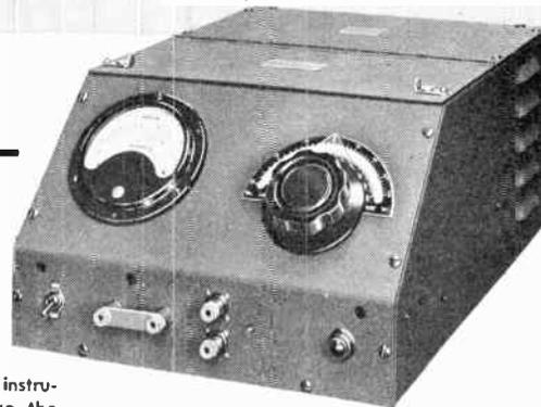
The QX-Checker is a production type test instrument specifically designed to compare the reactance and relative Q of small RF inductors with approved standards. The two factors, reactance and relative Q, are separately indicated, one on the meter and the other on a condenser dial, so that the deviation of either from established tolerances is immediately shown. Built to laboratory standards, the QX-Checker is a sturdy, foolproof instrument for use in production work by factory personnel.
