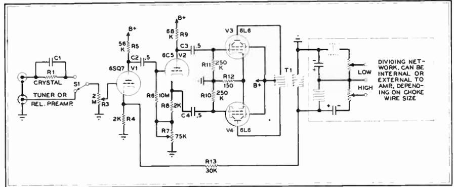
Fig. 2. Complete circuit of FAS amplifier, with one flat and one crystal input
