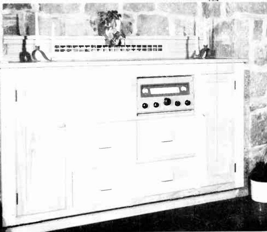
*Fig. 12, above. This installation has a special high-power audio amplifier and an equalizer to regulate speakers in several rooms. A neat, careful layout prevents confusion among the many control knobs and switches required.*
