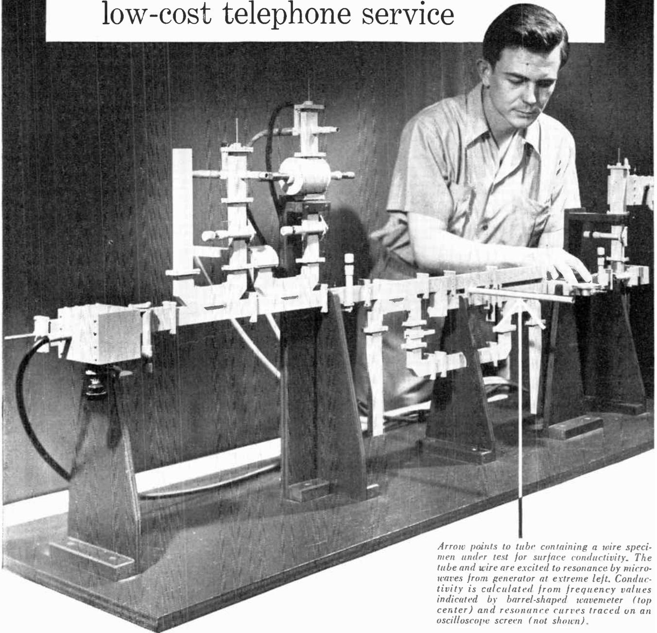
Arrow points to tube containing a wire specimen under test for surface conductivity. The tube and wire are excited to resonance by microwaves from generator at extreme left. Conductivity is calculated from frequency values indicated by barrel-shaped wavemeter (top center) and resonance curves traced on an oscilloscope screen (not shown).
