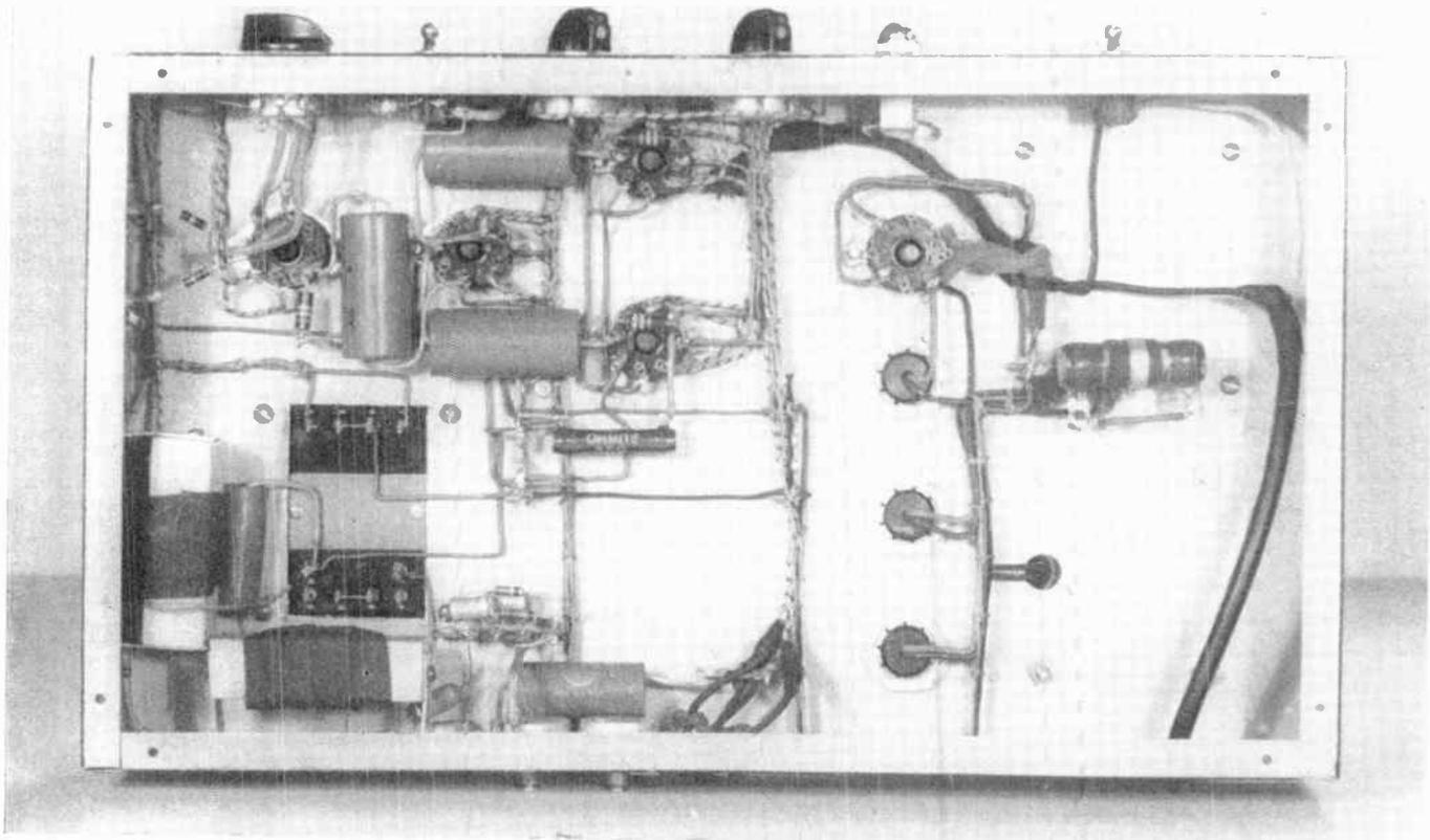
Fig. 5. Plenty of working room is provided underneath the chassis. Note extremely short AC leads from power transformer
