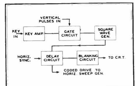
Fig. 7. Components of the decoder unit
