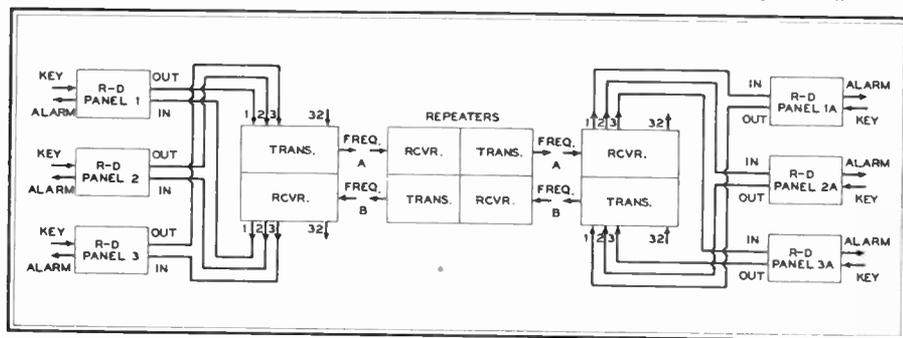
Fig. 1. How the ringdown panel can be used for multiplex channel signaling
