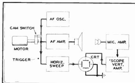
Fig. 2. Tone-pulse measuring equipment
