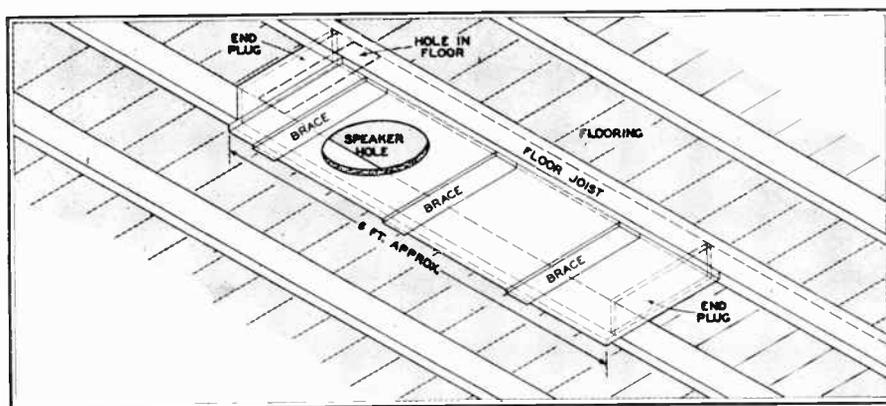
Fig. 3. How to construct an Air-coupler by enclosing space between 2 floor joists
