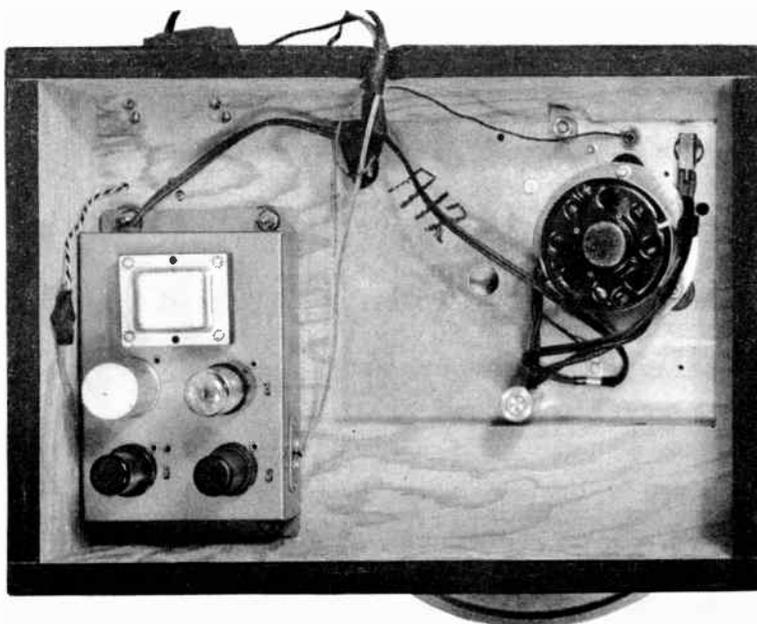
Fig. 6. A preamplifier for the reluctance cartridge is mounted under turntable base
