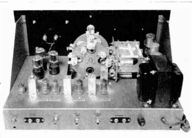
Figs. 3, above, and 4, left. Rear-panel controls for meter and peak flasher adjustments. Turret band switch can be seen at top
