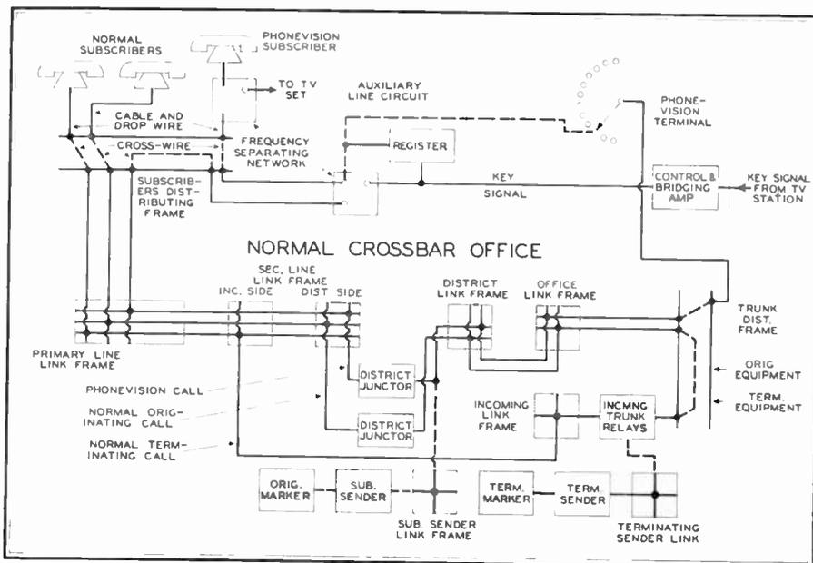
Fig. 3. How the key signal can be distributed through a crossbar telephone office
