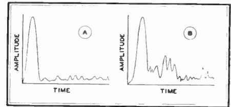
Fig. 3. CRT display of sound-decay
