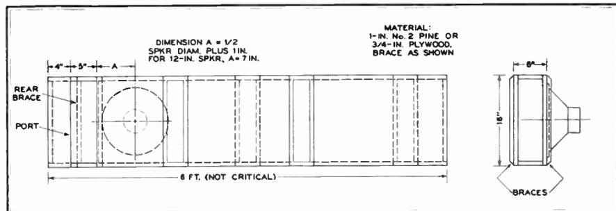
Fig. 2. Dimensions of the Air-coupler, which are apparently not at all critical
