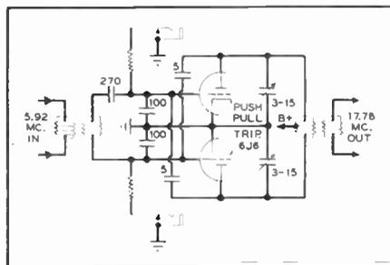
Fig. 4. Push-pull tripler stage circuit
