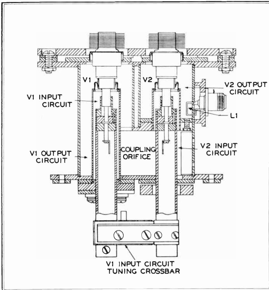
Fig. 5. Final transmitter stages are grounded-grid tripler and doubler circuits
