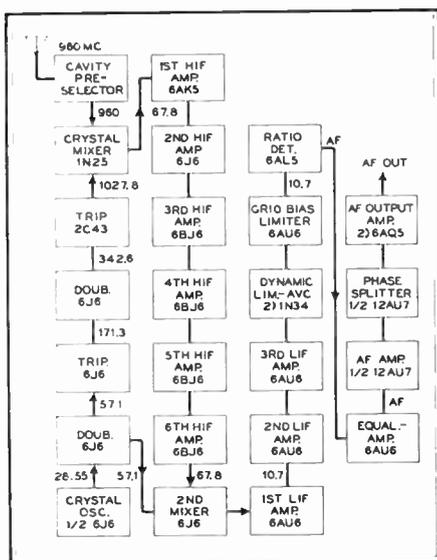
Fig. 6. Double-superheterodyne receiver
