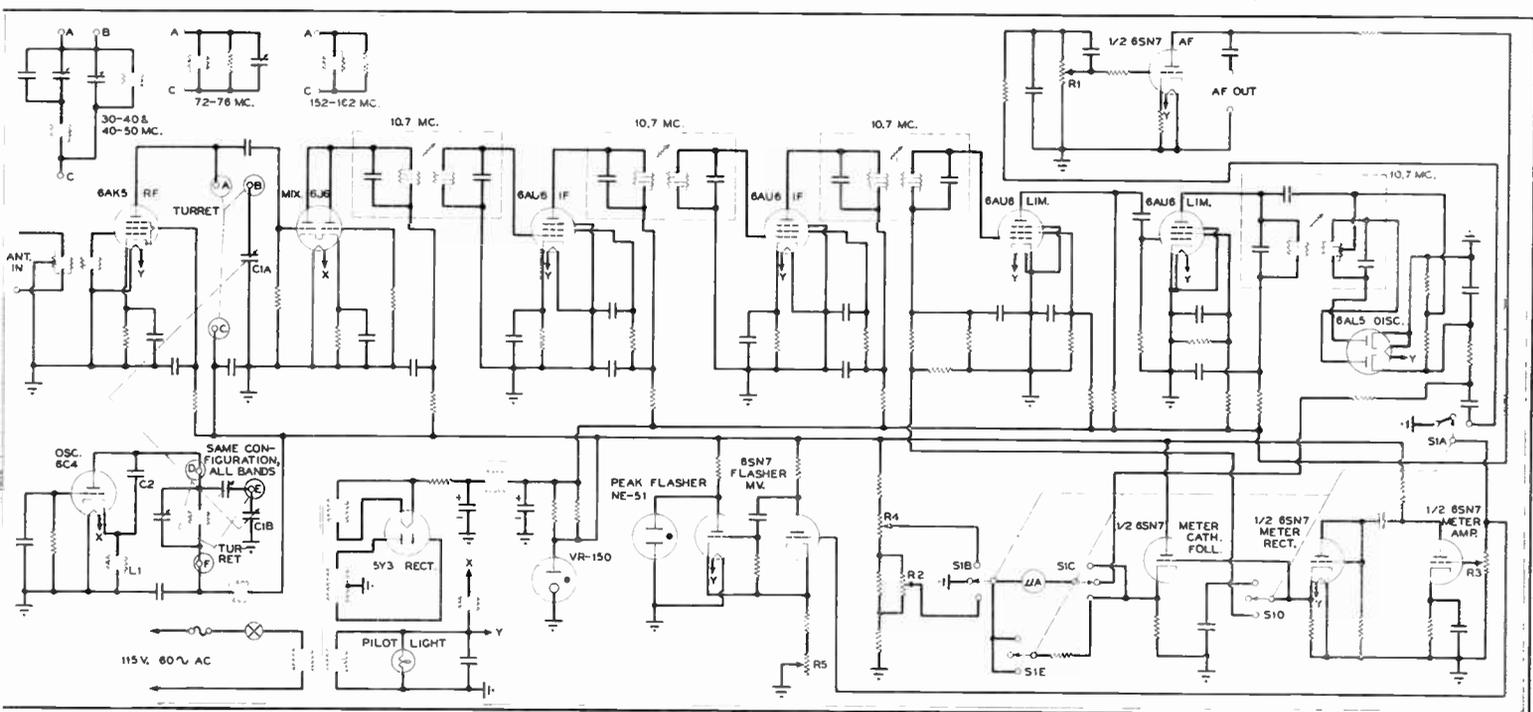
Fig. 5. Complete schematic of the MD-25 monitor. A turret band switch provides coverage of all mobile-service frequencies
