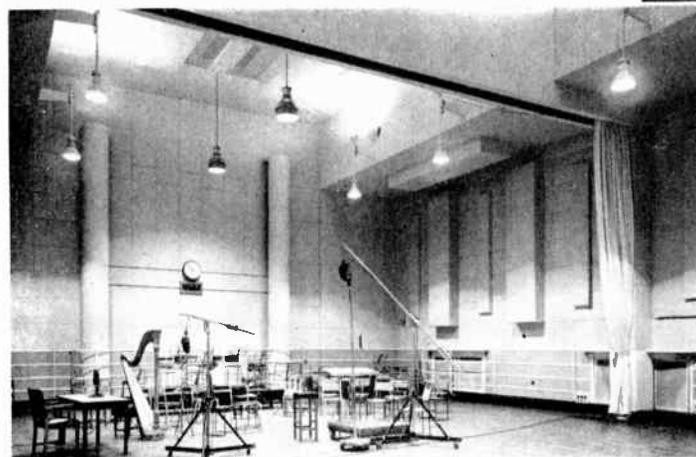
Fig. 7, left: A studio provided with resonant bass absorbers. These are long boxes fastened to the ceiling and the walls
