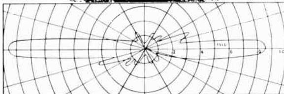
VERTICAL RADIATION PATTERN OF TYPE 3000 ANTENNA
