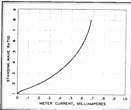
Fig. 3. Calibration chart for SWR bridge
