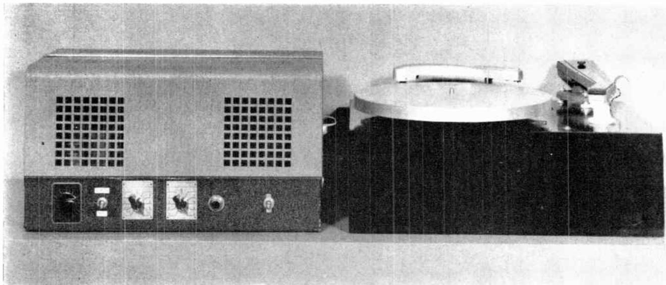
Fig. 5. The FAS amplifier and a 3-speed turntable, with crystal pickup for 78's and reluctance pickup for 45's and LP records
