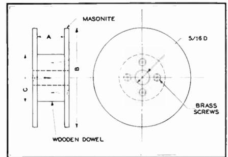
Fig. 8. Coil form for winding the chokes
