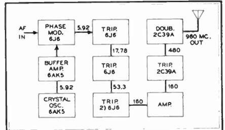
Fig. 1. The transmitter employs phase-to-frequency modulation, at 960-mc. output
