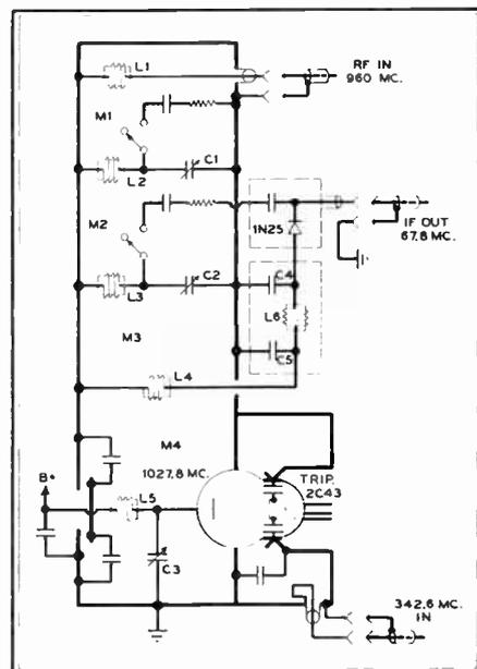
Fig. 7. The cavity preselector and mixer
