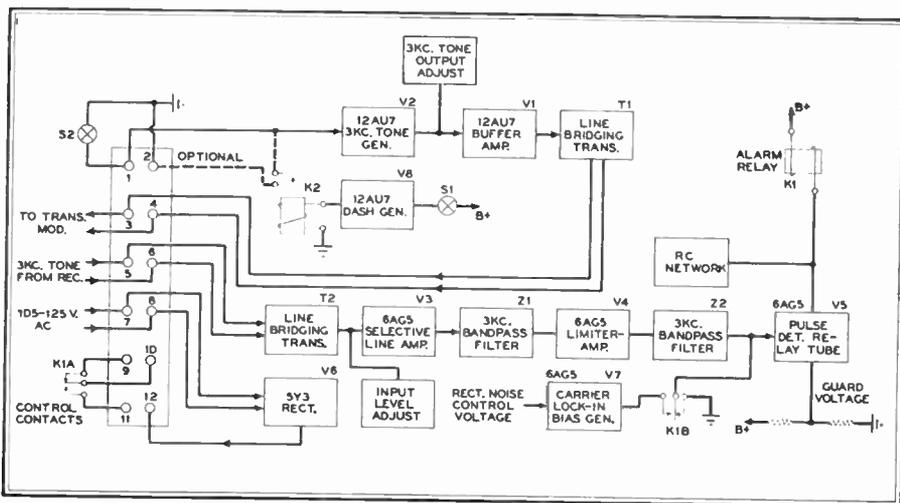
Fig. 2. Ringdown panel circuits. A panel is required at each end of each channel
