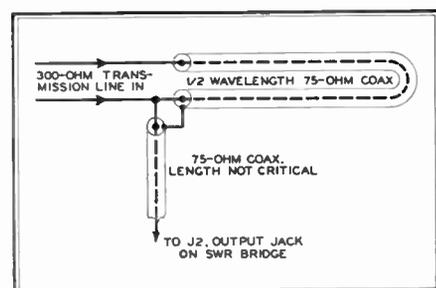
Fig. 4. Simple adapter for 300-ohm line
