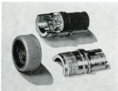
**New Connectors:** Separable cable connectors introduced by Harwood Company, 747 N. Highland Avenue, Los Angeles, feature split-shell socket that eliminates one coupling nut and one barrel. Split construction simplifies and speeds soldering of cable wires. Types range from 10 S to 48. All conform to A-N specs.
