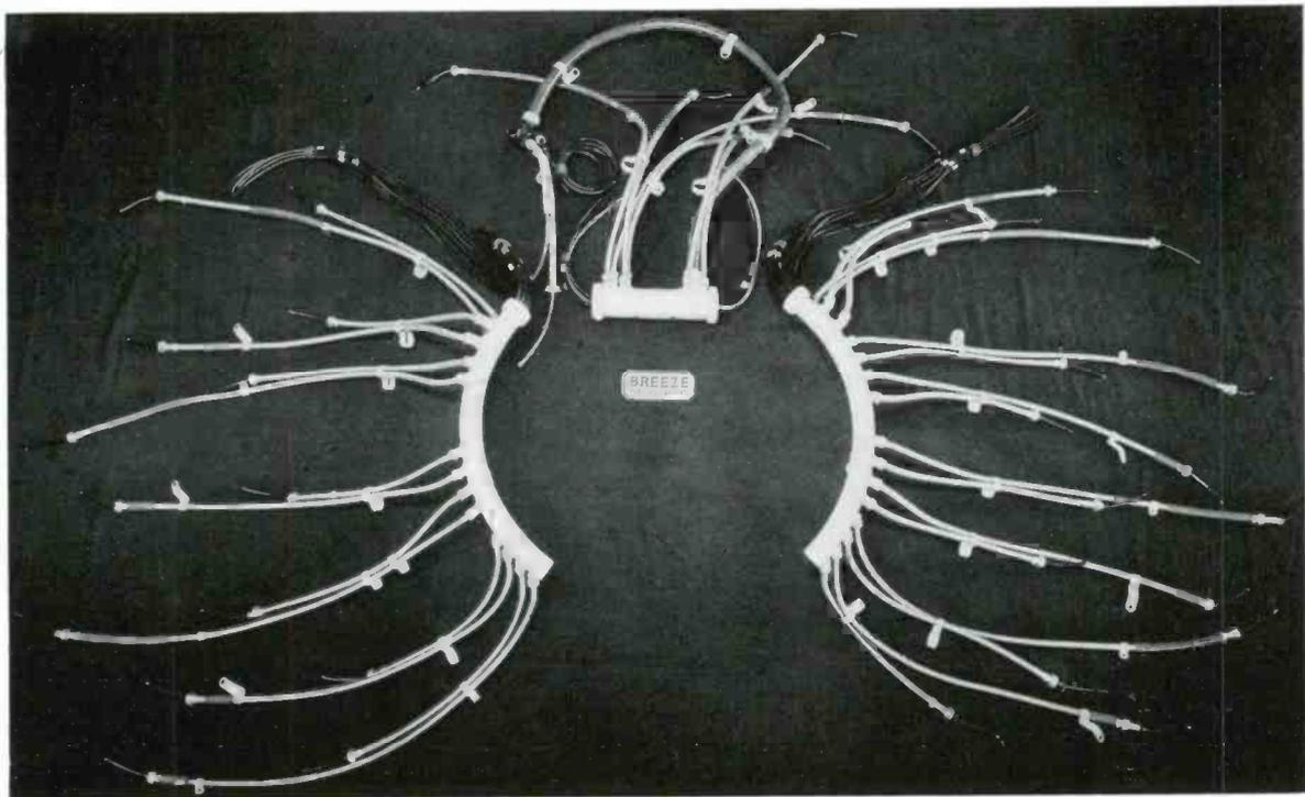
FIG. 1. SHIELDING HARNESS FOR THE 2,000 H.P. WRIGHT CYCLONE AIRCRAFT ENGINE. CLAMPS ARE SHOWN IN PLACE ON THE CABLES
