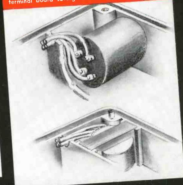
One UTC design eliminated a threaded shank, lockwasher and nut by changing to a spun-over shoulder on the shank. Saving . . . 150,000 lockwashers and nuts . . . 150,000 threading operations.
