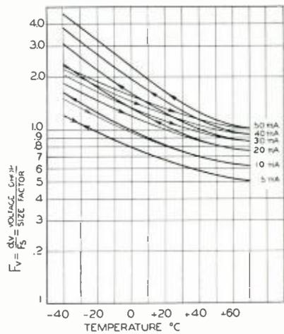
FIG. 13. FV AT VARYING CURRENT DENSITIES AGAINST AMBIENT TEMPERATURE
