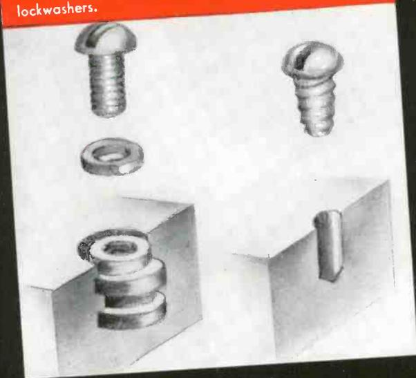
In die cast structures, covers and nameplates were held on by screws. A UTC design modification added a round projection in the casting, which is spun over to hold the plate or cover. Saving: over 2,000,000 screws and lockwashers . . . over 2,000,000 tapping operations.
