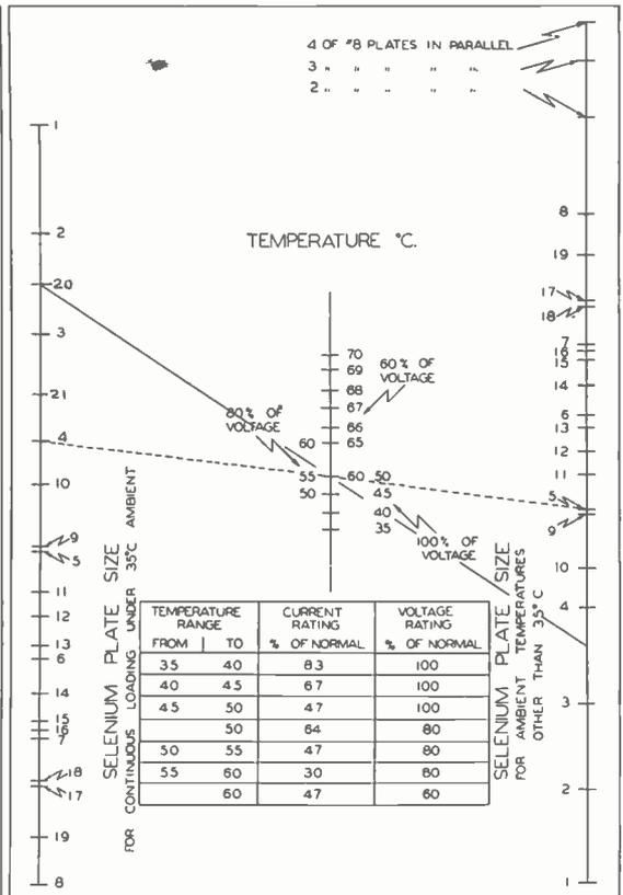
FIG. 14, LEFT. RECTIFIER TYPE FOR GIVEN OUTPUT, LOAD, AND CIRCUIT. FIG. 15, RIGHT. RELATION TO AMBIENT TEMPERATURE
