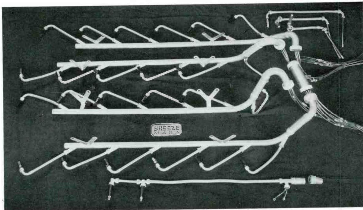
FIG. 4. THE TYPE OF SHIELDING DEVELOPED FOR AIRCRAFT IS EQUALLY EFFECTIVE FOR APPLICATION TO A PACKARD MARINE ENGINE
