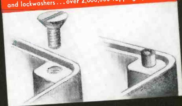
This structure employed a cased transformer fastened to a compartment wall with screws. A changed design permitted potting the transformer directly in the compartment. Saving . . . 1,000,000 terminals . . . 300,000 screws . . . 400,000 aluminum cans . . . plus terminal board saving and reduction in overall size.
