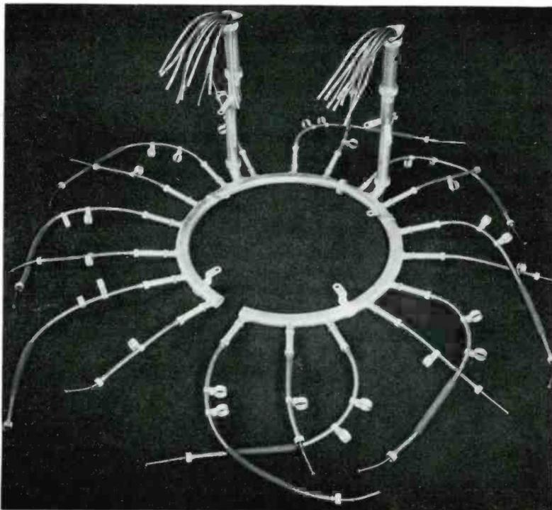
FIG. 2. SHIELDING ASSEMBLY USED ON THE IGNITION SYSTEM OF THE WRIGHT D-1820
