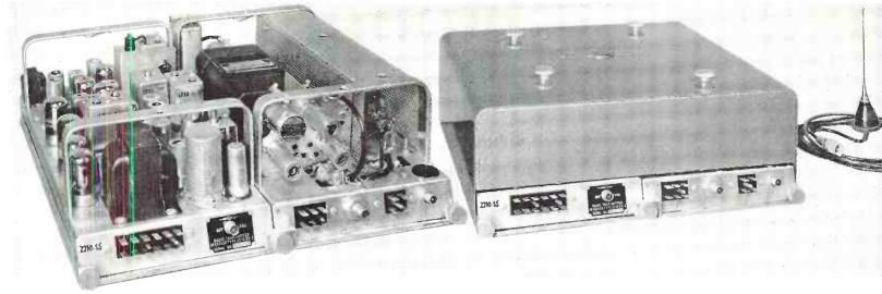
FIG. 1. COMPLETE 450 MC. MOBILE TRANSMITTER AND RECEIVER ARE SHOWN WITH COVER REMOVED AT THE LEFT.
