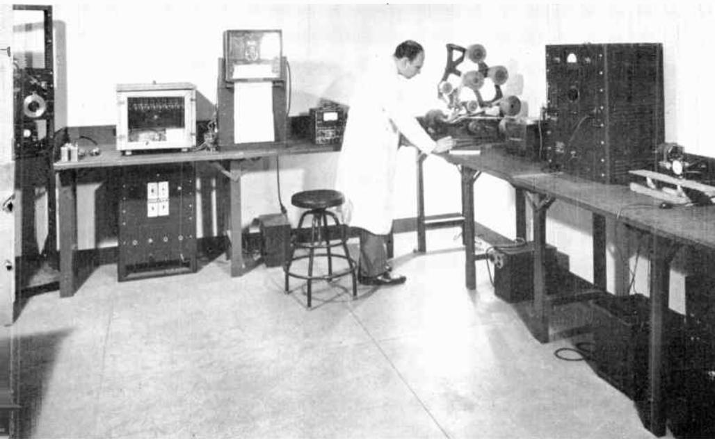
FIG. 17. LEFT TO RIGHT, EQUIPMENT FOR MEASURING POWER FACTOR, ACCELERATED LIFE TEST, AND A CONDENSER WINDING MACHINE FOR MAKING TEST UNITS
