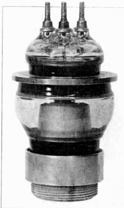
FIG. 3. TYPE 6C22 AMPLIFIER TUBE
