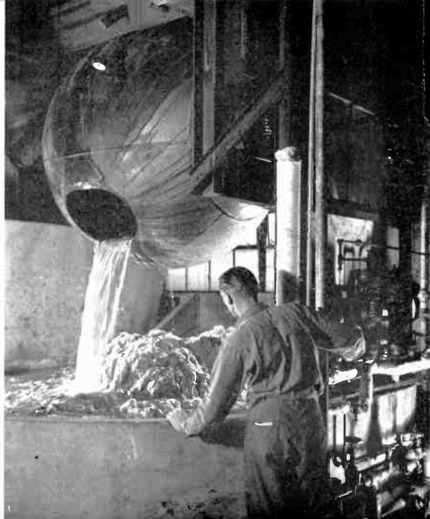
FIG. 4. A BATCH OF STOCK COOKED IN A SMALL LABORATORY BOILER, OR DIGESTER, BEING EMPTIED INTO A WASHER
