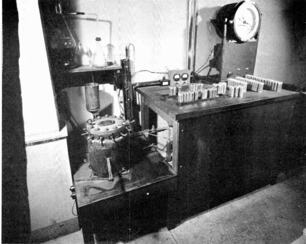
**FIG. 16. A SMALL-SCALE IMPREGNATING TANK IS USED TO MANUFACTURE SAMPLE CONDENSERS SO THAT THE CHARACTERISTICS OF THE PAPER CAN BE TESTED**
