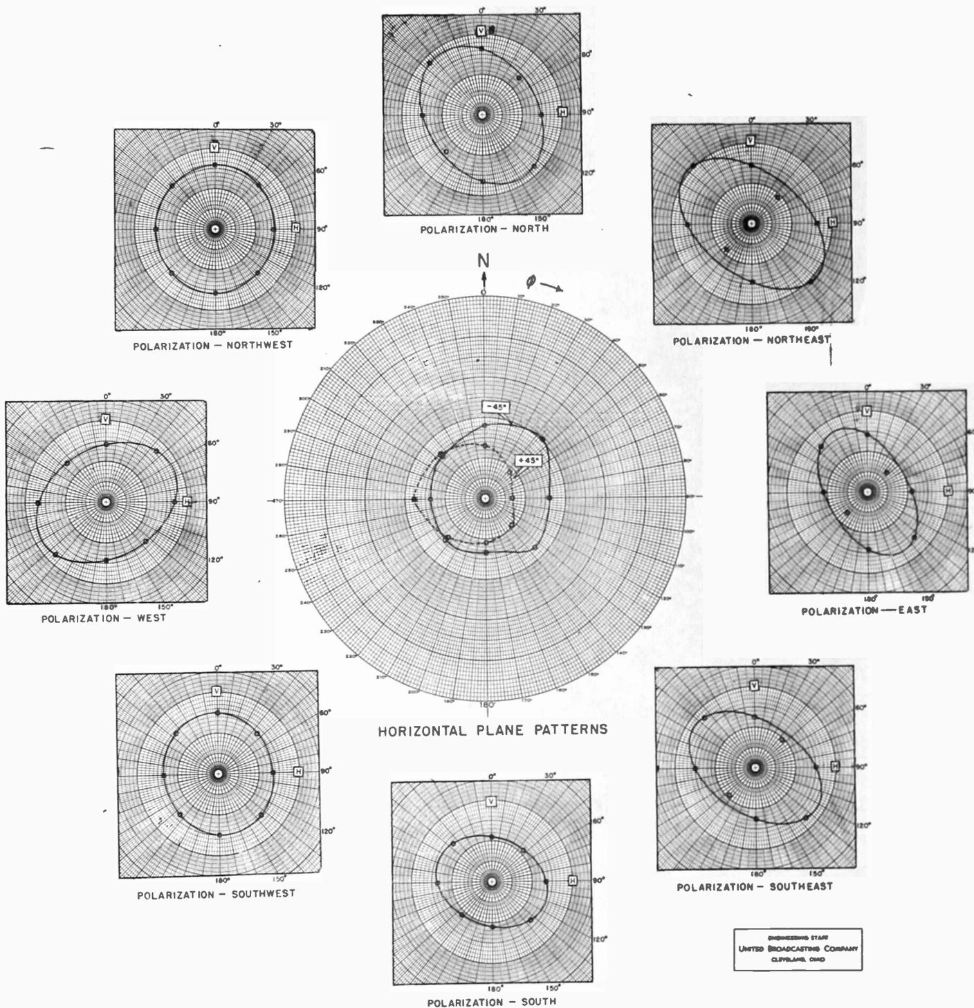
PATTERN AT CENTER SHOWS RELATIVE DIAGONAL POLARIZATION FIELD INTENSITY IN THE HORIZONTAL PLANE AND THE 8 PATTERNS FOR THE INDICATED DIRECTIONS GIVE THE RELATIVE FIELD INTENSITY PATTERN IN THE HORIZONTAL PLANE FOR ALL POLARIZATIONS IN A VERTICAL PLANE AT RIGHT ANGLES TO THE DIRECTION OF PROPAGATION.
