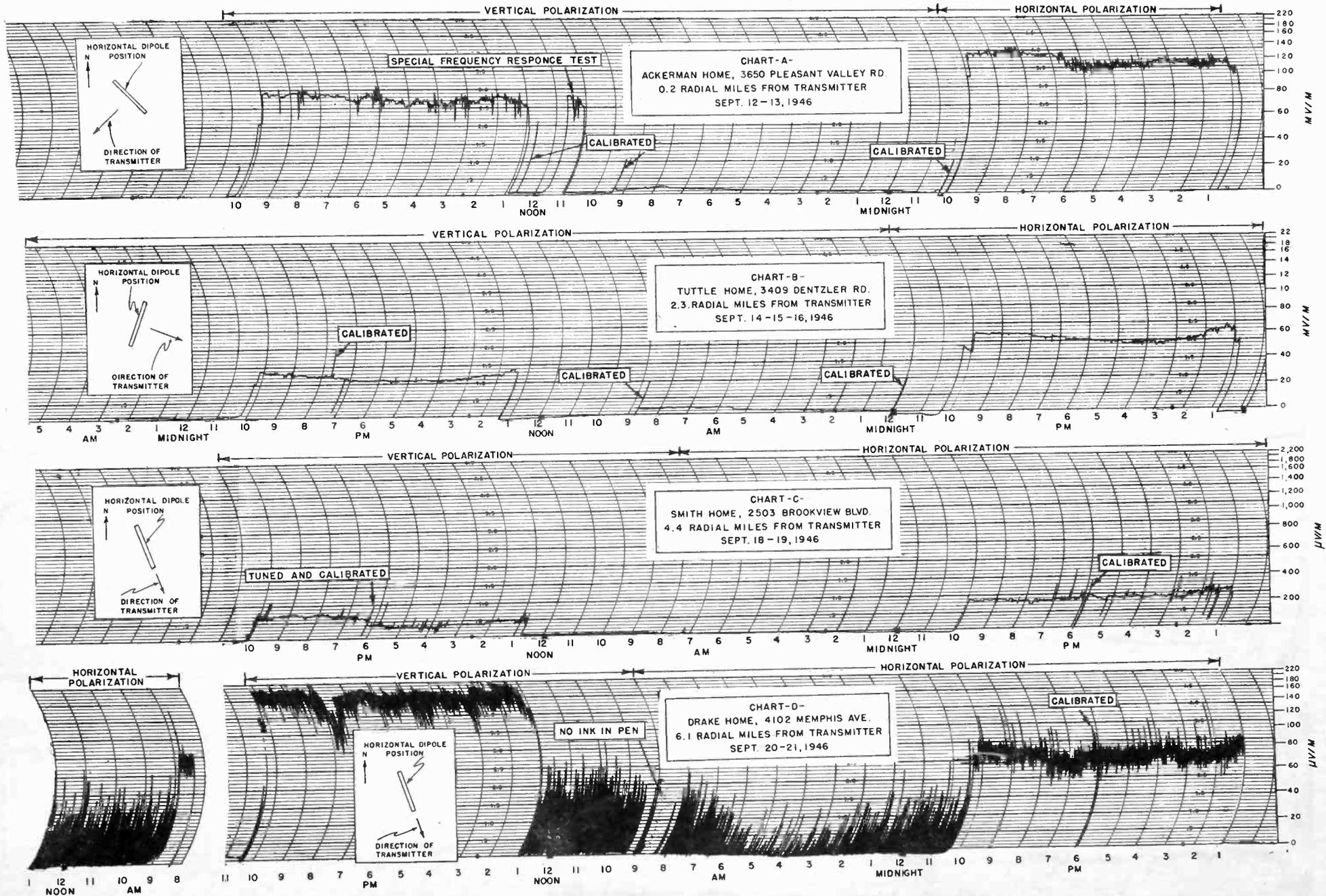
FIG. 24 d.— FIXED POINT RECORDINGS OF CIRCULARLY POLARIZED PROPAGATION
