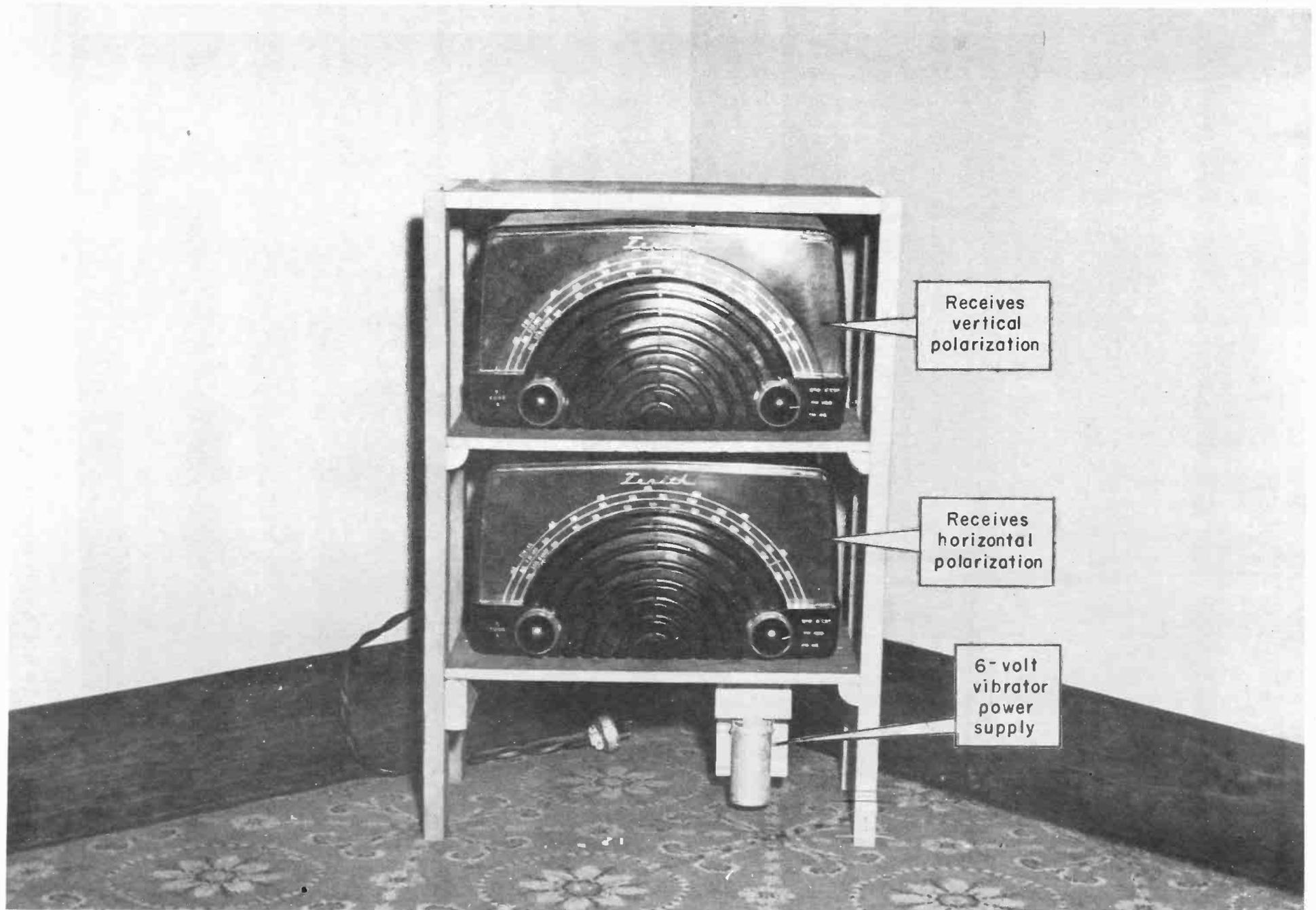
Fig. 17.—Receivers for simultaneous reception of vertically and horizontally polarized waves.
