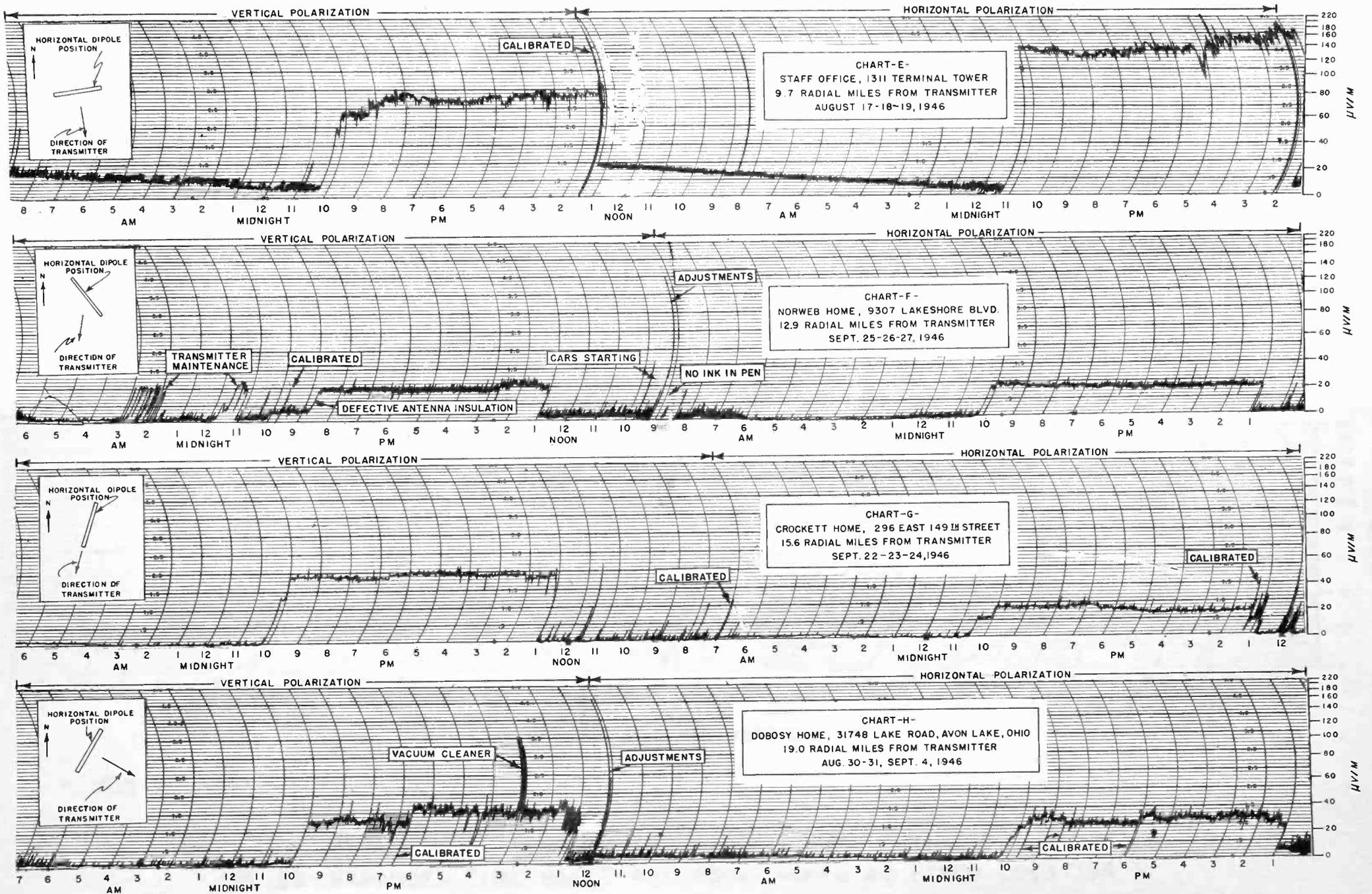
FIG. 24 b.— FIXED POINT RECORDINGS OF CIRCULARLY POLARIZED PROPAGATION
