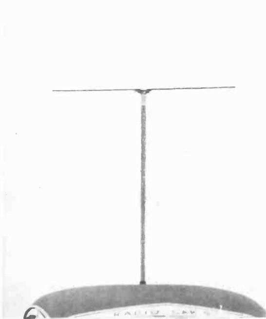
Fig. 13.— Horizontal receiving antenna on field car.
