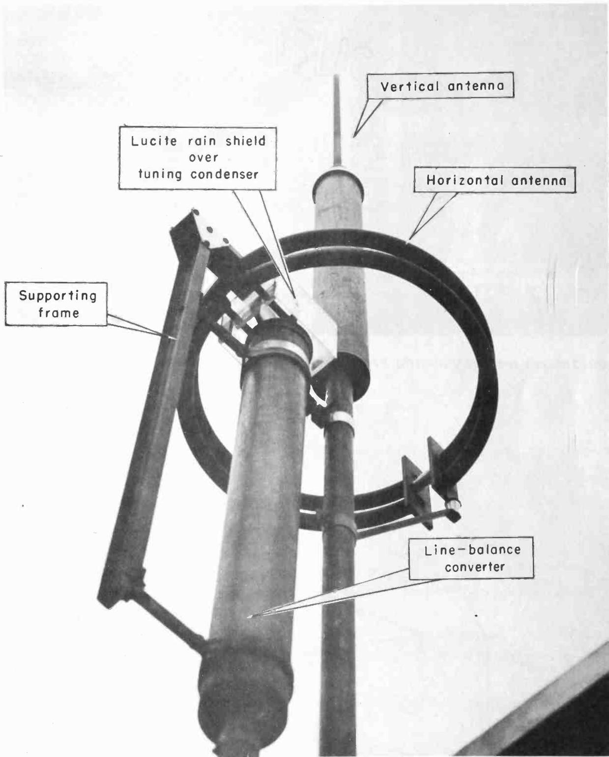
Fig. 5.— Transmitting antenna close-up.
