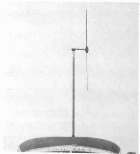
Fig. 14.— Vertical receiving antenna on field car.
