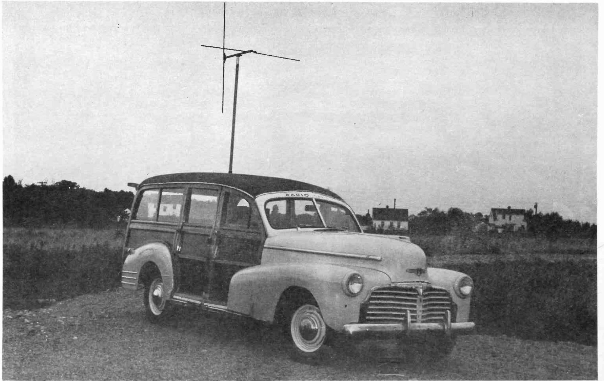
Fig. 10.— Field car showing installation of circular receiving antenna.
