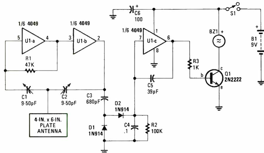
Fig.2—Wave your hand, a finger, or any part of your body to set off this simplified proximity alarm.
