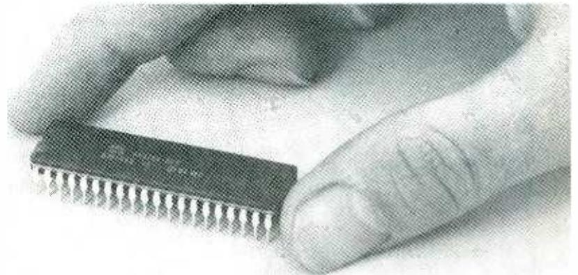
The V-20 microprocessor looks exactly like the 8080. It will function as an 8088 unless specifically software-instructed to emulate an 8080. The software toggles the operating modes.
