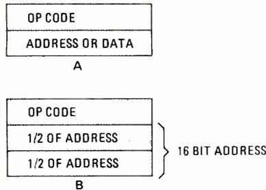
**Fig. 3—A 2-byte instruction puts the complete address or data in one memory location. A 3-byte instruction puts only half the address in a memory location.**
