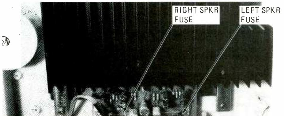
Many amplifiers have a speaker fuse built into in each output channel. Don't replace them with a larger fuse, or wrap tin-foil around the fuse to just "get by" until the store opens.
