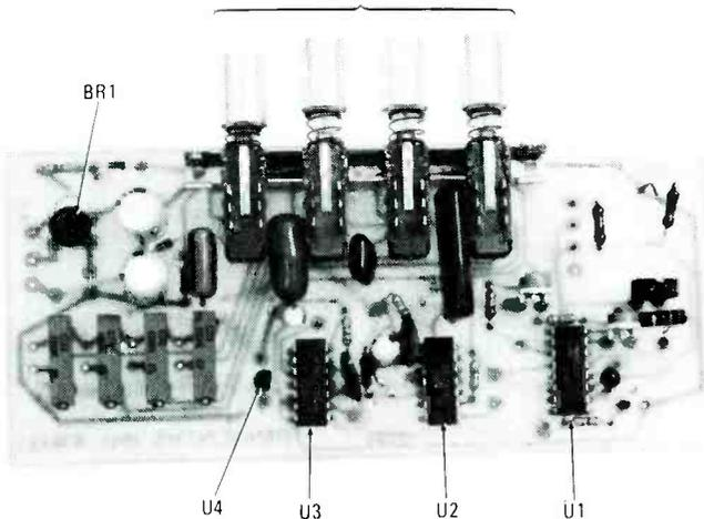
The Function-Generator circuit uses two switch assemblies, one of which is circuit-board mounted to provide support for the board when installed in its enclosure.
