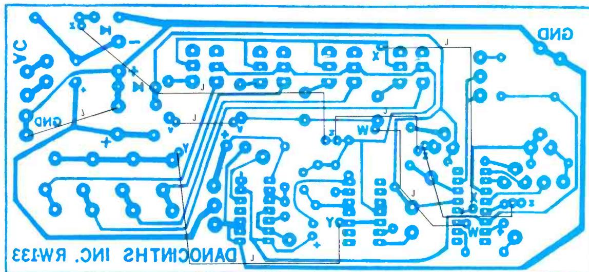
Fig. 5—The five jumper connections can be made on the unclad side of the board prior to component installation or after installation on the copper side of the board as the author did.
