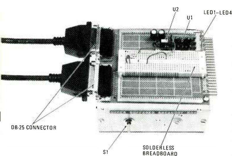
Two female DB-25 connectors mount on the PC board in pre-etched and pre-drilled pads. The solderless breadboard is held in place by 50 J-type wirewrap pins.
