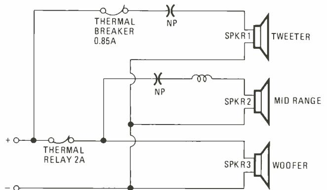
Fig. 3—Many expensive speaker systems use thermal relays or circuit breakers to protect the various speakers. Reduce the volume and wait thirty seconds—with no sound coming from the amplifier—before resetting the overload buttons.
