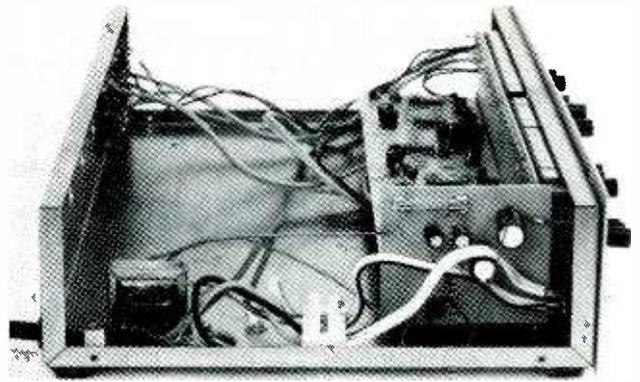
The main circuit board, the power-supply board, and the control board are held together by nothing more than a few blobs of solder, so be very careful once they are joined. The assembly is then mounted with spacers and held in place by six screws and nuts.
