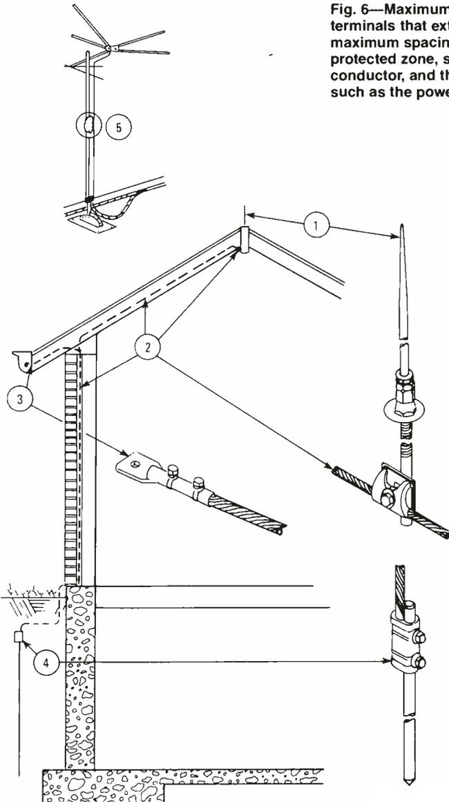
**Fig. 6—Maximum lightning protection involves: 1) Spacing of the air terminals: air terminals that extend at least 10-in. above the protected object are located at a maximum spacing of 20-ft. 2) Conductor size; 3) Bonding of metal bodies not within the protected zone, such as rain gutters; 4) A grounding system connection at each downconductor, and the interconnection with utility grounds; 5) Protected external wiring, such as the powerline, TV antenna cable, and telephone and data wires.**
