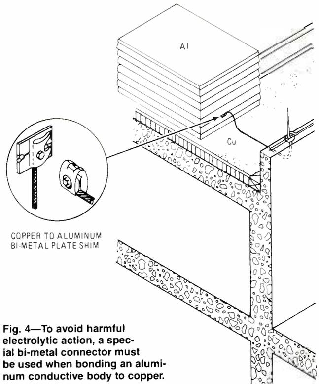
**Fig. 4—To avoid harmful electrolytic action, a special bi-metal connector must be used when bonding an aluminum conductive body to copper.**
