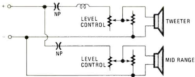
**Fig. 4—Mid-range and tweeter speakers in multi-speaker systems may be protected with level controls located on the front or rear panels. The right amount of high and mid-range level balance can be attained using those controls.**
