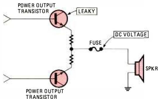
**Fig. 1—The speaker's voice coil can be damaged by a leaky power-output transistor (or integrated circuit) if the speaker isn't properly fused. Keep in mind that replacing the speaker fuse with another unit having a larger ampere rating might offer no protection to the speaker at all.**
