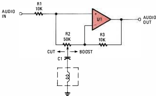
**Fig. 1—Early equalizers used inductors in the circuit's design. The inductors were expensive, bulky, tedious to wind, and the multiple-tuned circuits had a tendency to interact with each other.**
