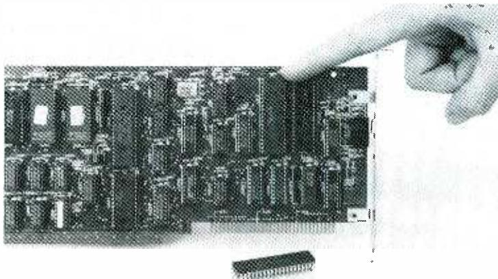
To retrofit consists of simply locating your computer's 8088 and then substituting the V-20 microprocessor.
