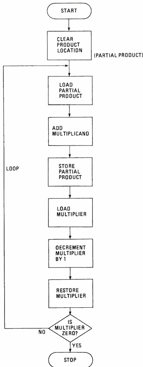
Fig. 6—A flowchart shows that multiplication is actually done by repeated addition.
