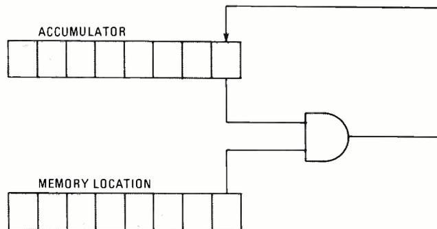
Fig. 7—The AND instruction is designated ANDA which means to AND the contents of accumulator A with the contents of the memory location designated in the instruction.
