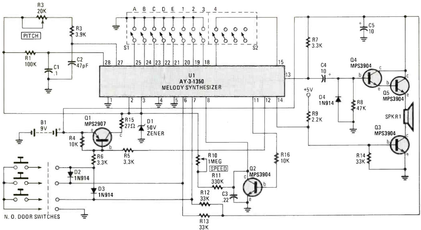
Fig. 1—Both the melodies and the chime effects are generated by integrated-circuit U1. However, potentiometers R3 and R10 determine the pitch and the speed of the melody.
