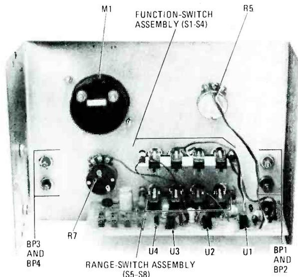
All off-board components are mounted to the front panel of the enclosure, along with the circuit board, which is held in place by the switch-assembly's mounting hardware. Connections between the circuit board and the off-board components are then completed through hookup wire.
