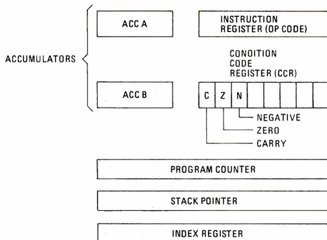
Fig. 2—This is the basic register organization in the 6800 microprocessor. Note that there are two accumulators.
