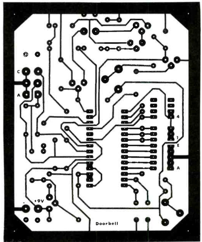
Fig. 2—In addition to holes for the components, the printed-circuit board contains larger openings for the plastic ties used to secure the wires from the door switches.
