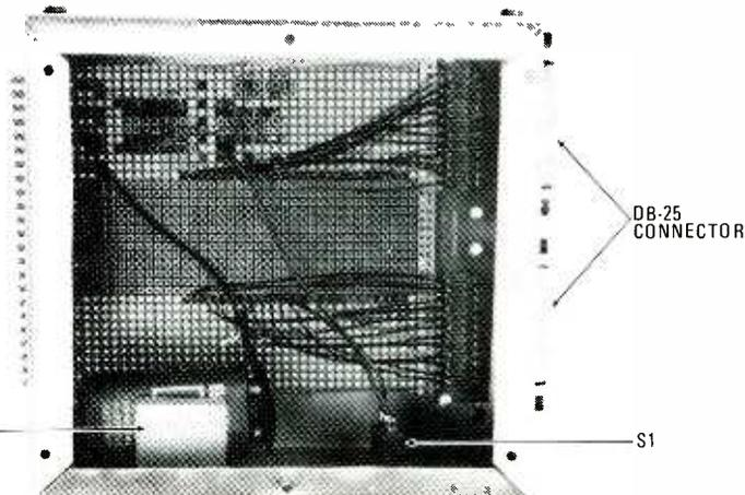
All of the electronic components mount in the upper left corner of the circuit board; then they're interconnected with wirewrap wire.
