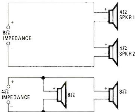
**Fig. 5—The total speaker impedance is 4 ohms when two 8-ohm speakers are connected in parallel. The total impedance is 8 ohms when two 4-ohm speakers are connected in series.**
