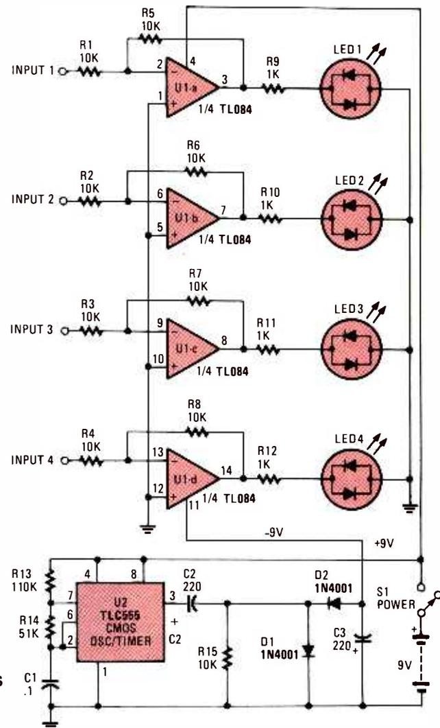
**Fig. 1—Four buffered tri-color LED's provide high/low indication of RS-232 signal lines, while the TLC555 CMOS timer/oscillator circuit provides a -9-volt DC source.**
