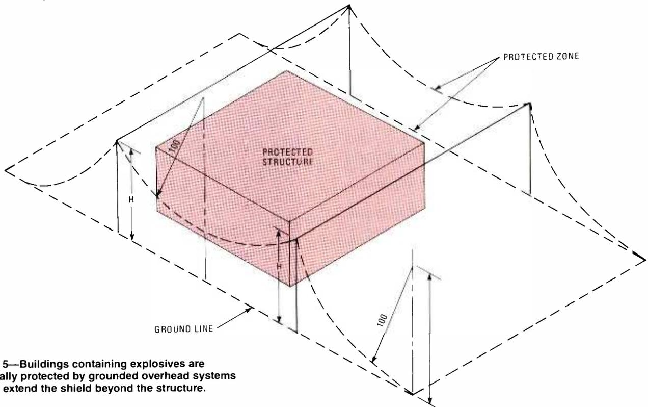
**Fig. 5—Buildings containing explosives are usually protected by grounded overhead systems that extend the shield beyond the structure.**
