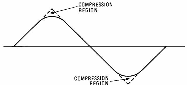
**Fig. 2—A triangular wave is fed to a sinewave-shaper circuit, which clips and rounds off the peaks (shown as a dashed line curve) of the input waveform to provide a sinewave output.**
