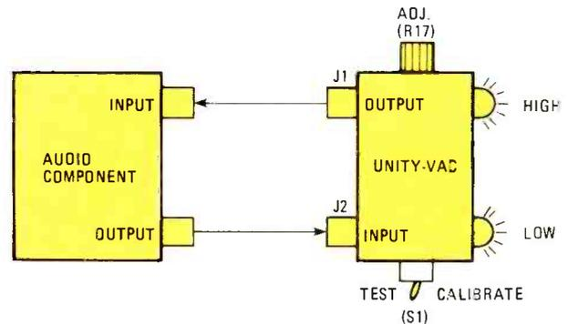
Fig. 3—After calibration, Unity-Vac is connected to the unit-under-test as shown. Unity-Vac's signal from the noise generator is then fed as a reference to the comparator circuit. That signal is also routed through J1 to the audio component and back to Unity-Vac. Depending on the condition of the returning signal, one or the other LED will be on while one is off, or both will flicker.
