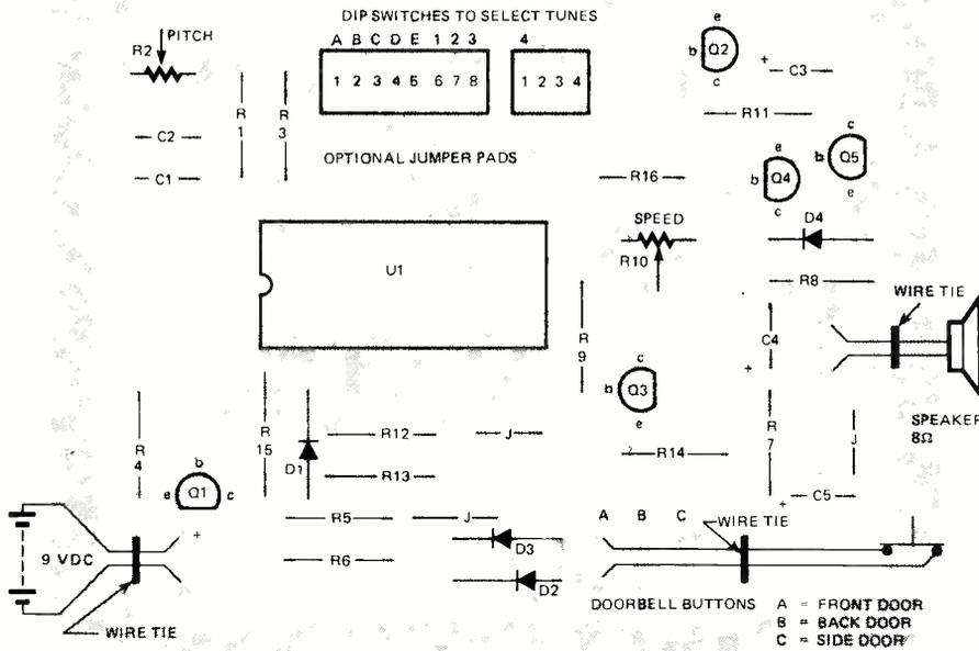
Fig. 3—Be very careful, when installing the components on the printed-circuit board that you position U1's "notch" correctly. The notch should point toward the nearest edge of the printed-circuit board; away from speed potentiometer R10.
