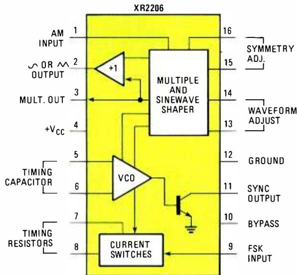
**Fig 1—Functional block diagram of XR2206 single-chip function generator. The chip, along with a few support components, is all that's needed to produce a reliable test instrument.**
