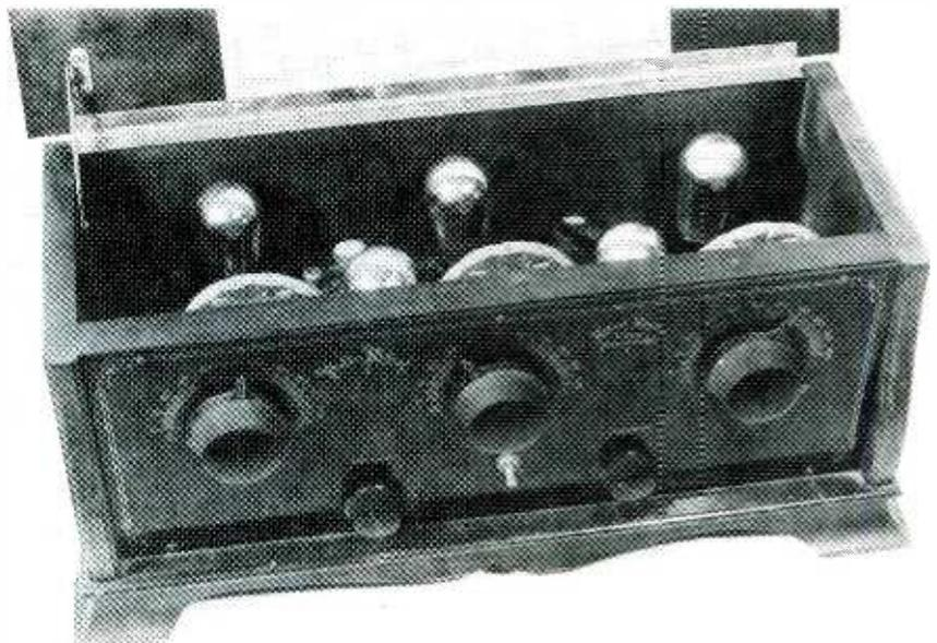
The Polle Royale is a 5-tube battery set of about the same era as the Radiola III. A staggered tube arrangement gave it an unusually compact "footprint" for its type.
