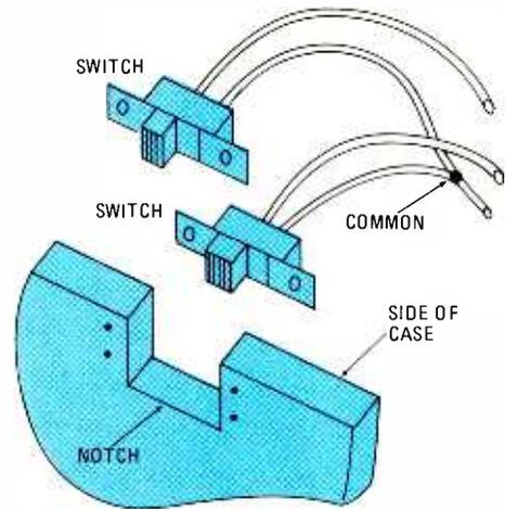
Fig.2—Cut individual notches for each switch in the side of the case. Don't attempt to gang the switches in a single notch because the switches must be rigidly mounted.
