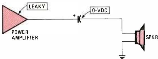
**Fig. 2—Amplifiers having a large coupling capacitor between the power output stage and the speaker will not place a DC voltage on the speaker if the amplifier is leaky; however, excessive high volume or abnormal sounds (filed with sharp peaks) may still destroy the speaker's voice coil.**
