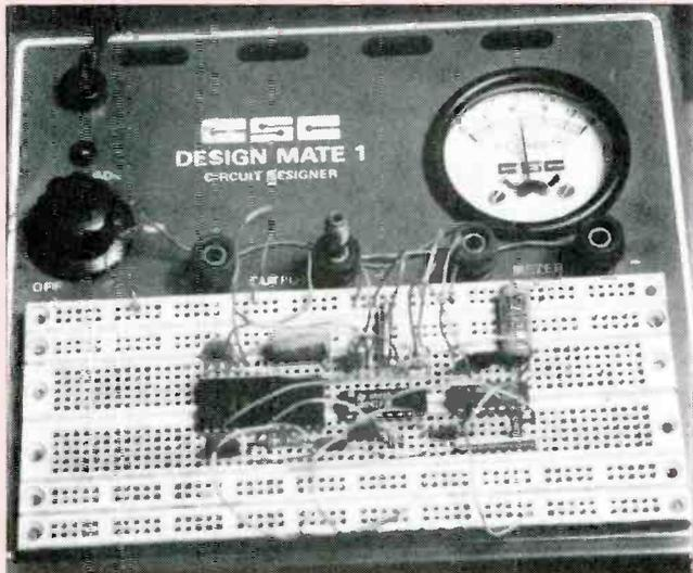
If you're substituting parts, make certain they aren't working in a very narrow voltage range. For battery-powered circuits, use a variable supply to test the complete range of voltages expected as the battery ages.
