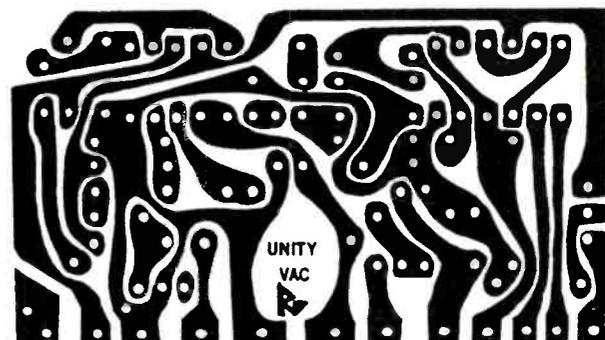
Fig. 4—The author built Unity-Vac on a small piece of printed-circuit board, for which a template is shown. It may be copied or lifted from the page to produce your own circuit board.
