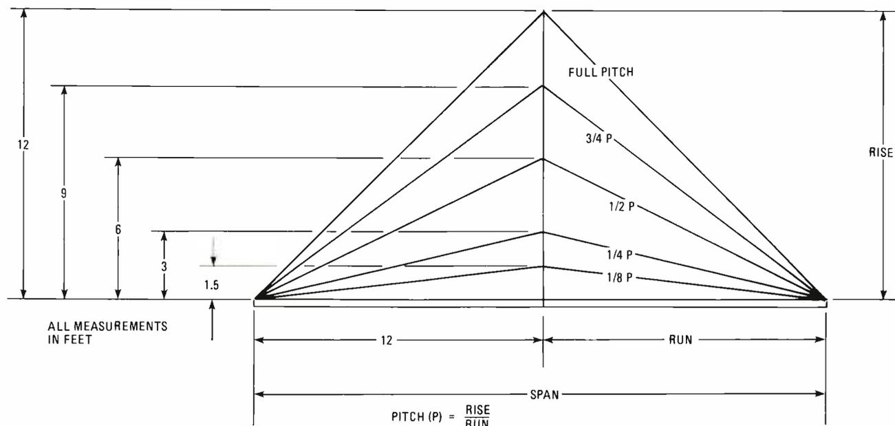
Fig. 3—The span of a roof and its rise determines the location and number of air terminals needed. Flat roofs require air terminals along the edges, and at the corners.
