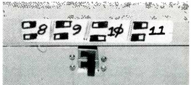
Apply a small drawing directly above the switches indicating the correct setting for the various drive assignments.
