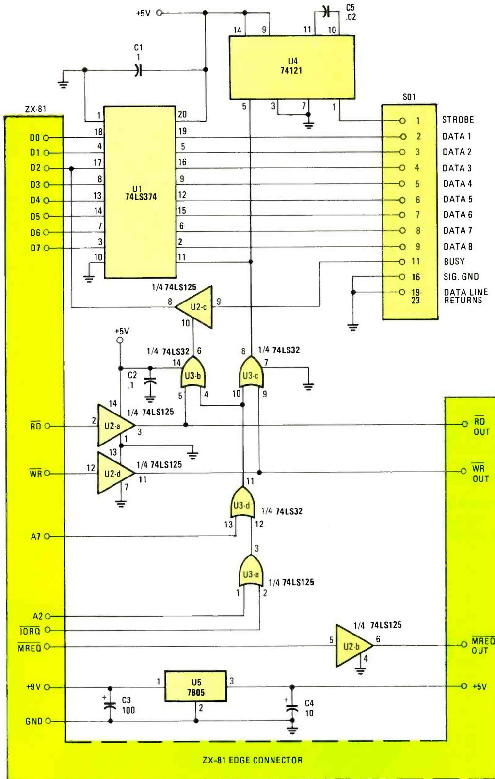
Fig. 2—The ZX-81's connections on the top and bottom of the system connector are different. Make certain that you get them right the first time—you might not get a second chance.
