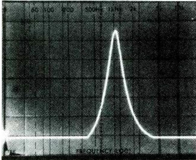
**The Playmaster Equalizer is capable of boosting or cutting the frequency in any of its 10 bands by as much as 12 dB. Note that maximum gain is centered around the resonant frequency; in this case, the 1-kHz band. Gain is decreased as the signal moves away from resonance.**
