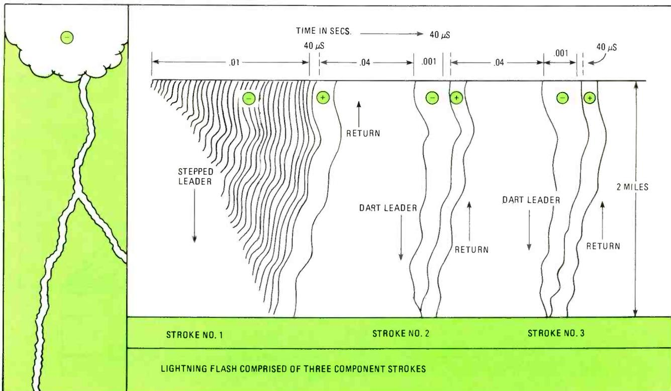
Fig. 1—Although a lightning strike appears to be a single flash, in actual fact it consists of three individual strokes, each having a *leader*—a downward negative stroke—and a *return*—a positive upward stroke.
