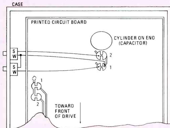
Fig.1—This figure is not to scale and not proportional. It is specifically intended to help you locate the drive-select solder pads by showing only their shape and relative location.
