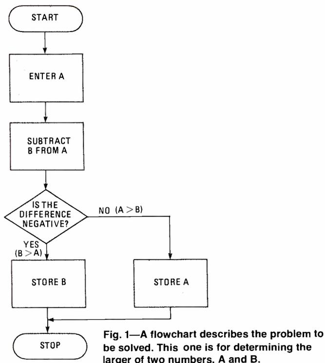
Fig. 1—A flowchart describes the problem to be solved. This one is for determining the larger of two numbers, A and B.
