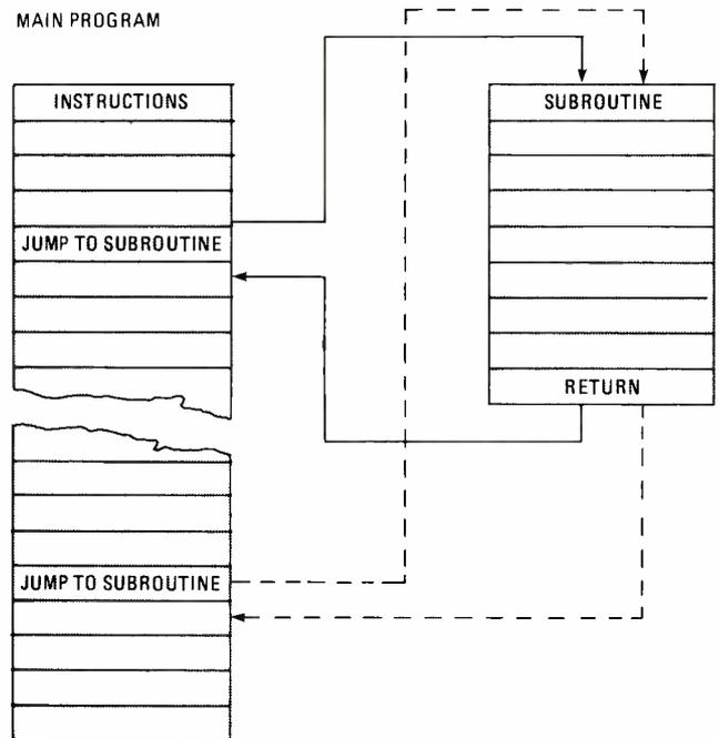
Fig. 5—A small program which will be used many times by the main program can be stored as a subroutine, to which the main program jumps (and returns) when it's needed.
