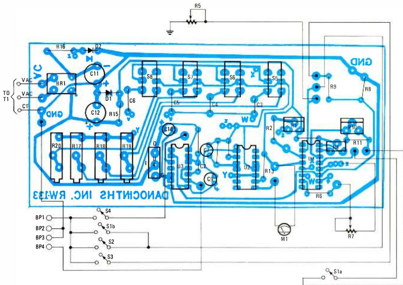
Fig. 6—When used in conjunction with the template in Fig. 4, plus the jumper-positioning guide in Fig. 5, this layout makes putting the circuit together a simple task.
