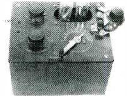
The RCA Radiola III is a good example of an early 2-tuber. It has a regenerative detector and a one-stage audio amplifier.
