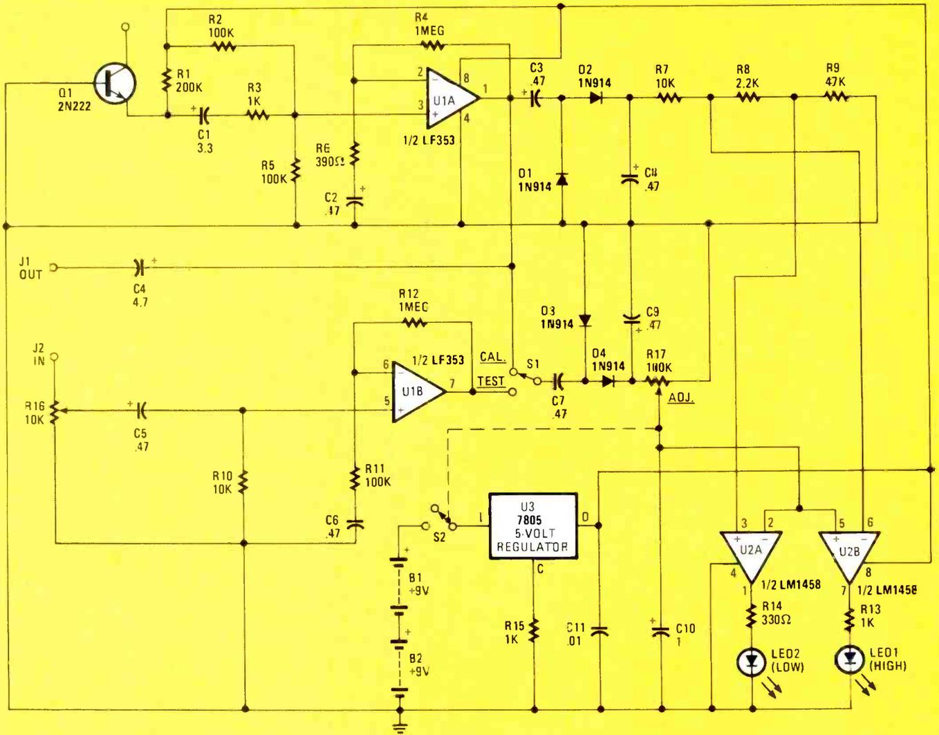
Fig. 2—The schematic diagram reveals that the noise-generator portion of the circuit is really nothing more than a reverse-biased general-purpose, Q1. You'll also note that our comparator circuit is actually two comparators: one configured as negative comparator and the other as a positive one. Each comparator drives an LED to indicate the condition of the input signal.
