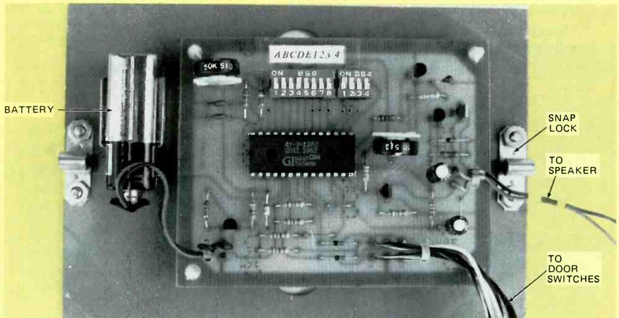
The printed-circuit assembly is installed on the cabinet's rear panel using stand-off insulators at each corner. The battery is held in place by a small clamp. The cabinet latch at each end of the panel will secure the panel to the cabinet.
