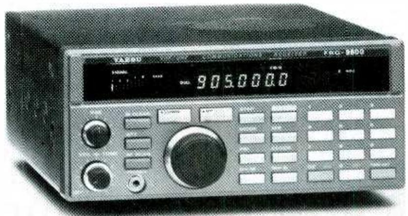
The Yaesu FRG-9600 communications receiver does the work of a scanner and is tuneable from .905 to 60 MHz. It detects both narrow- and wide-band FM, CW, AM, and SSB.
