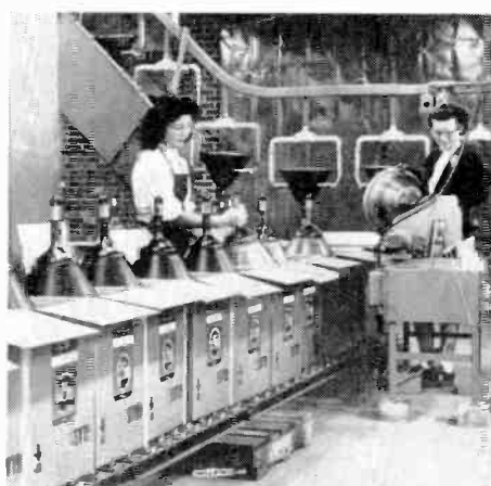
15. Having received the stamp of approval, the tube is given a final polish and placed in its shipping carton.
