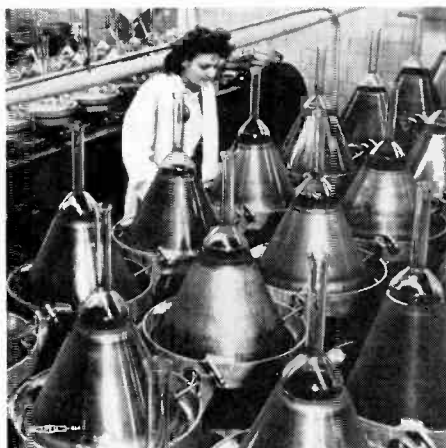
5. Metal tubes are placed on a crawling conveyor belt to permit the phosphor to settle on the face-plate.
