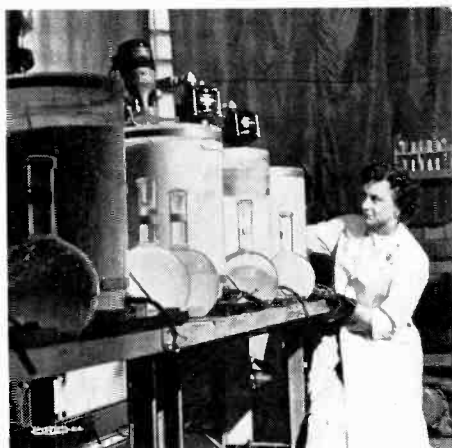
4. Purity of the phosphor solution is rigidly inspected to prevent the entrance of injurious foreign material.
