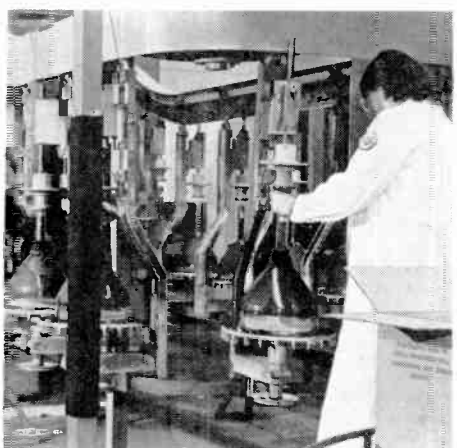
13. After the tube has passed all tests it is given its final washing before paint is applied to the outside.
