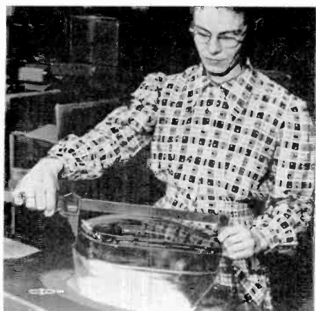
1. Manufacturing process begins with inspection of all parts comprising the tube, whether glass or metal-shell type.
