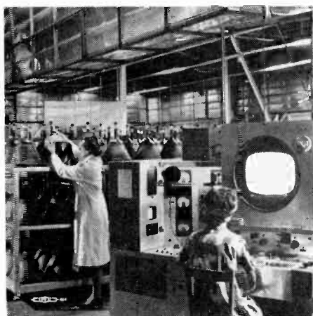
11. As a tube approaches completion it is tested for picture brightness under home lighting conditions.
