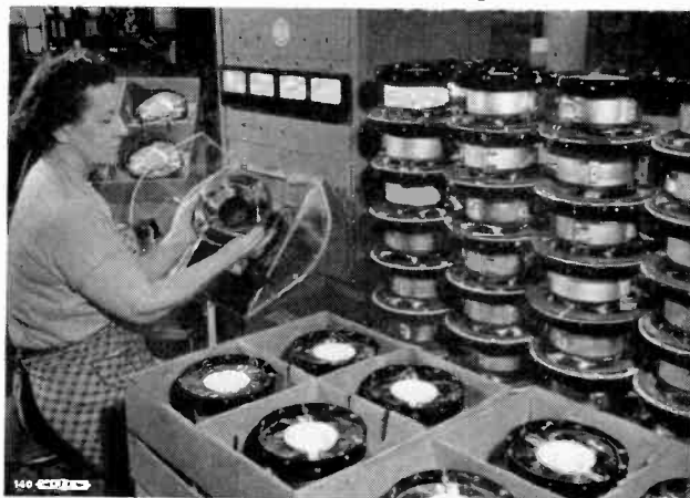
COLOR TV deflecting yokes roll off production line at RCA's Camden, N. J., plant. Yoke is designed for use with RCA tricolor picture tube in home color receivers, and is being produced in quantities to meet needs of manufacturers who are expected to produce 100,000 color sets this year. Deflecting yoke is vital element in scanning operation, during which tricolor tube's three electron beams "paint" color pictures on tube screen. Above, RCA color yokes undergo electrical test as they near end of production.
