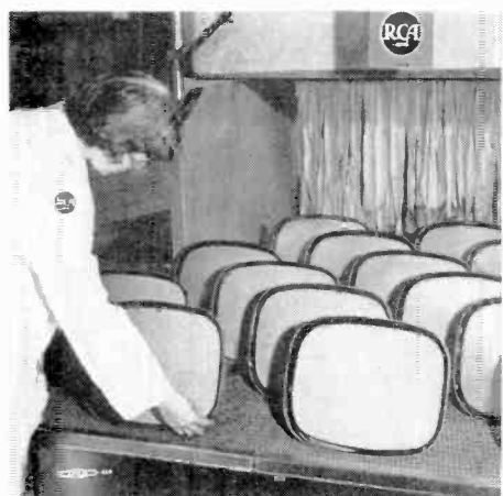
7. Kinescopes are baked in huge ovens to "boil" out impurities and to dry the inside graphite coating.
