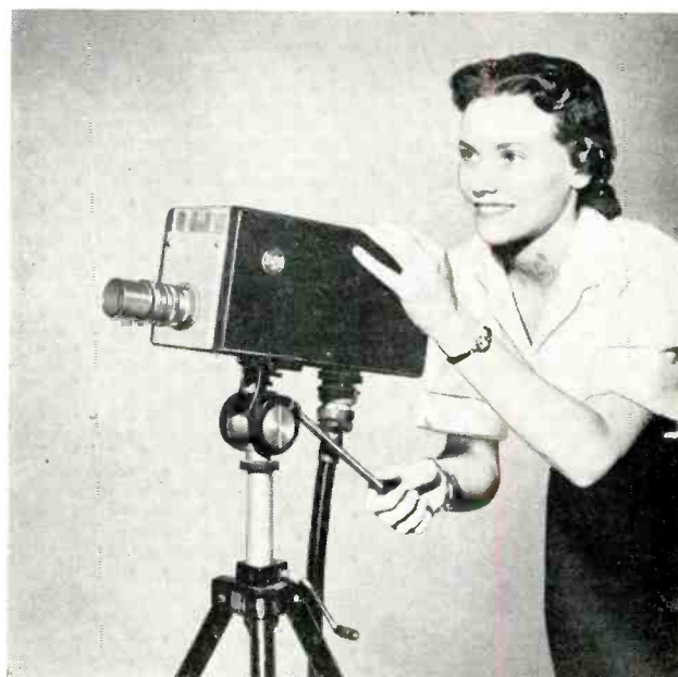
A model demonstrates the new ITV-201 camera produced by RCA for use with closed circuit networks. The camera is useful in educational, industrial, and commercial work.
