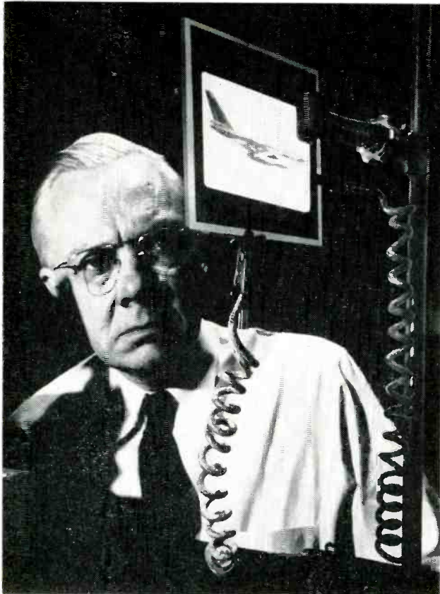
An image-producing panel is put through laboratory tests by Dr. Keith Butler, manager of general engineering laboratories of Sylvania's Lighting Division. This "Sylvatron" unit converts electrical data into simultaneous dots of light.
