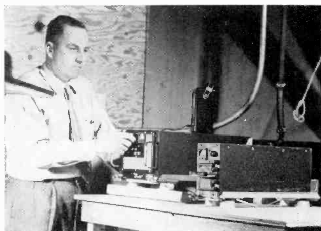
ABOVE: Gerald King-Ellison checks the voltages on the transmitter-receiver unit used in radar weathercasting. The Synchro-power supply unit is on the right.
