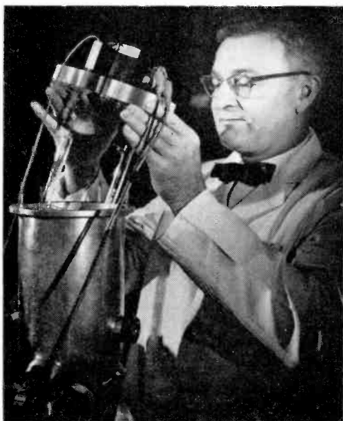
A krypton-86 lamp is lowered into its liquid nitrogen bath. Its light is "laid" alongside the meter bar that has already been mechanically determined to an accuracy of less than one wave-length.
