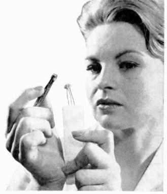
Nanita Greene inspects the cap and internal structure of a valuable addition to RCA's family of transistors. Dubbed the "Siamese-Twin," it incorporates revolutionary design and construction principles in which it combines two identical transistors capable of boosting ten-fold the voltage of a standard car battery. Two transistors formerly were required to achieve the same performance.
