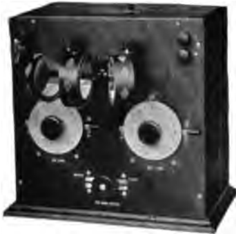
TYPE T-200 Multi-Wave Tuner Wave Length, 150-25,000 Meters
