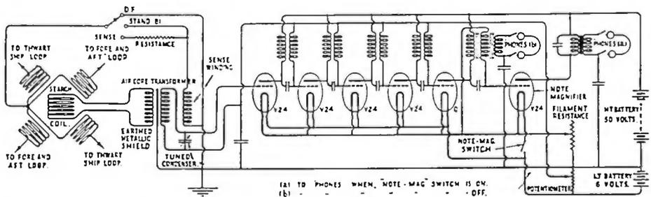
FIGURE 10—Two Small Variable Calibrating Chokers Are Omitted for Sake of Clearness. (These Are Actually Connected in Each Side of Fore and Aft Loop Circuit)
