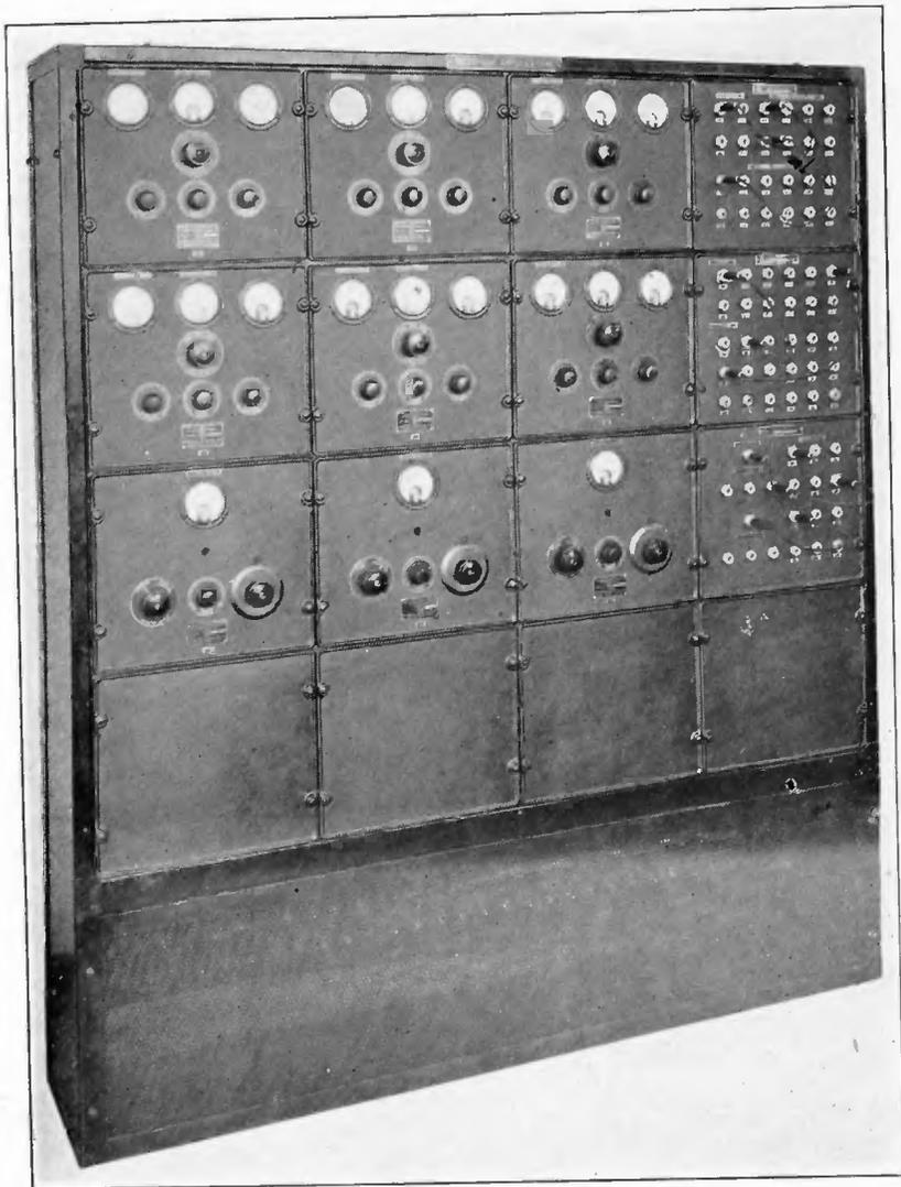
FIGURE 68—5 Watt Amplifier Bank (Microphone Amplifier)
