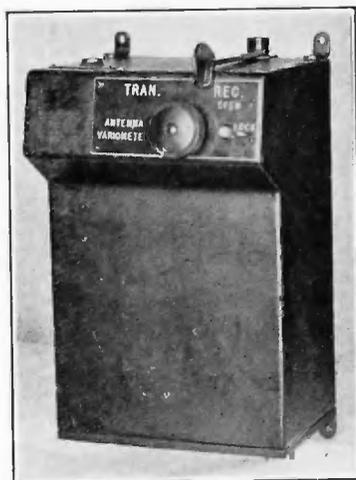
FIGURE 49—Radio Control Box for Air Mail Plane
