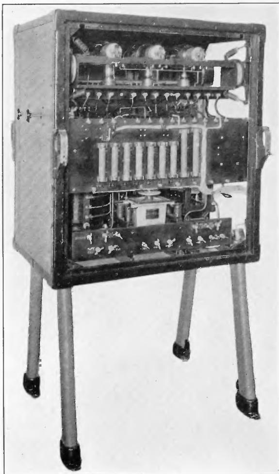
FIGURE 45—400-Watt Portable Radio Transmitter SCR-132 (Rear Panel Removed)
