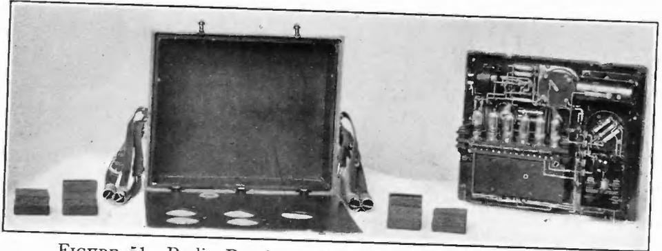
FIGURE 51—Radio Receiver—Air Mail Plane (Disassembled)
