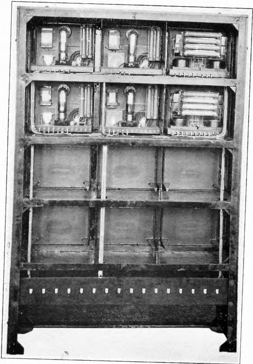
FIGURE 71—50-Watt Amplifier Rack (Intermediate Amplifier Bank)
