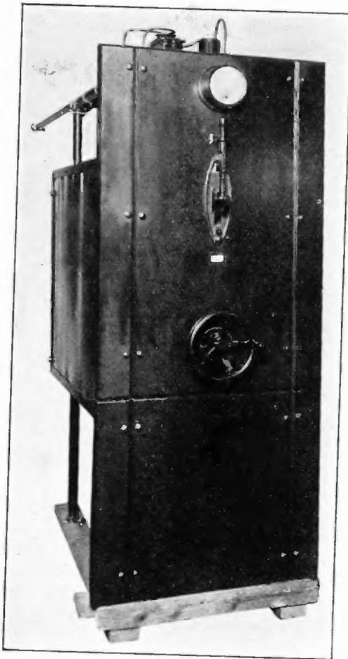
FIGURE 65—Grid Tuning Unit (Front View)
