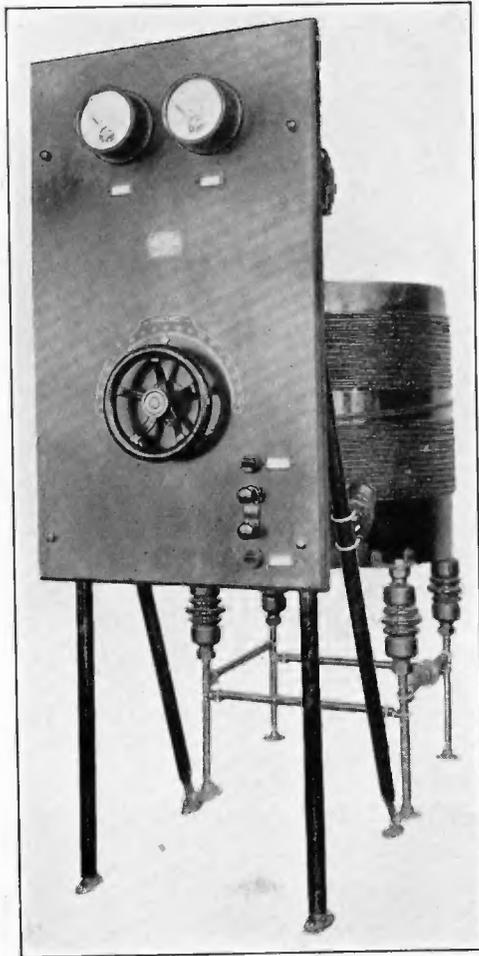
FIGURE 19—Intermediate Circuit Variometer, Front View
