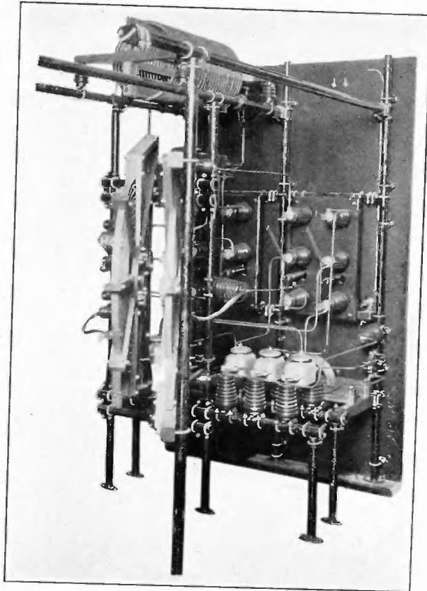
FIGURE 67—Oscillator Tuning Unit (Rear View)
