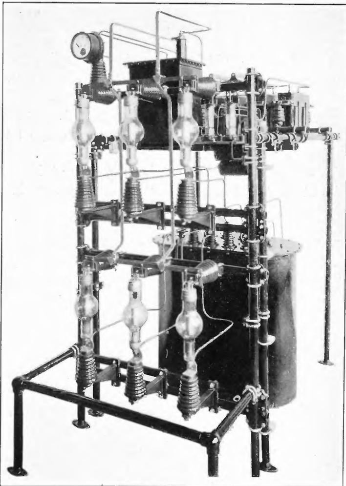
FIGURE 22—Kenotron Rectifier Unit (Signal Corps) Type RA-6
