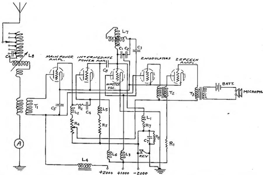
FIGURE 41—Schematic Diagrams of Connections Radio Transmitter BC-127
