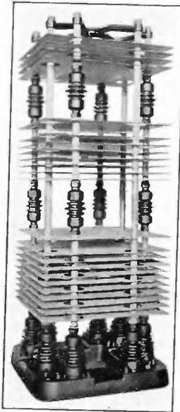
FIGURE 29—Intermediate Circuit Condensers (Signal Corps)
