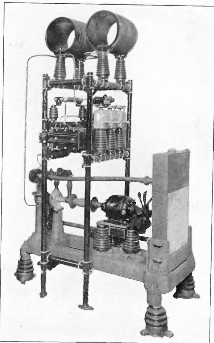
FIGURE 14—20-KW. (Radiotron UV-207) Water Cooled Tube Unit (Side View)
