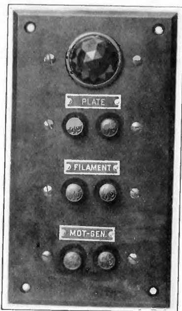
FIGURE 20—Operators' Control for Use with 20-KW. Transmitting Equipment
