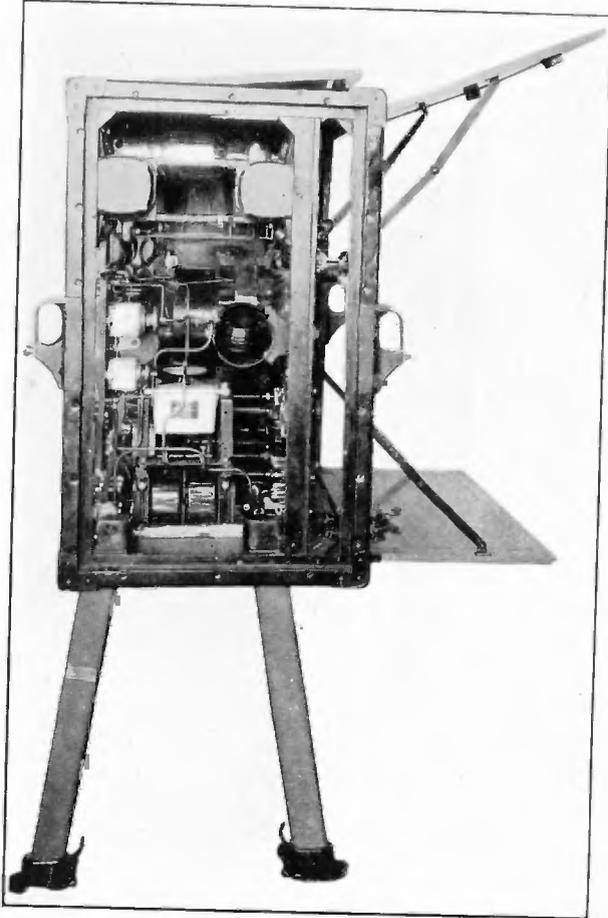
FIGURE 44—400-Watt Portable Radio Transmitter SCR-132 (Left Side Panel Removed)
