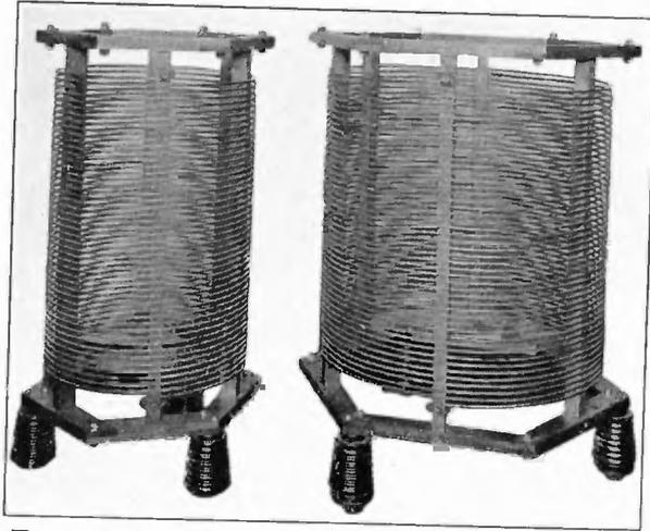
FIGURE 28—Antenna Loading Coils (Signal Corps) ID-6 and ID-7
