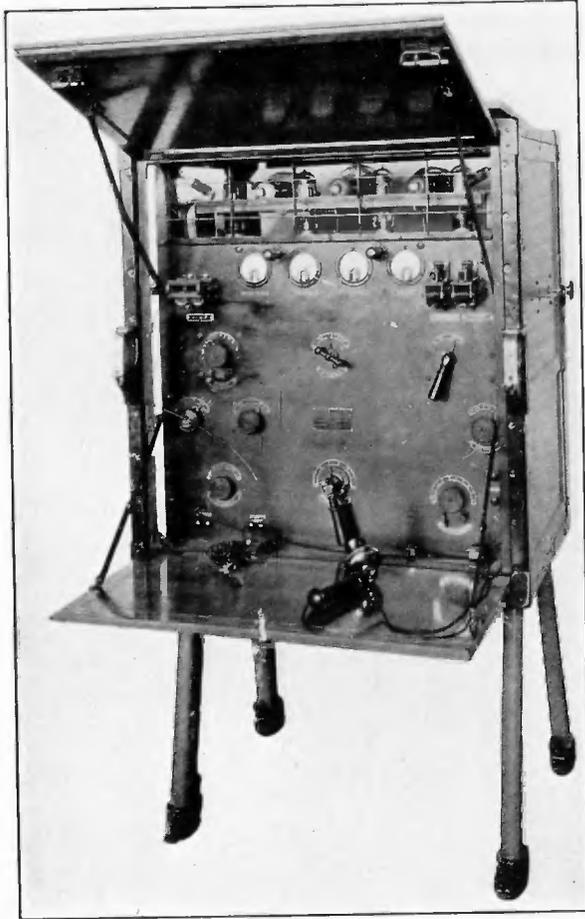
FIGURE 43—400-Watt Portable Radio Transmitter SCR-132 (Front View)
