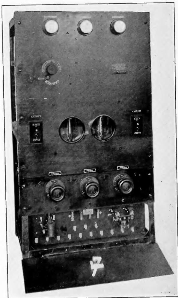
FIGURE 55—Radio Fog Signal Tube Transmitter
