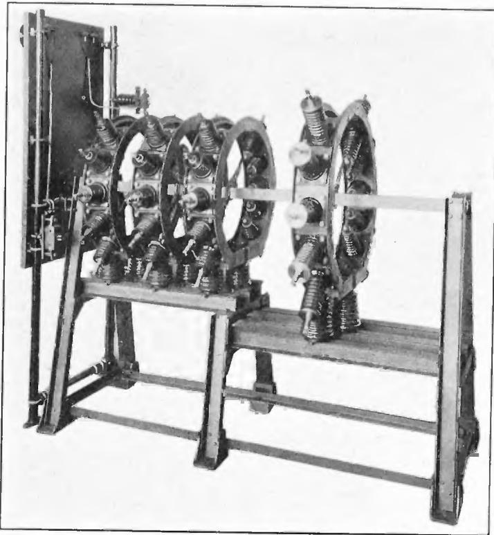
FIGURE 26—Wave Change Switch (Signal Corps) Type SW-83 (Side View)
