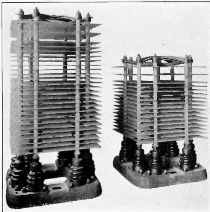
FIGURE 16—High Voltage Air Condensers
