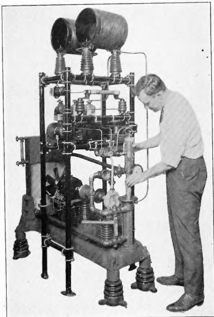
FIGURE 15—20-KW. (Radiotron UV-207) Water Cooled Tube Unit
