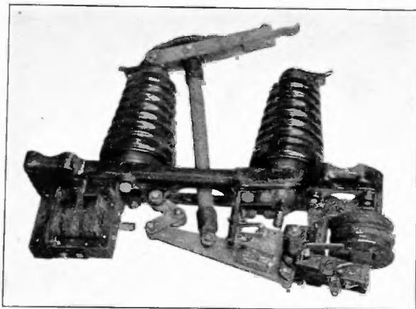
FIGURE 18—High Voltage Disconnecting Switch (Solenoid Operated), 25,000 Volts
