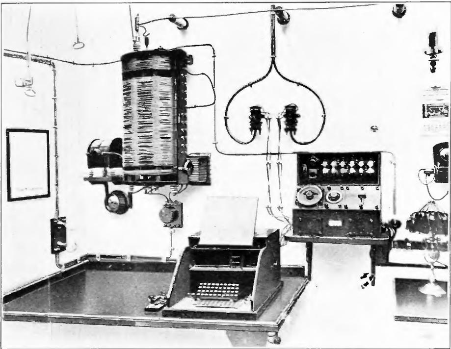
FIGURE 6—Connections of Radiogoniometer. (Inside Wireless Room).
