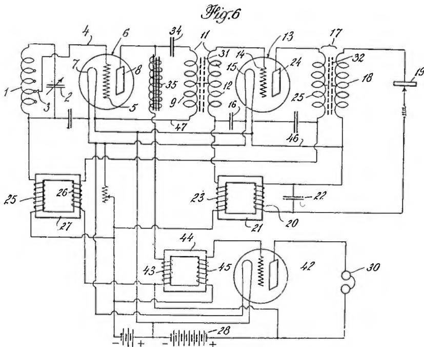
NUMBER 1,517,058—Inverse Duplex Vacuum Tube Circuit
