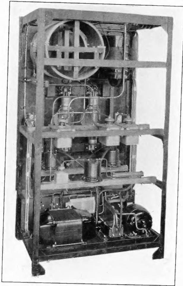
FIGURE 56—Radio Fog Signal Tube Transmitter
