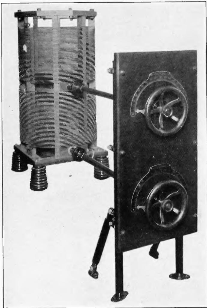
FIGURE 25—Master Oscillator Inductance (Signal Corps)
