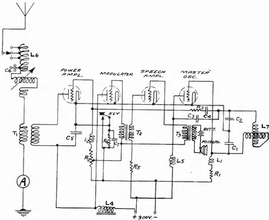
FIGURE 40—Schematic Diagram of Connections Radio Transmitter SCR-136
