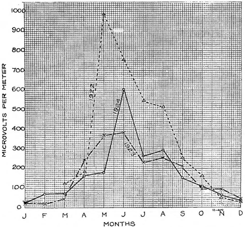
FIGURE 6—Average Atmospheric Disturbances 3 P.M. for 1922–1923–1924
