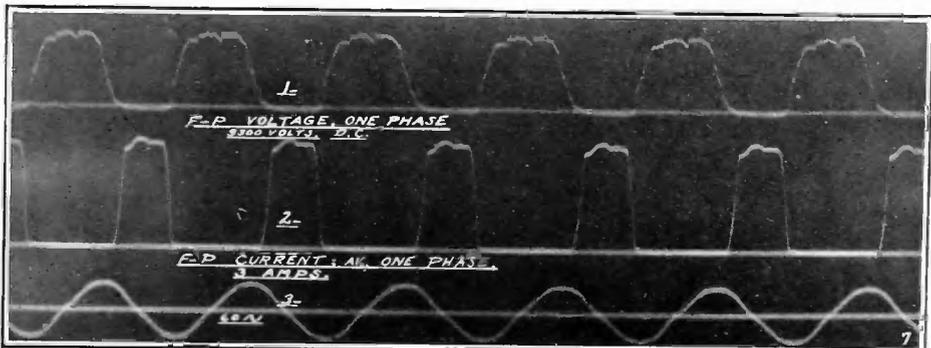
FIGURE 31—Oscillogram Showing Current and Voltage for the Rectifier Tubes in One of the Six Phases
