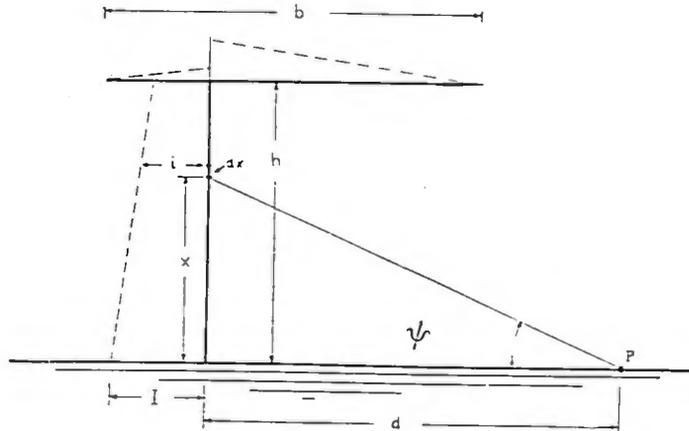
FIGURE 3—Flat-top Antenna—Linear Current Distribution
