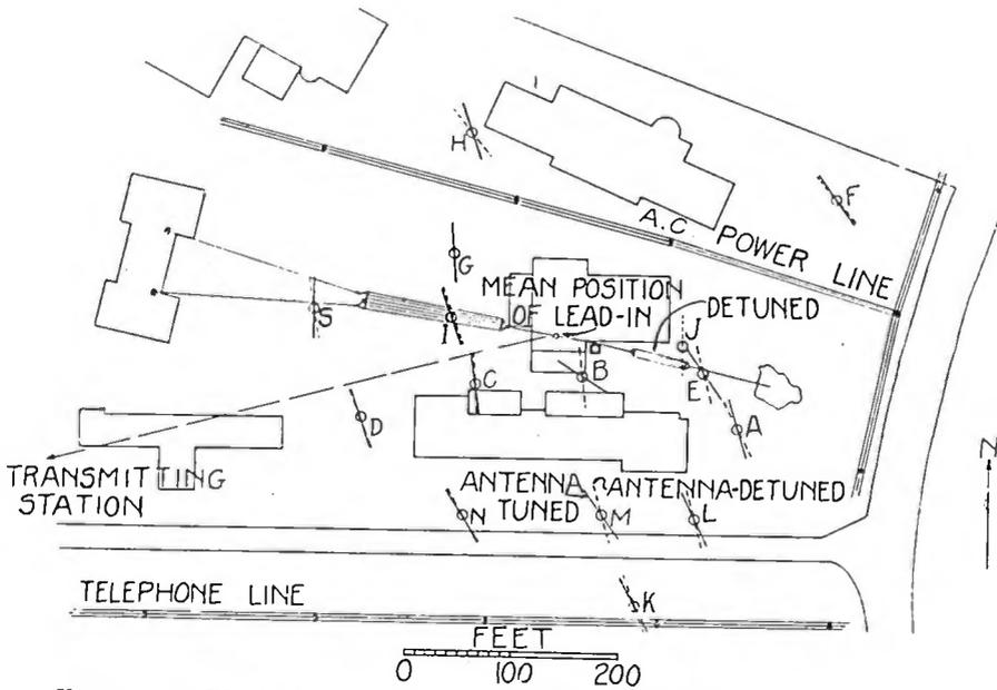
FIGURE 8—Field Distortion Due to Tuned Antenna at University of Minnesota
