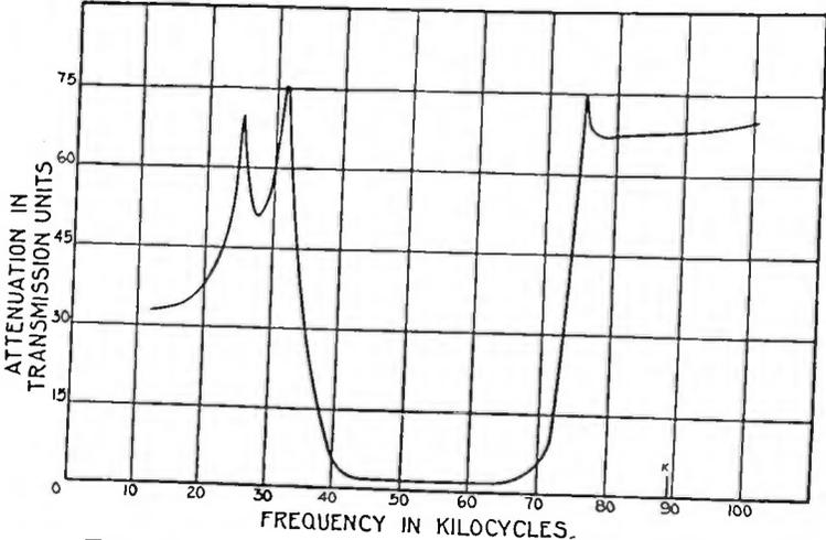
FIGURE 11—Attenuation Curve of Second Filter
