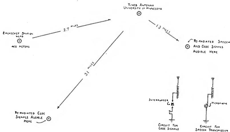
FIGURE 9—Transmission Without Local Power by Re-radiation
