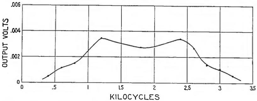
FIGURE 16—Amplitude of the Sideband Frequencies at the Output Terminals of the First Filter as a Function of Modulating Frequency. Input at All Frequencies Constant
