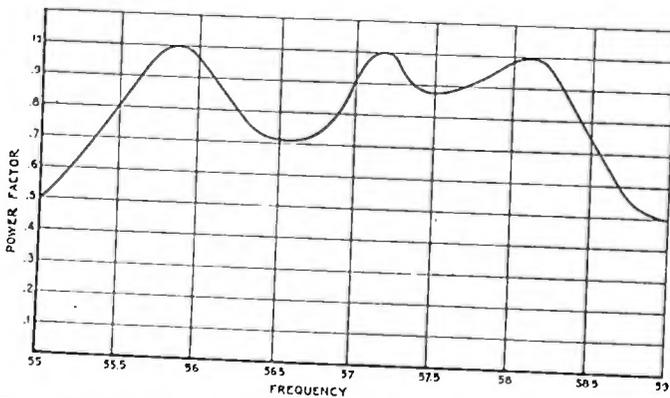
FIGURE 25—Power Factor of the Output Circuit. The middle maximum corresponds to the tuning frequency, the other two to points B and C of Figure 24
