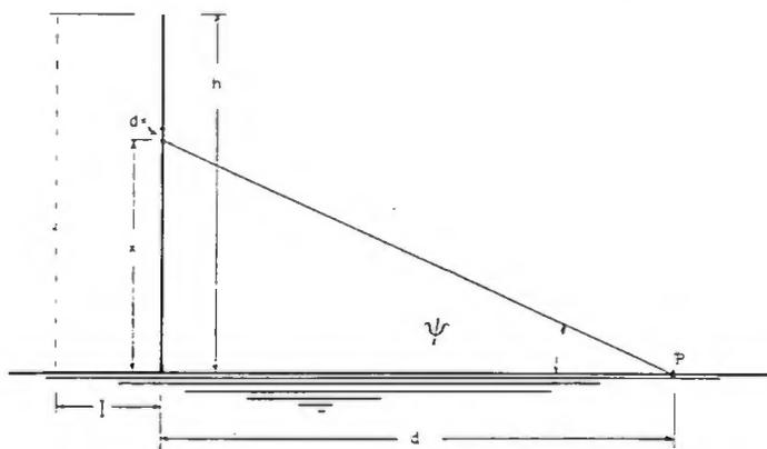
FIGURE 1—Vertical Antenna—Uniform Current Distribution
