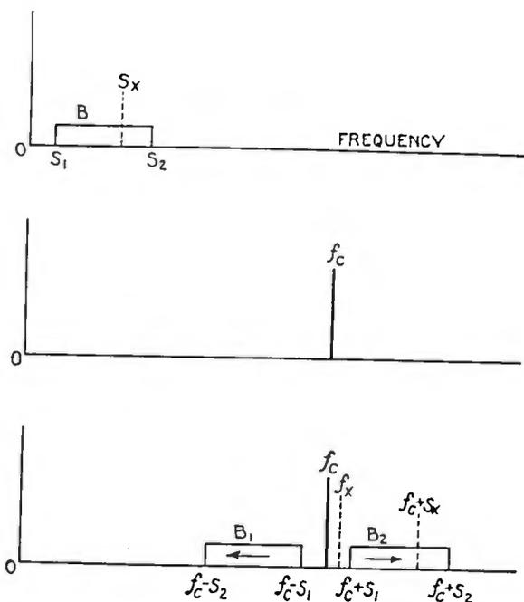
FIGURE 1—Frequency Spectra in Radio Telephone Modulation
