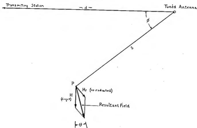
FIGURE 4—Field Distortion Due to Re-radiation
