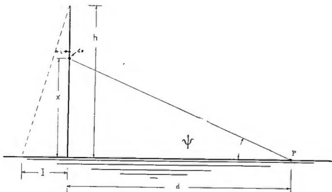
FIGURE 2—Vertical Antenna—Linear Current Distribution
