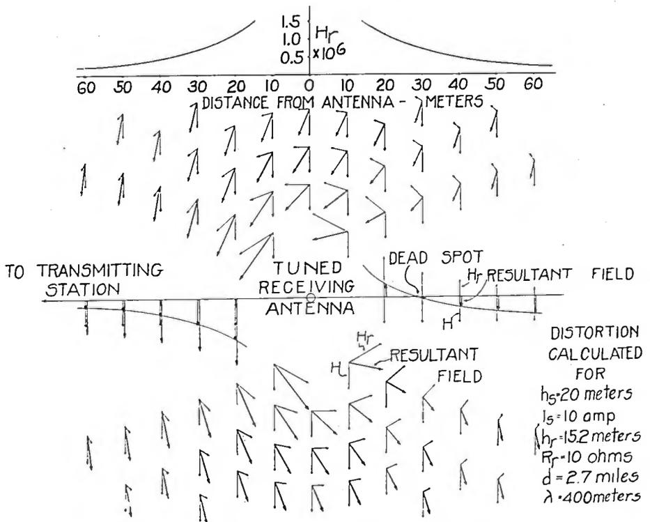
FIGURE 5—Calculated Field Distortion Near a Tuned Receiving Antenna
