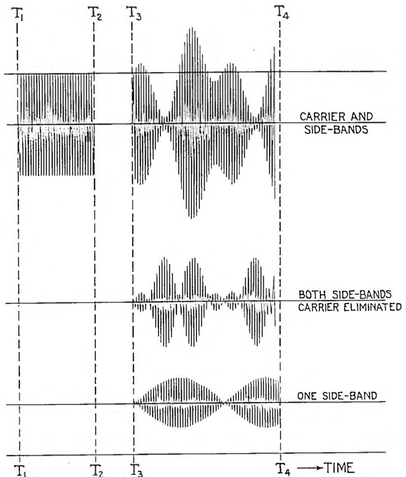
FIGURE 2—Wave Radiated in Three Systems of Transmission. In interval  $T_1$ — $T_2$  there is no modulation. In  $T_3$ — $T_4$  there is modulation by two audio frequencies, a fundamental and its second harmonic
