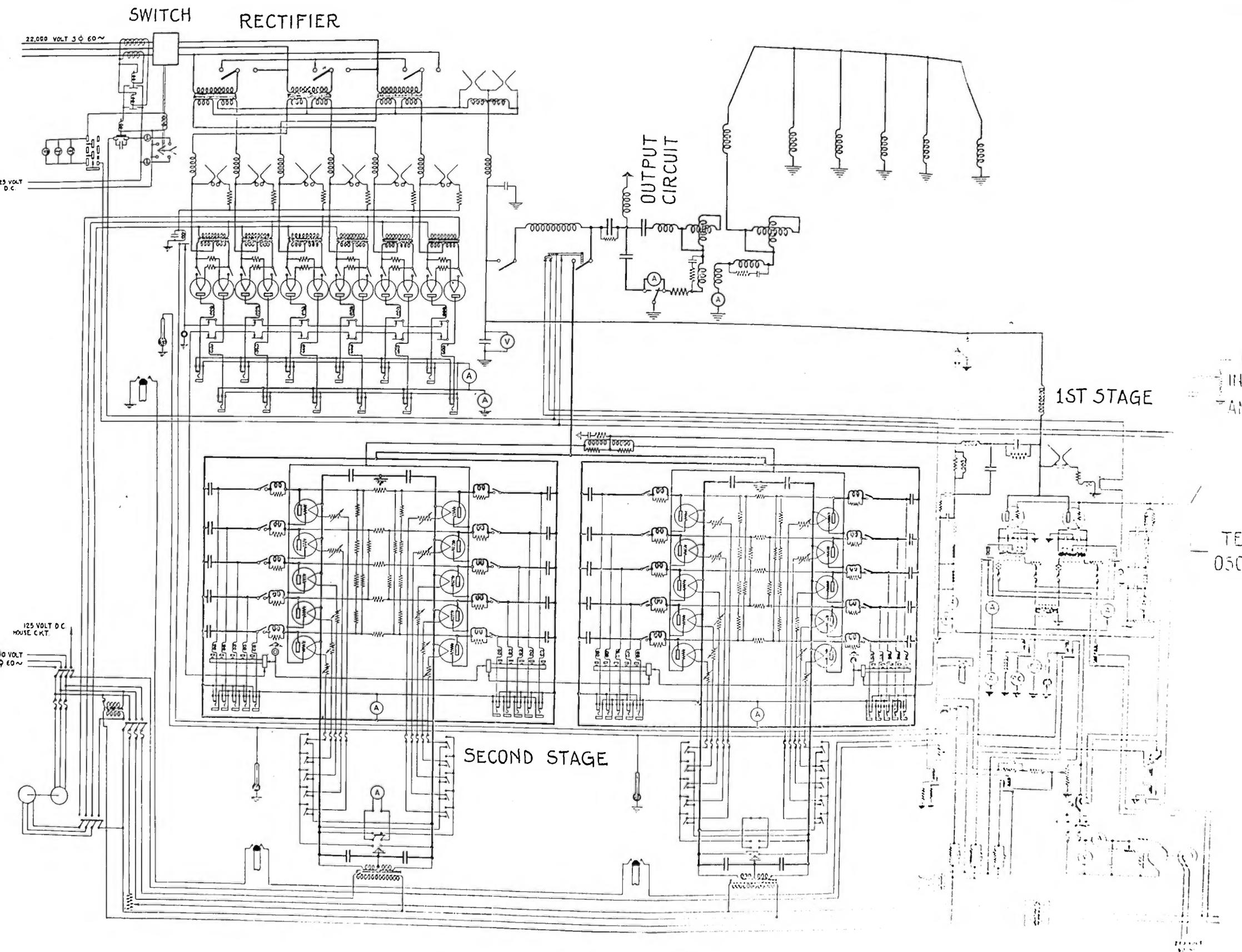
FIGURE 35—Schematic of Complete Rectifier and Power Amplifier System
