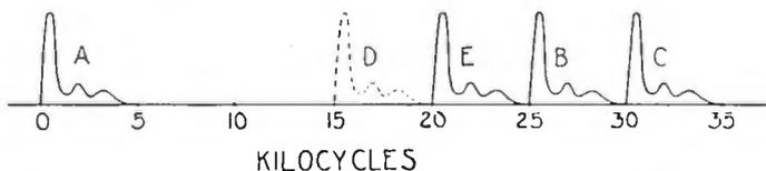
FIGURE 1—Shifted Speech Frequency Bands for Multiplex Communication
