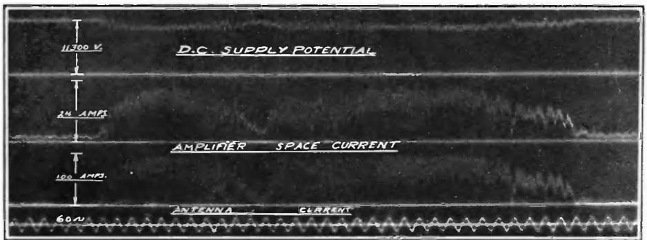
FIGURE 6—Oscillogram Taken During Transmission of the Word "Bordeaux." Note particularly that before and after the word there is but little amplifier space current and no antenna current. This oscillogram was taken with a dummy antenna
