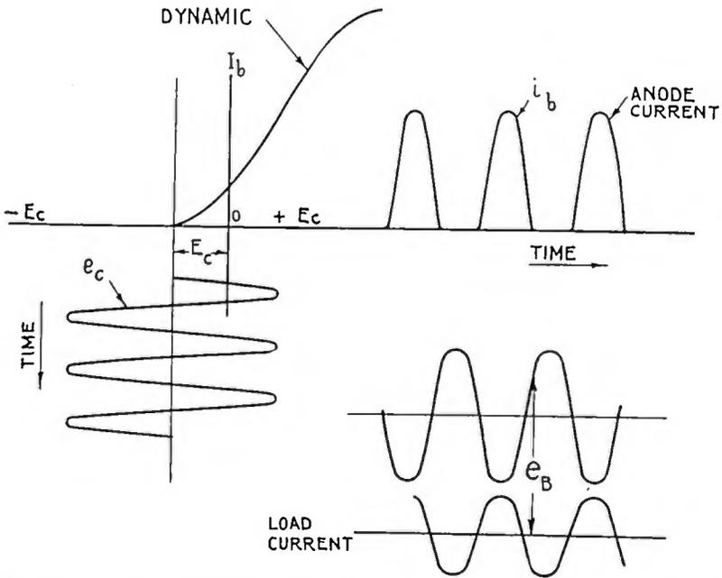
FIGURE 5—Current and Voltage Relations in Typical Amplifier of the Third Class
