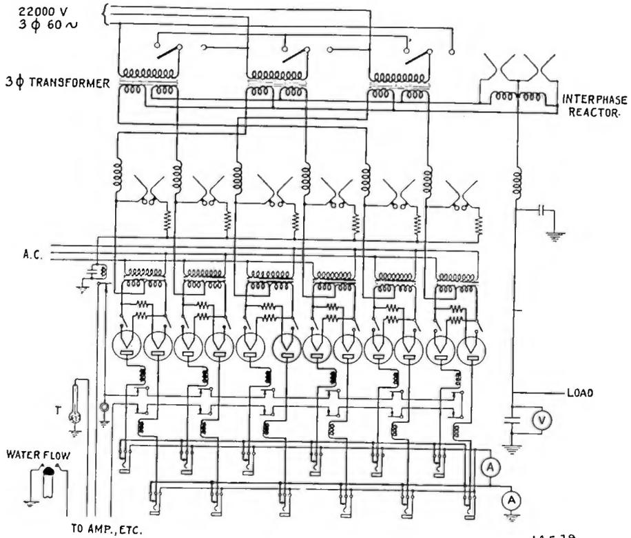
FIGURE 30—Schematic of Six-phase Rectifier Circuit
