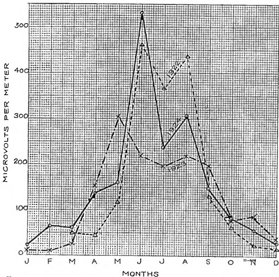
FIGURE 5—Average Atmospheric Disturbances 3 P.M. for 1922-1923-1924
