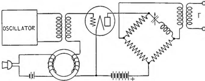
FIGURE 3—Modulator Tube with Bridge Circuit to Eliminate the Carrier
