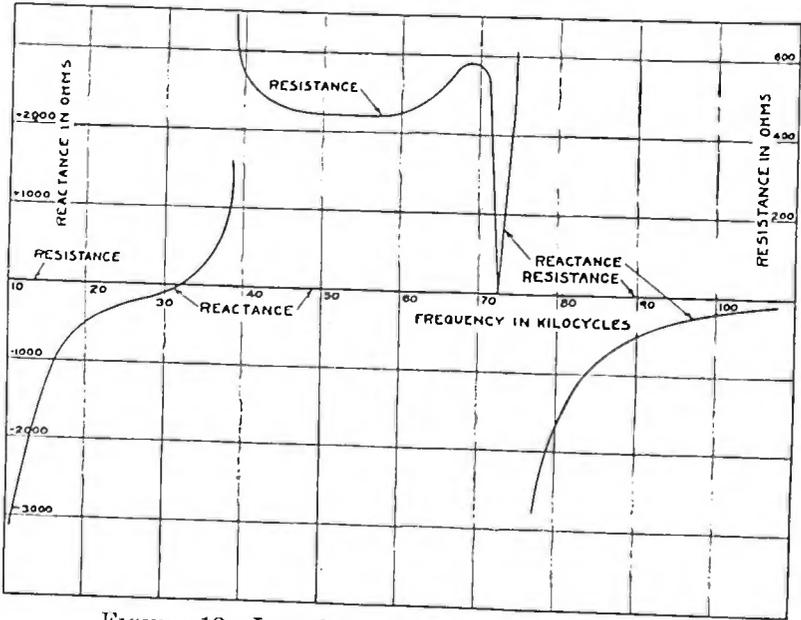
FIGURE 12—Impedance Curves of Second Filter
