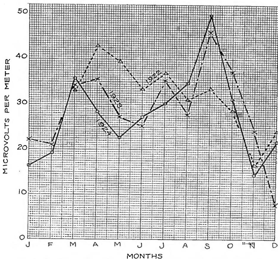
FIGURE 2—Average Signal for Nauen (POZ) 10 A.M., 1922-1923-1924
