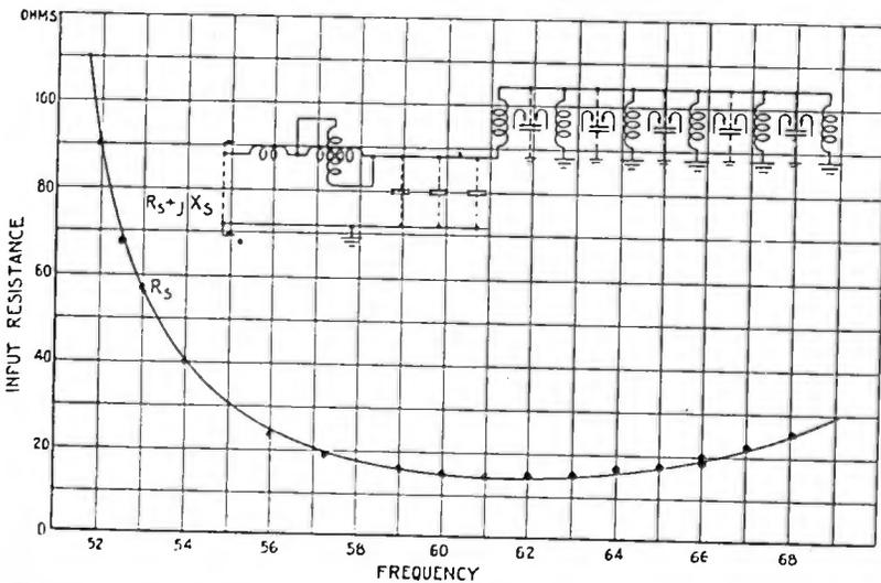
FIGURE 19—Resistance Characteristic of Multiple Tuned Antenna
