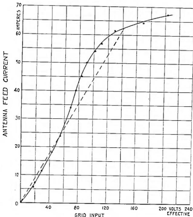
FIGURE 28—Input-response Curve at Constant Frequency
