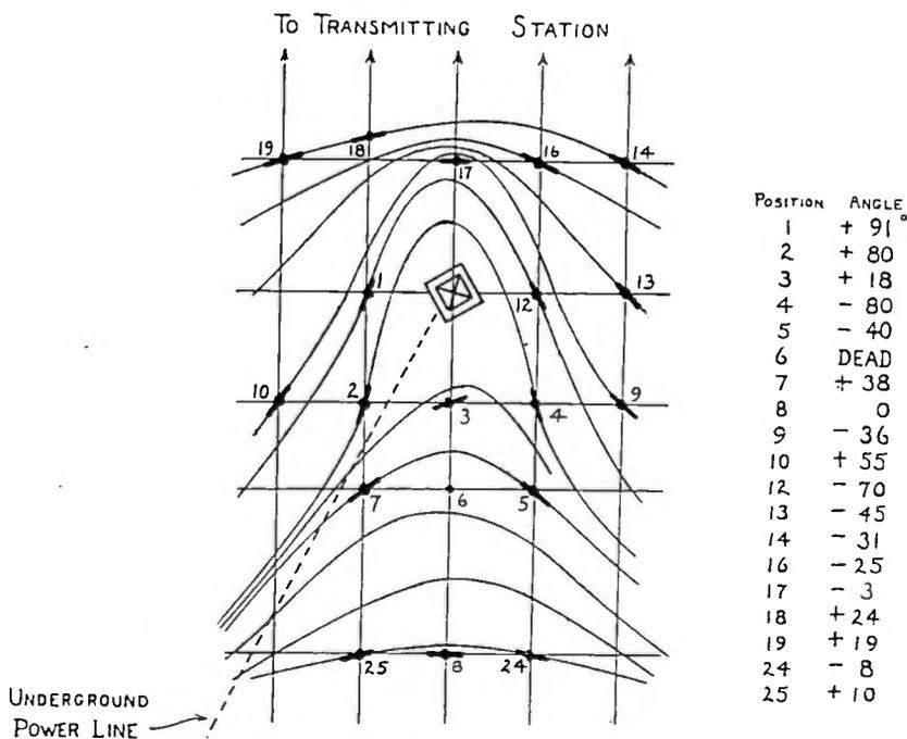
FIGURE 6—Field Distortion Caused by Washington Monument
