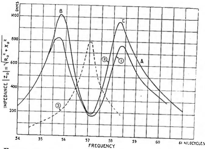
FIGURE 24—1. Impedance of the output circuit as a function of frequency, measured values. 2. The same, calculated values. 3. Resonance curve of antenna
