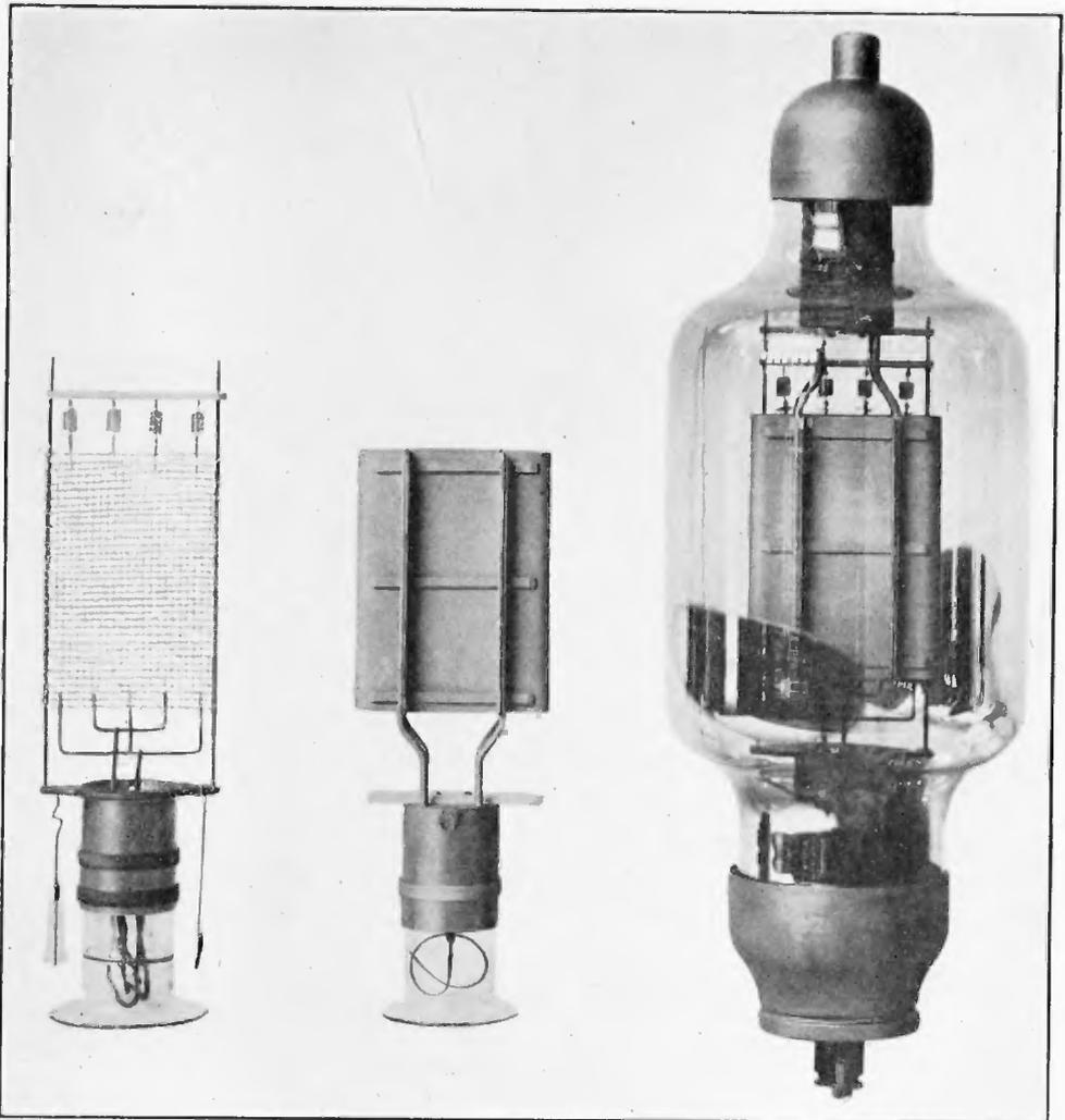
FIGURE 13—Radiotron UV-851 1 KW Output
