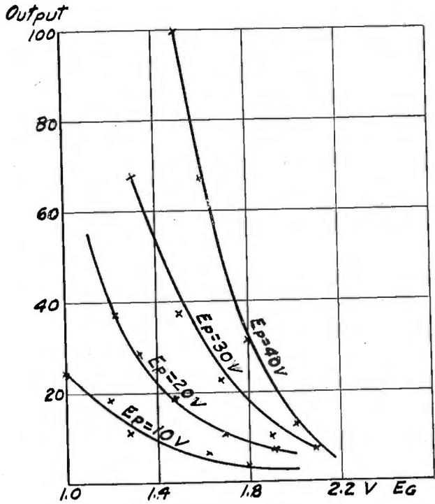
FIGURE 12—Tube DT-1, Comparison Experimental and Derived Curve. Detector Output
