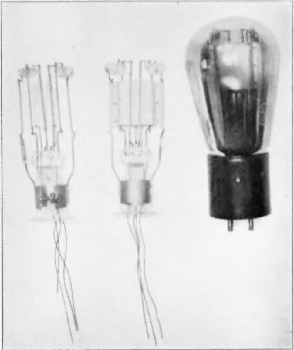
FIGURE 3—XL-7 1/2 Watt Transmitting Tube
