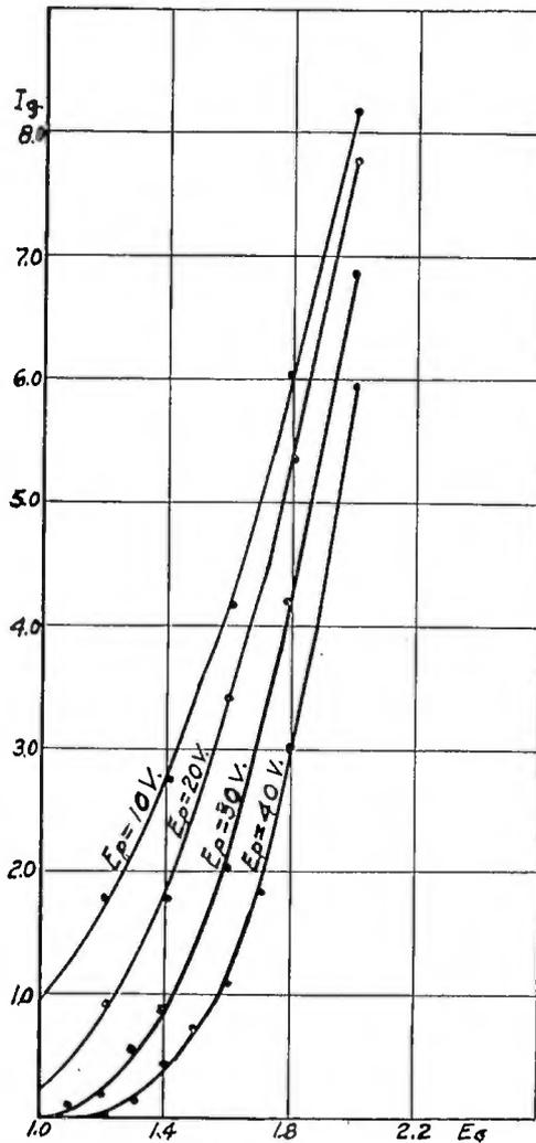
FIGURE 2—Tube DT-1, Grid Characteristics
