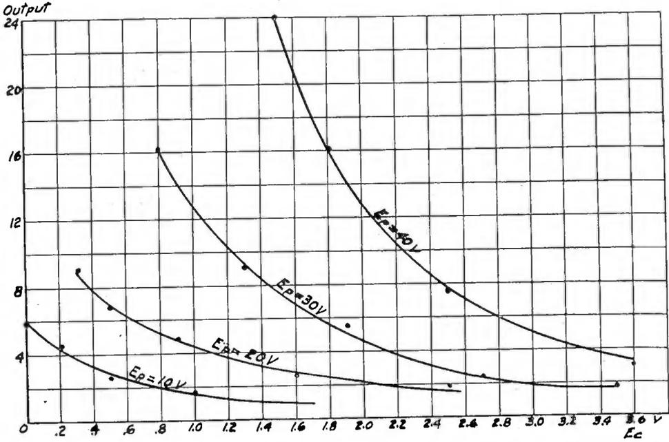
FIGURE 11—Tube DT-1, Experimental Curves, Detector Output
