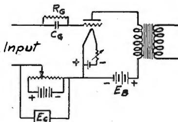
FIGURE 1—Circuit Used for Detector Test
