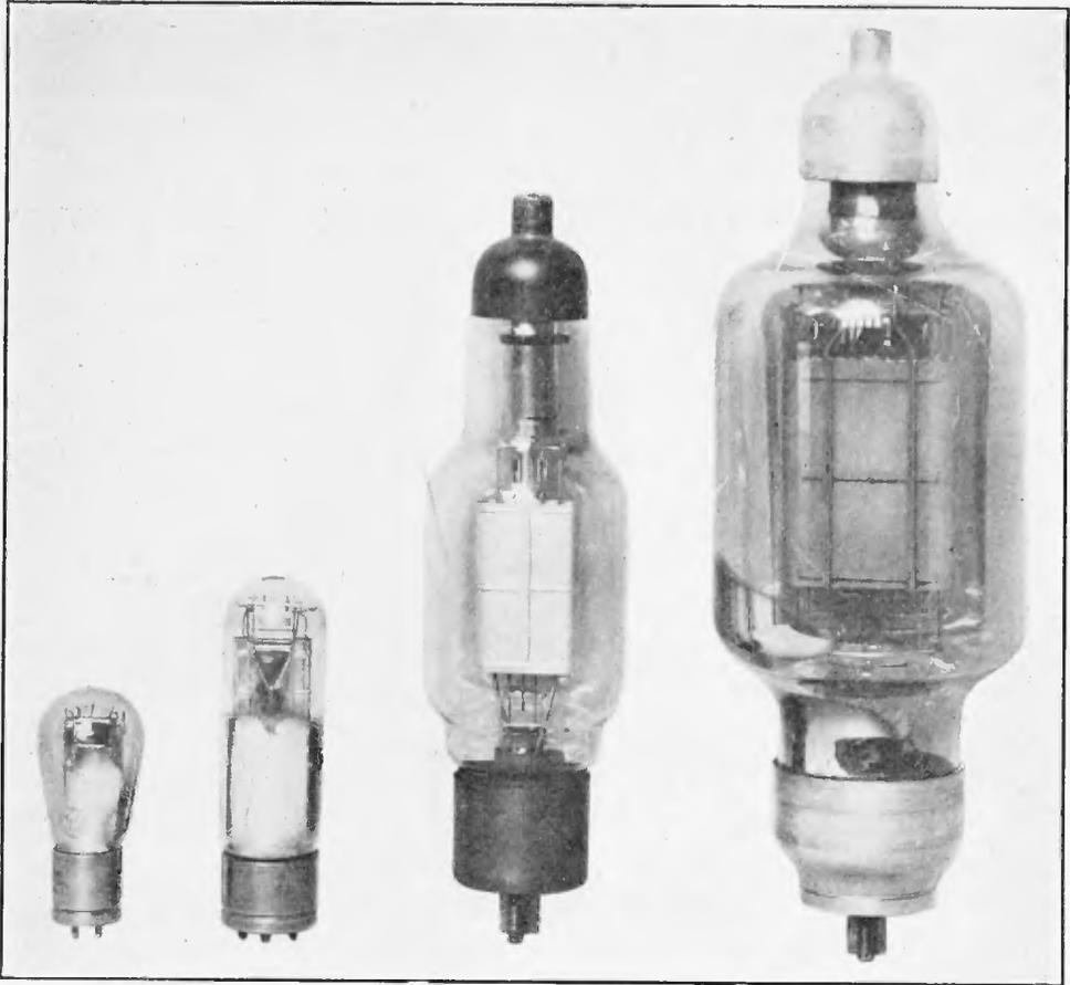
FIGURE 1—X-L Filament Transmitting Tubes
