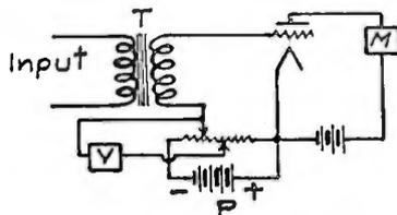
FIGURE 9—Circuit of Tube Voltmeter
