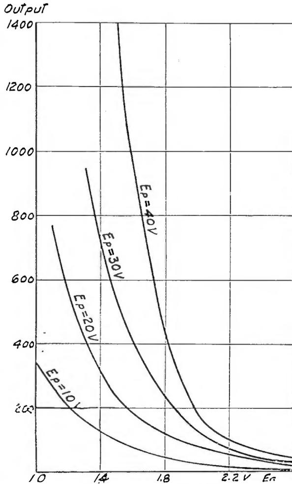
FIGURE 7—Tube DT-1, Derived Curves. Detector Output
