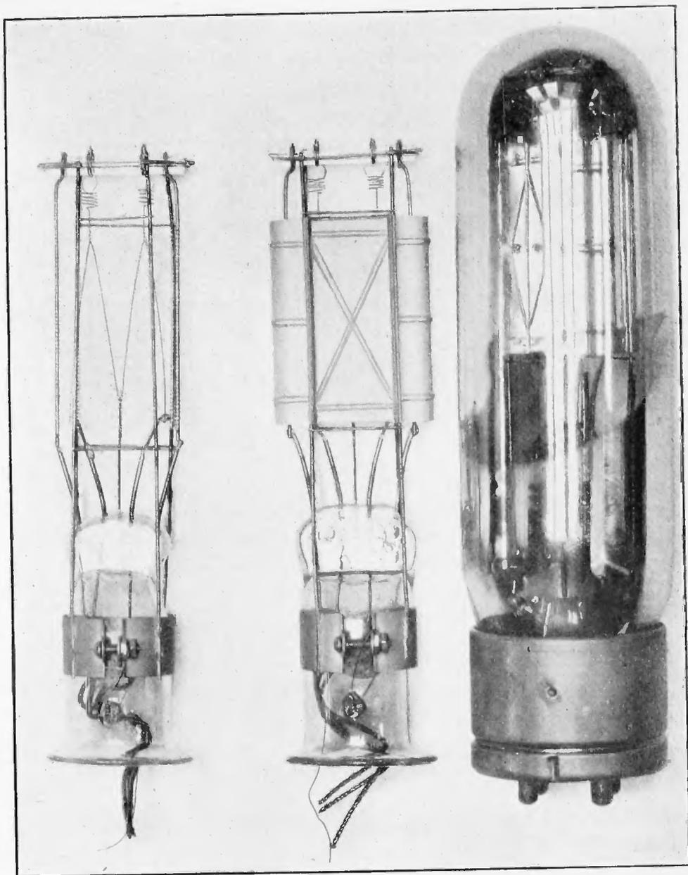
FIGURE 6—XL 50-Watt Transmitting Tube
