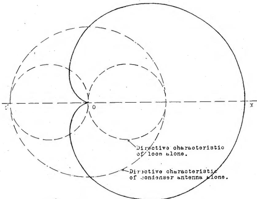
FIGURE 13—Directive Characteristic of "Condenser Antenna-Loop System"
