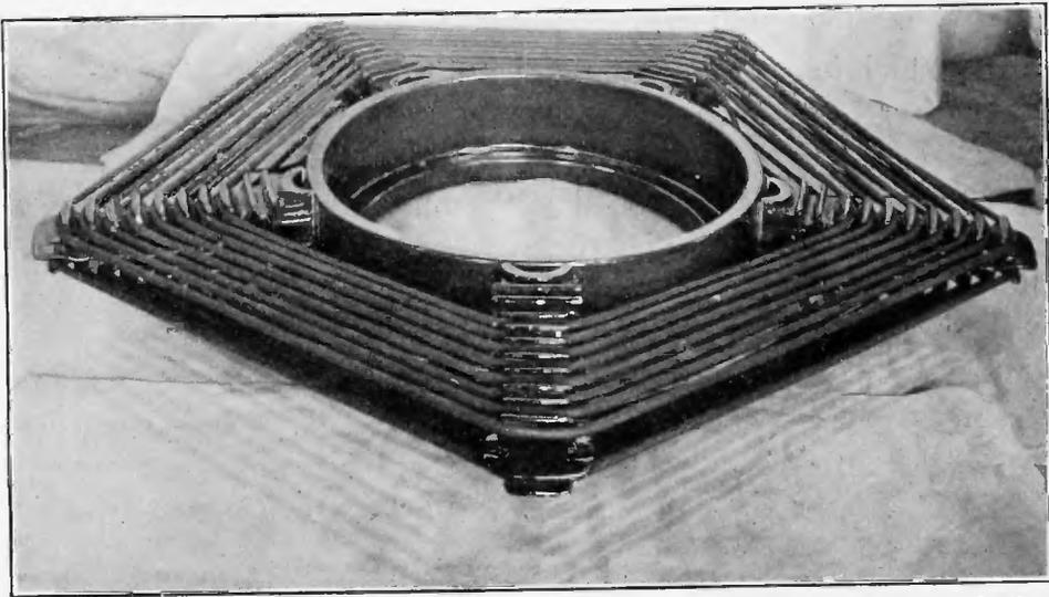
FIGURE 10—One Section of Unit Type High Power Antenna Tuning Coil
