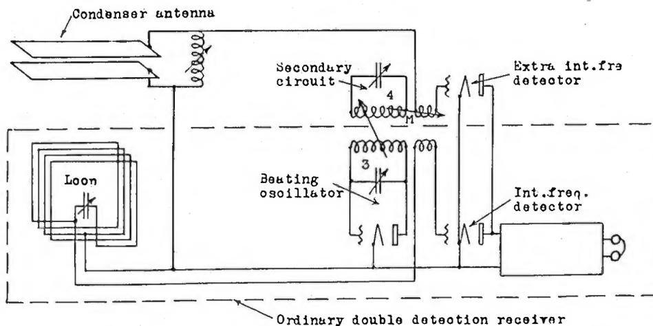
FIGURE 16—Schematic Circuit Diagram of "Condenser Antenna-Loop System"
