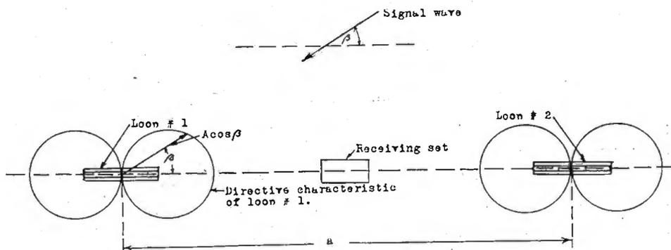
FIGURE 2—Top View of "Two-Loop System"
