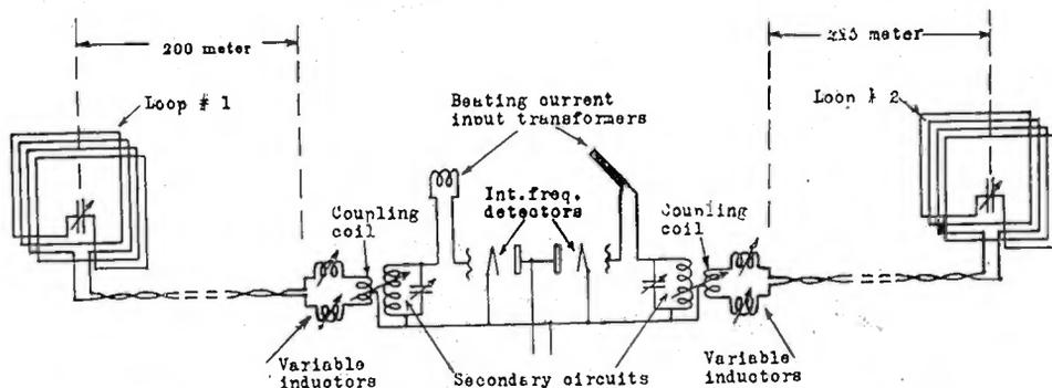
FIGURE 11—Antenna Circuits of "Long-Wave Two-Loop System"
