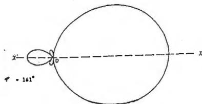
FIGURE 4—Directive Characteristics of "Two-Loop System." ( $a = 1/12$ )
