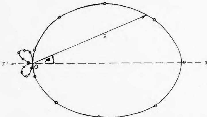
FIGURE 9—Experimental Directive Characteristic of "Two-Loop System"
