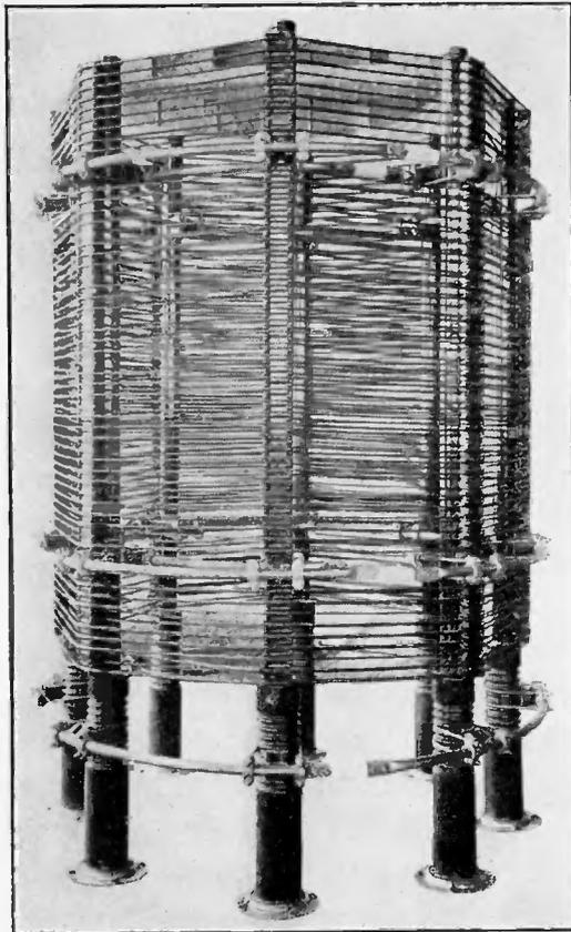
FIGURE 1—Antenna Tuning Coil
