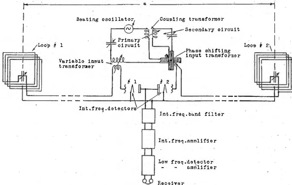
FIGURE 1—Schematic Circuit Diagram of "Two-Loop System"
