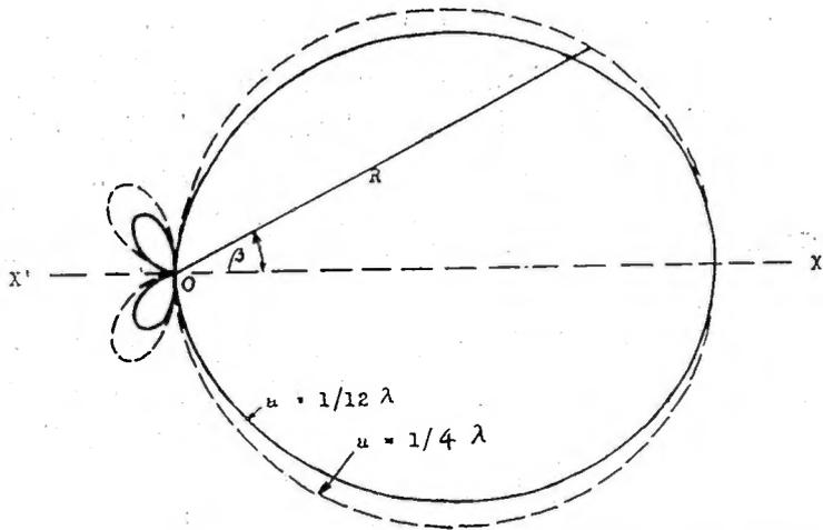
FIGURE 3—Directive Characteristic of "Two Loop System"
