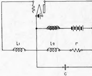
FIGURE 45—Diagram of an Oscillator Circuit
