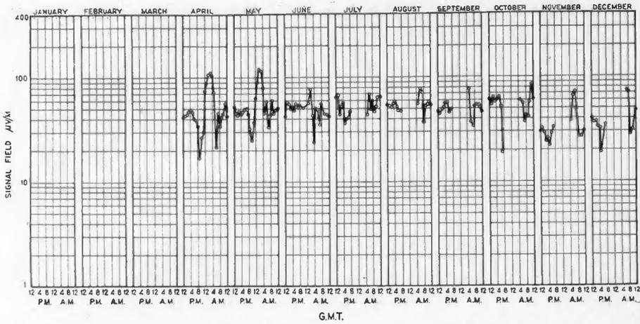
Monthly Averages of Diurnal Variation of Signal Field Strength. Leafield England. (GBL) Measured at Belfast, Maine. Corrected to 300 Amperes Antenna Current
