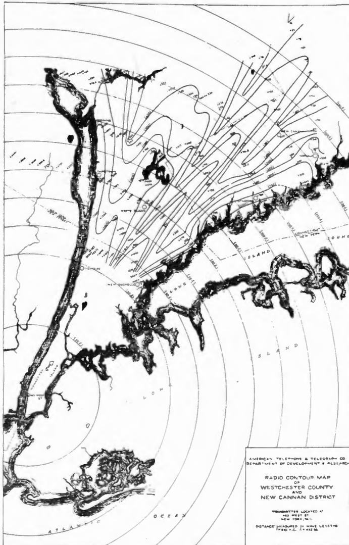
FIGURE 1—Radio Contour Map Showing Wave Interference Pattern
