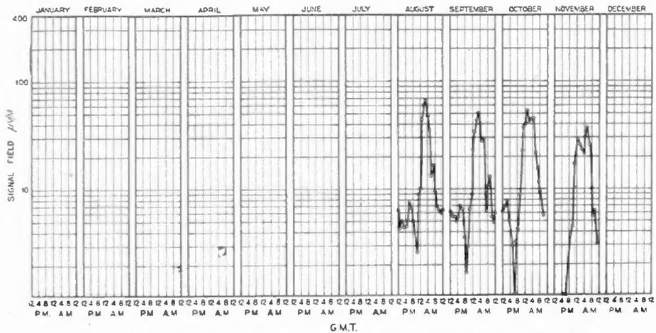
Monthly Averages of Diurnal Variation of Signal Field Strength. Northolt, England. (GKB) Measured at Riverhead, L. I., Corrected to 100 Amperes Antenna Current
