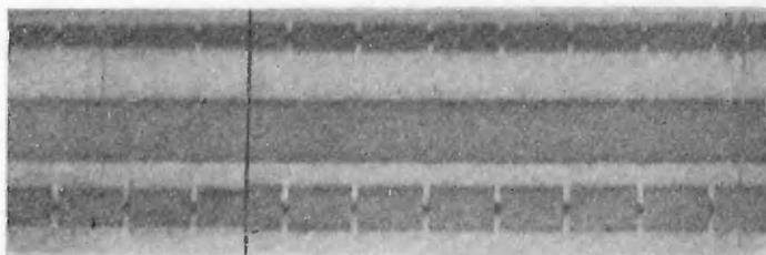
FIGURE 15—Daytime Record of Carrier and Side-Band Signals
