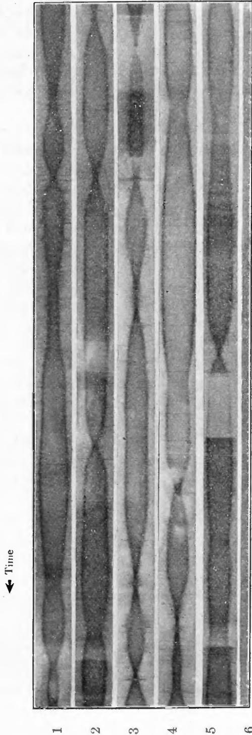
FIGURE 8—Single-Frequency Fading Record. Made at Stamford, Conn., May 16, 1924, 1.54 A. M. Timing Marks, on Strip 6, 2.5 Seconds Apart
