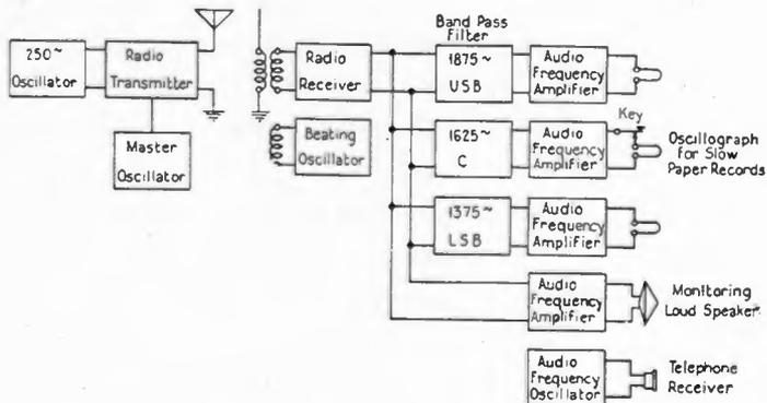
FIGURE 11—Diagram of System Used for Three-Frequency Tests
