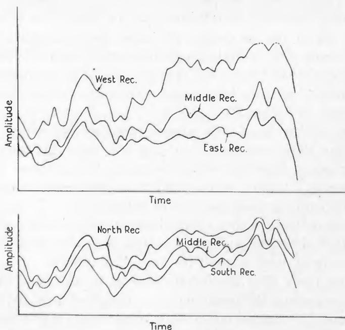
FIGURE 35—Curves Showing Single Frequency Fading on Spaced Receivers, Condensed from Long Record
