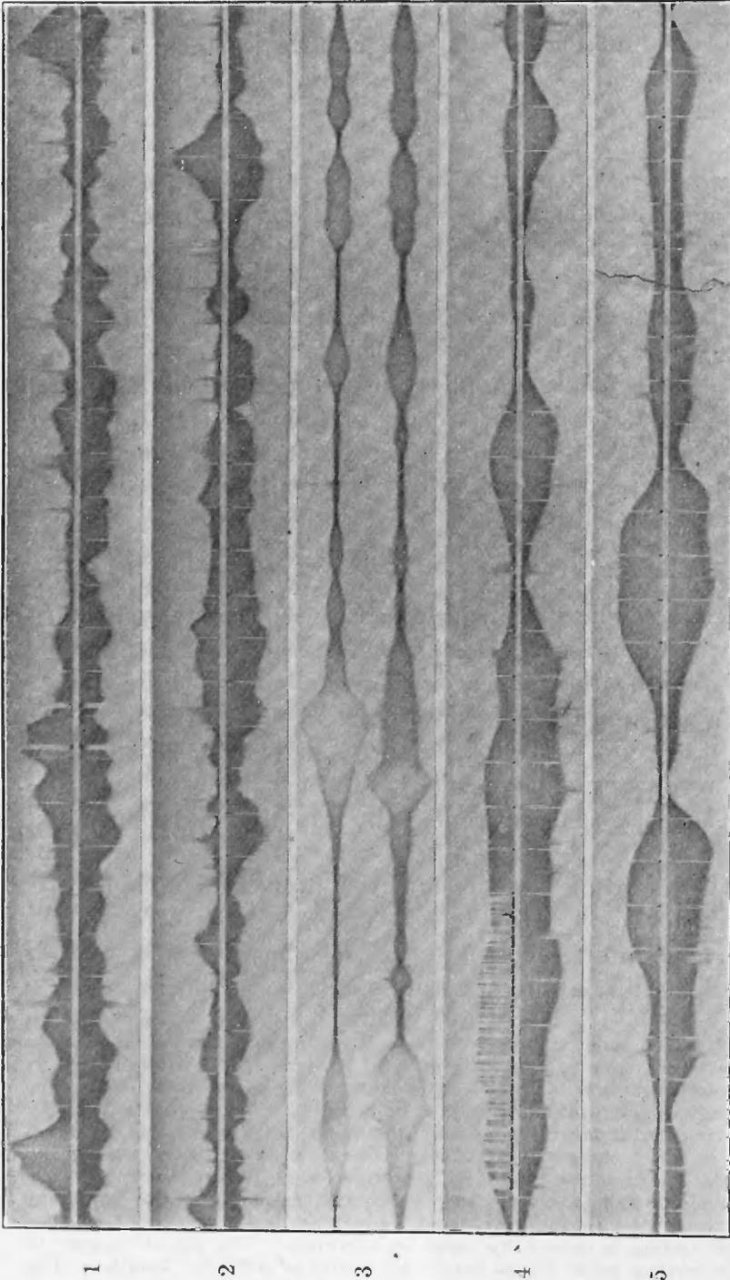
FIGURE 50—Slow Record Comparing the Signal Detected from Carrier and One Side Band with Signal Detected from Carrier and Both Side Bands. Made at Riverhead, L. I. Upper trace carrier+both side bands, lower trace carrier+one side band. Strips 1 and 2, July 22, 1925, 1.46 A. M. 250-cycle modulating tone. Strip 3, July 21, 1925, 3.10 A. M. 250-cycle modulating tone. Strips 4 and 5, July 23, 1925, 2.47 A. M., 500-cycle modulating tone
