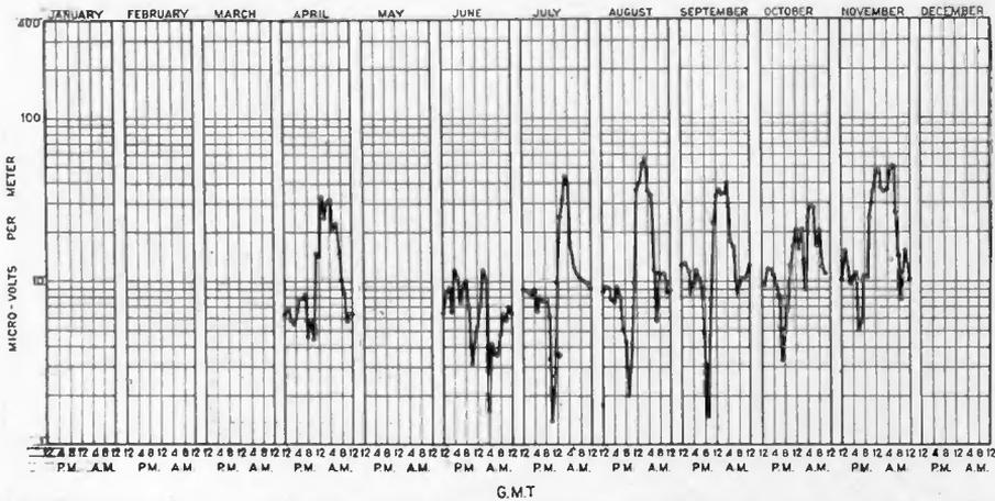
Monthly Averages of Diurnal Variations of Signal Field Strength. Northolt, England. (GKB) Measured at Belfast, Maine. Corrected to 100 Amperes Antenna Current
