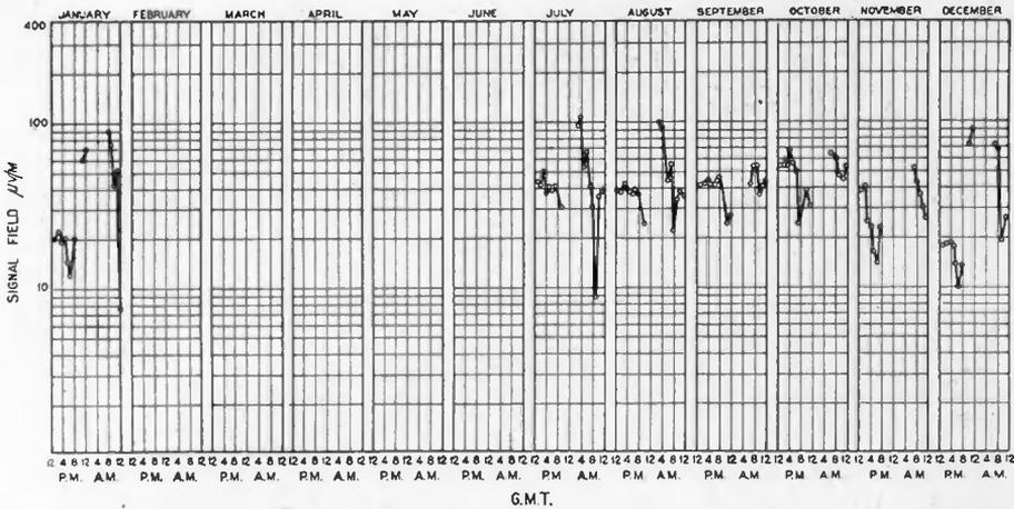
Monthly Averages of Diurnal Variation of Signal Field Strength. Leaffield, England. (GBL) Measured at Green Harbor, Mass. Corrected to 300 Amperes Antenna Current
