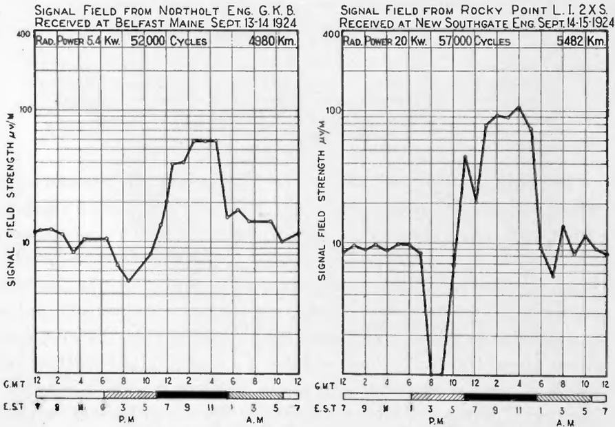
upper curves are for similar averages of measurements made on the lower frequencies. These curves show clearly that the range of the diurnal fluctuation is less for the lower frequencies. This is because of the lesser daylight absorption.
