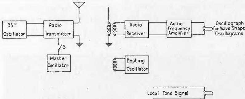
FIGURE 39—Diagram of System Used to Measure Frequency Modulation
