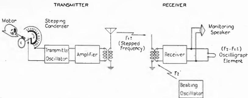
FIGURE 16—Diagram of System Used to Obtain Records of Selective Fading or "Band Fading" Records
