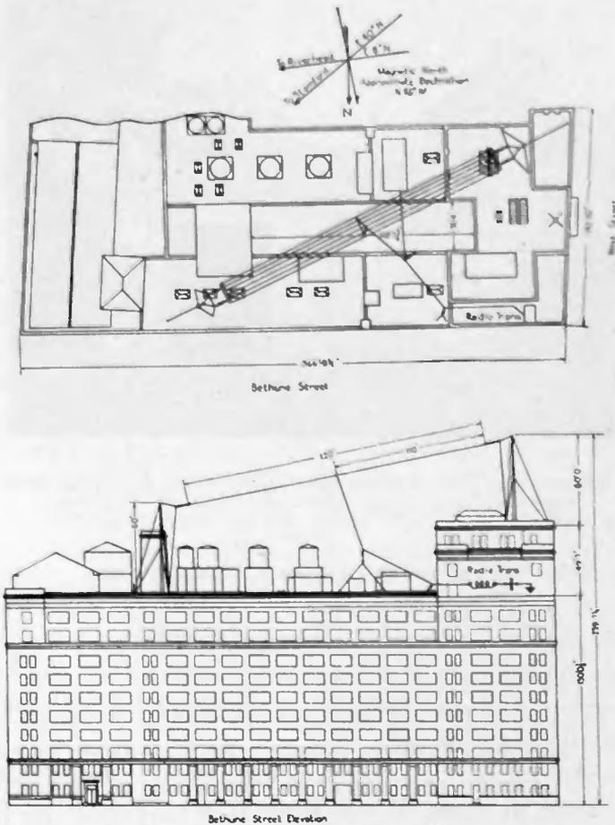
FIGURE 4—Plan—Elevation of the Transmitting Antenna
