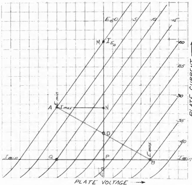
FIGURE 7--Tube Characteristics for Showing Conditions for Maximum Understorted Output
