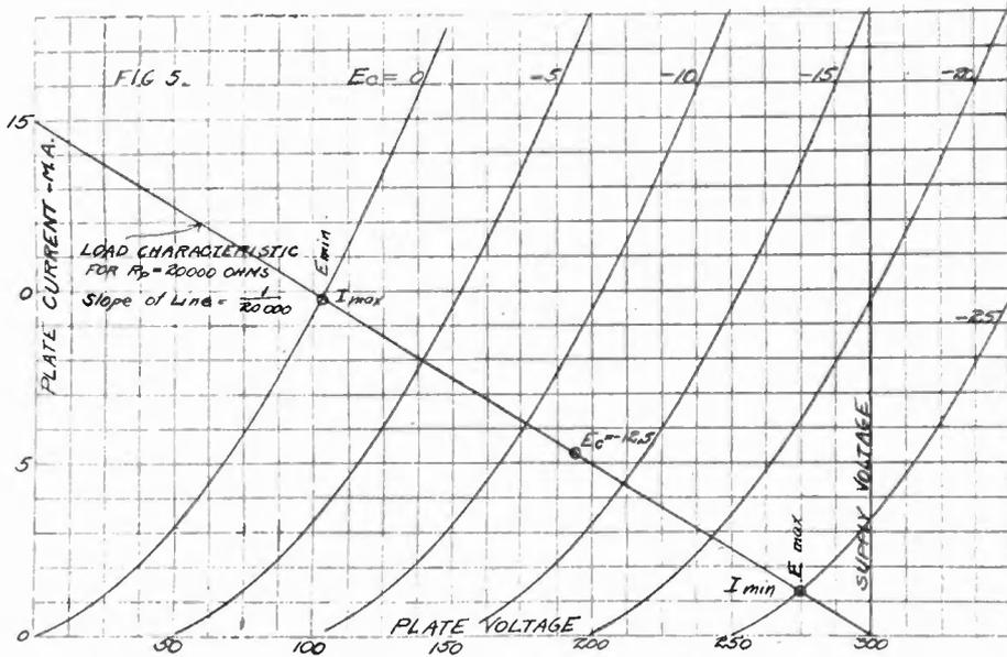
FIGURE 5—Tube and Load Characteristics
