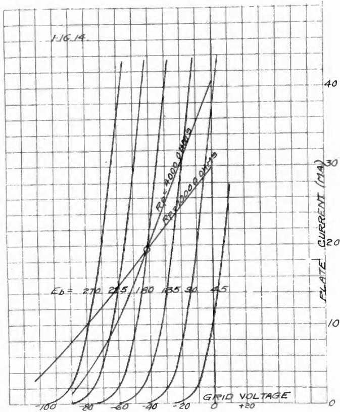
FIGURE 14—Static and Dynamic Characteristics—UX 171
