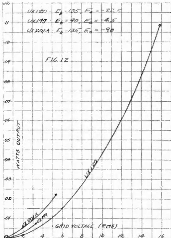
FIGURE 12—Input Voltage—Undistorted Power Output—Load Resistance 10,000 Ohms
