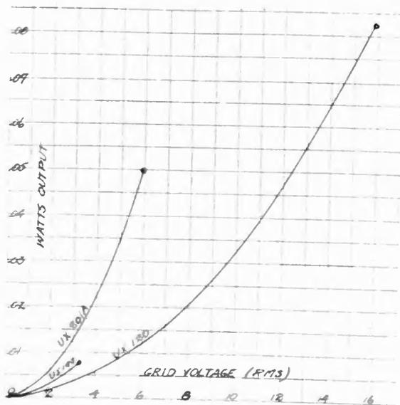
FIGURE 13—Input Voltage—Undistorted Power
