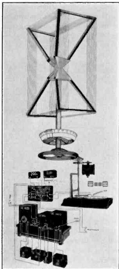
Fig. 8—Kincaid Static Recorder
