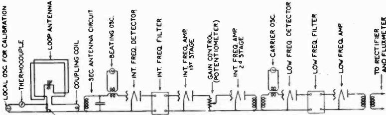
Fig. 10—Schematic Circuit Diagram of Receiving Set.
