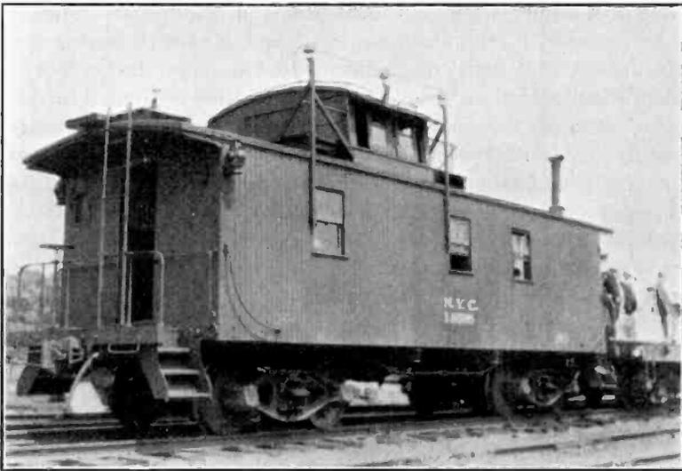
Fig. 3—Antenna on Caboose.
