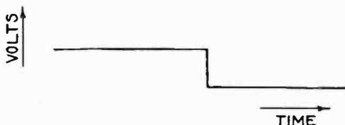
Fig. 13—Shape of Impulse Voltage.
