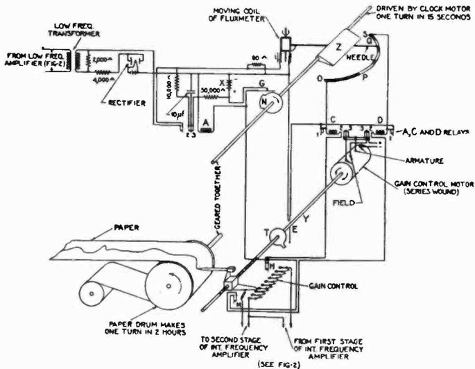
Fig. 11—Schematic Circuit of Constant-Output Control Apparatus.
