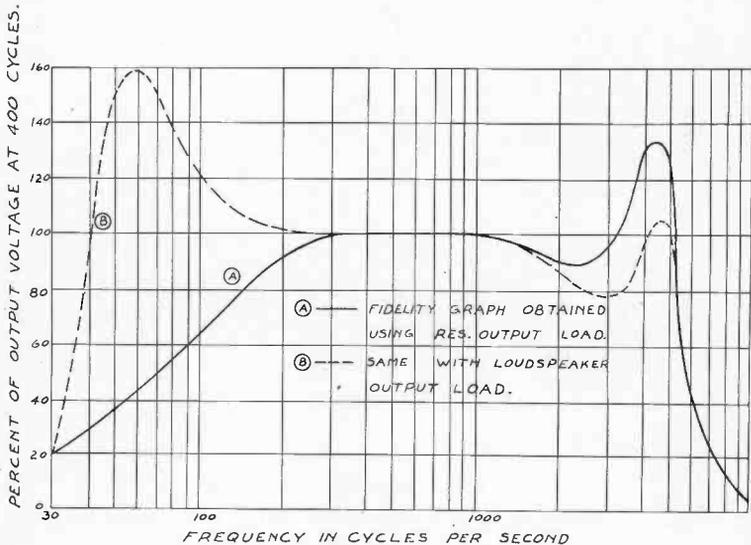
Fig. 13—Effect of Output Load on Fidelity Graph.
