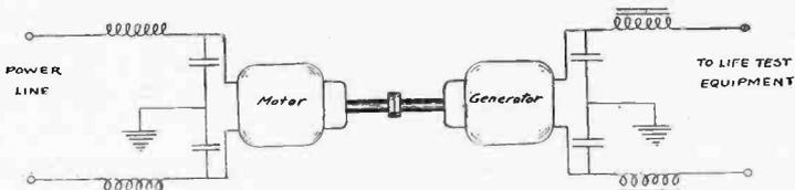
Fig. 16—Motor-Generator Filter Circuits.
