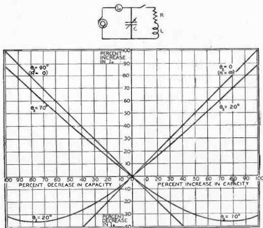
Fig. 3—Measurement of Inductance. Change in Sharpness of Tuning of Parallel Circuit Due to Change in Capacity. Impressed Frequency Critical for  $C=100$  per cent.
