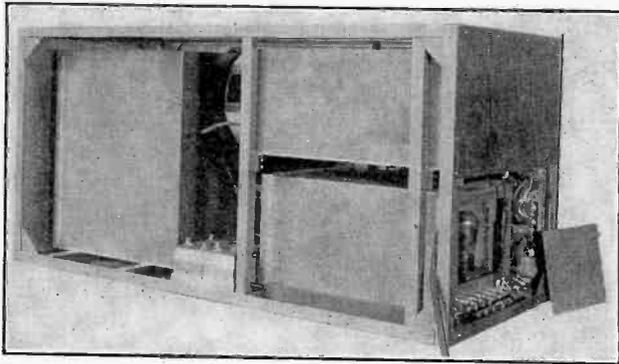
Fig. 5—Back of R. F. Oscillator Showing Separate Shielded Compartments.
