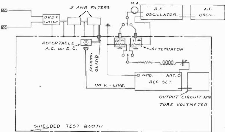
Fig. 9—Apparatus Arrangement in Test Booth.
