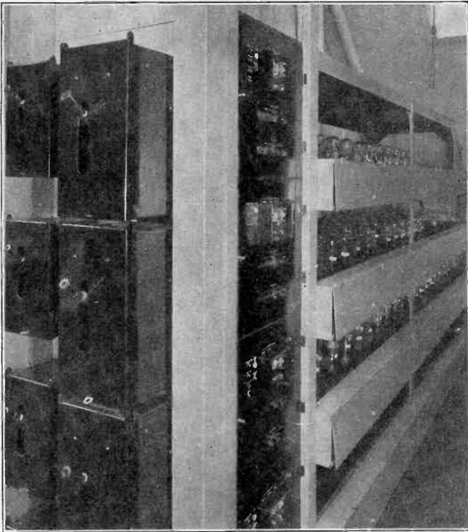
Fig. 21—View of Three-Electrode Tube Life Test Rack.
