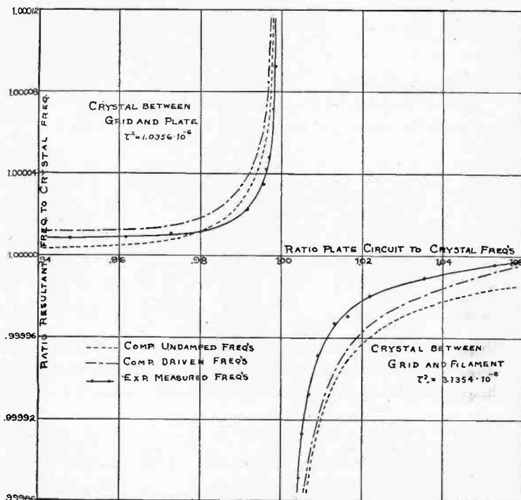
Fig. 6—Variation of Driven Frequency with Plate Circuit Frequency.
