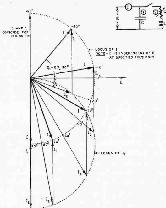
Fig. 2—Change of Phase of Line Current Due to Change in Resistance, with Critical Impressed Frequency.
