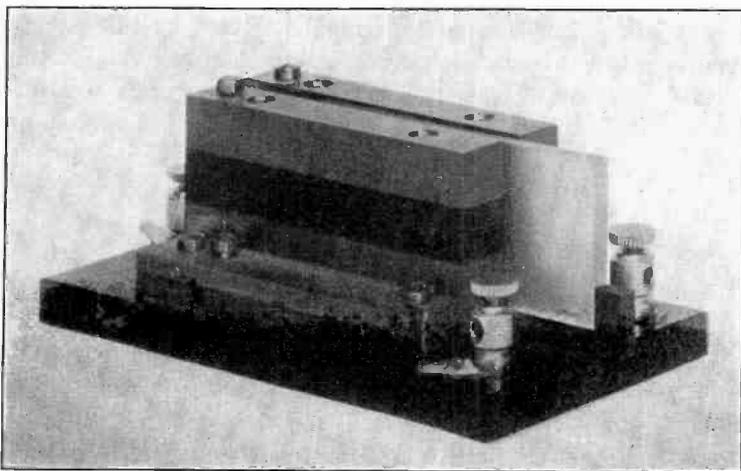
Fig. 3—Quartz Crystal in Flexural Vibration Mounting.
