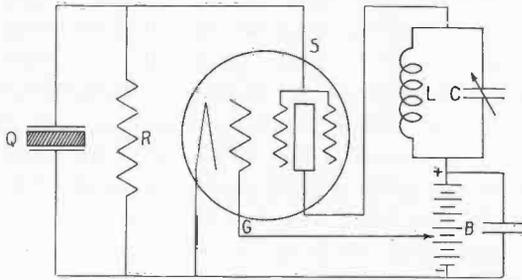
Fig. 7—Hull's Piezo-Oscillator Circuit Using the Four-Electrode Tube As A Space-Charge-Grid Device.
