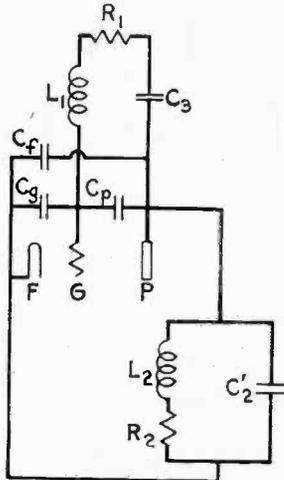
Fig. 2—Network for Crystal between Grid and Plate.
