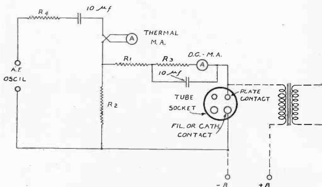
Fig. 11—Input Circuit for A. F. Amplifier Tests.
