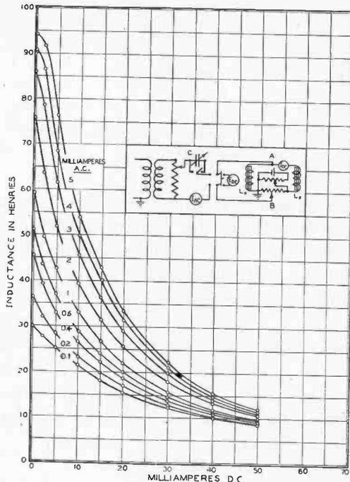
Fig. 6—Variation of Inductance with A.C. and D.C. Magnetization. 60 Cycles.
