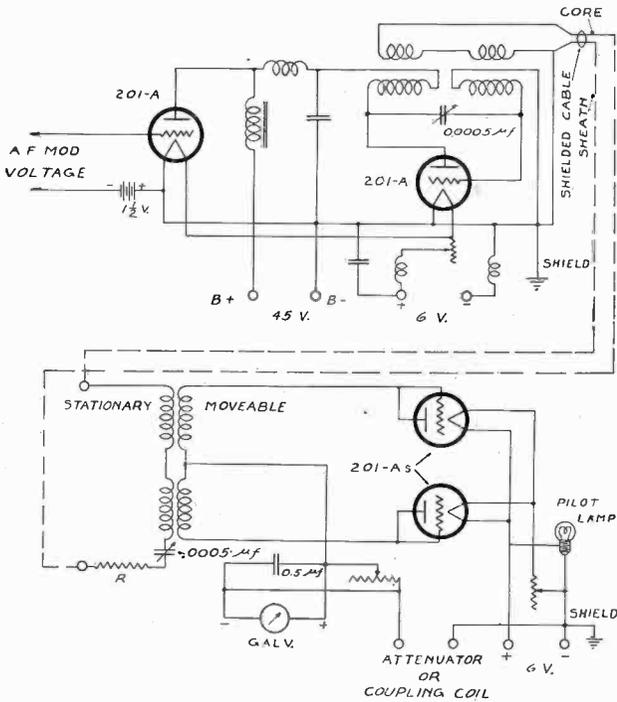
Fig. 16—Production Test R. F. Oscillator Circuit.
