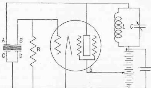
Fig. 2—Piezo-Oscillator with Screen-Grid Tube Similar in Operation to the Circuit of Fig. 1.
