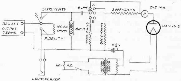
Fig. 19—Production Test Output Meter Circuit.
