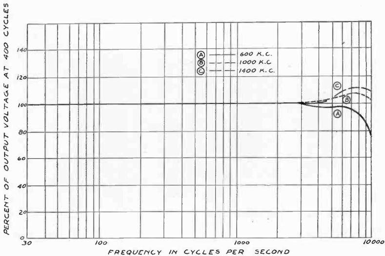
Fig. 4—Overall A. F. Characteristics of Engineering Test R. F. Oscillator.
