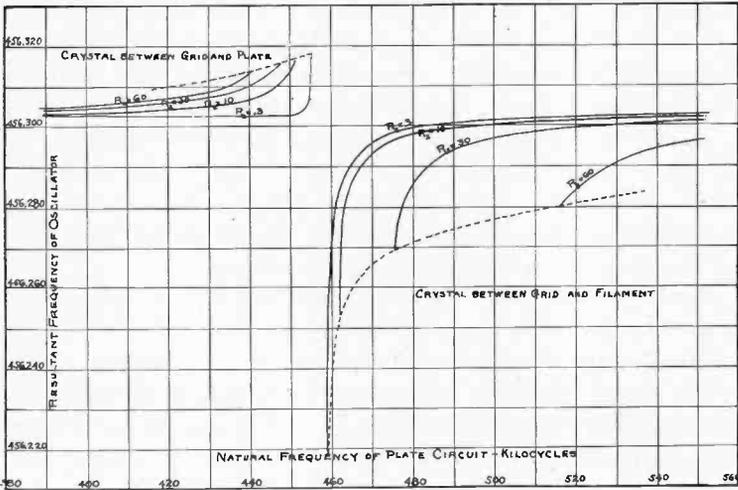
Fig. 7—Variation of Driven Frequency with Resistance of Tuned Plate Circuit.
