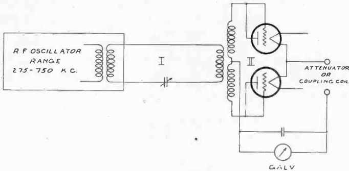
Fig. 14—Production Test R. F. Oscillator Theoretical Circuit.
