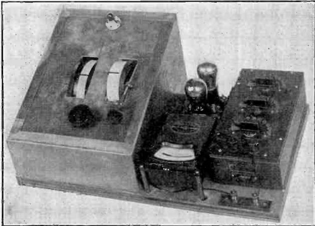
Fig. 18—Rectifier and Meter of R. F. Oscillator.
