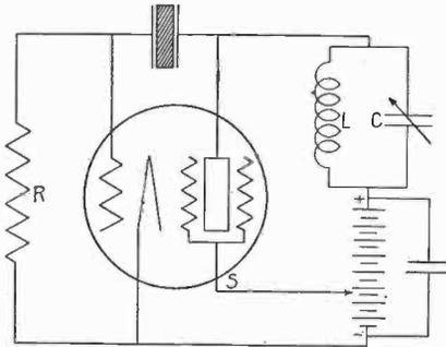
Fig. 5—Piezo-Oscillator with Screen-Grid Tube Similar in Operation to the Pierce Circuit.
