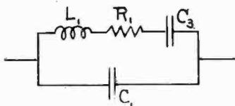
Fig. 1—Equivalent Network.
