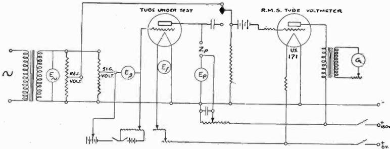
Fig. 9—Universal Test Set. Schematic Diagram.
