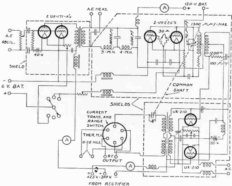
Fig. 3—Circuit of Engineering Test R. F. Oscillator.
