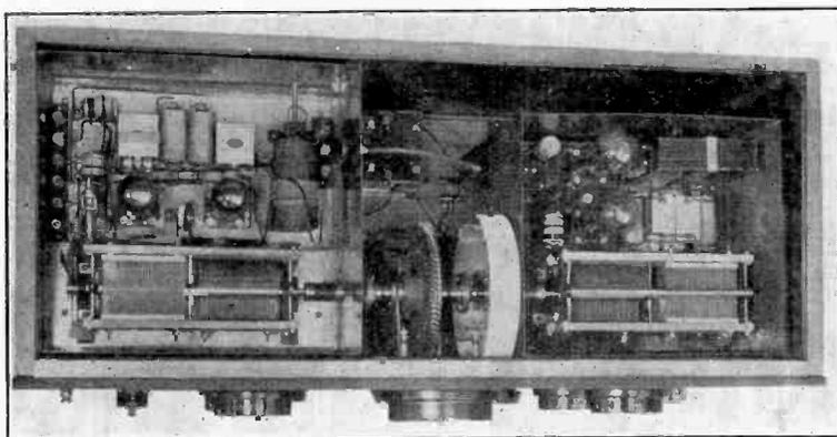
Fig. 6—Top of R. F. Oscillator Showing Oscillator and Amplifier Compartments with Shield Covers Removed.
