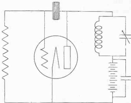
Fig. 6—Pierce Type of Piezo-Oscillator with Crystal Connected between Grid and Anode.
