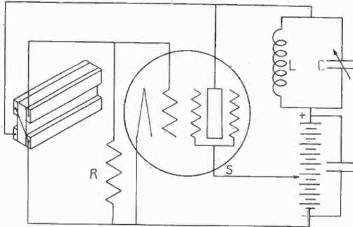
Fig. 8—Connections to the Flexural Vibration Mounting When Using the Screen-Grid Tube with Feedback through the Crystal.
