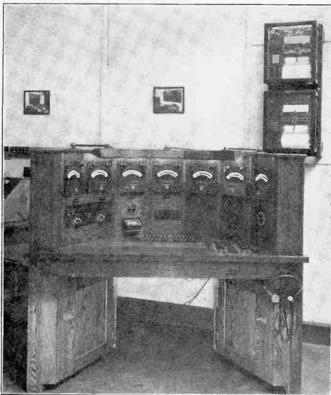
Fig. 5—Universal Test Bridge
