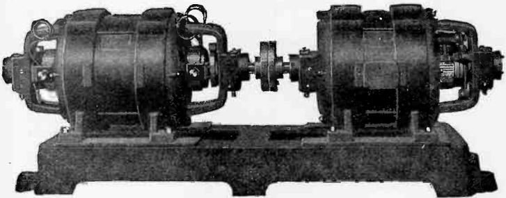
*Type P Three Unit Motor Generator*
