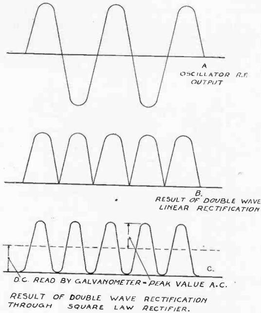
Fig. 15—Production Test R. F. Oscillator Frequency Doubling Action.
