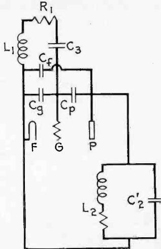
Fig. 4—Network for Crystal between Grid and Filament.
