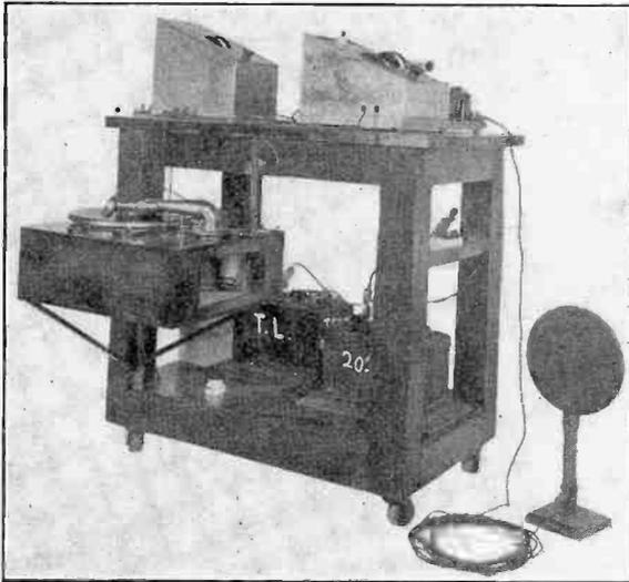
Fig. 17—Production Test R. F. Oscillator.
