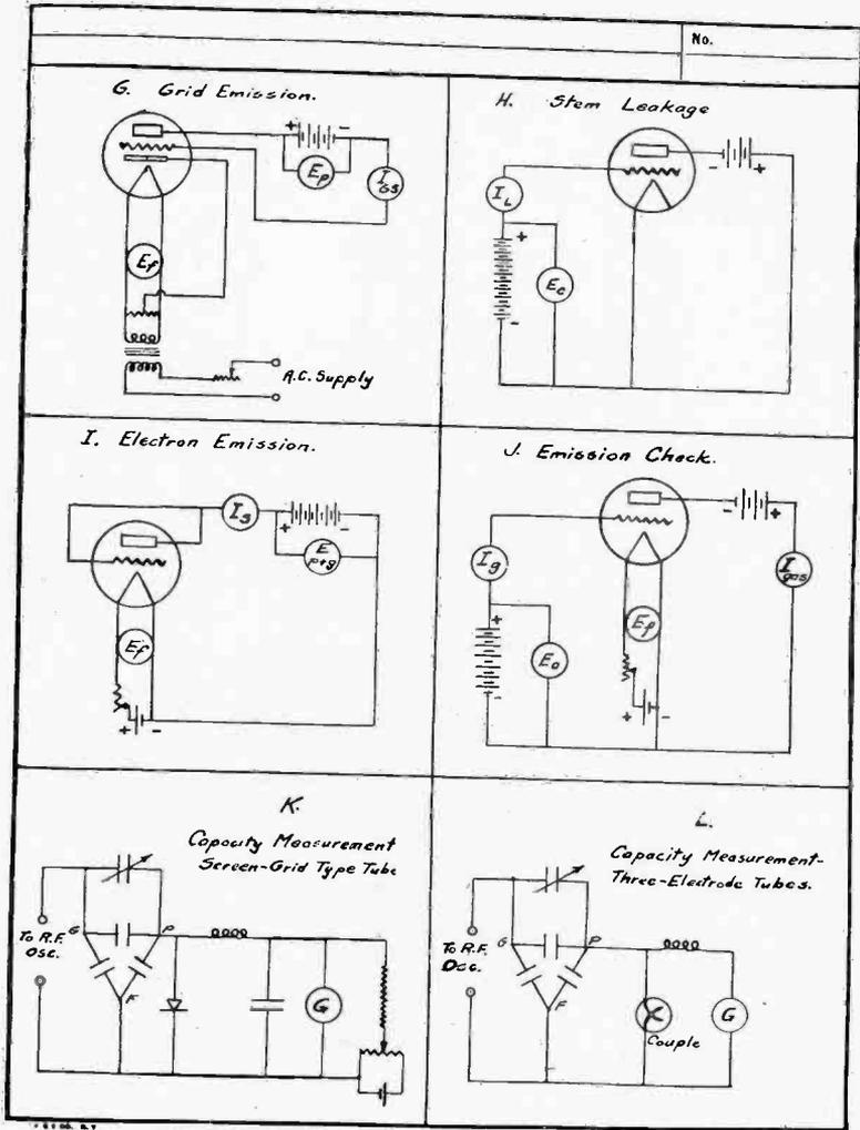
Fig. 8—Typical Test Positions.
