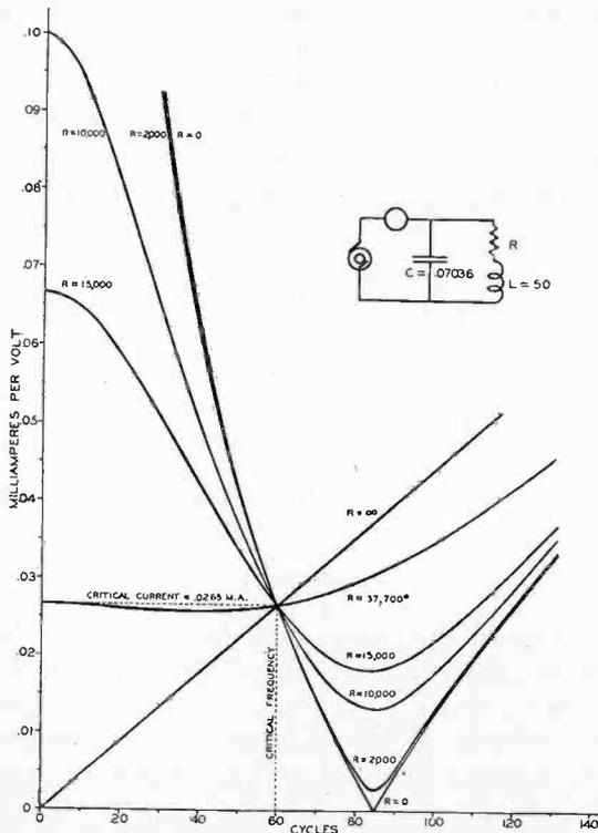
Fig. 1—Line Current Variation in Parallel Circuit Due to Frequency Variation.
