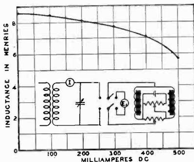
Fig. 5—Variation of Inductance with D.C. Magnetization. Filter Reactor Model UP-1627. 60 Cycles E.A.C. = 110.
