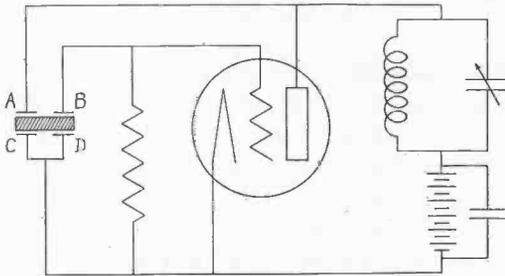
Fig. 1—Well-Known Type of Piezo-Oscillator Circuit Using Feedback through the Crystal.
