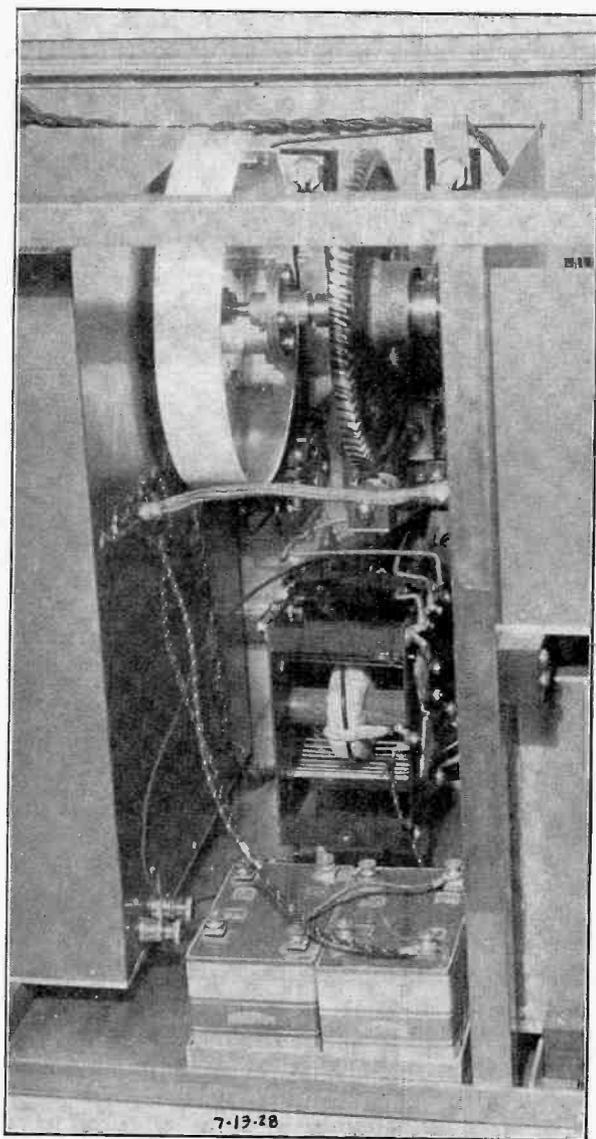
Fig. 7—View of Condenser Worm Drive and Current Transformer.
