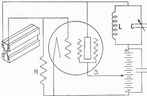
Fig. 9—Connections to Flexural Vibration Mounting When Using Screen-Grid Tube with Feedback through the Tube.
