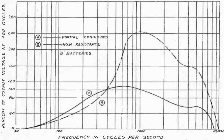
Fig. 12—Effect of High Resistance B Batteries on Fidelity of A. F. System.
