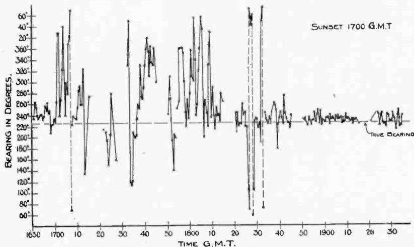
Fig. 8—Graphs of Observed Bearings of Bournemouth (undamped waves,  $\lambda = 386$  m) taken at Ditton Park, Slough. October 20, 1926.
