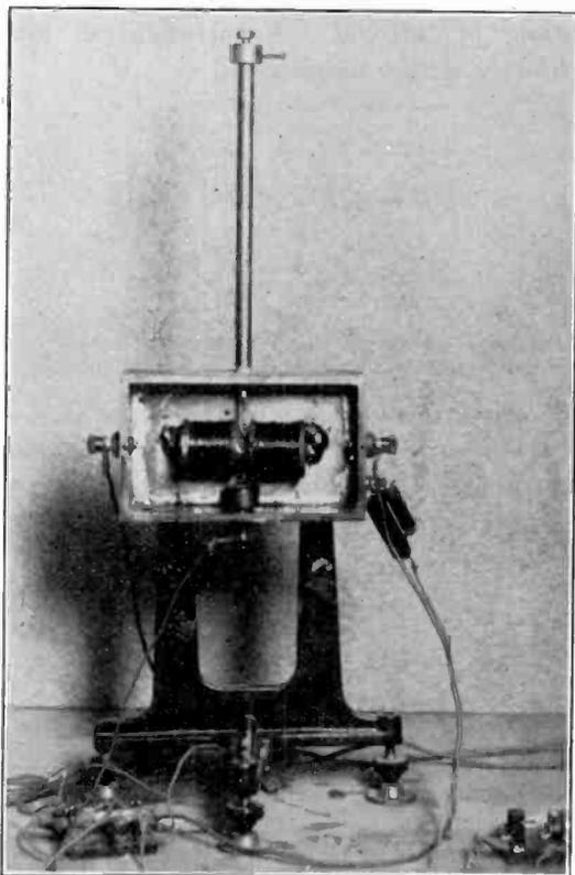
Fig. 8—The Electro-Dynamometer with the Front of the Brass Case Removed.
