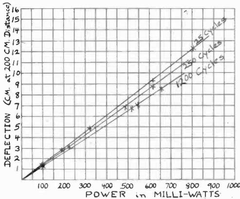
Fig. 11—Calibration Curves for the Wattmeter at Various Frequencies.
