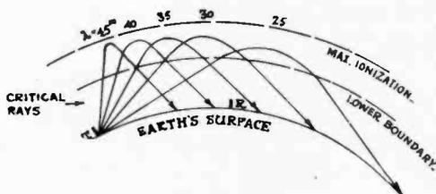
Fig. 2—Paths of the Critical Rays (*TG* of Fig. 1) for Various Wavelengths, Based on the Work of Baker and Rice.
