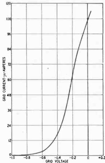
Fig. 1—Grid-Current Grid-Voltage Characteristics; Typical C-327 Tube.
