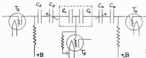
Fig. 1—The Variable Reactance Alternator with Associated Apparatus.
