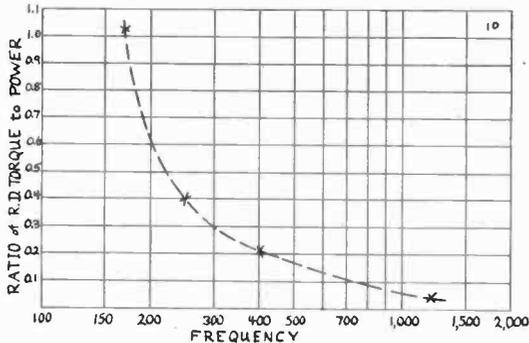
Fig. 14—Apparent Relative Efficiency of Loudspeaker.
