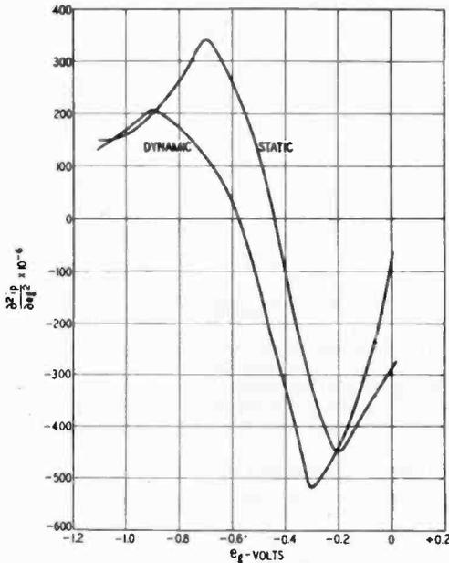
Fig. 7—Variation of Mutual Conductance,  $\partial g_m / \partial e_g$ , of Typical C-327 Tube.
