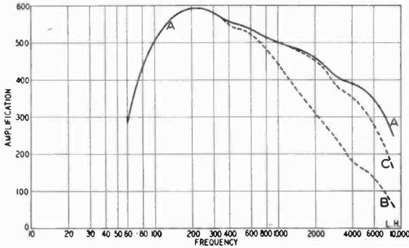
Fig. 8—Audio Amplification and Detector Frequency Distortion of a Commercial Set.
