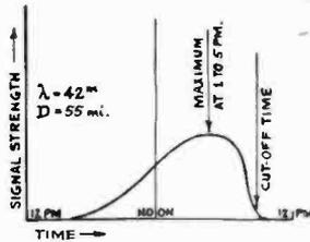
Fig. 4—Illustrating Average Variation in Received Signal Strength, for Short Distance Communication, as a Function of the Time of Day.
