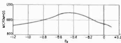
Fig. 6—Mutual Conductance,  $g_m$ , of Typical C-327 Tube.
