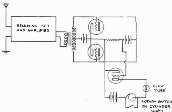
Fig. 9—Glow Tube Control Circuit.
