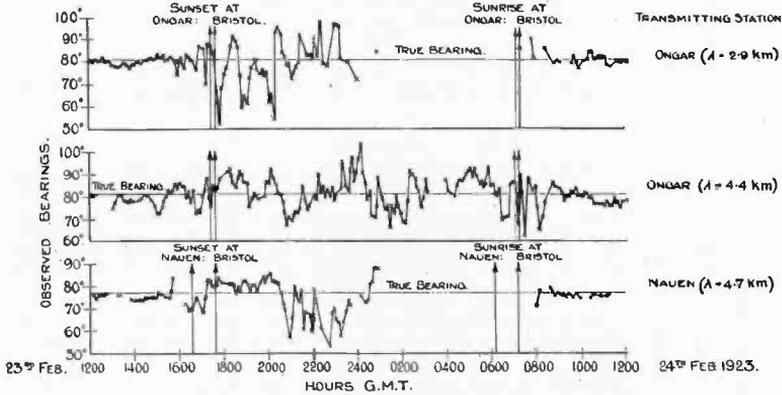
Fig. 6—Graphs of Observed Bearings of Ongar (undamped waves,  $\lambda = 2.9$  and  $4.4$  km) and Nauen (undamped waves,  $\lambda = 4.7$  km) taken at Bristol over a 24-hour period.
