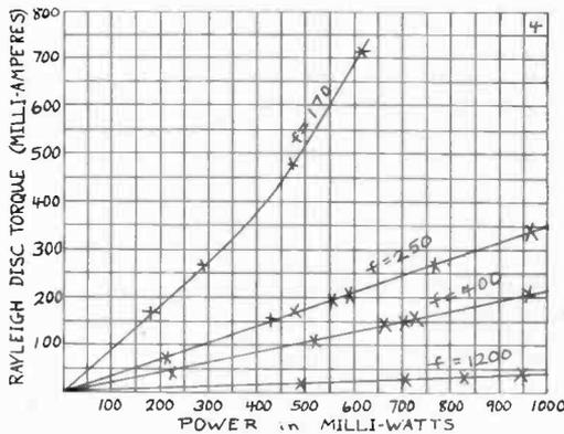
Fig. 7—Sound Intensity Compared to Power Input to the Loudspeaker at Various Frequencies.
