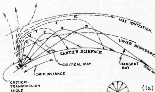
Fig. 1—Sketch Showing the Paths of the Various Rays Radiated by an Ideal Transmitter Having a Characteristic as Sketched in Fig. 1a, as Given by Baker and Rice.
