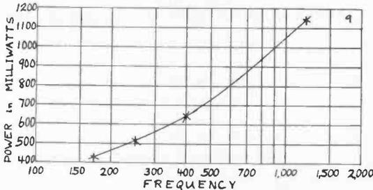
Fig. 13—Power Input Versus Frequency for Equal Apparent Intensity
