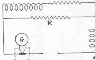
Fig. 10—Schematic Diagram for the Calibration of the Wattmeter.
