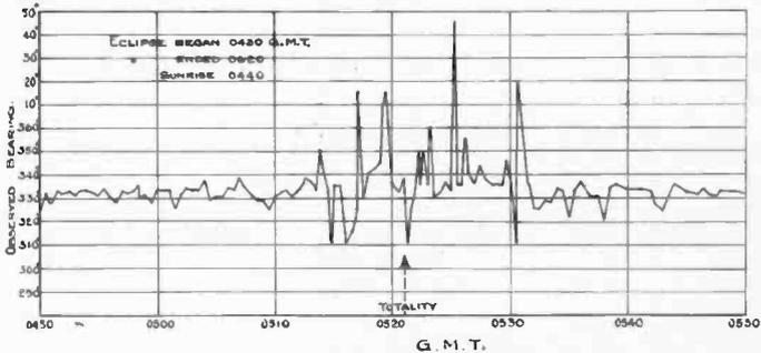
Fig. 12—Observations of Apparent Bearings of Manchester (2ZY) at Slough during the Solar Eclipse, June 29, 1927.
