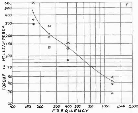
Fig. 12—Observations of Sound Intensity Versus Frequency for Equal Apparent Intensity. (See text for explanation of marks.)
