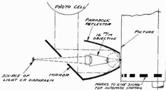
Fig. 1—Optical System of the Picture Machine.
