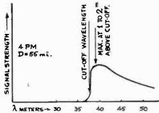
Fig. 5—Illustrating the Variation in Received Signal Strength, for Short Distance Communication, at a Given Time of Day, as a Function of the Wavelength of the Transmitter.
