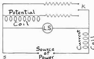
Fig. 9—Schematic Diagram of the Wattmeter Showing Connections to the Source of Power and to the Loudspeaker.
