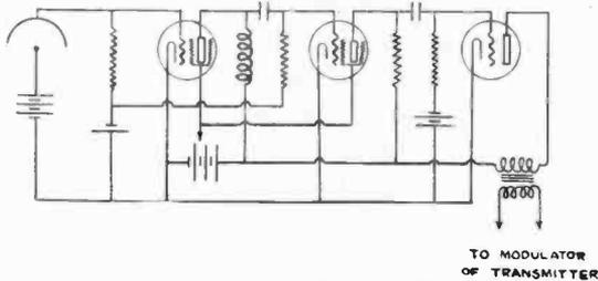
Fig. 7—Photo-Cell Amplifier.
