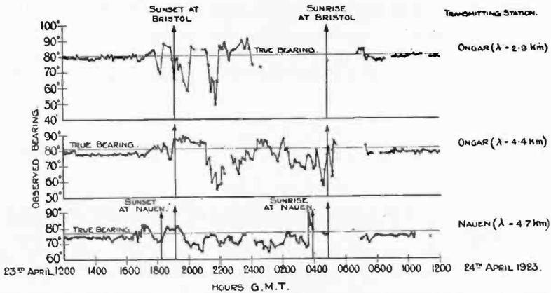
Fig. 7—Graphs of Observed Bearings of Ongar (undamped waves,  $\lambda = 2.9$  and  $4.4$  km) and Nauen (undamped waves,  $\lambda = 4.7$  km) taken at Bristol over a 24-hour period.
