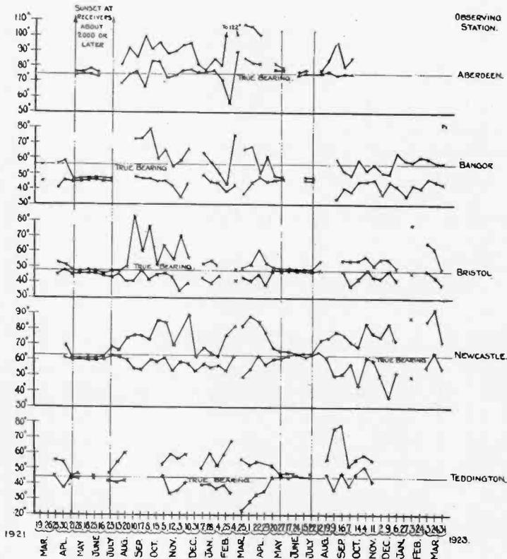
Fig. 9—Graphs of Weekly Extreme Bearings of Karlsborg (damped waves,  $\lambda = 2.5$  km) observed on the transmissions at 2000 G.M.T. during the two years, March, 1921 to March, 1923.
