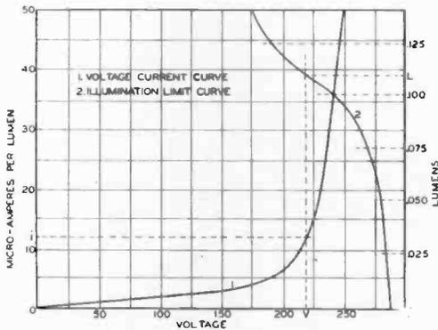
Fig. 6—Characteristics of Gas-Filled Photo-Electric Cell.
