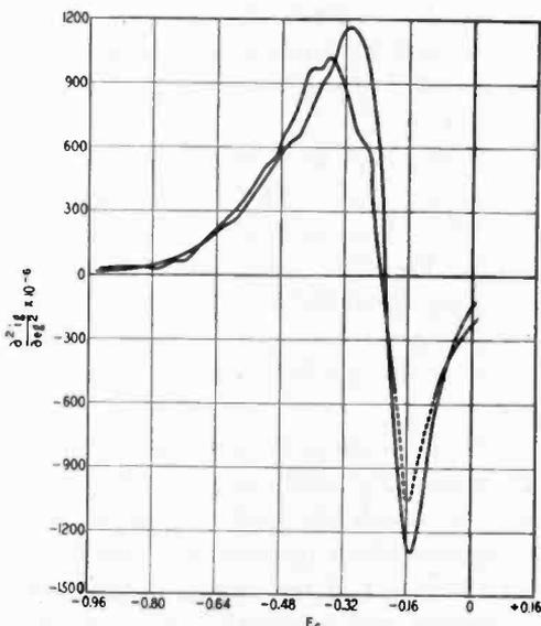
Fig. 3—Variation of Grid Conductance,  $\frac{\partial K_g}{\partial e_g}$ , of Typical C-327 Tube.
