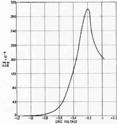
Fig. 2—Grid Conductance,  $\partial i_g / \partial e_g$ , of Typical C-327 Tube.
