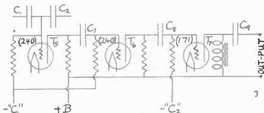
Fig. 4—Resistance Coupled Amplifier. The coupling condensers are  $1 \mu\text{f}$  each. The filaments are in parallel with a common rheostat. Both grid and plate resistances are  $\frac{1}{2}$  megohm each.
