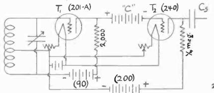
Fig. 3—Oscillator with Conductively Coupled Amplifier.
