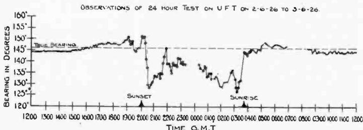
Fig. 11—Graphs of Observed Bearings of Ste. Assise (UFT,  $\lambda = 14.3$  km) taken at Teddington during a 24-hour period, June 2 to 3, 1926.
