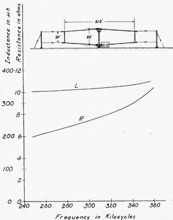
Fig. 31—Variation of antenna resistance and effective inductance with frequency.
