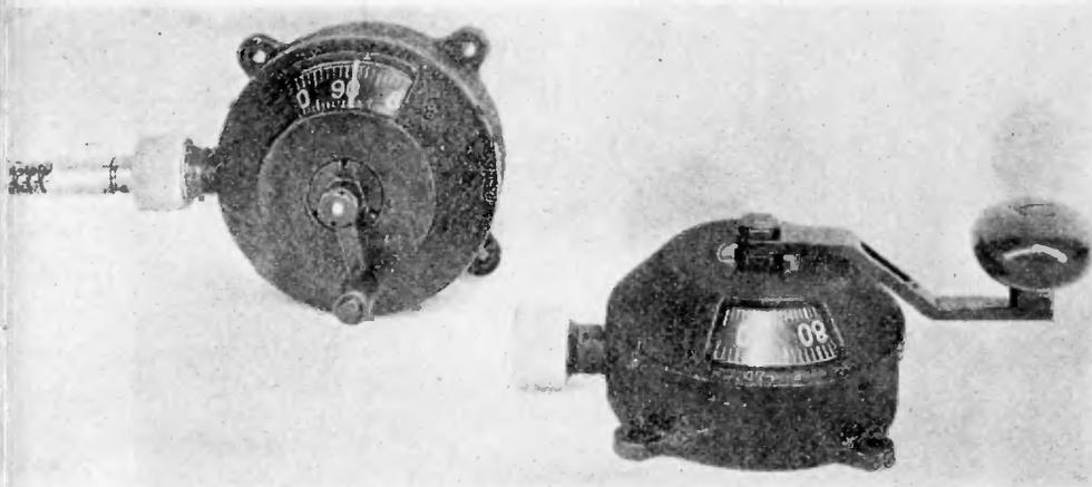
Fig. 7—Two types of tuning control. These may be placed within reach of the pilot and are connected with the condenser drive spindle of the receiver by means of a flexible shaft.
