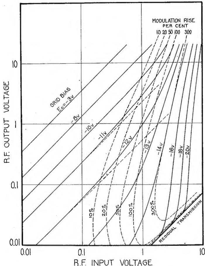
Fig. 2—Input-output voltage diagram for a single tuned r-f amplifier stage employing type 24 tetrode ( $E_b = 180$  v;  $E_a = 90$  v). The dotted lines are contours of constant modulation rise.
