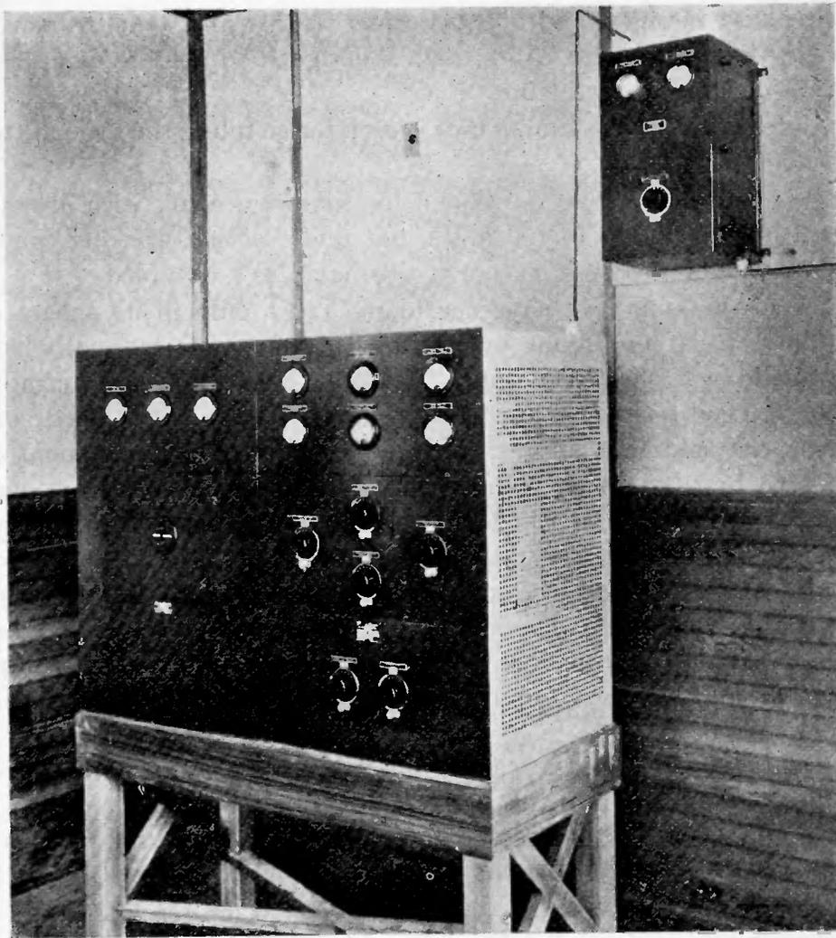
Fig. 11—400-watt ground transmitter developed for communication with aircraft. This shows the power-supply unit, the transmitter, and the antenna tuning unit.
