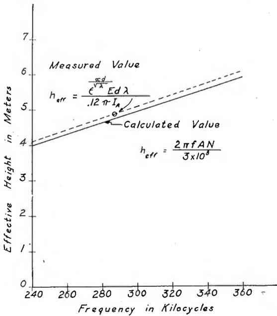
Fig. 32—Variation of effective height with frequency of antenna shown in Fig. 31.
