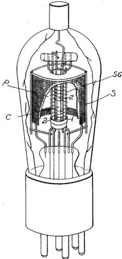
Fig. 12—Structure of tetrode of variable-mu type.
