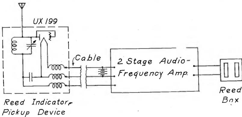
Fig. 33—Schematic diagram of course indicating device.
