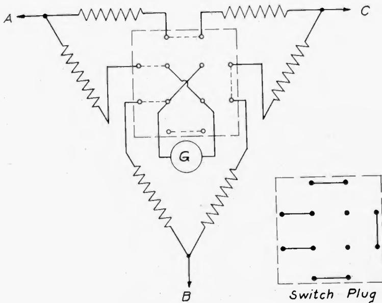
Fig. 22—Diagram showing the connections used in the instrument shown in Fig. 21.
