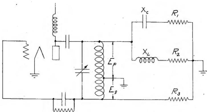
Fig. 15—Diagram showing fundamental circuit utilized in obtaining three-phase radio-frequency supply.
