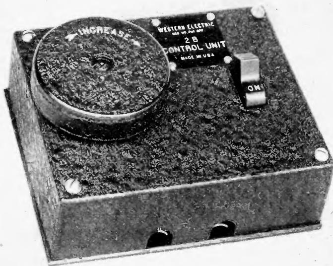
Fig. 6—Remote volume control. This includes a switch for applying power to the filament and plate circuits, and a potentiometer for controlling the shield-grid potential of the radio-frequency tubes.
