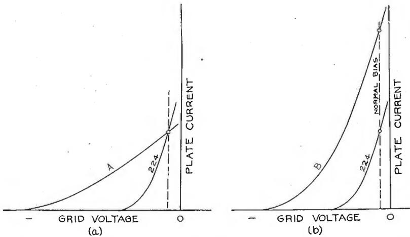
Fig. 10—Showing (a) decreasing transconductance and (b) increasing plate current accompanying attempts to decrease distortion by decreasing the  $\mu$ -factor.
