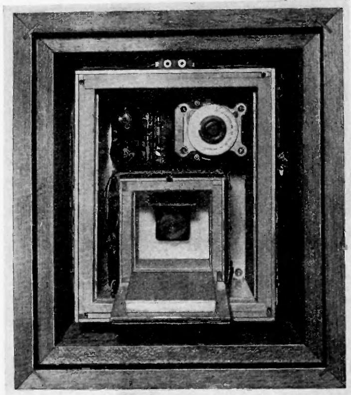
Fig. 4. Top view of complete crystal oscillator with double temperature control. Shows location of crystal holder in inner unit, with thermostat on right wall; oscillator tube, circuits, and isolating amplifier are shown in position in outer unit. Outer thermostat is mounted on left wall. The entire assembly is mounted in a balsa-wood box, with two-inch walls
