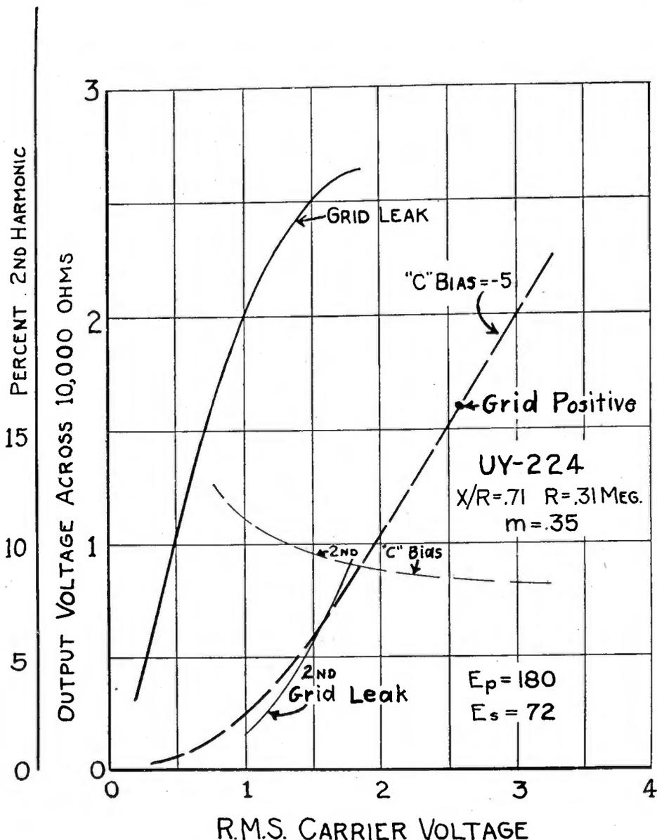
Fig. 7—Comparison of grid leak and plate detection with the screen-grid tube operating at high power levels.
