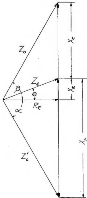
Fig. 27—Impedance vector diagram showing relationship between different vectors.
