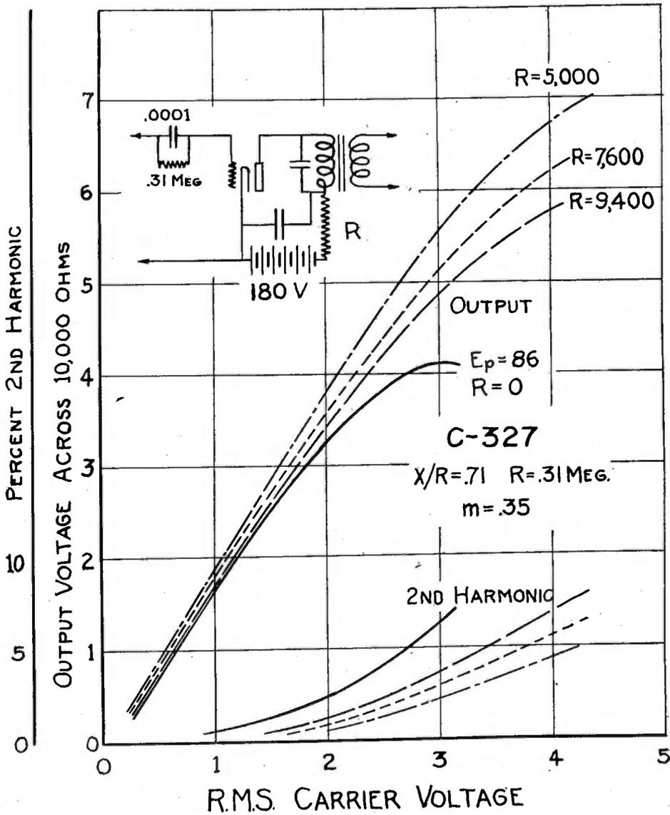
Fig. 6—Performance of grid leak power detector when operated with a high plate battery voltage that is reduced to a safe value by a series resistance, showing increased undistorted output that may be obtained with the aid of this expedient to keep the plate current to a safe magnitude.
