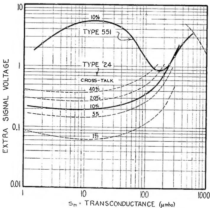
Fig. 8—Diagram showing relation between tube transconductance, produced by grid bias variation, and maximum voltage of interfering signal for various percentages of cross-talk.
