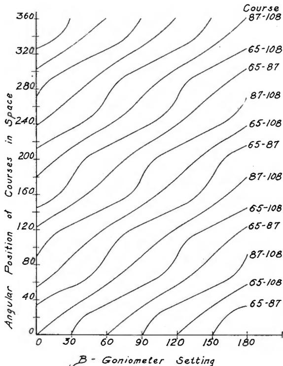
Fig. 12—Effect on course positions caused by deviation of actual goniometer from the perfect sinusoidal characteristic.
