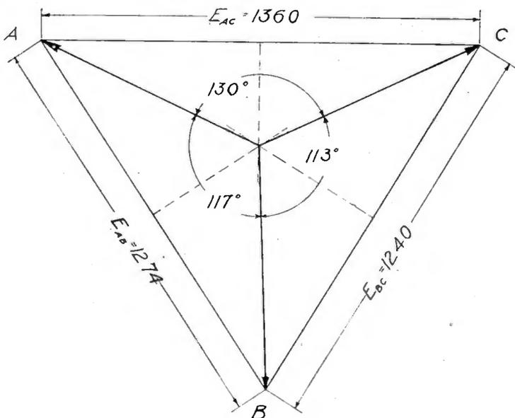
Fig. 20—Vector diagram showing method used to determine the phase relationships between each of the phases when knowing the voltages across each delta branch.
