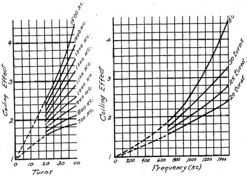
20-MIL WIRE 3.82-IN. COIL DIAMETER. 33.6 TURNS PER INCH.
