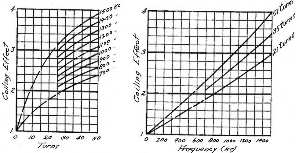
51-MIL WIRE 3.27-IN. COIL DIAMETER. 16 TURNS PER INCH.
