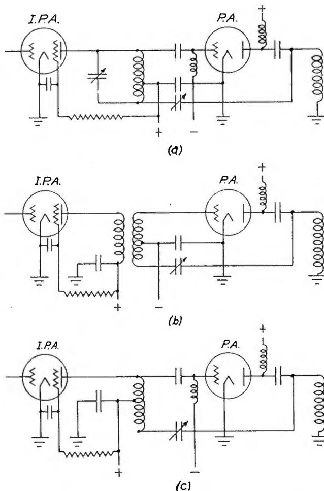
Fig. 14—(a) Schematic diagram of tuned tank coupling. (b) Schematic diagram of transformer coupling. (c) Schematic diagram of impedance coupling.
