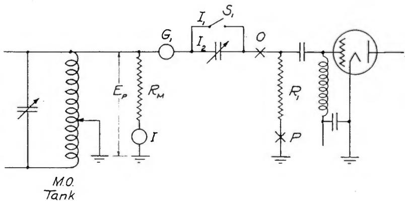
Fig. 29—Schematic diagram showing methods used in determining the voltage ratio.
