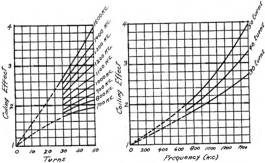
20-MIL WIRE 3.27 IN. COIL DIAMETER. 33.6 TURNS PER INCH.
