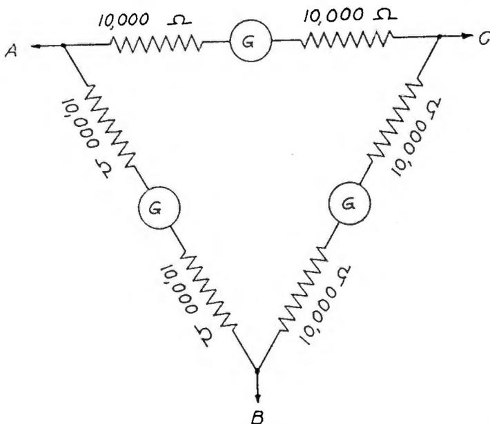
Fig. 19—Diagram showing delta arrangement used to determine the radio-frequency time phase relationship between each of the phases.
