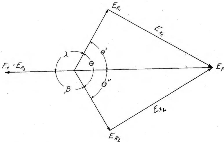
Fig. 16—Vector diagram showing fundamental phase relationships of voltages across  $R_1$ ,  $R_2$ , and  $R_3$  in Fig. 15.
