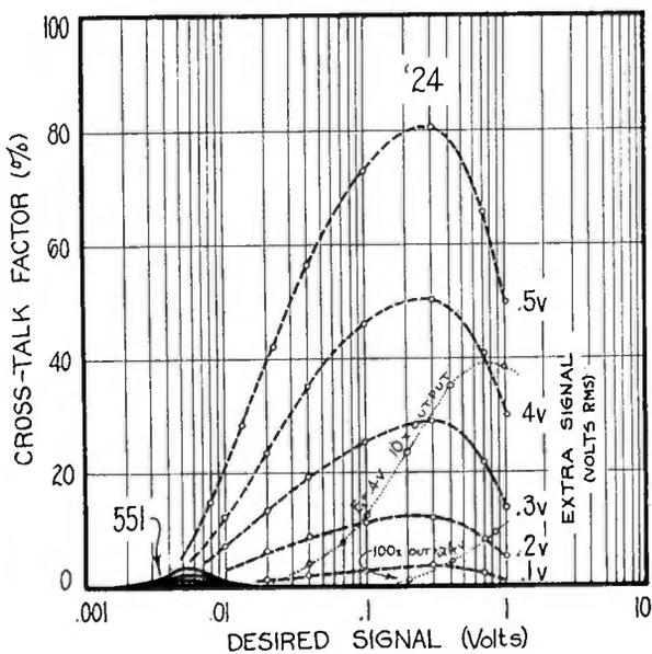
Fig. 7—Experimental curves showing cross-talk production in 24 and 551 tetrodes. Constant output maintained, corresponding to 0.001 volt desired signal at -3-volt bias.
