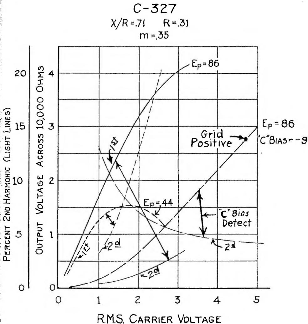
Fig. 4—Performance of grid leak and “C” bias power detectors under favorable conditions. The solid and dotted lines are for grid leak detection, while the dash line applies to plate rectification.
