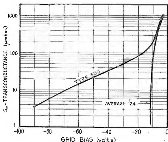
Fig. 16—Transconductance-grid voltage characteristic of Types 550 and 24 tubes.
