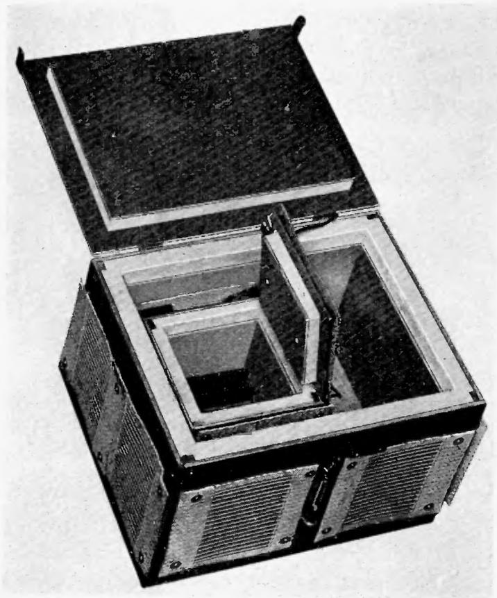
Fig. 5. The interior assembly of the double temperature-control box is here shown removed from the balsa-wood insulating container. The unit inside the larger box has heaters on all six faces, controlled by a thermostat mounted on the rear face. The outer unit also has heaters distributed over all six faces, the thermostat being mounted at the center of the front face.
