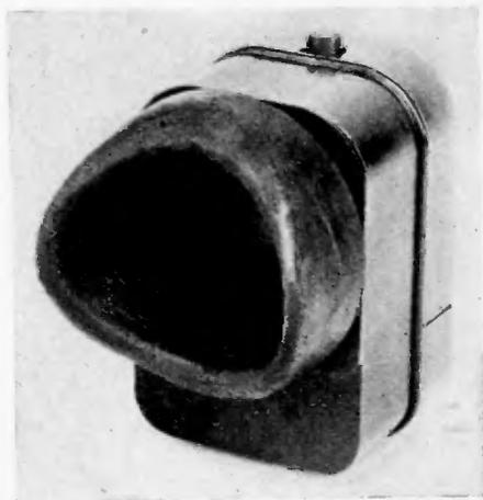
Fig. 9—Type of microphone for use in aircraft where the noise level is high. The push button on the top is pressed for speaking and controls the oscillations in the transmitter.
