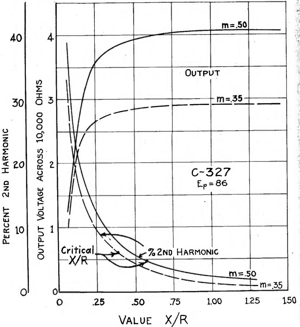
Fig. 5—Effect of  $X/R$  on sensitivity and quality, showing how both rapidly become poorer when the critical value of  $X/R$  as determined from Fig. 2 is passed.
