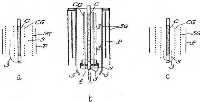
Fig. 14—Several types of variable-mu structure.
