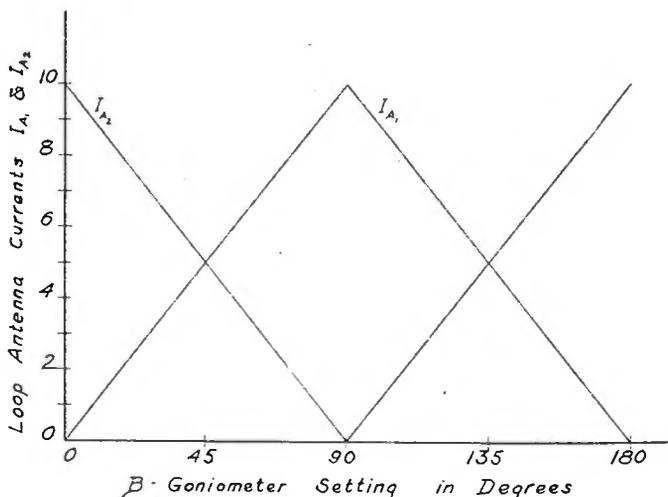
Fig. 8—Linear characteristics of a theoretical goniometer, showing the relation between goniometer setting and antenna current.
