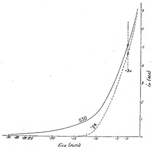
Fig. 15—Plate current-grid voltage characteristic of variable-mu tube showing reshaped characteristic for reduction of distortion and cross-talk.
