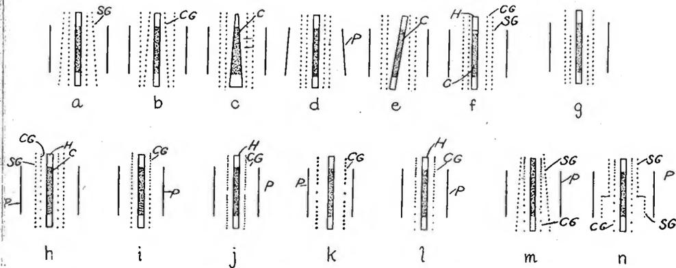
Fig. 13—Illustrating several types of variable-mu tube structure.
