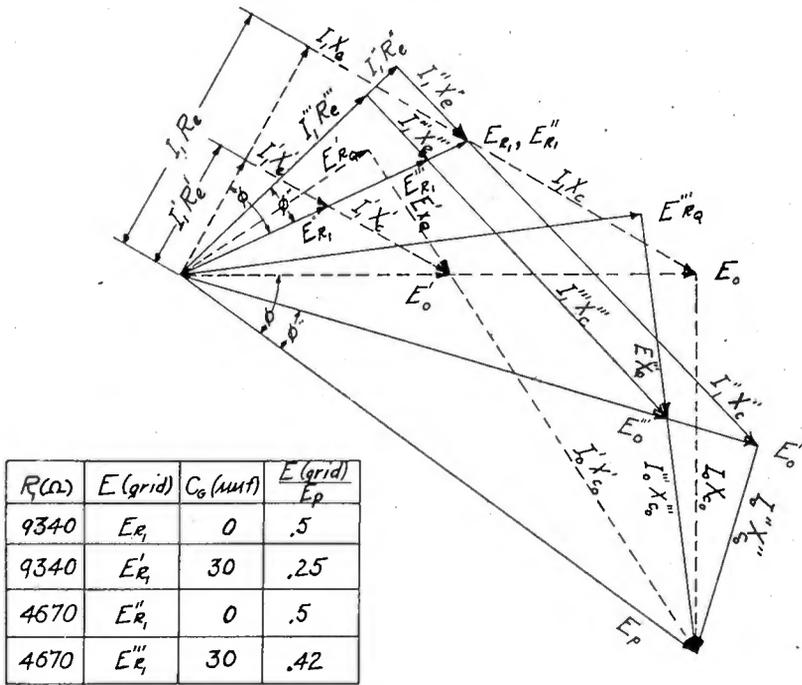
Fig. 24—Vector diagram showing the greatly reduced effect of  $C_G$  on the available voltage supplied to the tube when utilizing a low value of shunt resistance.
