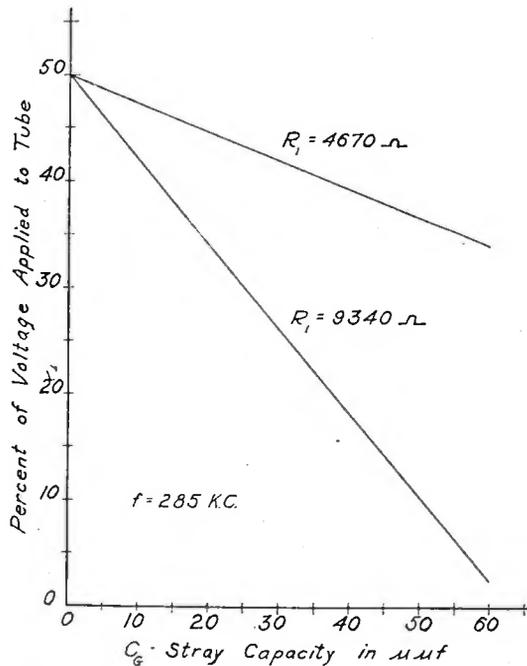
Fig. 26—Curves showing effect of stray capacity upon the per cent of total voltage  $E_p$  capable of application to the tube with different values of  $R_1$ .
