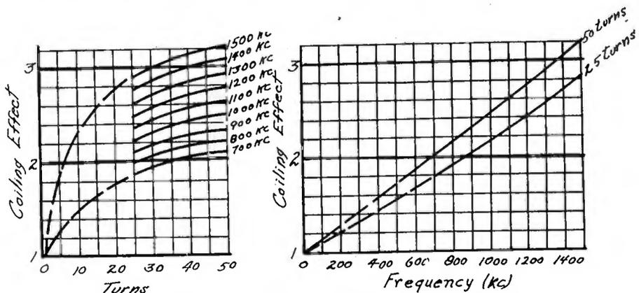
40-MIL WIRE 2.68-IN. COIL DIAMETER. 19.6 TURNS PER INCH. RESISTANCE RATIO FOR 40-MIL WIRE (STRAIGHT) GIVEN ABOVE.
