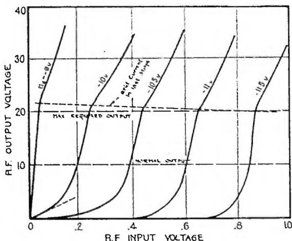
Fig. 1—Relation between input and output voltages in a 4-stage r-f amplifier employing 227 tubes ( $E_b = 90$  v) showing nonlinearity at high input voltages.
