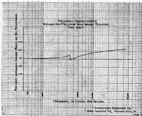
cycles is so low that it can be used in the most exacting work. It will be noticed that the break in the curve is almost imperceptible. The temperature co-efficient of resistance is 0.0002 per °C. These resistors have a safe power rating of 1 watt.
