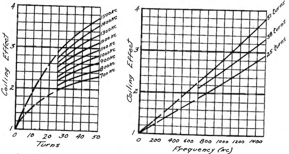
40-MIL WIRE 3.27-IN. COIL DIAMETER. 19.6 TURNS PER INCH.
