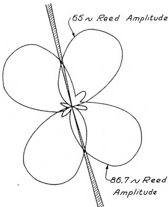
Fig. 35—Observed reed amplitude space patterns of a two-course radio range.
