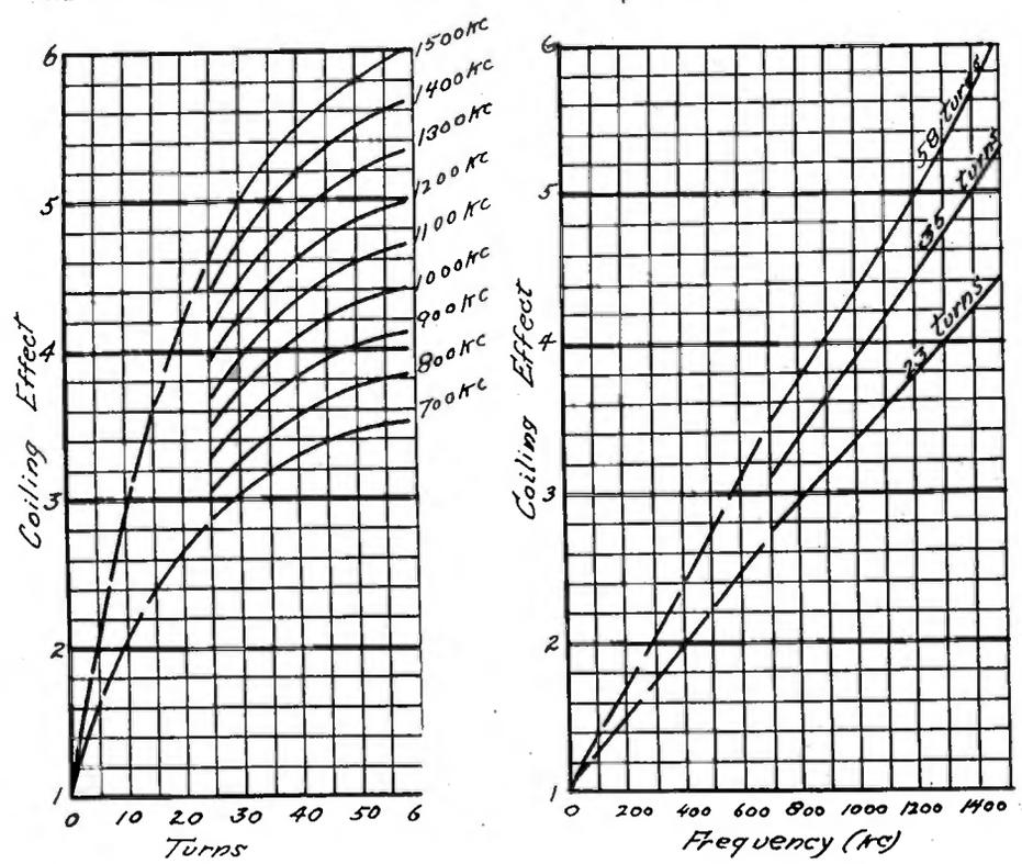
S.C.C. 40-MIL WIRE ALLOWING 21.7 TURNS PER INCH ON A WINDING DIAMETER OF 3.82 INCHES SHOWING INCREASED COILING EFFECT WITH SMALLER PITCH.
