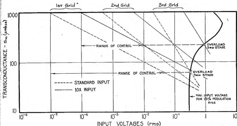
Fig. 4—Control analysis: Diagram of input voltages in a 3-stage amplifier employing 24 tetrodes; controlled by common grid bias in all stages.
