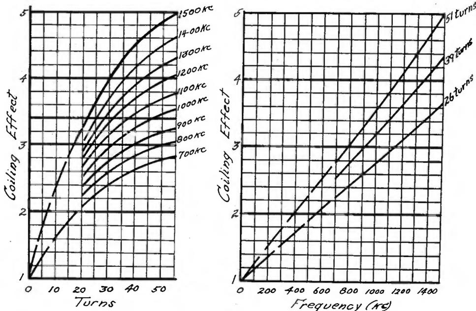
51-MIL WIRE 3.82-IN. COIL DIAMETER. 16 TURNS PER INCH.
