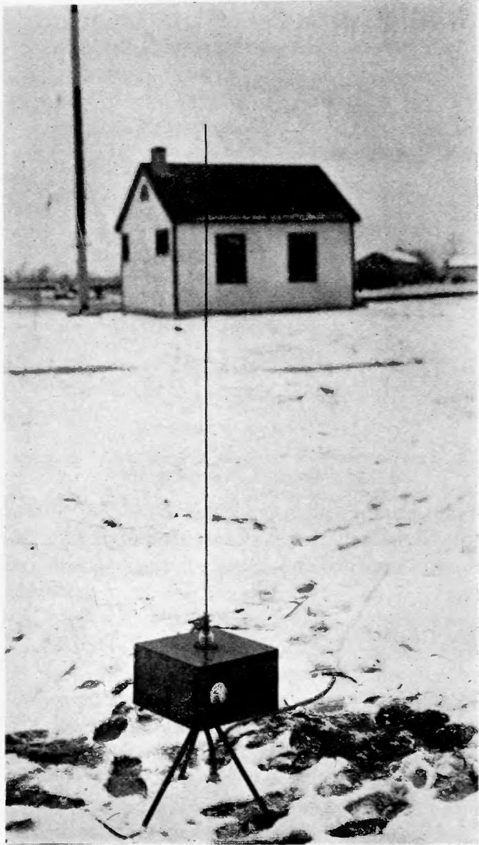
Fig. 34—Pick-up unit of course indicating device.
