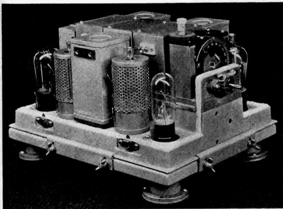
Fig. 4—Aircraft radio receiver with cover removed showing cushioned mounting base.
