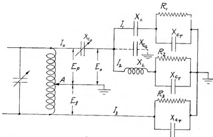
Fig. 17—Diagram showing final circuit adopted to obtain a three-phase radio-frequency supply.
