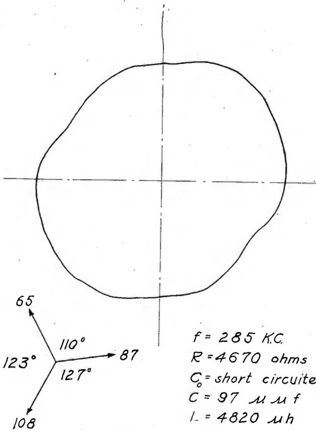
Fig. 23—Vector diagram showing time-phase relationships and the resultant polar diagram of  $I_A$ , plotted against the goniometer setting. (a), (b), and (c) show the effect of varying  $C_0$ . (d) shows the effect of making  $R$  relatively large.
