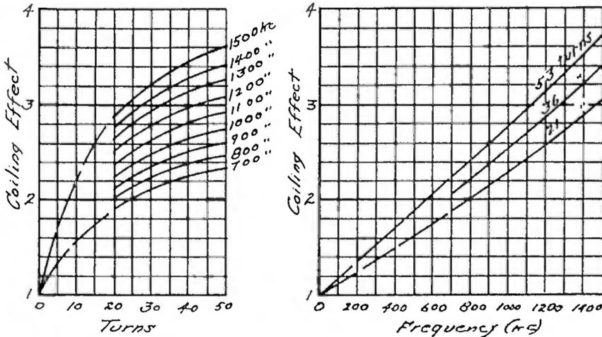
51-MIL WIRE 2.68-IN. COIL DIAMETER. 16 TURNS PER INCH. RESISTANCE RATIO FOR 51-MIL STRAIGHT WIRE GIVEN ABOVE.
