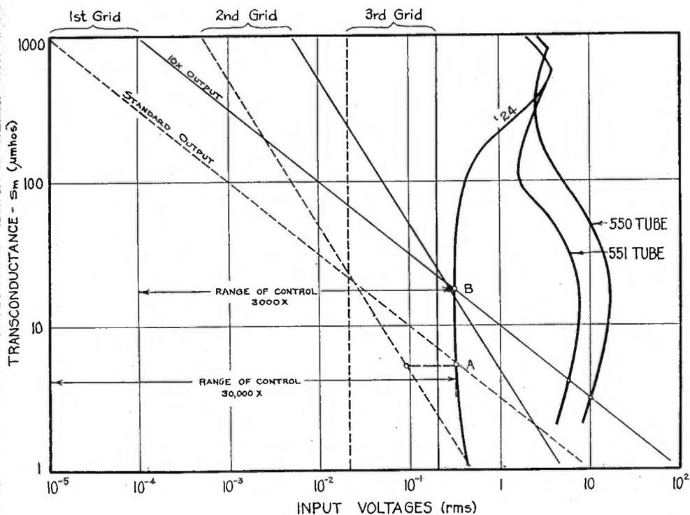
Fig. 5—Control analysis for graduated bias control; stage 3 uncontrolled; stages 1 and 2 controlled by common bias. Other conditions identical with Fig. 4.
