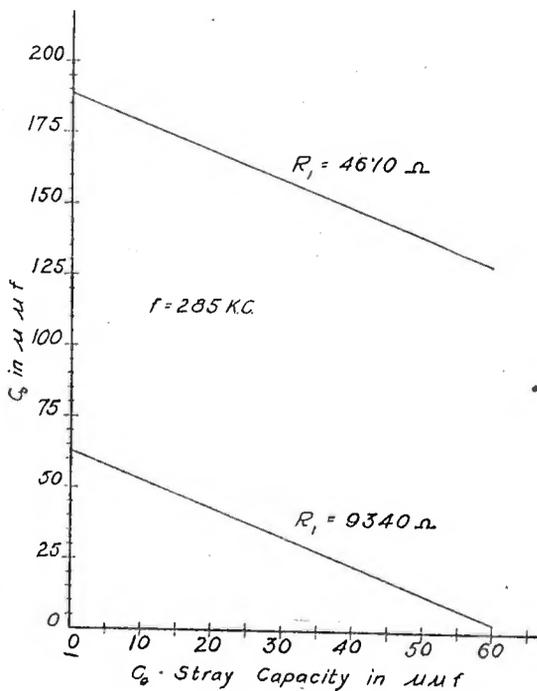
Fig. 25—Curves showing the value of  $C_0$  required to maintain 120-degree time-phase displacements for different values of stray capacity when utilizing two different values of tube shunt resistance.
