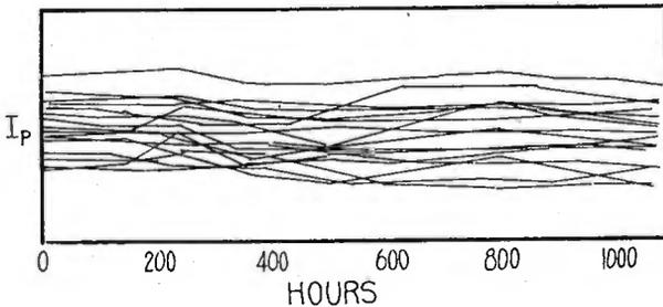
Fig. 18—Typical results of 1000-hour life test on current from low- $\mu$  area of Type 551 cathode.
