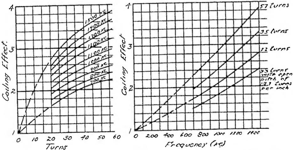
32-MIL WIRE 3.27-IN. COIL DIAMETER. 22 TURNS PER INCH (CLOSED PITCH)
