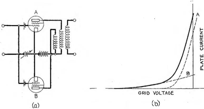
Fig. 11—Method of decreasing distortion and cross-talk.
