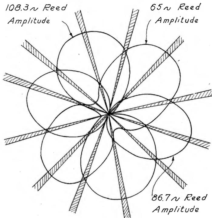
Fig. 37—Observed reed amplitude space patterns of a twelve-course radio range.
