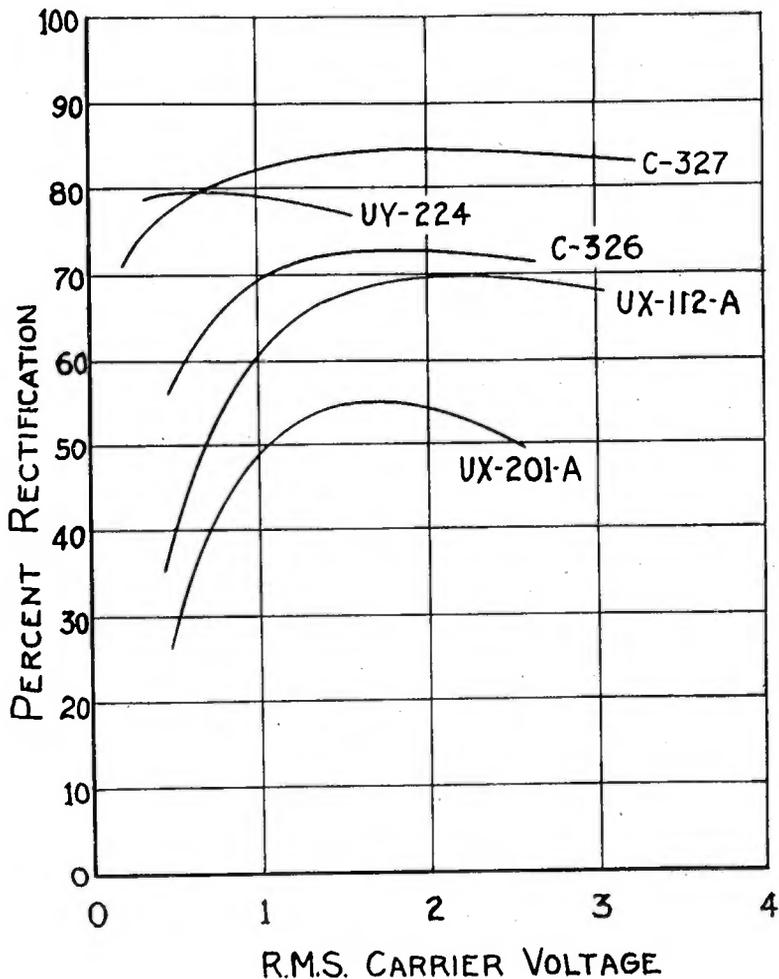
Fig. 8—Completeness of grid leak power detection as a function of signal amplitude for a number of representative tubes.
