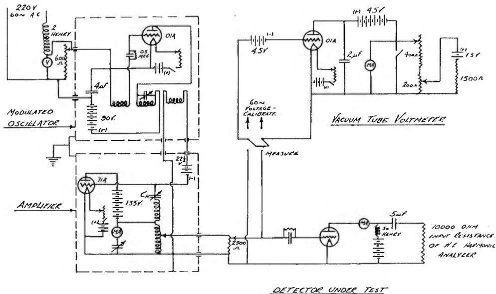
Fig. 9—Circuit diagram of experimental set-up used in making measurements on grid leak power detectors.
