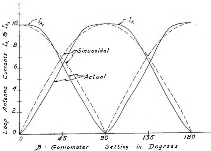
Fig. 11—Final goniometer characteristic showing deviation from theoretically perfect type.
