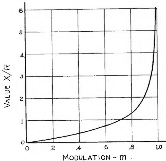
Fig. 2—Graph of the equation ( $X/R = m/\sqrt{1 - m^2}$ ) showing the relation of  $X/R$  to  $m$  at which distortion begins to become serious.
