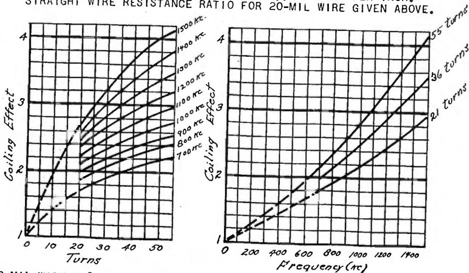
32-MIL WIRE 3.82-IN. COIL DIAMETER. 22 TURNS PER INCH.
