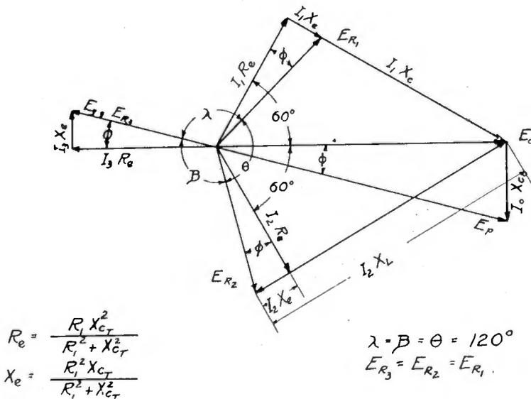
Fig. 18—Vector diagram showing phase relationships of voltages existing in Fig. 17.
