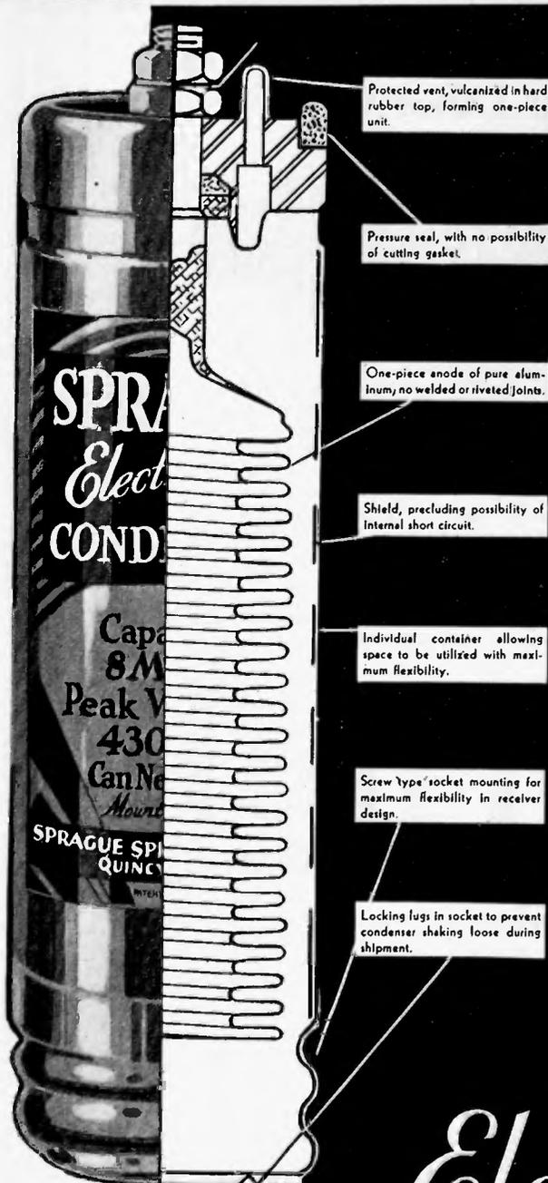
WHEN you take a look at the Sprague condenser's "innards", you'll see why this new type electrolytic condenser has literally swept the radio industry off its feet, for here's a standardized unit of 9 MFD capacity, with a rating of 430 volts DC, in a space of 1 3/8" diameter x 4 11/16" height.
