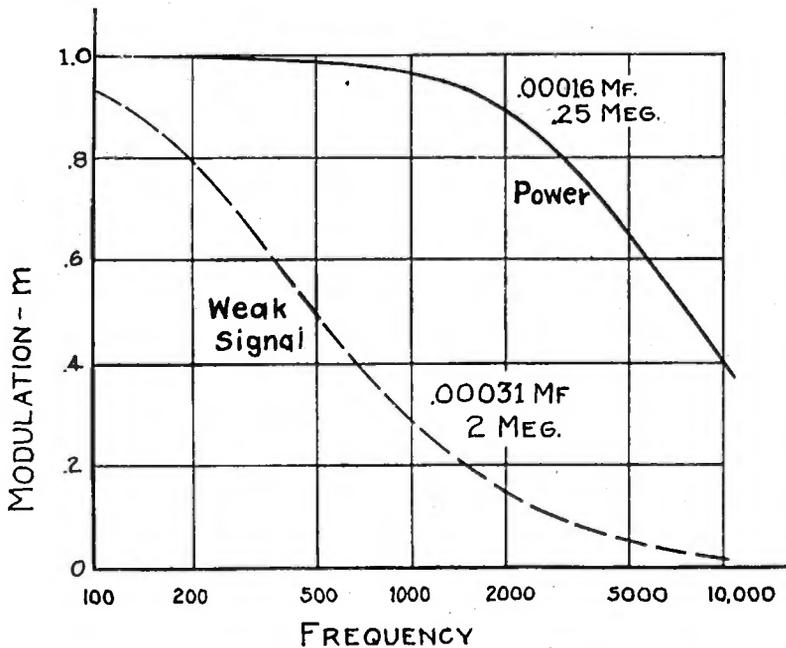
Fig. 3—Allowable  $m$  as a function of modulation frequency for grid leak power detection for proportions of grid leak and condenser suitable for weak signal detection compared with those recommended for power detection.
