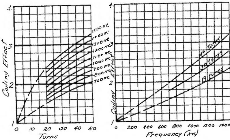
32-MIL WIRE 2.68-IN. COIL DIAMETER. 22 TURNS PER INCH.
