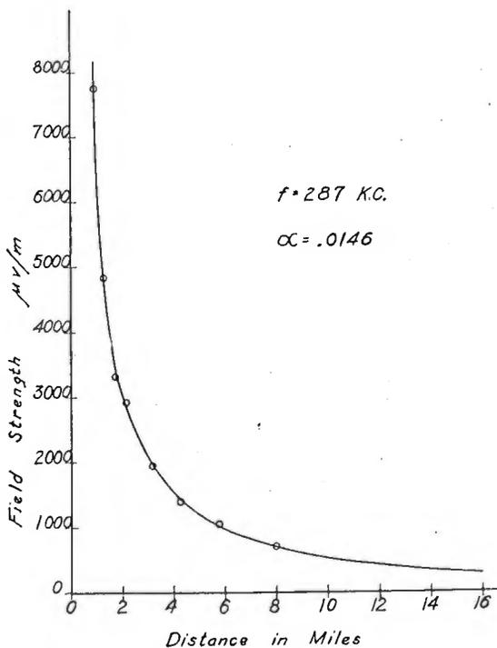
Fig. 38—Attenuation curve showing the field strength of the polydirectional radio range at different distances from the station.
