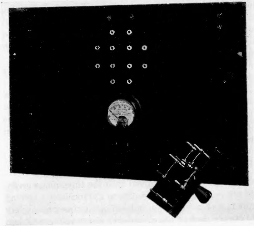
Fig. 21—View showing device used in determining the radio-frequency phase relationships.
