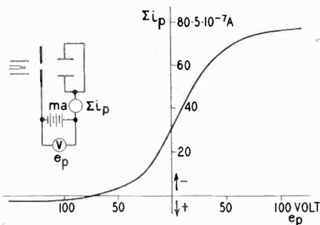
FIG. 12—Total plate current and plate bias.
