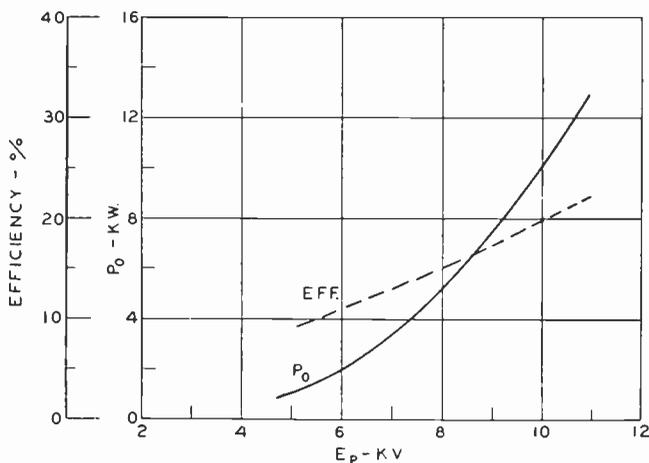
Fig. 13—Standing wave oscillator.  $\lambda = 2.8$  meters.
