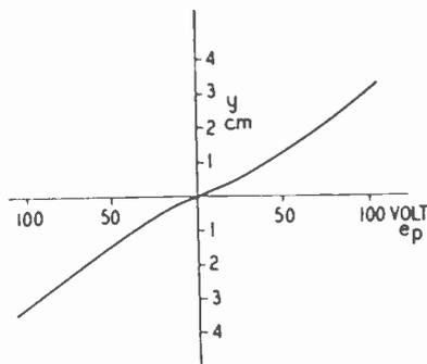
FIG. 15—Typical curve for cathode ray deflection as a function of the deflecting potentials.
