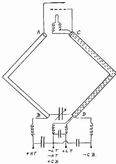
Fig. 4—Schematic of oscillator used in experiments.
