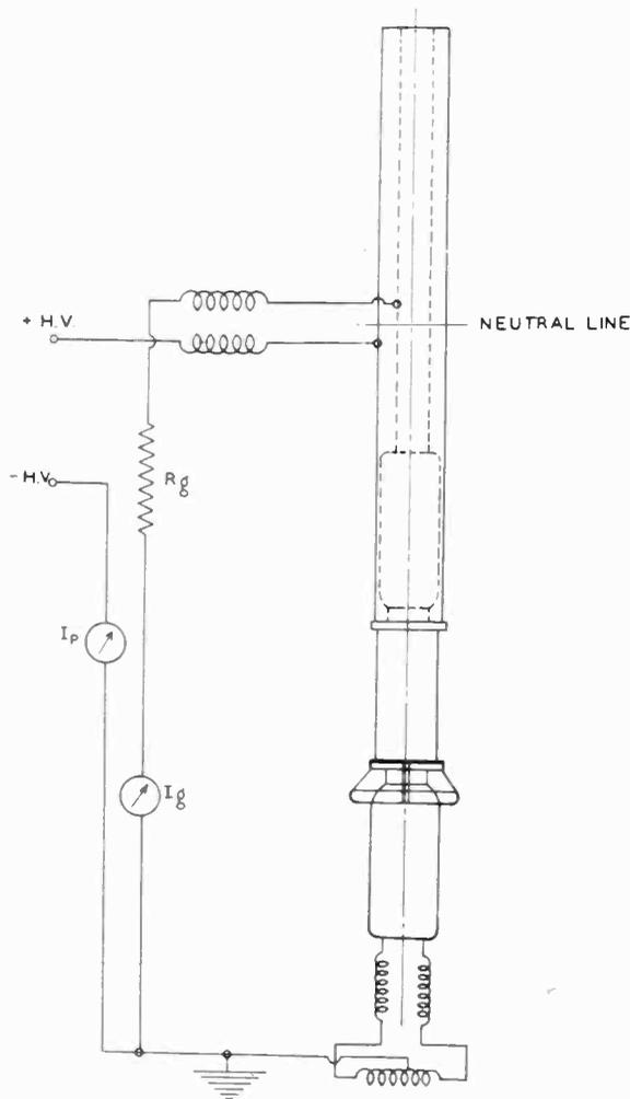
Fig. 7—Oscillating circuit using AW-200 tube.
