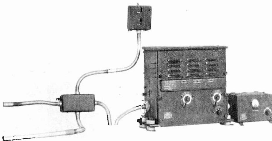
Fig. 7—Complete aircraft transmitter equipment type RT-76-A.
