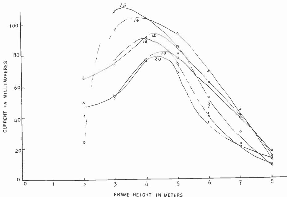
Fig. 12—Variation of received current with frame height for formatised frames of a given area.
