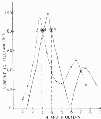
Fig. 9—Variation of received current with dimension of frame aerial (In one case  $H$  is kept at 3 meters while  $W$  is varied as indicated. In the other case  $W$  is kept at 4 meters while  $H$  is varied.)
