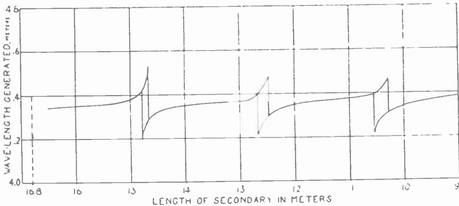
Fig. 13—Experimental curve of the wavelength generated by the bridged-end secondary two-circuit oscillator for different lengths of the secondary.
