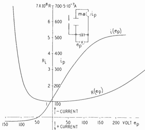
FIG. 14. Resistance of an argon-filled Braun tube
