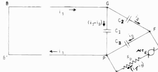
Fig. 2—Schematic circuit diagram of the simple oscillator.
