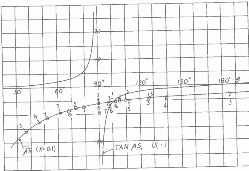
Fig. 8—Graphical solution of (22). Intersections with the first four branches of the cotangent curve are denoted respectively by circles, squares, triangles, and crosses. The numbers written in are the values of  $s_2$  in each case.
