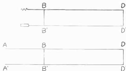
Fig. 7—Schematic diagram of actual and idealized circuits for a bridged-end secondary.
