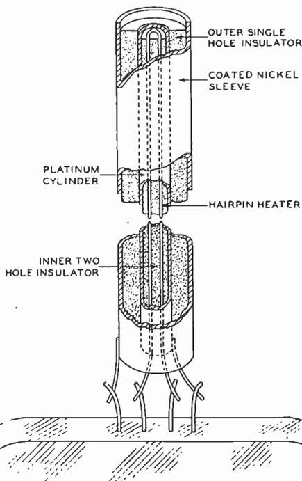
Fig. 6—Experimental heater arrangement for the study of the magnetic effect.
