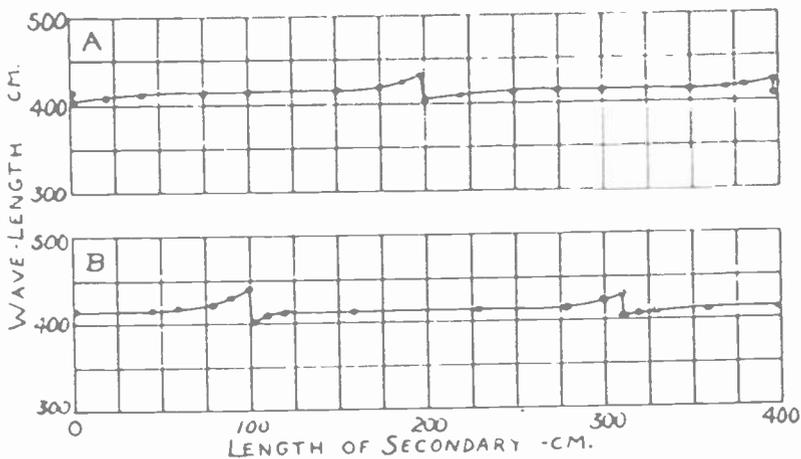
Fig. 11—Experimental wavelength characteristics with the secondary bridged at the end  $EE'$  in curve A, open at this end in curve B.
