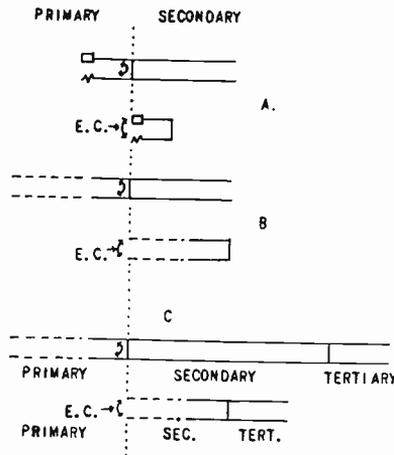
Fig. 15—Electron and regenerative circuits compared. The upper diagram in each pair is for the regenerative, the lower for the electron oscillator. *E.C.* = electron cloud.
