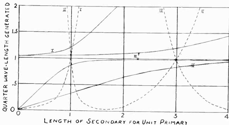
Fig. 10—Theoretical characteristics like those of Fig. 4 but derived assuming mutual distributed coupling instead of coupling through the bridge  $BB'$ .
