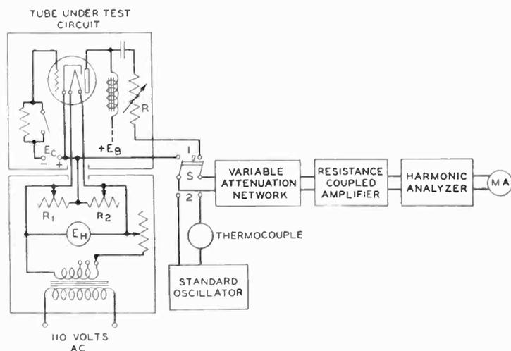
Fig. 1—Schematic diagram of disturbance current measuring circuit.
