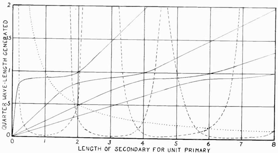
Fig. 9—Theoretical curves for wavelength (solid lines), damping (dashed lines), and excitation for  $N = 2r$  (dotted line) for the bridged-end secondary. The legend is the same as that of Fig. 4.
