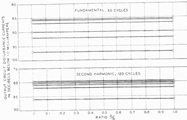
Fig. 3—Disturbance currents in indirectly heated cathode triodes having shields to reduce the electric field of the heater in the cathode-plate space.
