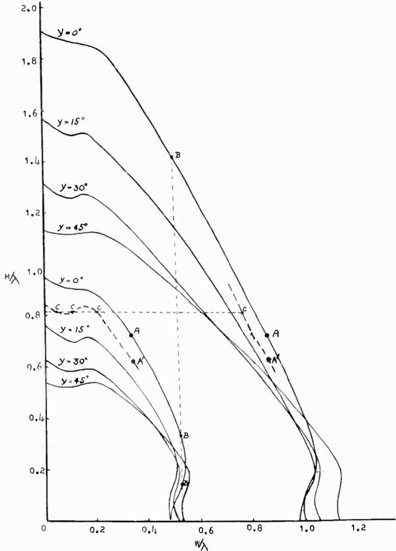
Fig. 3—Graphs showing frame dimension for which lag or lead angles between currents in sides are compensated by corresponding lead or lag angles in top and bottom.
