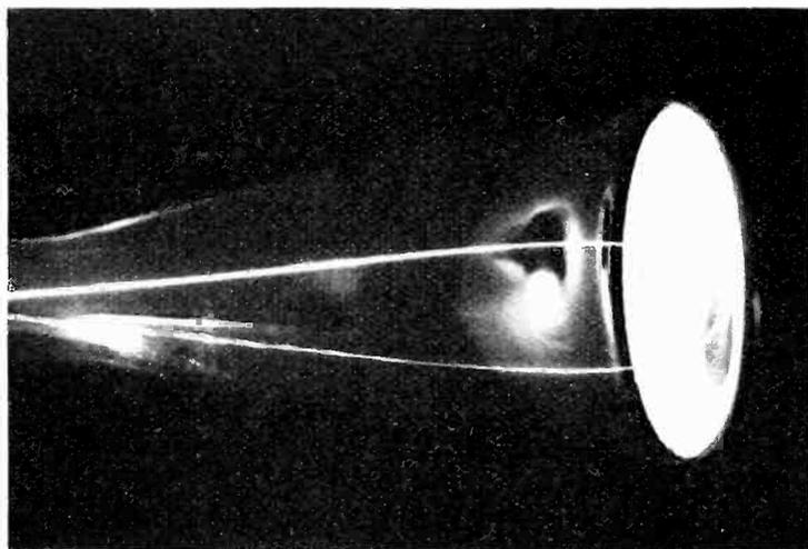
FIG. 10—Simultaneous deflection of stray electrons and beam by a magnetic field.
