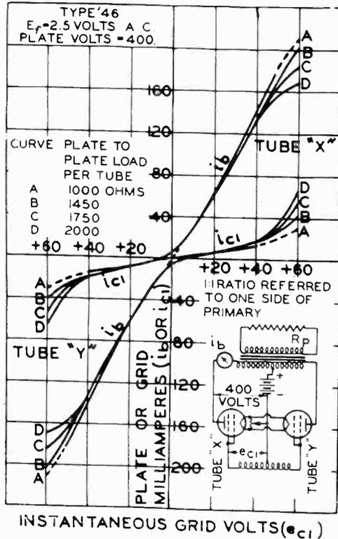
Fig. 13—Dynamic transfer characteristics. Class B operation.
