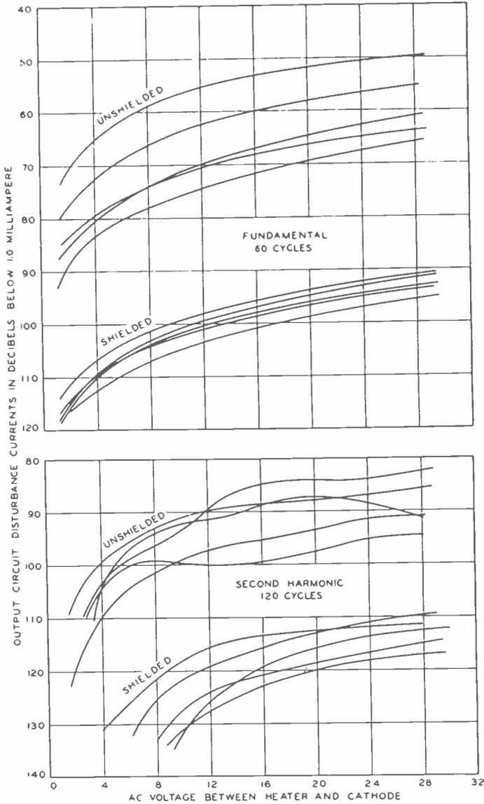
Fig. 5—Disturbance current measurements on shielded and unshielded tubes with the circuit of Fig. 4.
