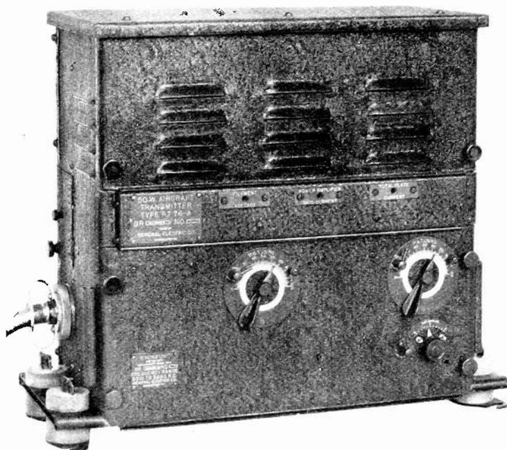
Fig. 8—Transmitter, type RT-76-A.
