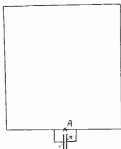
Fig. 8—Electrical circuit of adjustable frame aërial.
