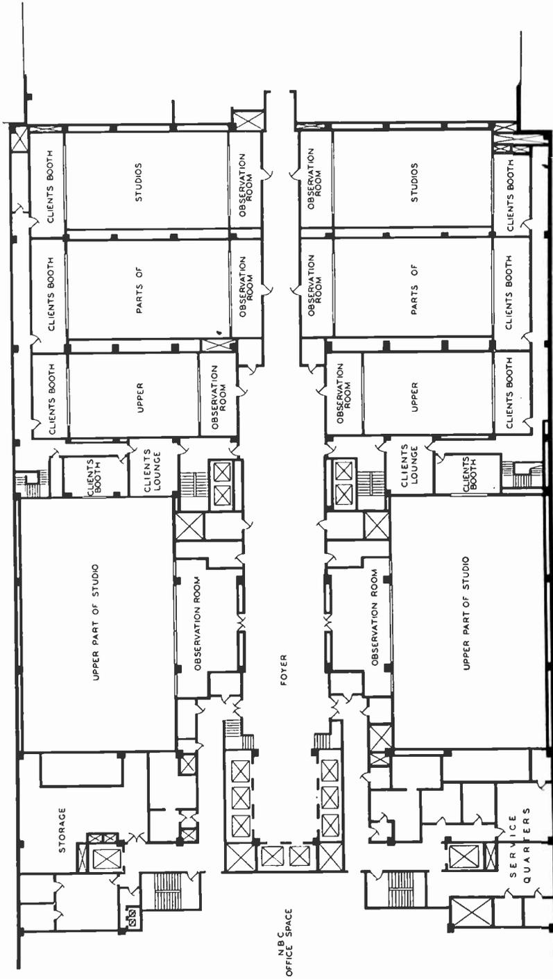
Fig. 6—Typical observation floor plan. Fifth and eighth floors.
