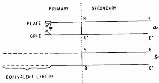
Fig. 1—Actual and idealized triode oscillatory circuit including an open-end variable secondary with distributed constants.
