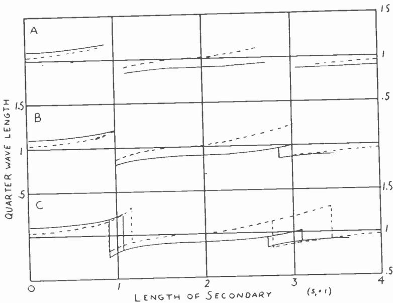
Fig. 5—Typical wavelength characteristics of the idealized coupled-circuit oscillator with an open-end secondary. The negative resistance is taken small for A, near critical for B, large for C.
