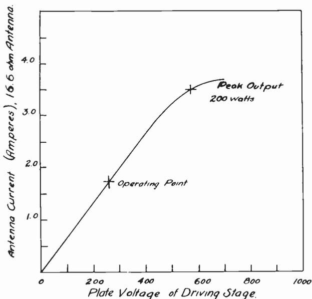
Fig. 1—Typical operation of a UV-211 as a class B amplifier. Drawing stage, UX-210.
