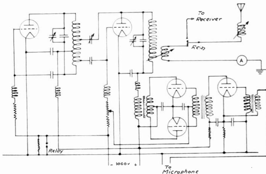
Fig. 3—Schematic diagram, RT-76-A transmitter.
