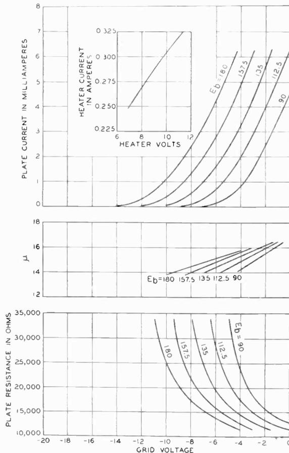
Fig. 11—Electrical characteristics of the No. 262A tube.
