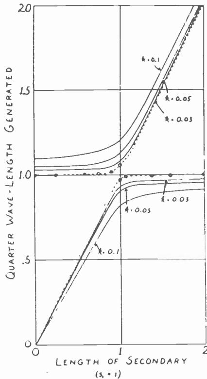
Fig. 6. Theoretical wavelength characteristics of the idealized coupled-circuit oscillator with open-end secondary for three different values of the coefficient  $k$ , (solid lines). A typical experimental curve is shown dotted.
