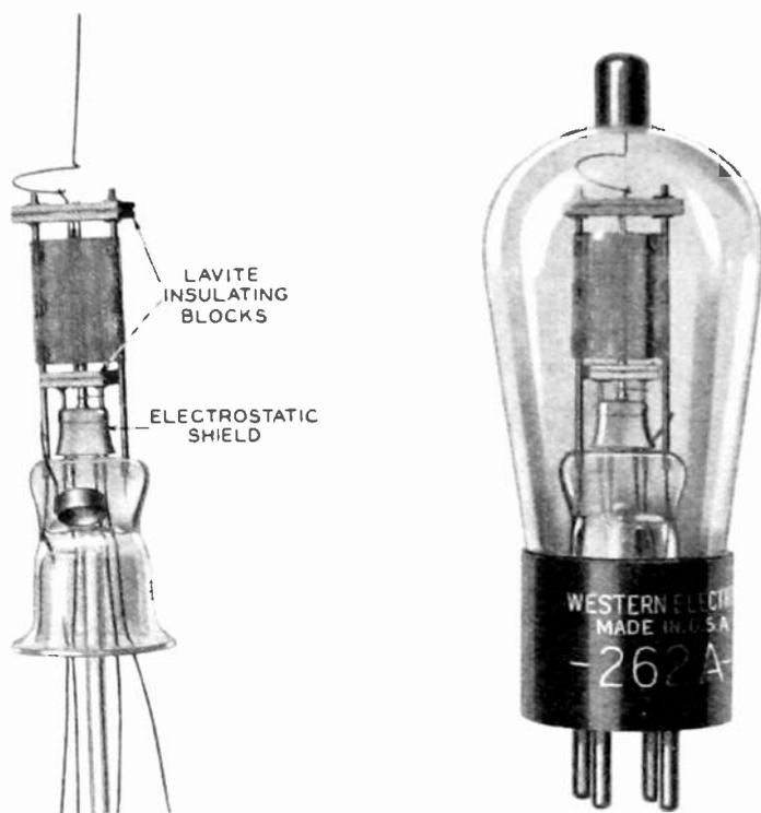
Fig. 10--No. 262A mount and completed tube.
