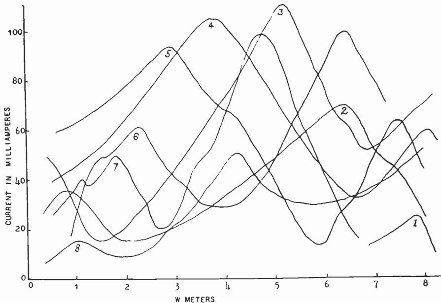
Fig. 10—Variation of received current with width ( $W$ ) of frame aerial.
