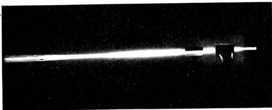
FIG. 4—200-volt beam in inert gas under  $10^{-3}$ -mm pressure.
