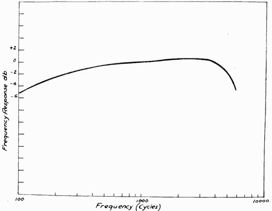
Fig. 4—Frequency response, RT-76-A transmitter.
