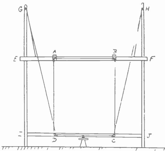
Fig. 7—Mechanical arrangement of adjustable frame aerial.
