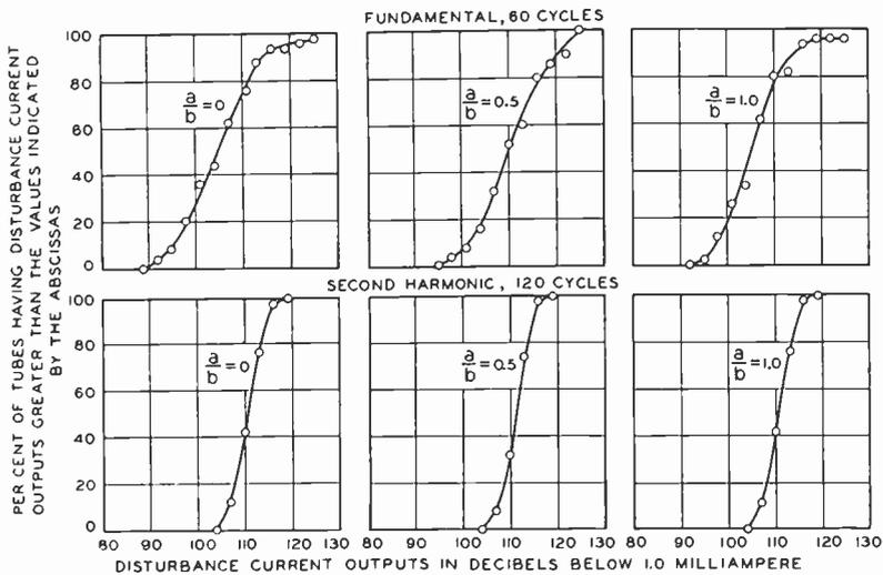
Fig. 12— Distribution of disturbance output currents in a representative number of No. 262A tubes picked at random.
