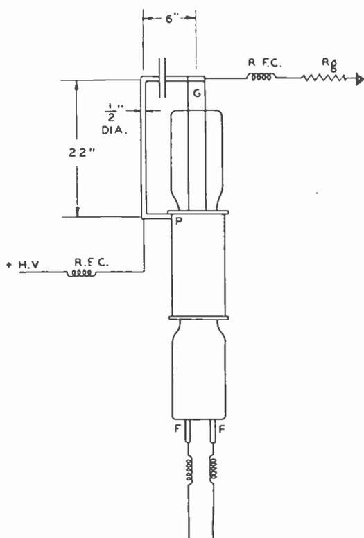
Fig. 8—Shortest connections for Hartley oscillator.  $\lambda = 6$  meters.
