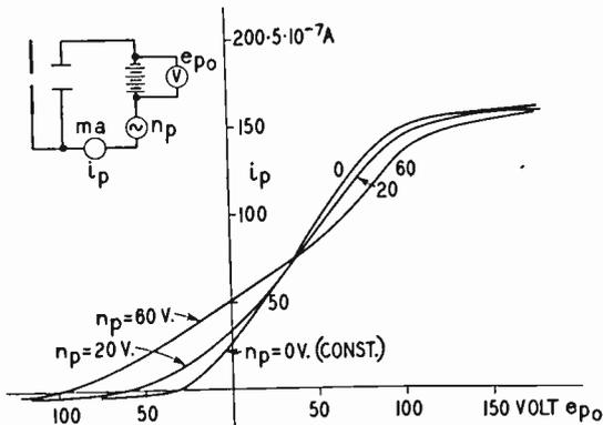
FIG. 13—Directional characteristic of the current across the deflection plates.
