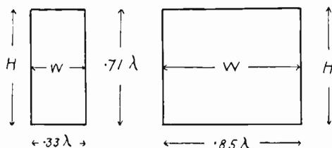
Fig. 2—Two critical dimensions of a frame aerial corresponding to optimum received current when  $\gamma$  equals zero.
