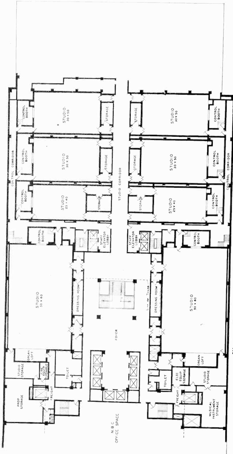
Fig. 4—Typical studio floor plan, National Broadcasting Company—
