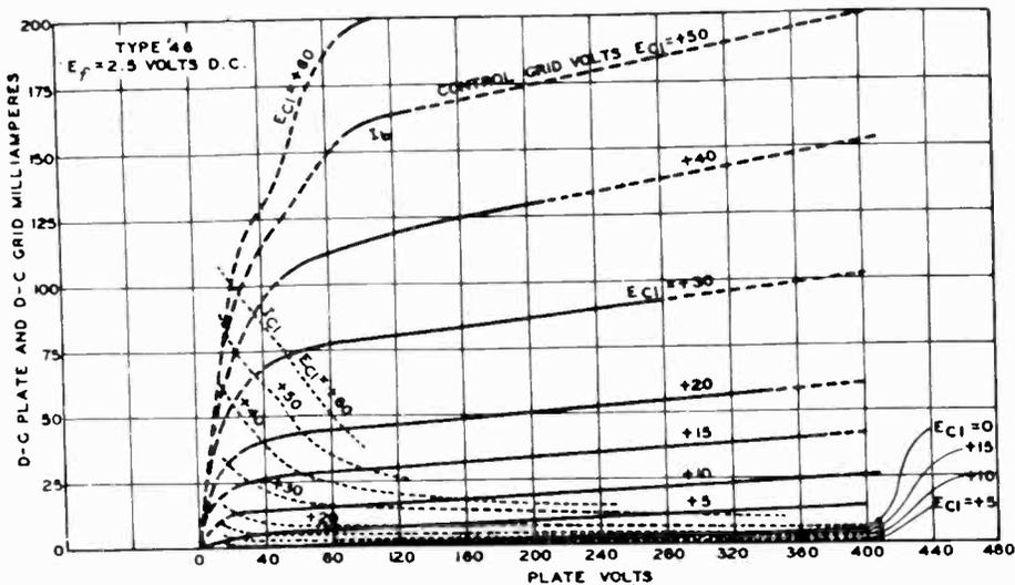
Fig. 12—Average plate characteristics. Class B operation.
