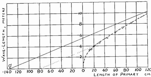
Fig. 3—Actual and idealized calibration curves of the simple oscillator.
