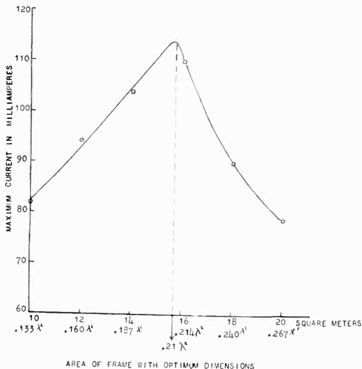
Fig. 13—Variation of received current with area for optimum ratios of width to height.
