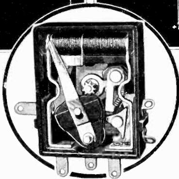
A single-pole line switch approved by the Underwriters' Laboratories and the Hydro Electric Power Commission of Ontario with a rating of 2 amperes, 125 volts, can be provided within the Bradleyometer and is operated by the regulator control knob.
