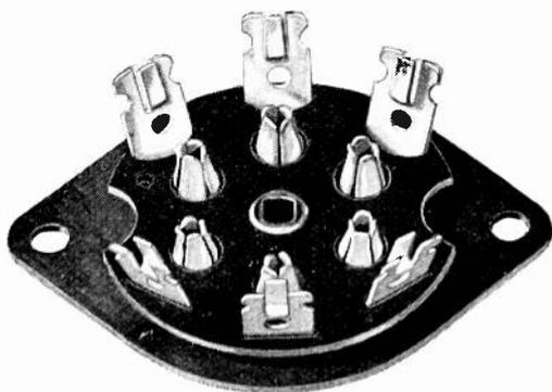
Another Cinch achievement! A new radio socket . . . with *floating contacts*. Scientifically designed to eliminate *all* strain on the bakelite . . . preventing warping and loss of tension after tube is inserted. *Floating* principle makes contacts self-aligning assuring a constant, rigid contact on each tube prong. Three styles of contacts. This construction eliminates all holes generally used for riveting contacts to bakelite . . . making the socket considerably *stronger*.
