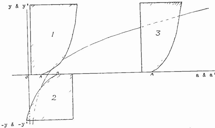
Fig. 14—Mechanical graph for solving transcendental equation.
