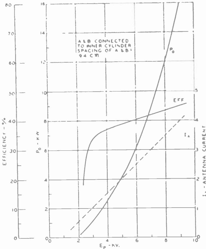
Fig. 12—Standing wave oscillator.  $\lambda = 5.5$  meters.
