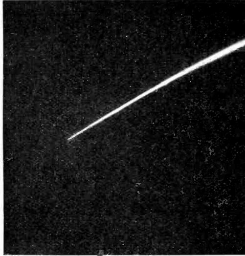
FIG. 11—Retardation of a slow (100-volt) cathode ray by screen charges.
