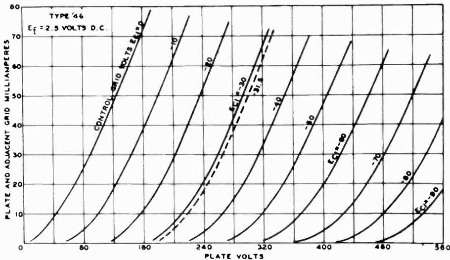
Fig. 14—Average plate characteristics. Class A operation.
