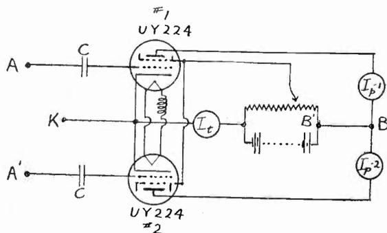
Fig. 9—Circuit for two tubes in push-pull arrangement.
