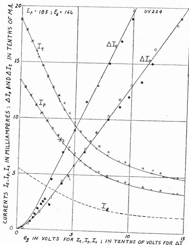
Fig. 6—Transrectification characteristics. On the  $I_p$  and  $I_t$  curves the small circles are points taken at 60 cycles, the crosses at 750 kilocycles. On the  $\Delta I_p$  and  $\Delta I_t$  curves the circles are at 60 cycles, the solid dots at 750 kilocycles.
