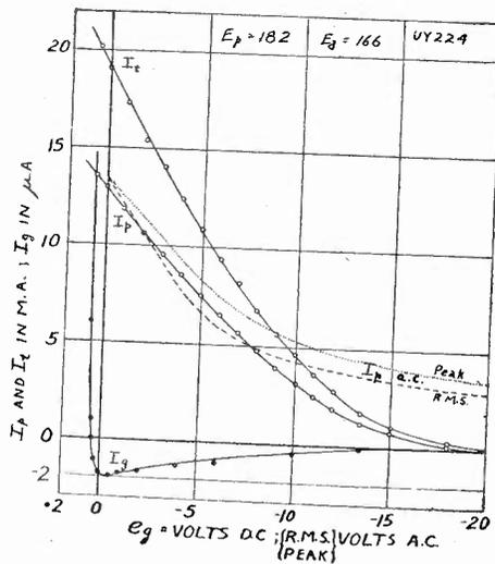
Fig. 3—Solid lines: static characteristics; broken lines: peak and root-mean-square transrectification characteristics.
