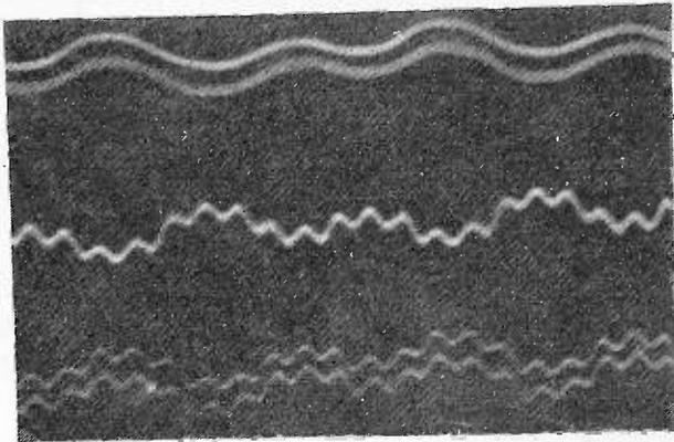
Fig. 12—Oscillograms of modulating and demodulated waves. The carrier was 75 megacycles. The smooth oscillograms at the top are the modulating wave (above) composed of 100 and 200 cycles with the demodulated wave below. The two waves at the bottom are the same as those at the top with 1000 cycles in addition. The center shows the two lower waves superposed.
