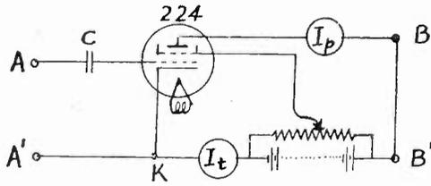
Fig. 1—Circuit for single tube voltmeter.
