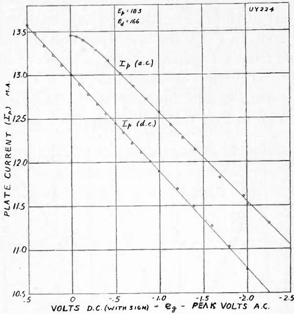
Fig. 4—Low voltage range of two of the characteristics of Fig. 3 replotted to bring out the relation between the direct-current and peak alternating-current curves.
