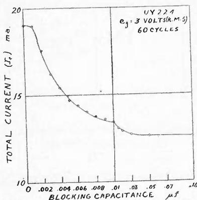
Fig. 7— $I_t$  as a function of blocking capacitance at 3 volts input.
