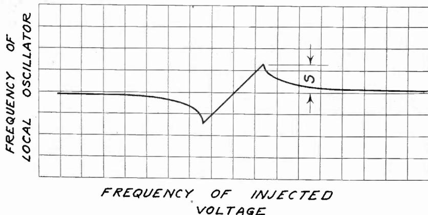
Fig. 2—Typical interlocking characteristic.
