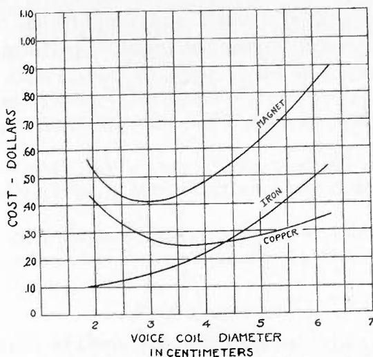
Fig. 6—Showing the effect of voice coil diameter upon the cost of the field magnet of an electrodynamic speaker.
