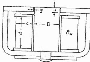
Fig. 5—Cross section of electrodynamic speaker field magnet.
