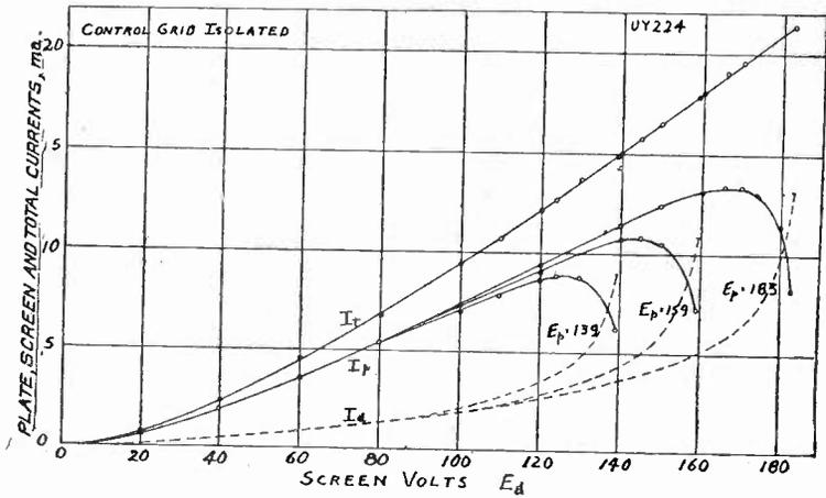
Fig. 2—Static characteristics of 24 tube with control grid isolated.
