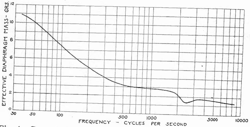
Fig. 4—General change in effective mass of the radiating surface of an electrodynamic speaker.
