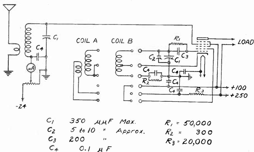
Fig. 7—Change-over circuit. The circuit used for comparison at high frequencies.
