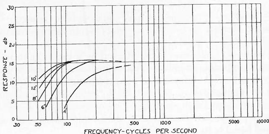
Fig. 2—Low-frequency response of an electrodynamic cone speaker with 48- by 48-inch baffle showing effect of diaphragms of from 4- to 12-inch diameters upon the low-frequency cut-off.
