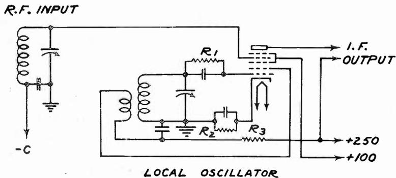
Fig. 1—Conventional pentagrid converter circuit.
