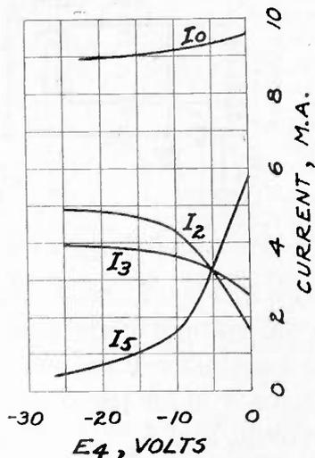
Fig. 4—Static curves for 2A7.  $I_0$ , total space current;  $I_2$ , current to grid no. 2 or oscillator anode;  $I_3$ , current to screen grids nos. 3 and 5;  $I_5$ , current to plate.  $E_4$  is the potential on the signal control grid no. 4.
