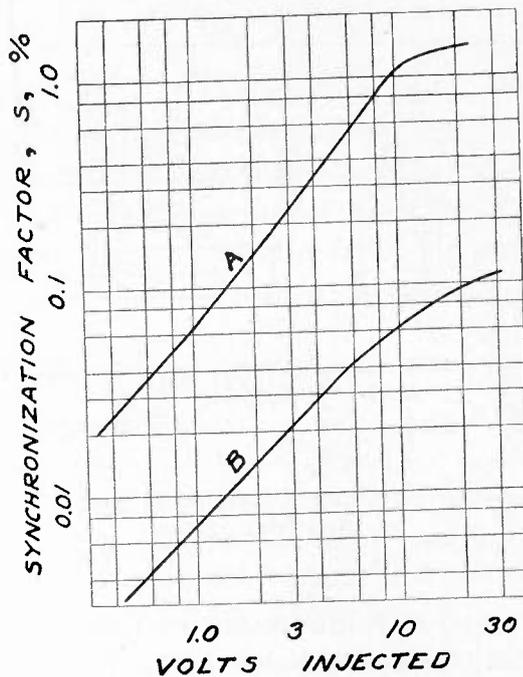
Fig. 6—Comparison of interlocking performance of circuits of Figs. 1 and 5. Synchronization factors; curve A, for circuit of Fig. 1; curve B, for circuit of Fig. 5.
