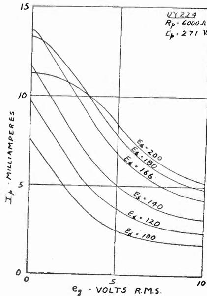
Fig. 8—Transrectification characteristics of a single tube circuit with 6000 ohms in the plate circuit.
