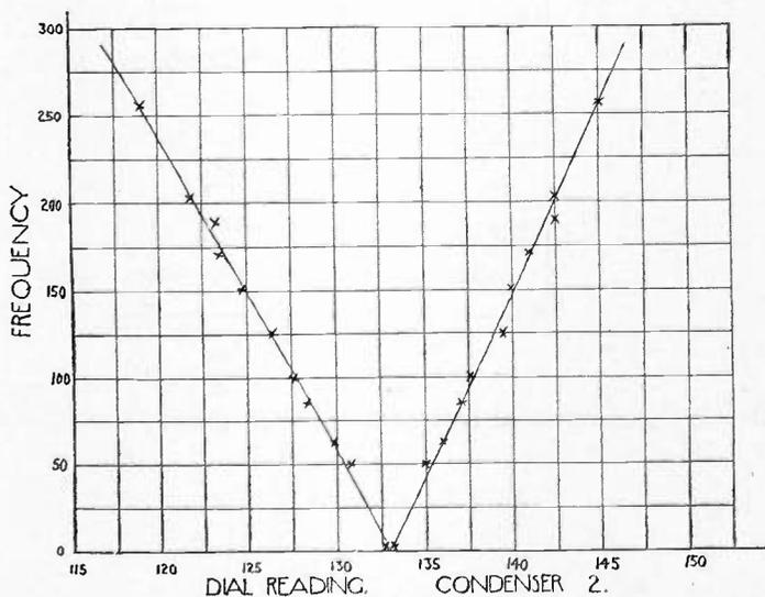
Fig. 2—Frequency calibration of oscillator.
