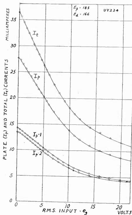
Fig. 11—Transrectification characteristics;  $I_p$  and  $I_t$  for two tubes; the curves  $I_p-1$  and  $I_p-2$  are the individual curves which when combined give the  $I_p$  curve.
