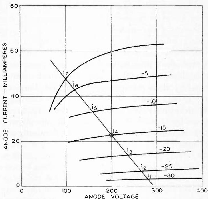
Fig. 1—Typical load line drawn on pentode characteristics
