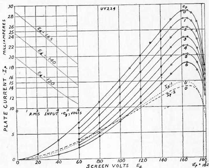
Fig. 10—Transrectification characteristics of two tubes with  $e_0$  in volts root-mean-square. The broken lines are the static characteristics for the separate tubes; their ordinates when added give the  $e_0 = 0$  curve for the two tubes.
