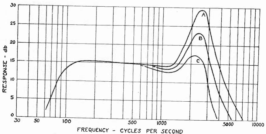
Fig. 1—Typical average response of an electrodynamic cone speaker with 48-inch by 48-inch flat baffle. Curve *A* is the response directly in line with speaker; curve *B* is  $30^\circ$  from center line; curve *C* is  $60^\circ$  from center line. Microphone 12 inches from cone.
