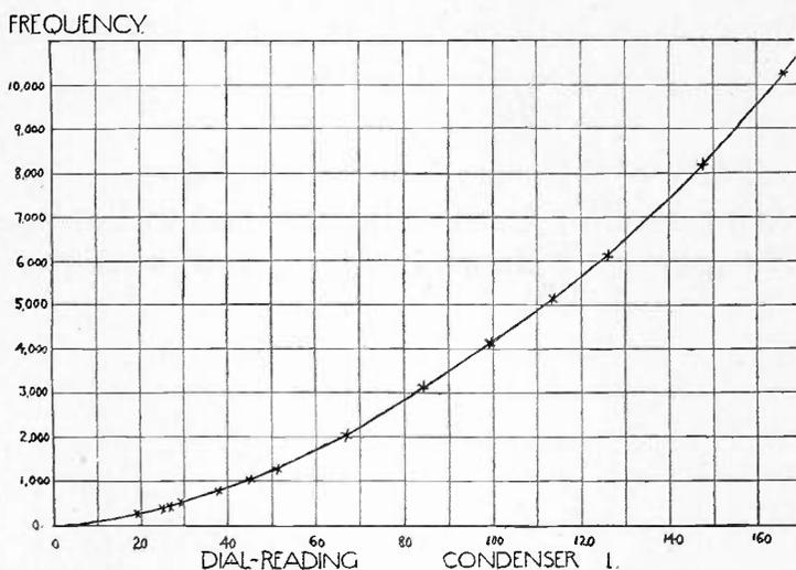
Fig. 1—Frequency calibration of oscillator.
