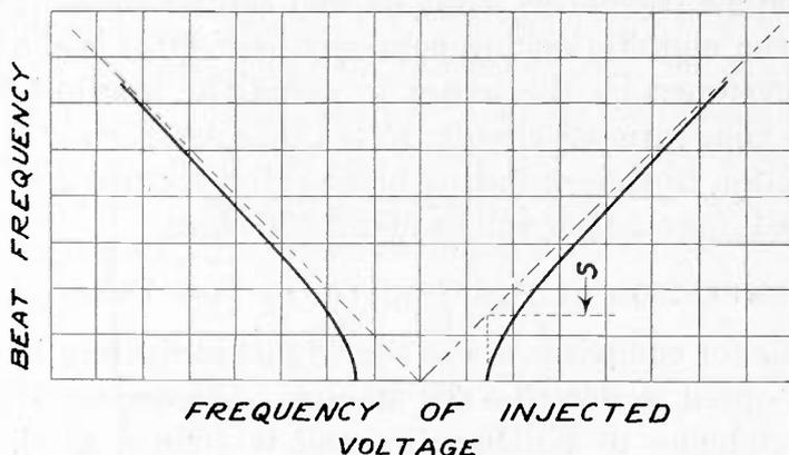
Fig. 3—Typical interlocking characteristic.
