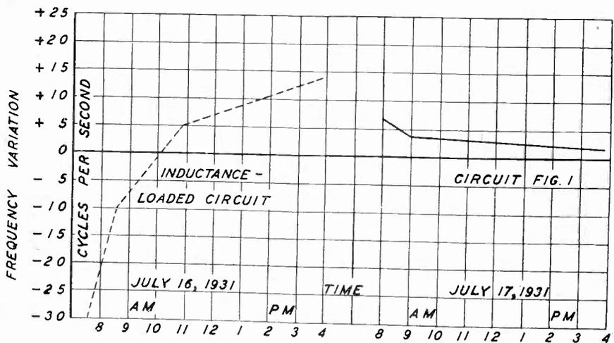
Fig. 2—Characteristic operation—790 kilocycles.
