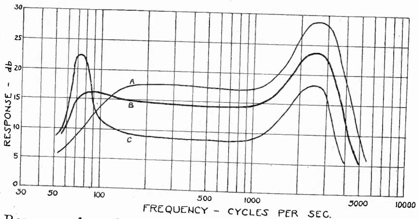
Fig. 3—Response of an electrodynamic cone speaker at various gap densities. Curve A is with gap density of 9600 gauss, curve B is with 7000 gauss, curve C is with 3500 gauss.
