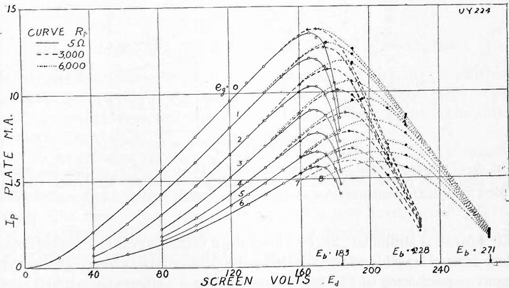
Fig. 5—Transrectification characteristics with indicated load resistance in plate circuit.  $e_g$  in volts root-mean-square.
