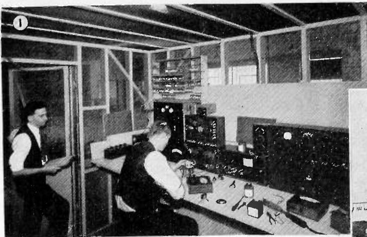
**1 NOISE TEST**—This test, made in a shielded chamber that eliminates external interference, reveals defects in internal resistor structure that cause noisy resistors. The accurately controlled Allen-Bradley processes result in such uniformity that quiet resistors can be consistently guaranteed.
