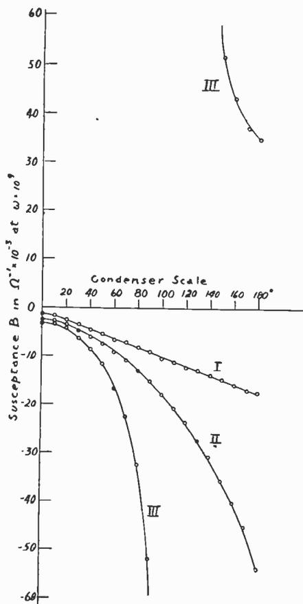
Fig. 15—Susceptance of 5-plate variable condenser. I. Ideal susceptance obtained by multiplying the capacitance measured at 400 meters by  $\omega = 10^9$ ; II. Susceptance measured at  $\omega = 10^9$ , short leads; III. Susceptance measured at  $\omega = 10^9$ , 3.5-centimeter leads.
