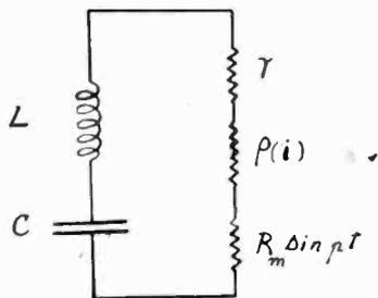
Fig. 1—Equivalent circuit of superregenerative receiver.
