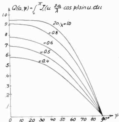
Fig. 8—Plot of the function  $Q(a, \psi) = \int_0^\pi J_1\left(u \cdot \frac{2a}{\lambda} \cos \psi\right) \sin u \cdot du$ .
