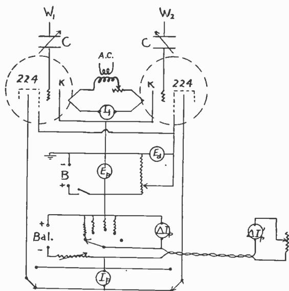
Fig. 6—Complete circuit diagram of the screen-grid voltmeter.  $W_1$  and  $W_2$  are the parallel wires. The series capacitances  $C$  consist, respectively, of two semicircular brass plates about 2 centimeters in diameter arranged on screws to permit moving the upper plate from contact with the lower one to a 4-centimeter separation. Operating voltages are:  $E_p = 150$  volts;  $E_d = 125$  volts (to give maximum plate current).
