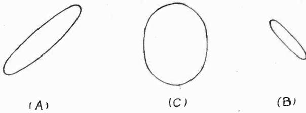
Fig. 24—Lissajous figures at the synchronization.
