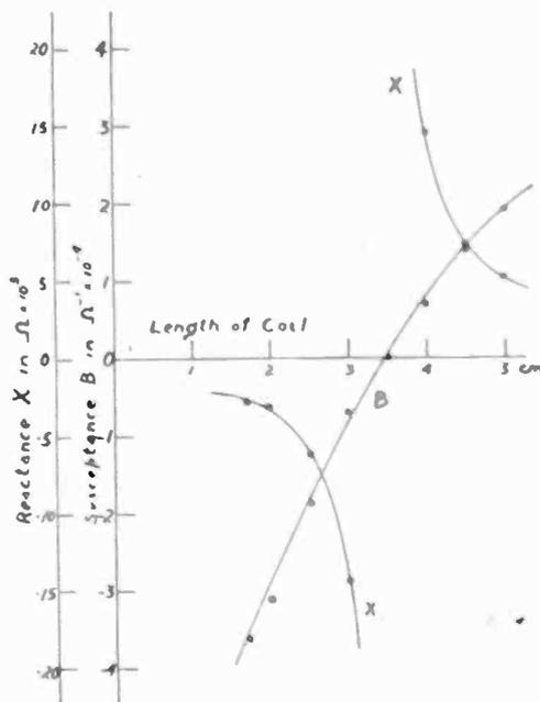
Fig. 16—Reactance and susceptance of single layer coil of variable length.
