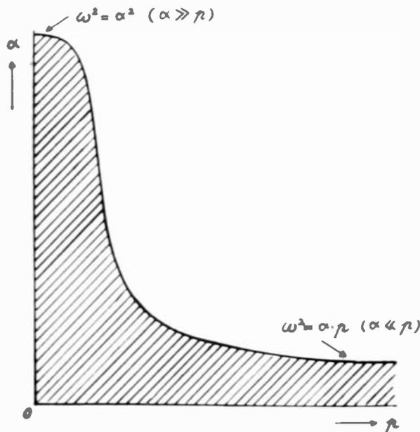
Fig. 3—Stable (shaded) and unstable (unshaded) regions given by a criterion.
