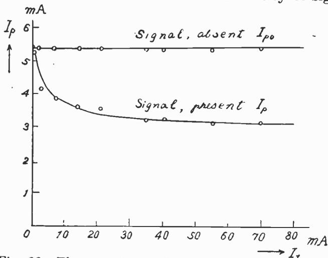
Fig. 33—The variation in the plate current due to the intensity of signal.
