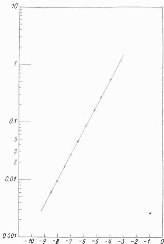
Fig. 3—Anode current  $i$  milliamperes (vertical) versus grid voltage  $V$  (horizontal) for Philips vacuum tube E 452 T. Points measured, curve calculated from  $i = 28.7 \cdot e^{0.995V}$ ;  $R = 0$ ;  $V_{an} = 200V$ ;  $V_{screen} = 100V$ .
