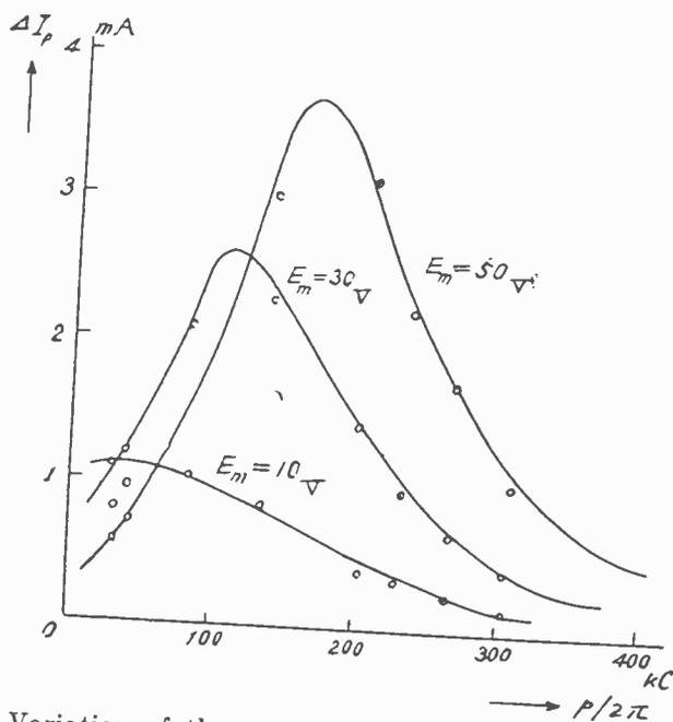
Fig. 36—Variation of the sensitivity due to the quenching action.
