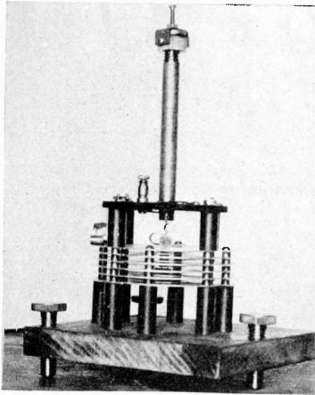
Fig. 5—The multicellular electrometer which was used as a radio-frequency wattmeter.
