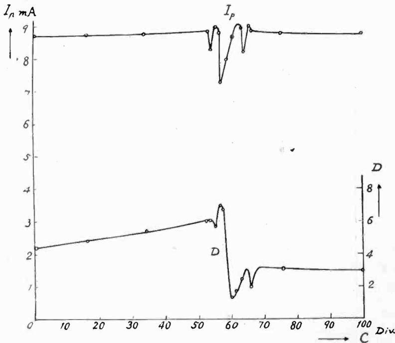
Fig. 25—Synchronization for a modulated wave.
