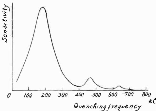
Fig. 37—Variation of the sensitivity due to the quenching frequency at the constant quenching voltage.
