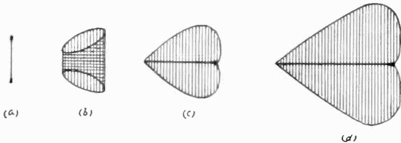
Fig. 14—Lissajous figures at  $E_p = 103V$ ,  $p/2\pi = 550$  kilocycles.
