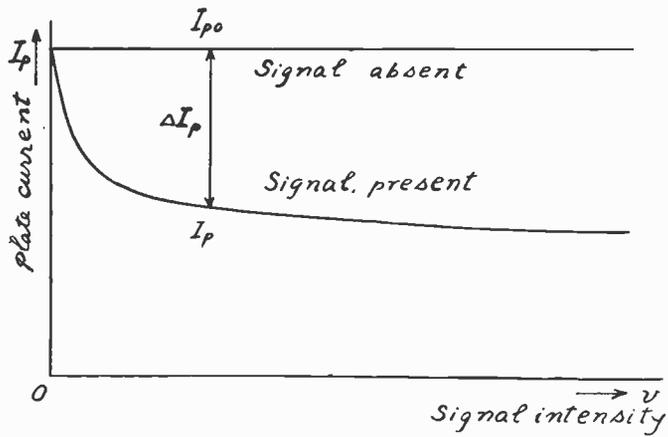
Fig. 40—Variation of the plate current due to the intensity of signal.
