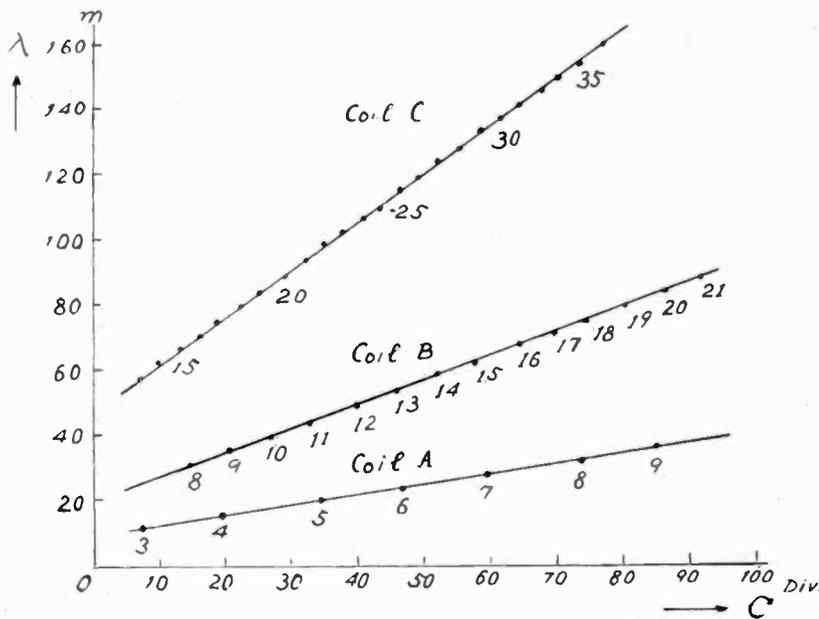
Fig. 32—Calibration curves of a wave meter by means of a superregenerative receiver.
