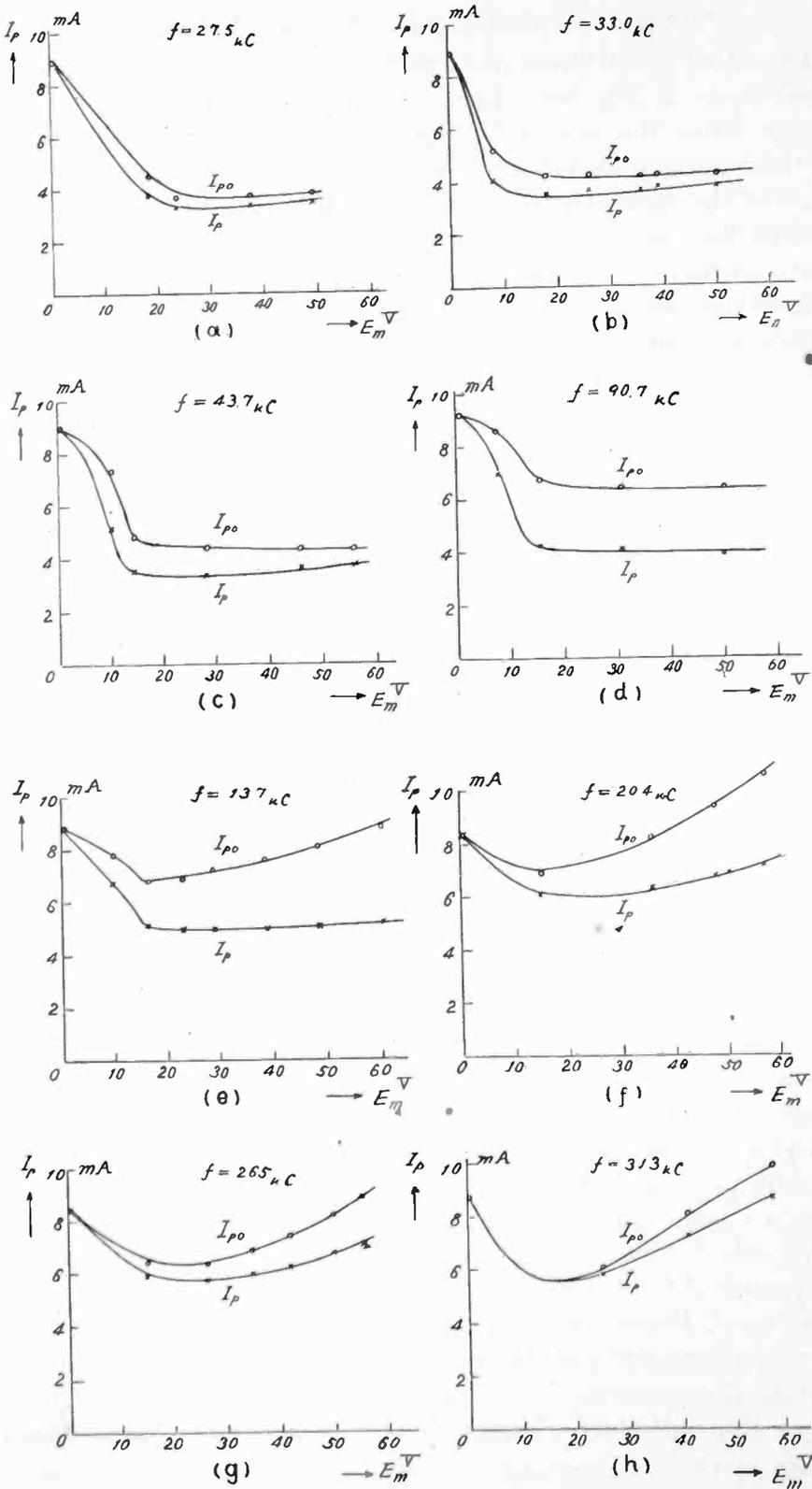
Fig. 35 (a)-(h)—Effects of the quenching voltage on the sensitivity at the various quenching frequencies.
