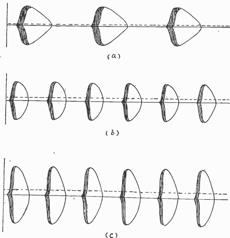
Fig. 39—Various modes of amplification by superregeneration.
