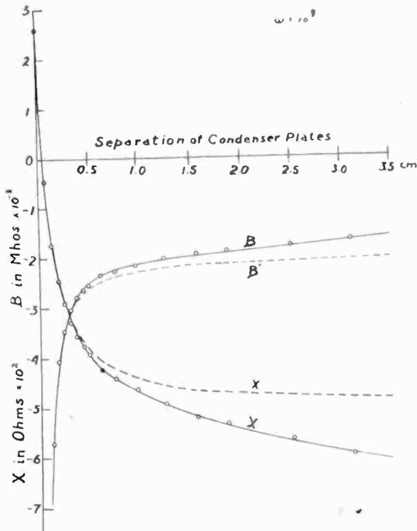
Fig. 12—Input reactance  $X$  and susceptance  $B$  of the symmetrical voltmeter as a function of the separation of the plates of the series capacitances  $C$ .  $X'$  and  $B'$  give the input reactance and susceptance, respectively, corrected to what they would be for changes only in the capacitances  $C$ , not including the change in inductance due to the shortening of the leads as the condenser plates are separated.
