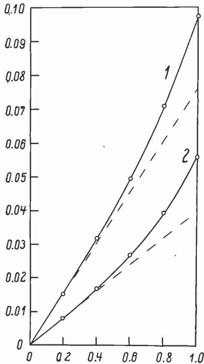
Fig. 5—Vertical axis, anode current component  $i_p$  (milliamperes). Horizontal axis, depth of modulation  $M$ . Points measured, curves calculated. Curve 1 for tube E 452 T. Curve 2 for tube E 446;  $R = 0.1$  megohm;  $V_{an} = 200V$ ;  $V_{screen} = 100V$ .
