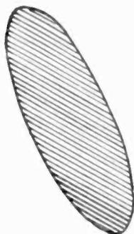
Fig. 28—Lissajous figure in the synchronization of the superregenerative receiver.
