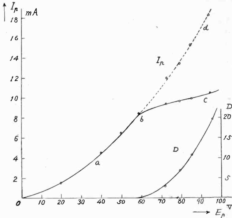
Fig. 8—Static characteristic of the ultra-short-wave oscillator.
