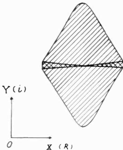
Fig. 6—The theoretical form of the Lissajous figure.
