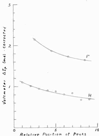
Fig. 19—Relative amplitudes of fundamental and harmonic maxima on the parallel wires. The abscissa scale is in units of the harmonic half wavelength.
