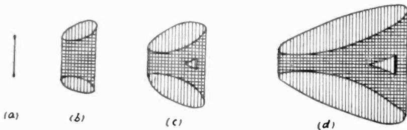
Fig. 15—Lissajous figures at  $E_p = 109V$ ,  $p/2\pi = 910$  kilocycles.
