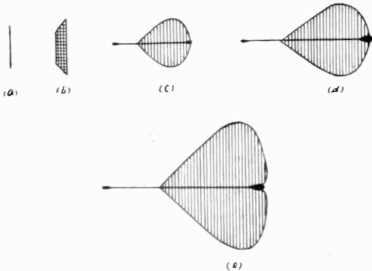
Fig. 13—Lissajous figures at  $E_p = 88V$ ,  $p/2\pi = 90$  kilocycles.
