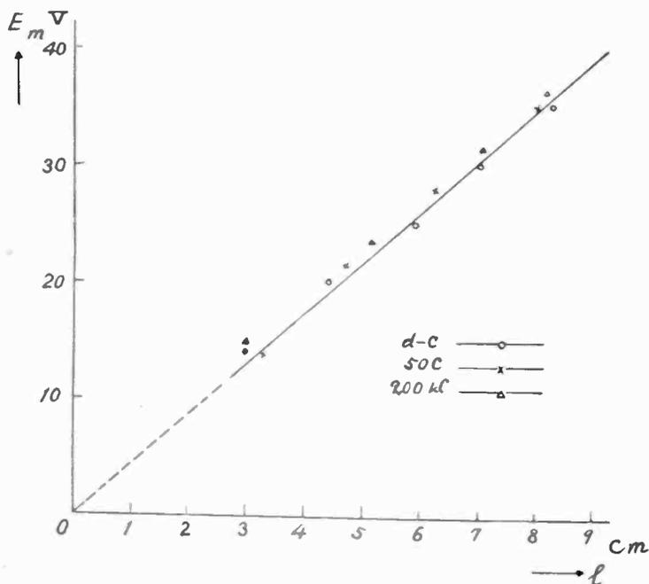
Fig. 9—Calibration curve of a Braun tube as a crest voltmeter.
