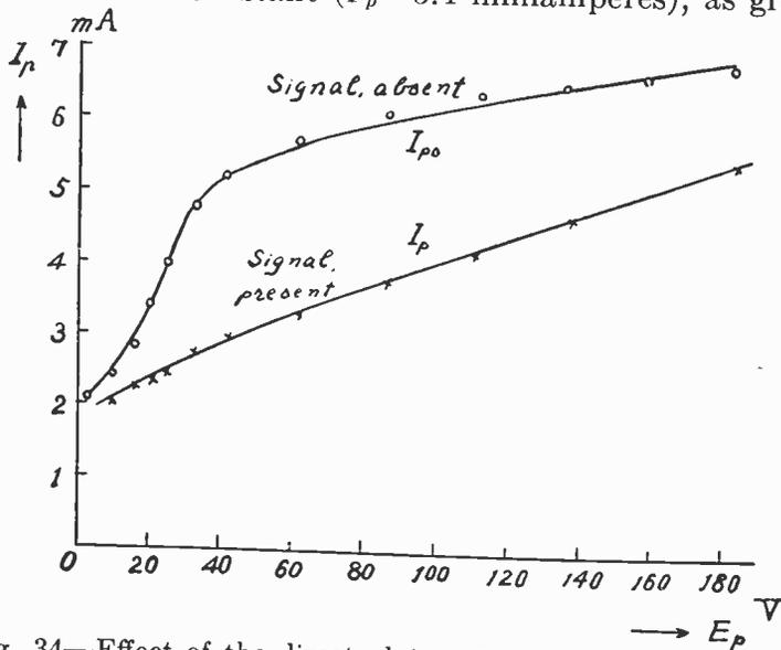
Fig. 34—Effect of the direct plate voltage on the plate current.
