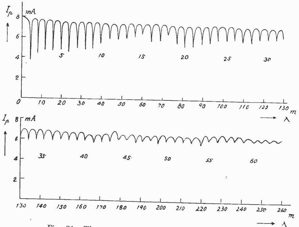
Fig. 31—The variation of the plate current with the wavelength of the signal wave.
