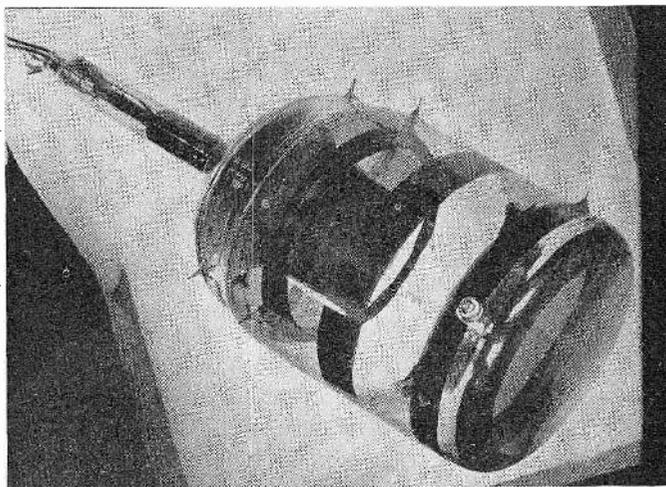
Fig. 16—Pickup tube utilizing magnetically focused electron picture.
