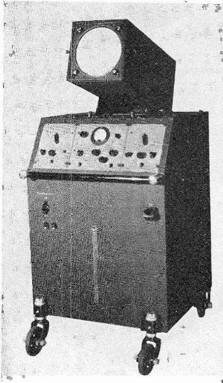
Fig. 1—Front view of cathode-ray oscillograph.
