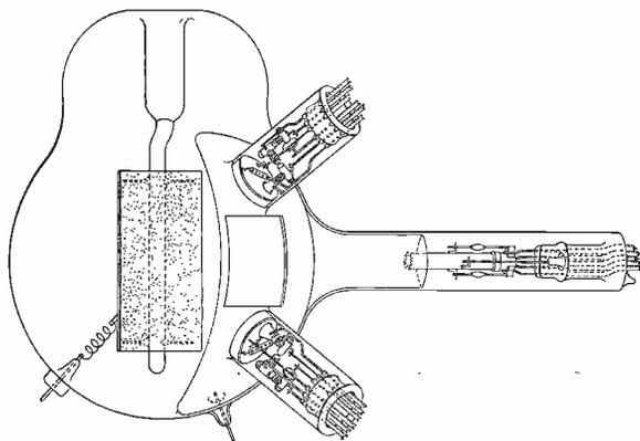
Fig. 12—Diagram of signal multiplier Iconoscope.
