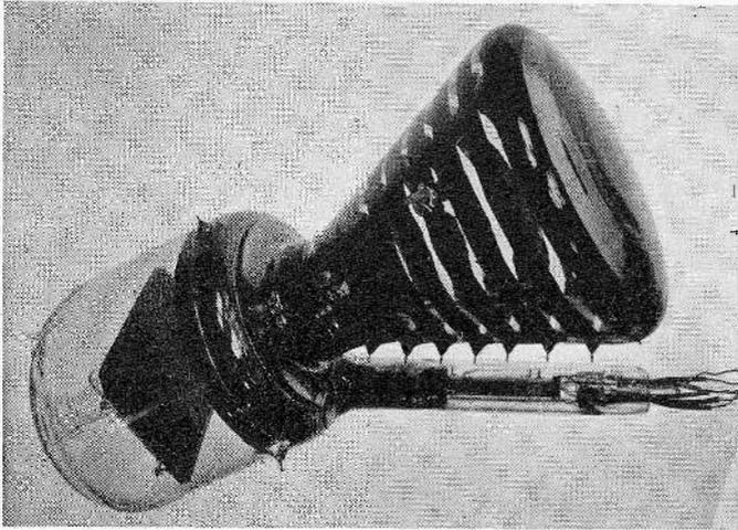
Fig. 14—Pickup tube using electrostatically focused electron picture.
