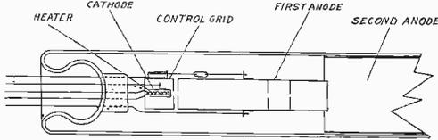
Fig. 3—Diagram of electron gun.
