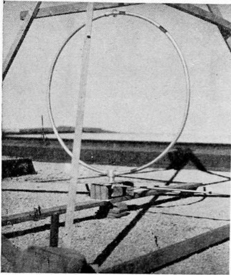
Fig. 18—Six-megacycle shielded-loop antenna for static reduction at ground stations.
