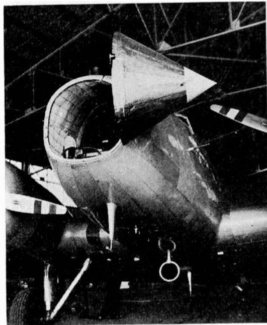
Fig. 8—Copper-covered wooden nose for testing loop antennas. Sharp point (white fabric) at end of nose used to reduce ice accumulation.
