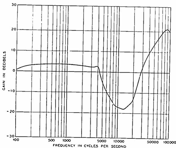
Fig. 7—Gain-frequency characteristic of corrective network inserted in signal feedback path.
