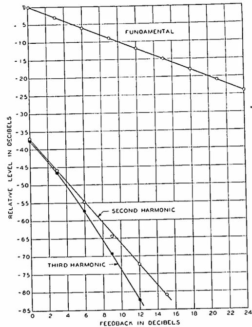
Fig. 11—Effect of feedback upon receiver distortion. Modulation held to a constant value of  $\pm 7$  kilocycles.
