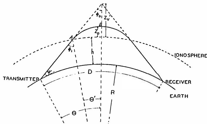
Fig. 6—Transmission through curved ionosphere.  $z_v'$  = height of equivalent triangular path,  $z_0$  = true height of reflection, at the level where  $\mu' = \sin \phi_1 (1 - z_0 / (R + h))$ ,  $R$  = radius of earth,  $D$  = distance of transmission.
