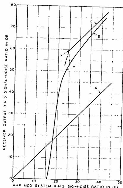
Fig. 16—Theoretical comparison of signal-to-noise ratios obtained at 25-decibel feedback (curve *B*) with amplitude-modulated system (curve *A*) and ideal limiter system with deviation ratio = 31.1 (curve *C*). Point *X* = threshold of noise improvement for limiter system. Point *Y* = point where "crackling" first became evident in the presence of  $\pm 124.5$ -kilocycle modulation.
