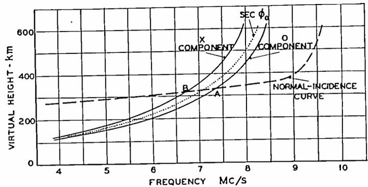
Fig. 10—Transmission curve, including effect of earth's magnetic field at level of reflection. Dotted line = secant-law curve ( $f' = f \sec \phi_0$ ) for the given distance  $D$  and wave frequency  $f'$ . Dashed line =  $(z_v, f)$  curve for the  $o$  component, this being the component which, at vertical incidence is a measure of the ionization density  $N$ . The  $o$  component of the frequency  $f'$  over the given distance is reflected at  $A$ , and the  $x$  component at  $B$ .
