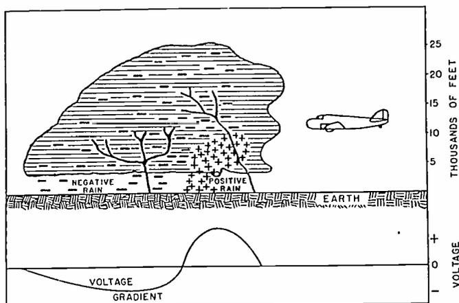
Fig. 3—Distribution of electrical charges in a thundercloud of the heat type.
