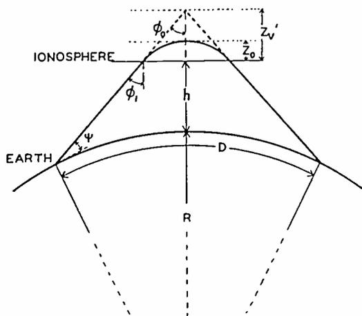
Fig. 4—Geometric relation for determining  $\phi_1$  in terms of transmission distance  $D$  for a curved earth and flat ionosphere. In this and in Figs. 5 and 6 the distance between the ionosphere and the earth is greatly exaggerated for clarity of representation.
