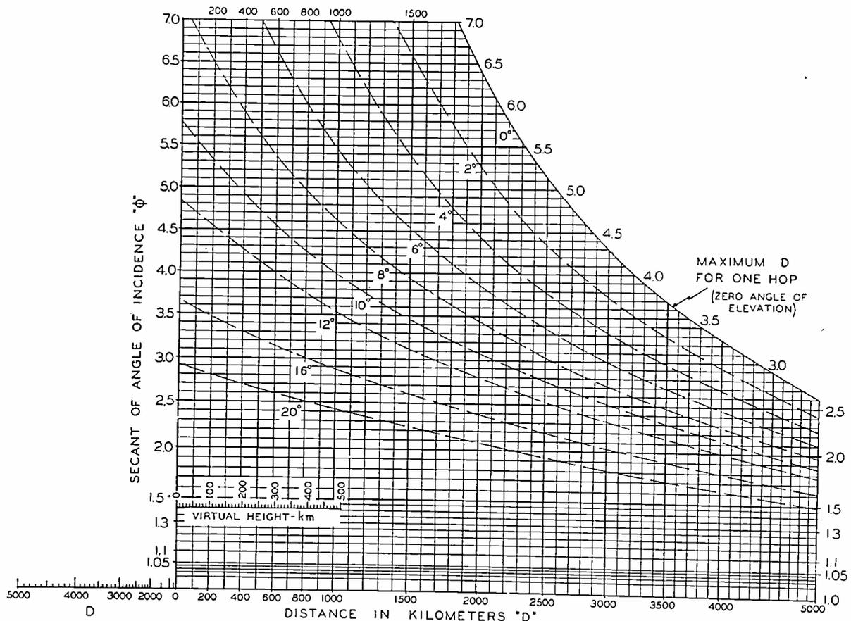
Fig. 15—Alignment chart for determining  $\sec \phi_0$  and  $\psi$ , the angle which the ray makes with the horizontal at the transmitter or receiver. The curved dashed lines are lines of equal  $\psi$ .
