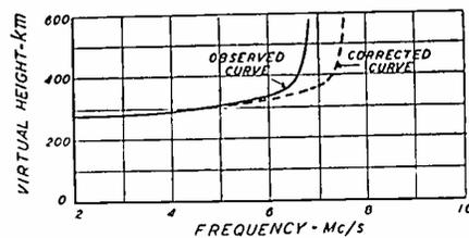
Fig. 8— $(z_v, f)$  curve corrected for a given distance (2000 kilometers) for the effect of the earth's curvature.
