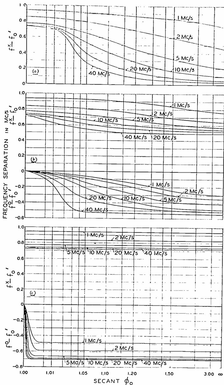
Fig. 11— $f^x - f_0'$  and  $f_0^x - f_0'$  plotted against  $\sec \phi_0$ .  $f^x$  = frequency whose  $x$  component is reflected at the same level as is the  $o$  component of  $f^0$ .  $f_0^x = f' \cos \phi_0$ .  $H = \sqrt{H_T^2 + H_L^2} = 0.5$  gauss. The value of  $f'$  is given, in megacycles, on each curve.
