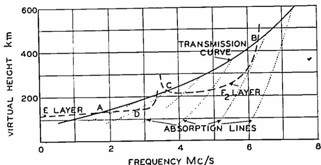
Fig. 13—Absorption lines on transmission curve. Dashed line =  $(z_v, f)$  curve. Dotted lines = absorption lines. E reflection takes place at point A and  $F_2$  reflection at point B.  $F_2$  reflection at C is shielded by the E layer at D.
