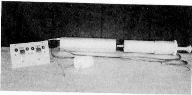
Fig. 16—Plane discharge-cartridge assembly. From left to right are shown the pilot's control panel for two cartridges, the socket for mounting on rear of the plane, and the cartridge with its plunger extended. The black flexible resistor lies in front of the socket and cartridge as does the fine wire which terminates at the white-paper wind cone in the foreground.
