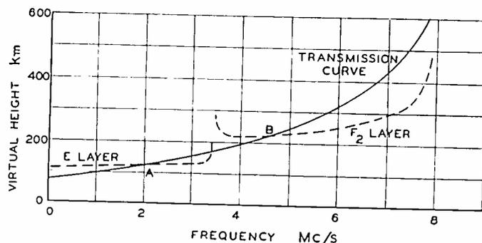
Fig. 12—Transmission by way of both E and  $F_2$  layers.
