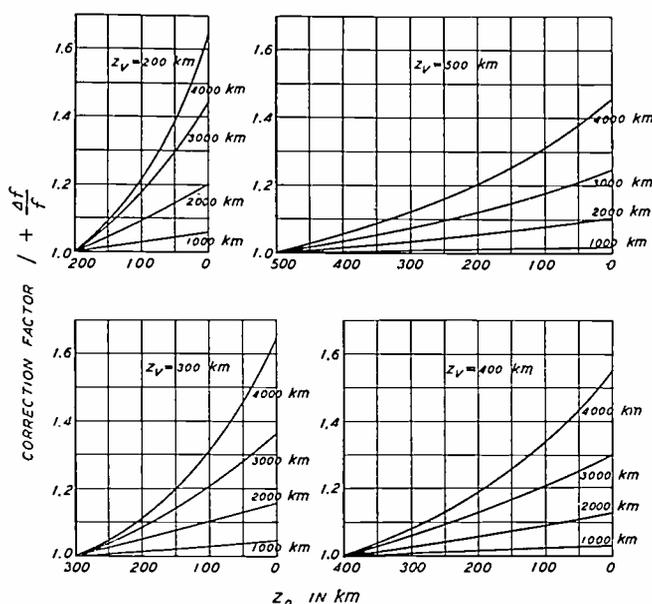
Fig. 9—Approximate factors by which the equivalent vertical-incidence frequency  $f$  must be multiplied to give the frequency  $f'/\sec \phi_0$  which is to be used in conjunction with the log sec  $\phi_0$  curves.
