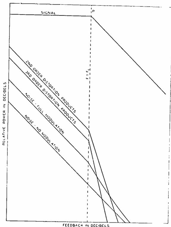
Fig. 3—Theoretical manner in which components of receiver output are modified by feedback. Modulation level at transmitter is assumed to be increased by the feedback factor up to point *B*, and subsequently to remain fixed.
