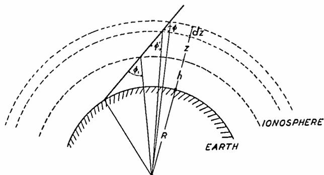
Fig. 5—Variation, with height, of the angle that a straight line makes with the normal to the earth's surface.
