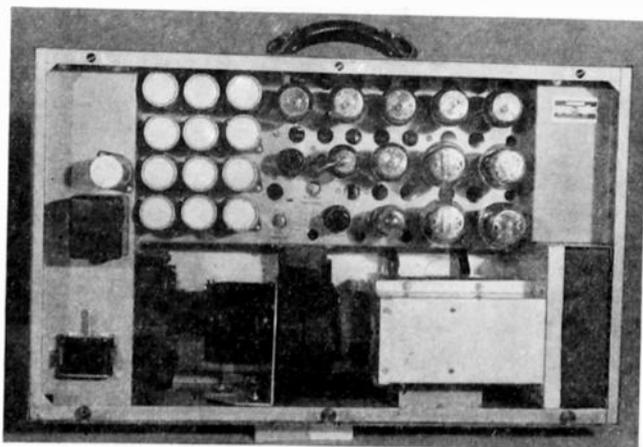
Fig. 10—Power-supply unit—tube side.
