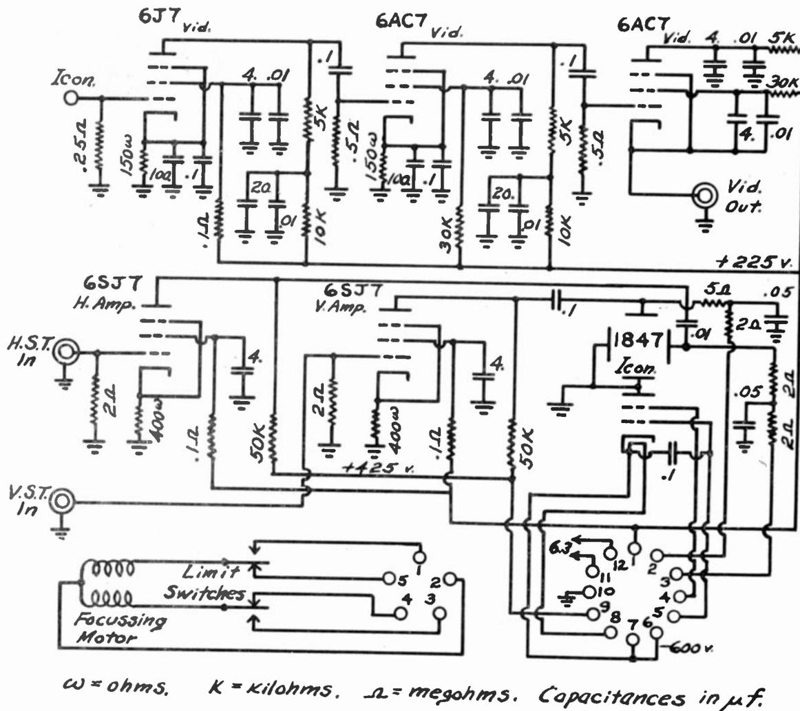
Fig. 1—Schematic wiring diagram of camera.
