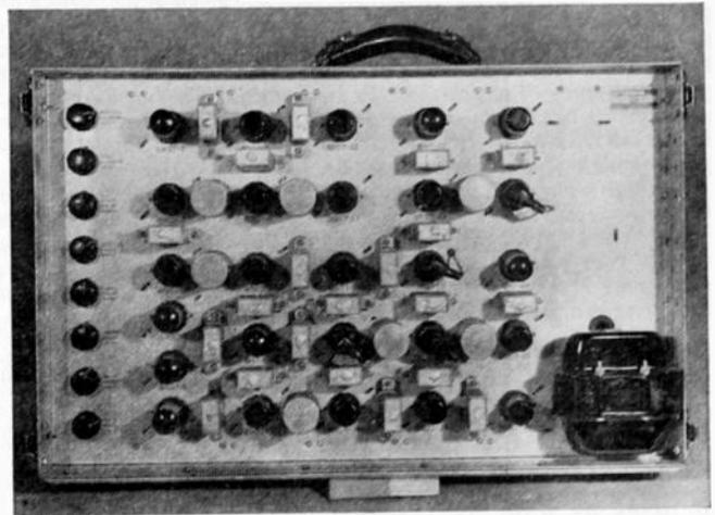
Fig. 14—Orthicon shaping unit—tube side.
