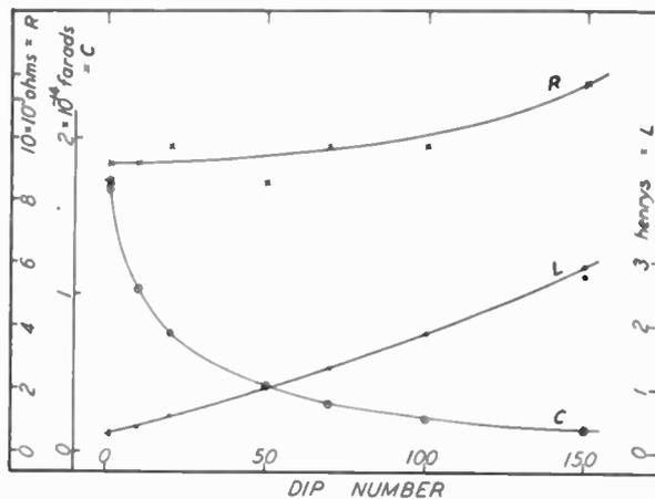
Fig. 4—Variation of inductance ( $L$ ), capacitance ( $C$ ), and resistance ( $R$ ) as a function of the length of the liquid column.
