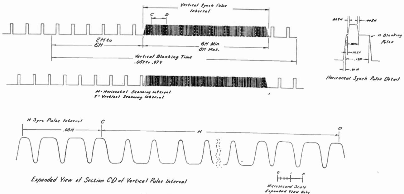
Fig. 2—DuMont synchronizing signal.
