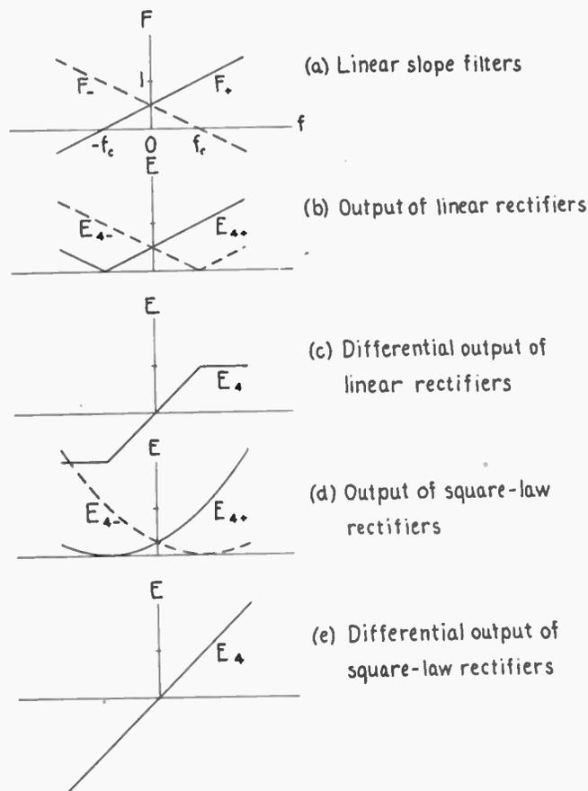
Fig. 2—The essential properties of balanced frequency detectors.
