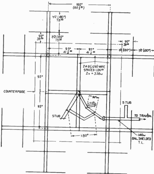
Fig. 3—Developed circuits for experimental cone-of-silence marker antenna system for St. Hubert range station.
