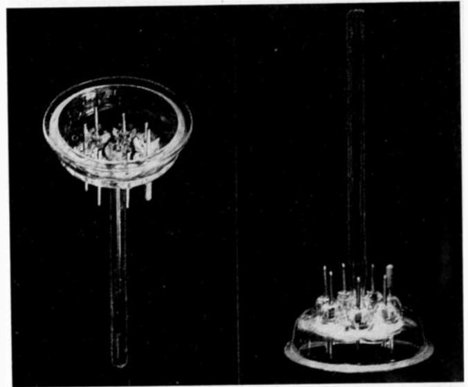
Fig. 3—Molded-flare stem as used on the RCA-826 and RCA-829.
