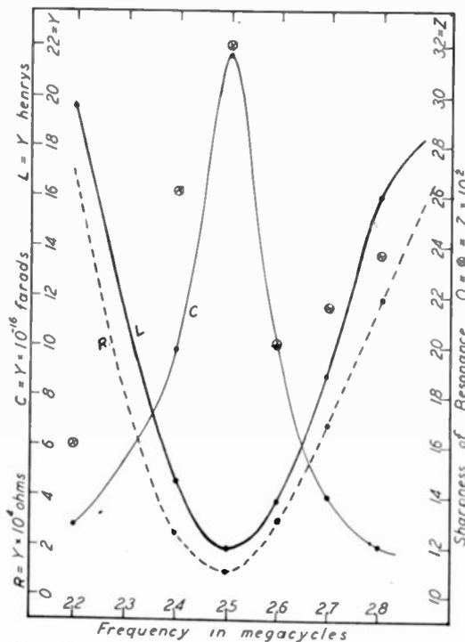
Fig. 5—Variation of inductance ( $L$ ), capacitance ( $C$ ), resistance ( $R$ ), and sharpness of resonance ( $Q$ ) as a function of frequency. Reflector set for the 100th dip.
