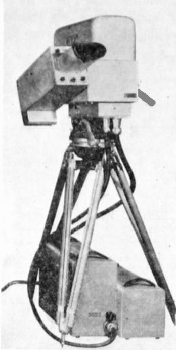
Fig. 6—Camera equipment (iconoscope).
