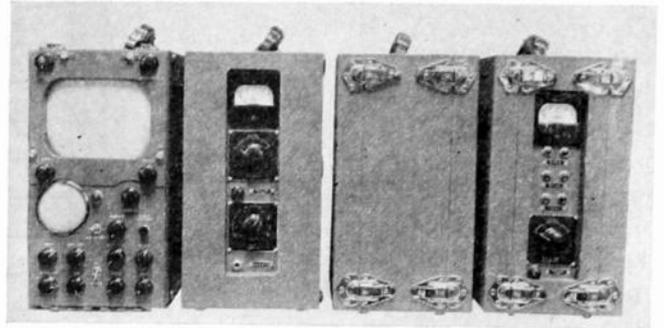
Fig. 4—Camera control, power-supply, shaping and pulse units. The last two constitute the synchronizing generator.
