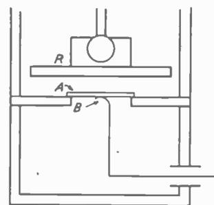
Fig. 1—Combination "quartz-plate and liquid-column" resonator.
