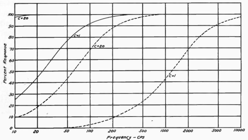
Fig. 16—Comparison of low-frequency response: constant-voltage source (dotted curves) and  $R_c/R_t = 50$  (solid curves).
