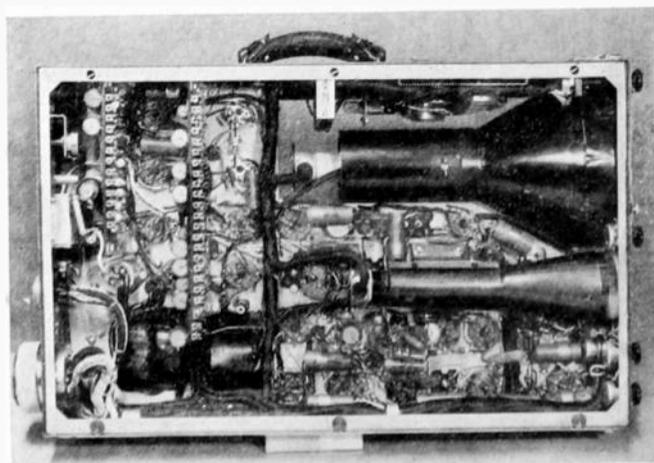
Fig. 8—Orthicon camera control unit—circuit side.
