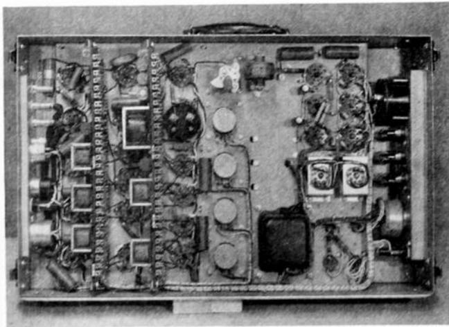
Fig. 13—Orthicon pulse unit—circuit side.
