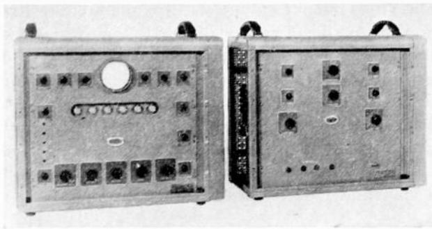
Fig. 3—Synchronizing generator with front cover removed.
