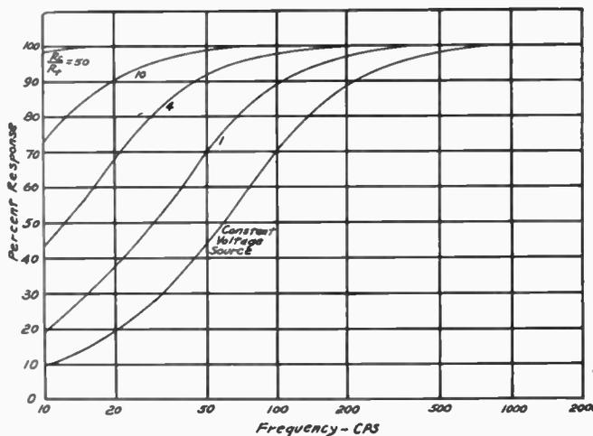
Fig. 15—Variation of low-frequency response with ratio of  $R_c$  to  $R_t$  ( $R_t = 75$  ohms).
