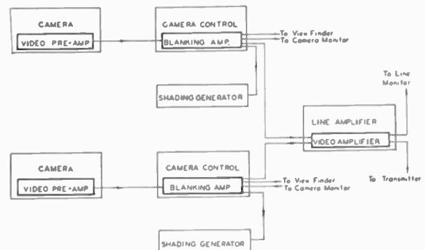
Fig. 5—Diagram of video system.
