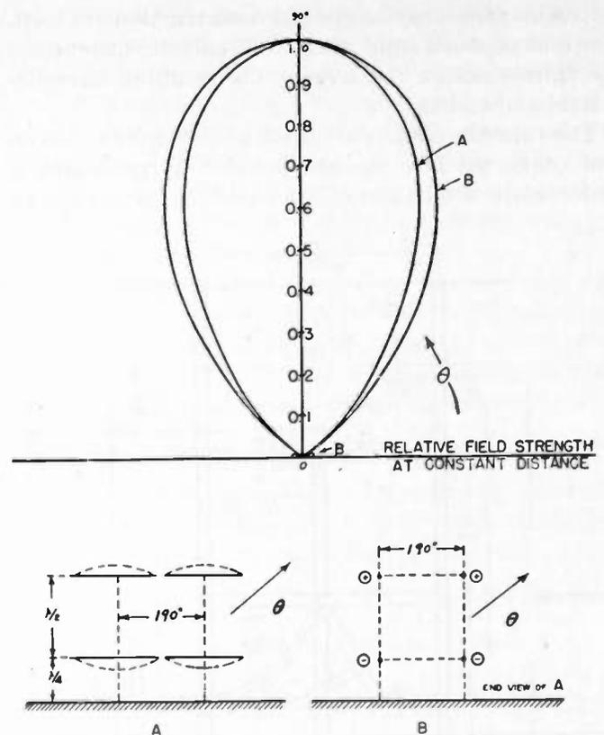
Fig. 1—Vertical radiation patterns for Department of Transport cone-of-silence marker antenna.
