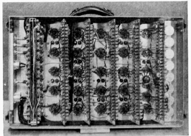
Fig. 15—Orthicon shaping unit—circuit side.
