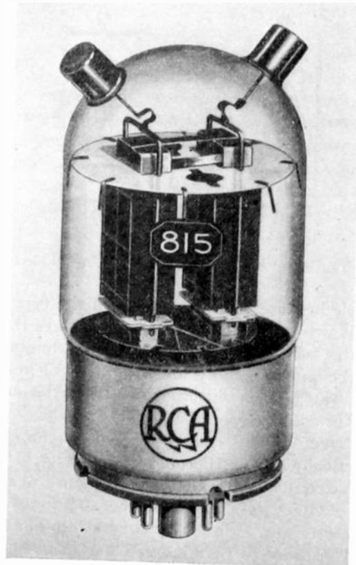
Fig. 5—A push-pull beam transmitting tube having oxide-coated cathodes and a total plate dissipation of 20 watts. It may be operated at full rating to frequencies as high as 150 megacycles.
