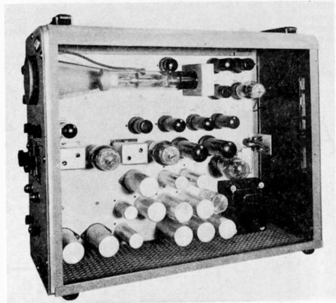
Fig. 14—Line amplifier, tube side.
