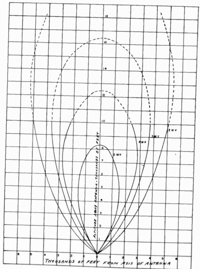
Fig. 4—Measured signal potentials induced in plane's marker antenna.
