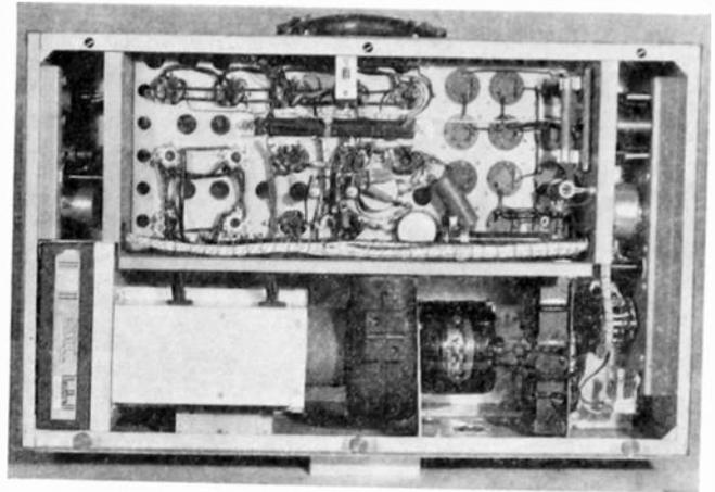
Fig. 11—Power-supply unit—circuit side.
