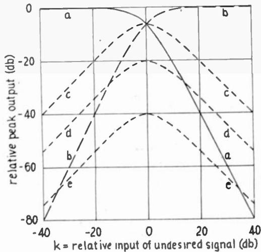
Fig. 12—The relative peak output of the individual components in the case of square-law rectifiers.
