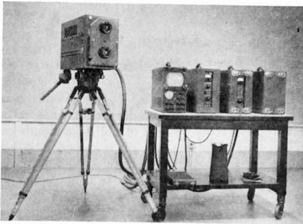
Fig. 2—Orthicon portable television equipment.
