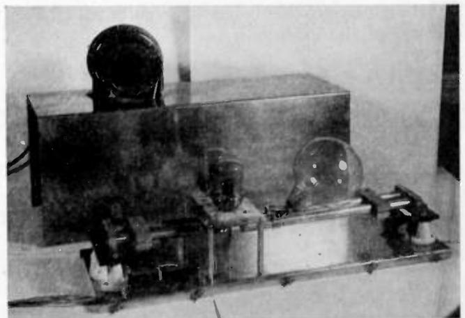
Fig. 8—A push-pull oscillator using RCA-826's.
