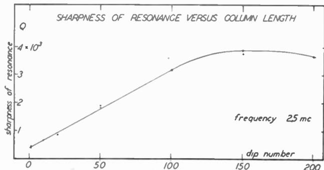
Fig. 3—Sharpness of resonance ( $Q$ ) as a function of the length of the liquid column.
