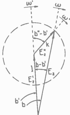
Fig. 3—The vector sum of two frequency-modulated signals.
