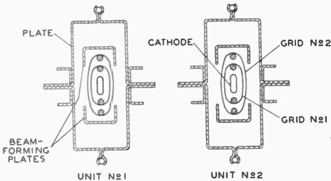
Fig. 2—Horizontal cross section of the RCA-829 electrodes.
