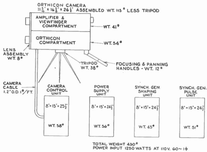
Fig. 1—Schematic diagram of orthicon television equipment.
