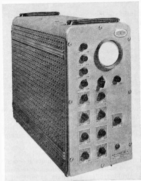
Fig. 11—Shading generator.
