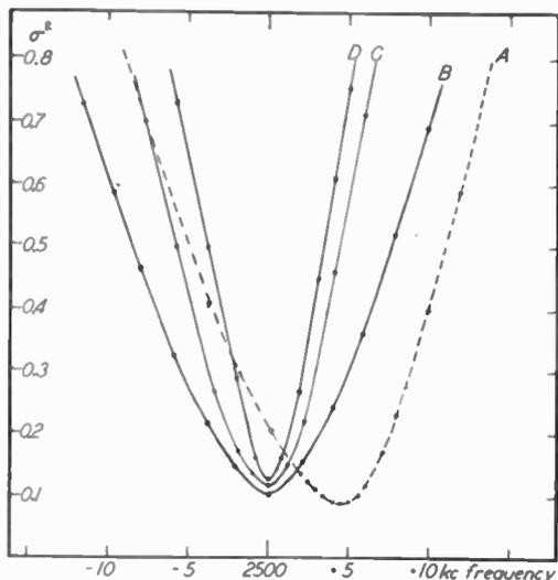
Fig. 2—Crevasse curves for quartz plate, and for combination resonator with various column lengths. A, mounted plate; B, C, and D are for the 1st, 10th, and 20th dips, respectively.
