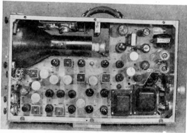
Fig. 9—Camera control unit—tube side.
