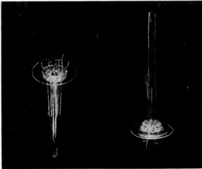
Fig. 6—Glass-button stem as used on the RCA-815.
