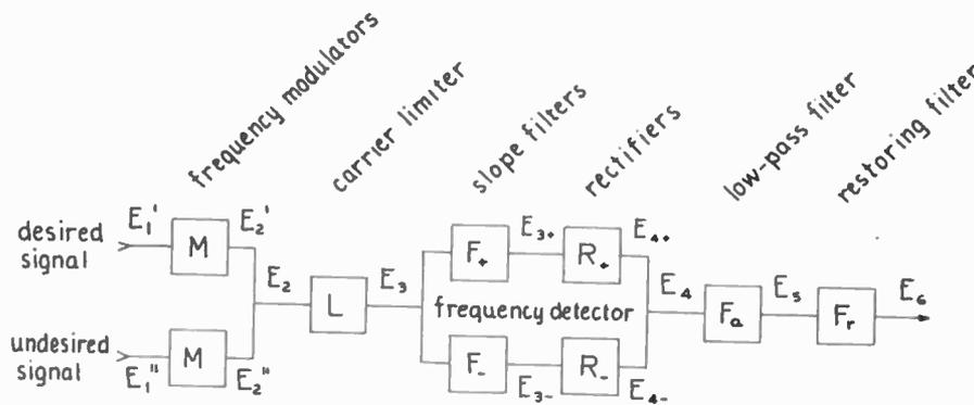
Fig. 1—Frequency-modulation system with interference between two signals in the same frequency band.
