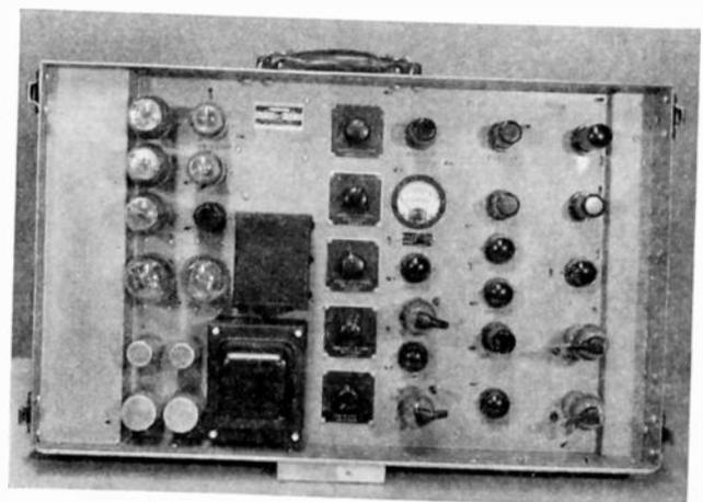
Fig. 12—Orthicon pulse unit—tube side.
