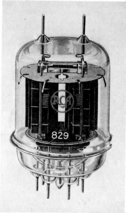
Fig. 1—A push-pull beam transmitting tube having oxide-coated cathodes and a total plate dissipation of 40 watts. It may be operated at full rating to frequencies as high as 200 megacycles.
