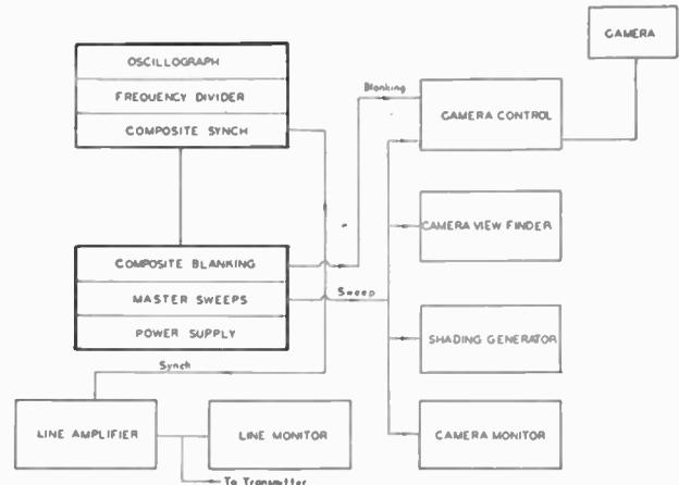
Fig. 4—Diagram of scanning and synchronizing system.
