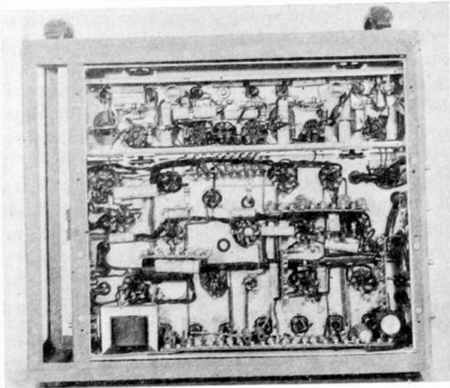
Fig. 8—Camera-control unit, wiring side.
