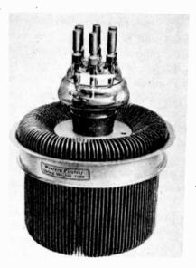
Fig. 1-Western Electric 389AA vacuum tube.
