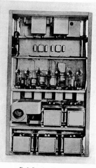
Fig. 8-Rear view of power unit.
