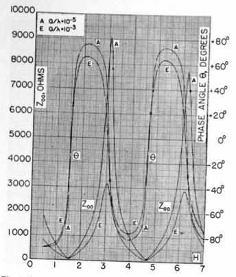
Fig. 6—The magnitude of the input self-impedance  $|Z_{00}|$  and its phase angle  $\theta$  as functions of  $H = 2\pi k/\lambda$  with  $a/\lambda$  as parameter. Values at  $H = n\pi/2$  are indicated by a small circle.
