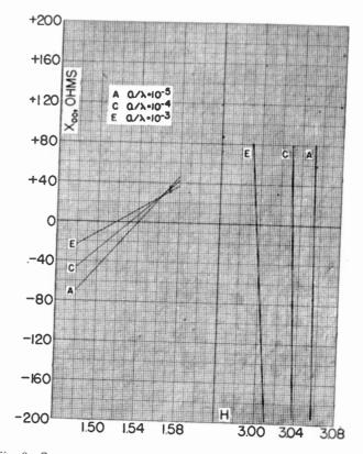
Fig. 8—Same as Fig. 4 for low-reactance ranges. Resonant points at intersections with the horizontal axis where  $X_{00}$  vanishes.
