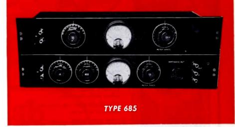
TYPE 685 An unusually flexible, universal gain measuring instrument for rapid and accurate measurement of overall gain, frequency response and power output of audio amplifiers, this assembly has a useful frequency range from 30 to 17,000 cycles.
