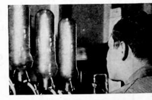
FLASH FILAMENT TESTER checks filaments before tubes are assembled and pumped. Here tubes are placed under a temporary vacuum, heated to much higher temperatures than will ever be required in normal use. Only perfect filaments reach the final stages of manufacture.
