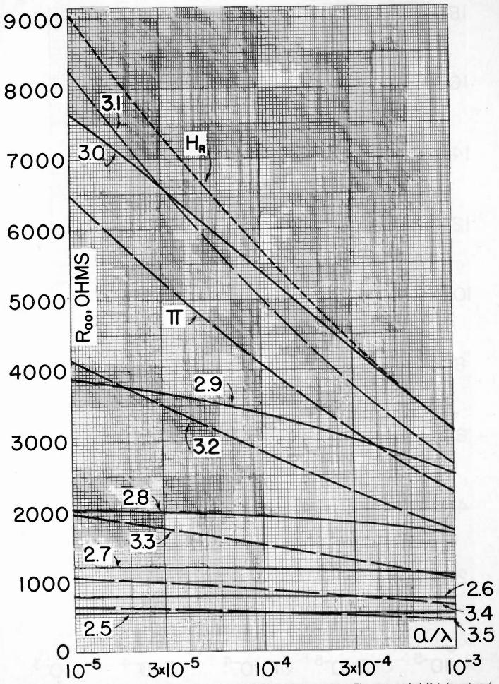
Fig. 9—The input self-resistance  $R_{00}$  as a function of  $a/\lambda$  with  $H = 2\pi h/\lambda$  as parameter. The curve marked  $H_r$  is for values of  $R_{00}$  when H is adjusted to antiresonance near  $H = \pi$  for indicated values of  $a/\lambda$ .
