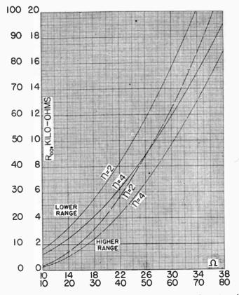
Fig. 14—The input self-resistance  $R_{00}$  at the n=2 and n=4 antiresonant lengths as functions of  $\Omega = 2 \log (2h/a)$ .
