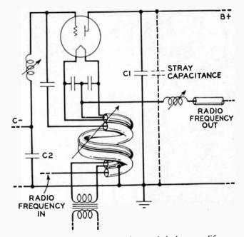
Fig. 3--Schematic diagram of grounded plate amplifier.
