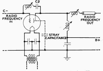
Fig. 2-Schematic diagram of conventional amplifier.
